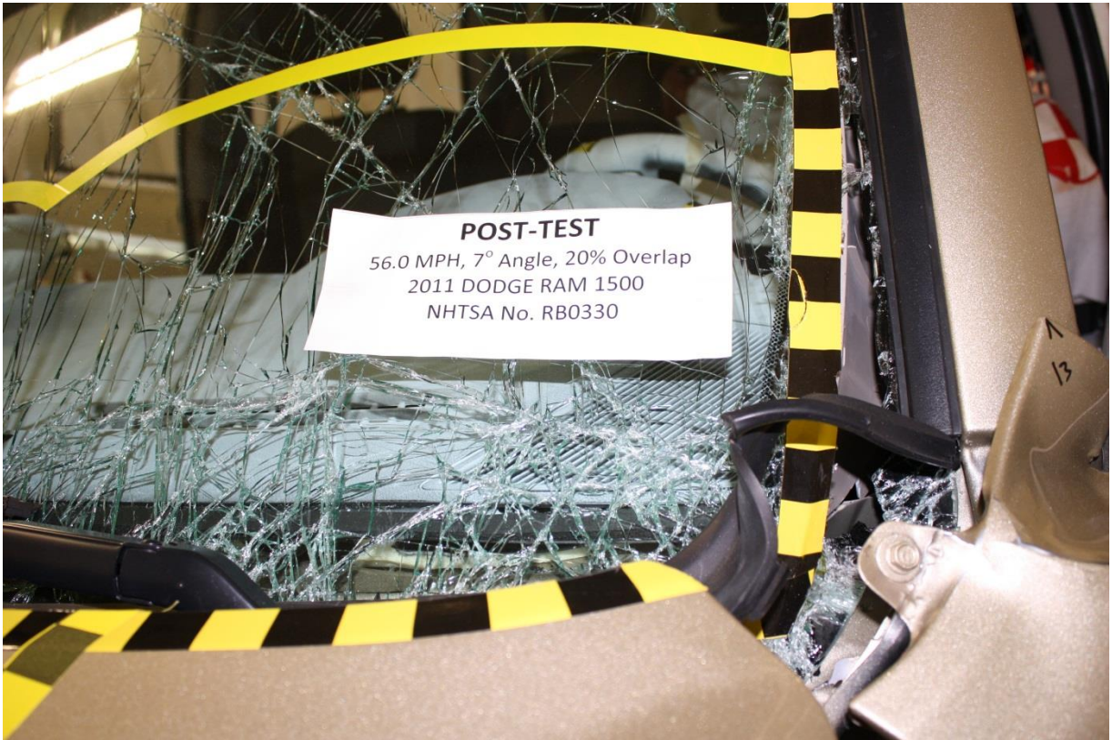
No. 127 Post-Test View of Windshield Separation
