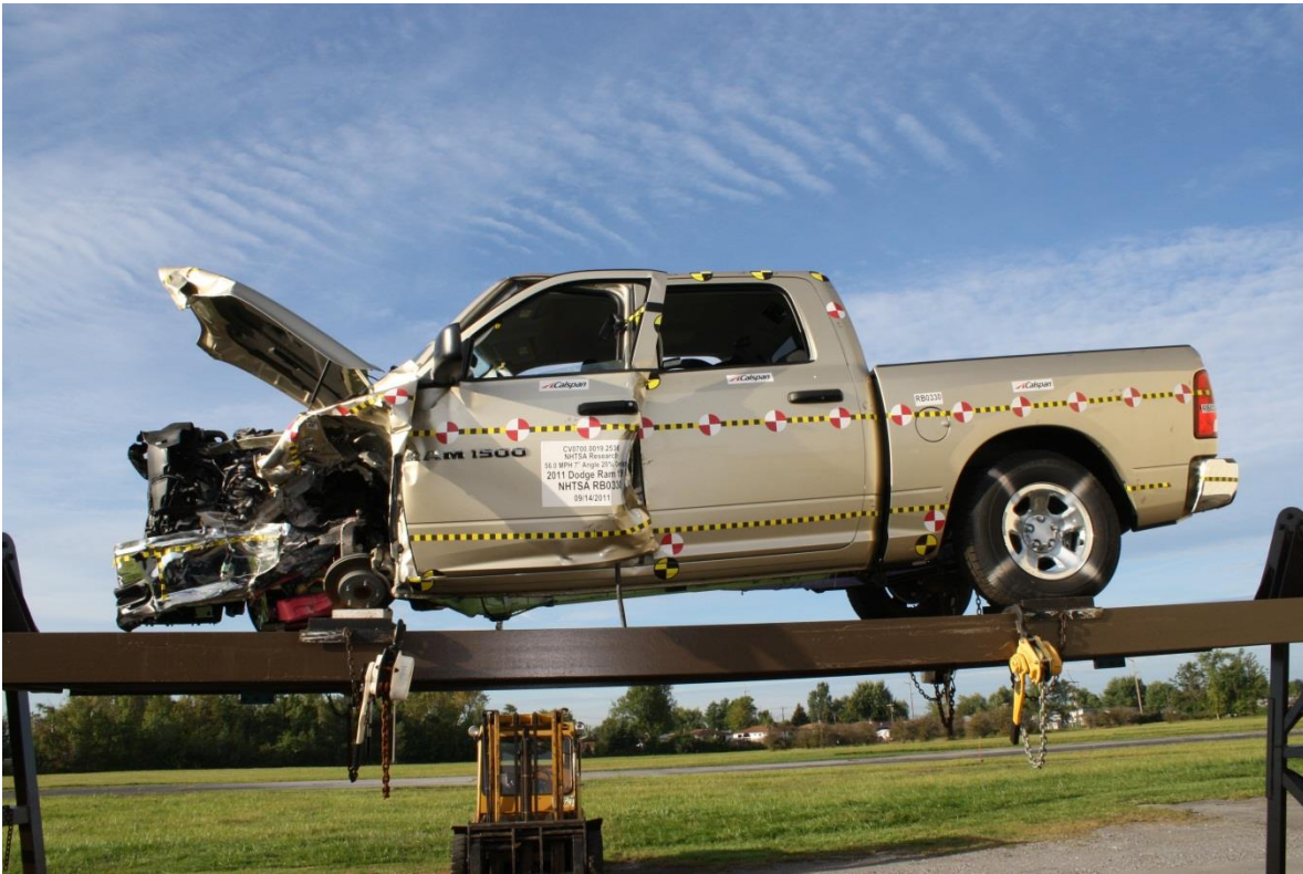
No. 136 Vehicle at 0 Degrees on Static Rollover Device
