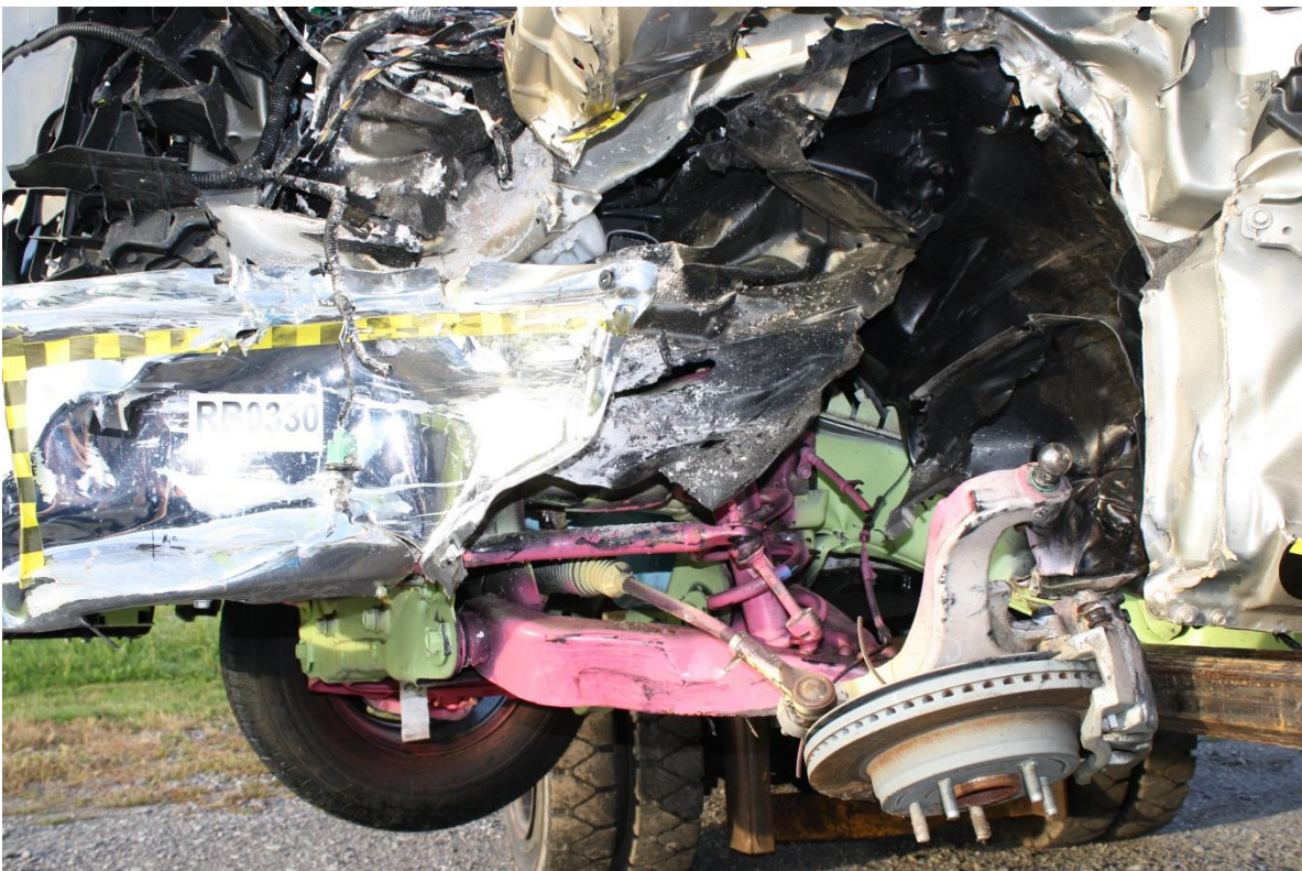
No. 118 Post-Test Frame Rail with tire removed
