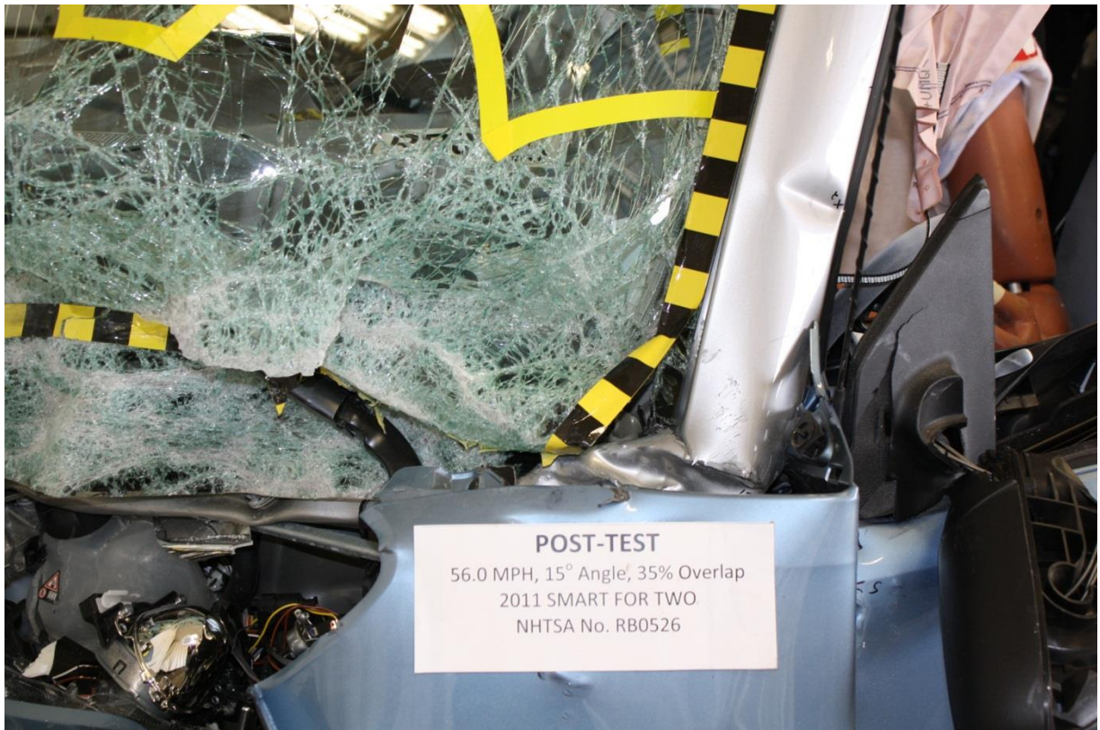
No. 127 Post-Test View of Windshield Separation
