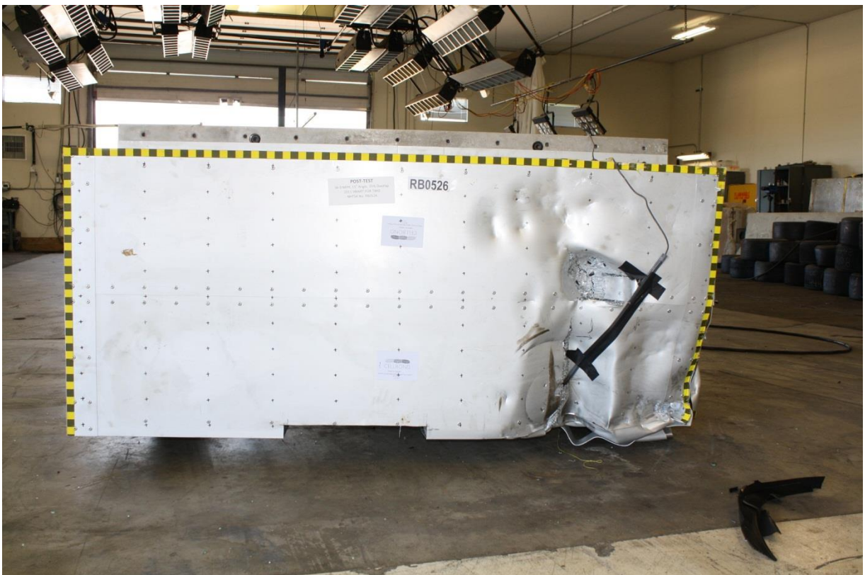
No. 135 Post-Test Front View of RRMDB
