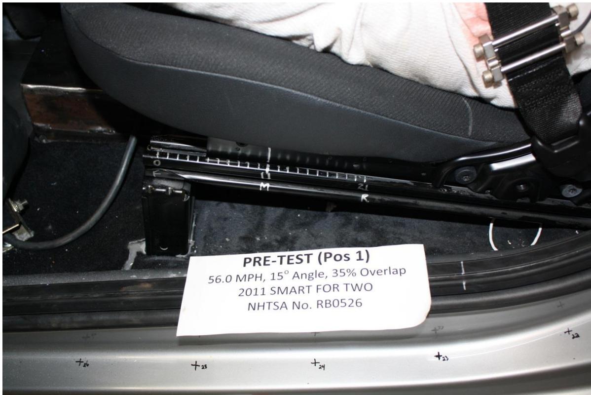
No. 066 Pre-Test Driver Seat Fore Aft Markings
