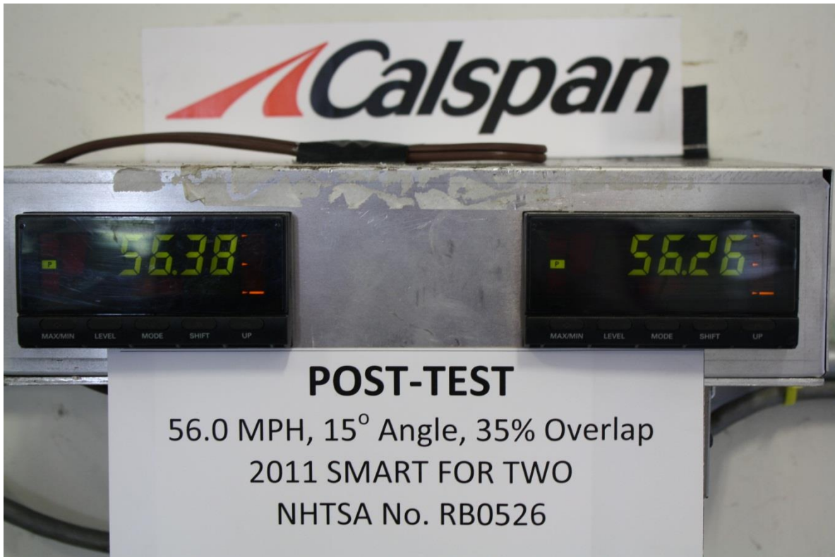
No. 104 Post-Test Speed Trap Readout
