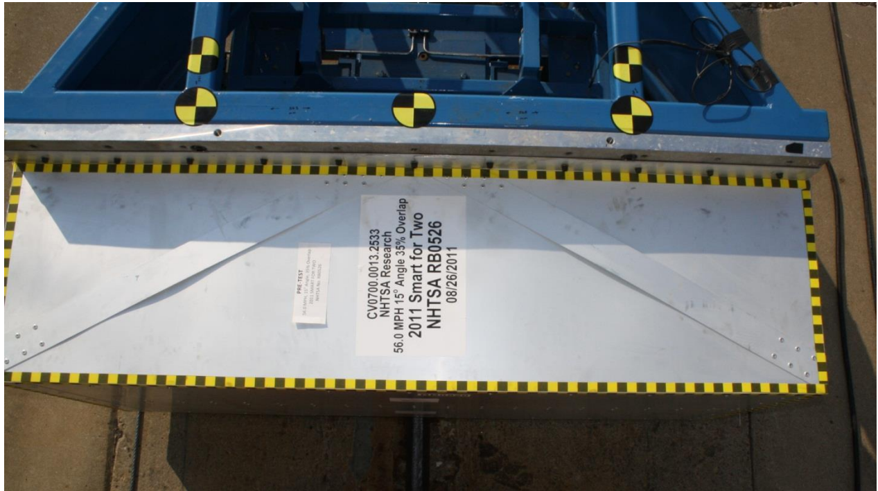
No. 132 Pre-Test Top View of RRMDB
