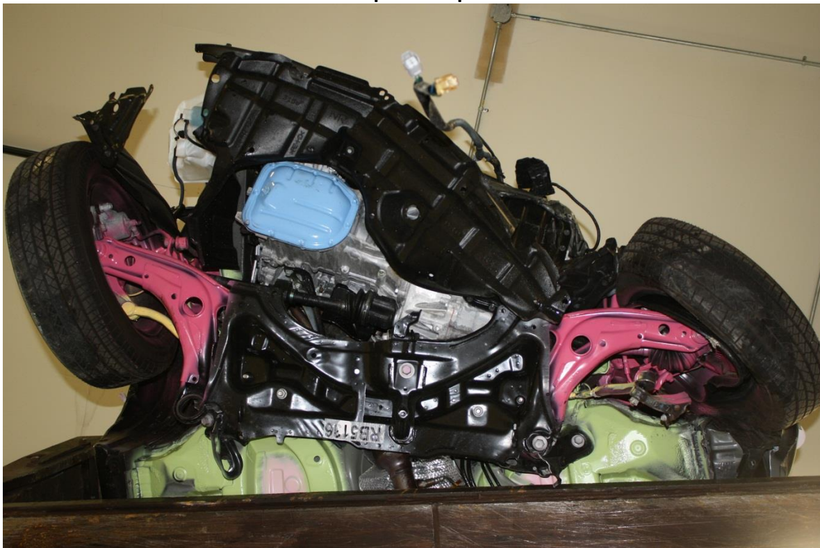
No. 116 Post-Test View of Front Sub-Frame Deformation
