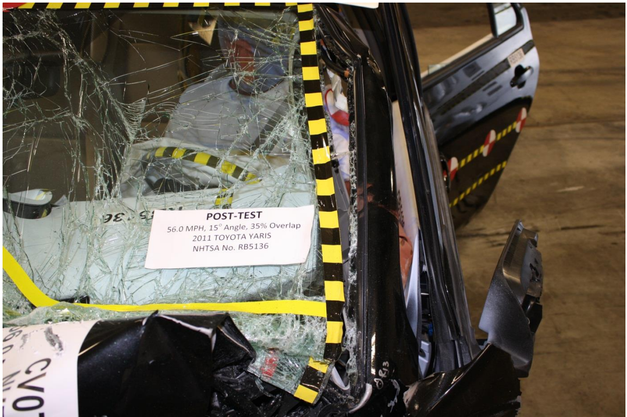
No. 127 Post-Test View of Windshield Separation
