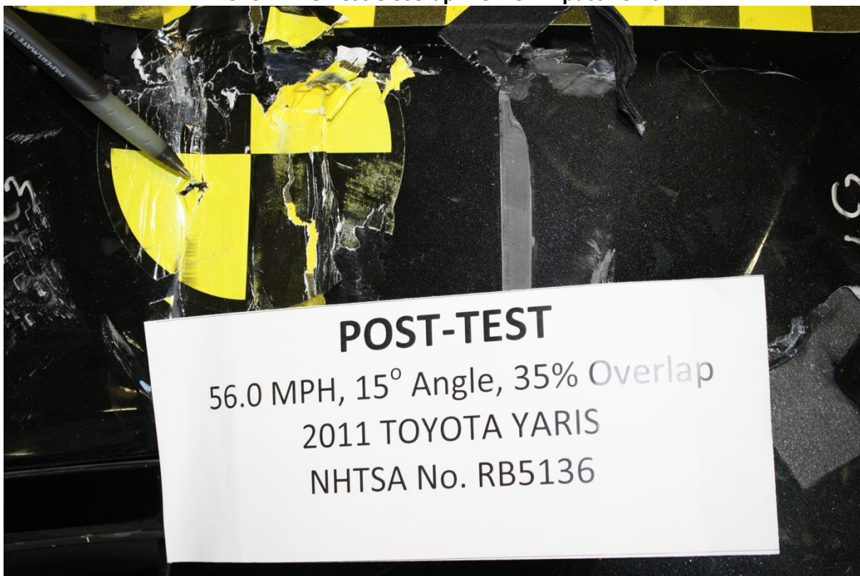
No. 023 Post-Test Close-up View of Impact Point
