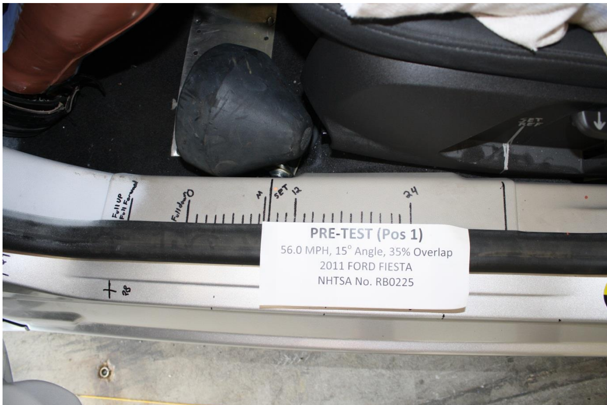
No. 066 Pre-Test Driver Seat Fore Aft Markings
