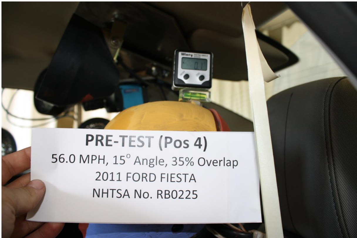
No. 093 Pre-Test Passenger View Showing Head Level
