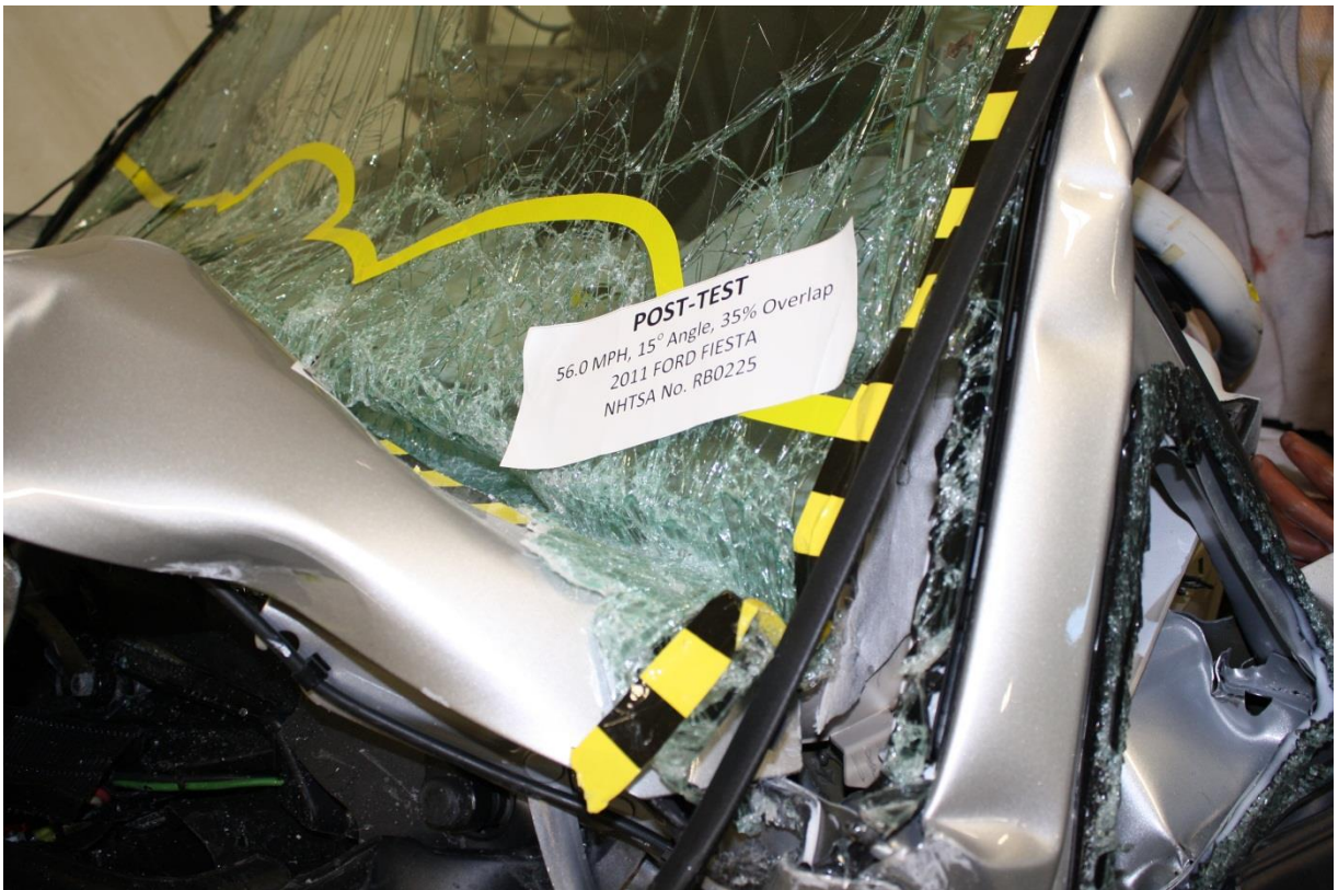
No. 127 Post-Test View of Windshield Separation
