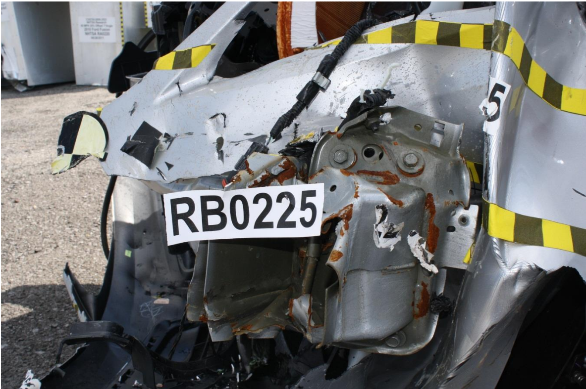
No. 118 Post-Test Frame Rail with tire removed
