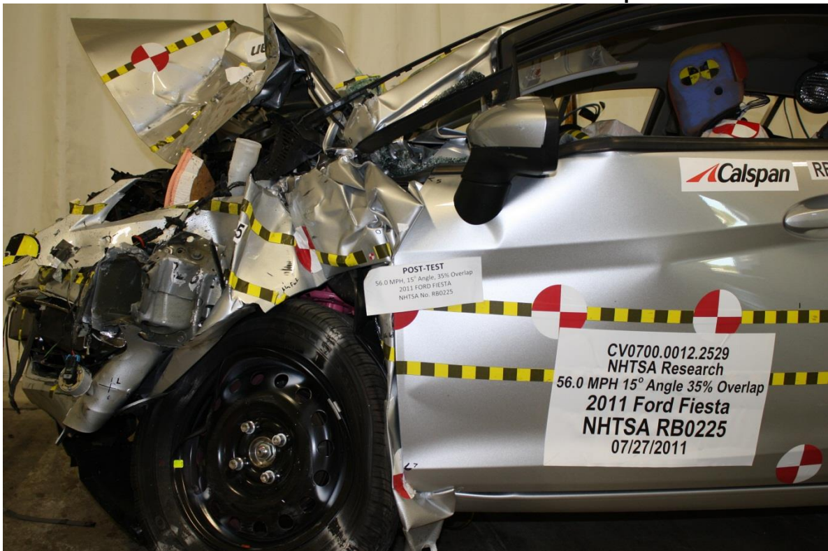
No. 122 Post-Test View of Deformation of A pillar
