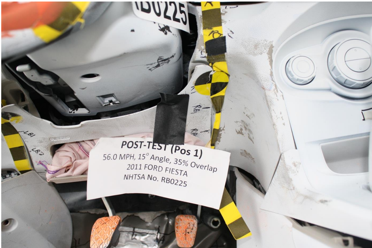
No. 047 Post-Test Right Side View of Driver Knee Bolsters
