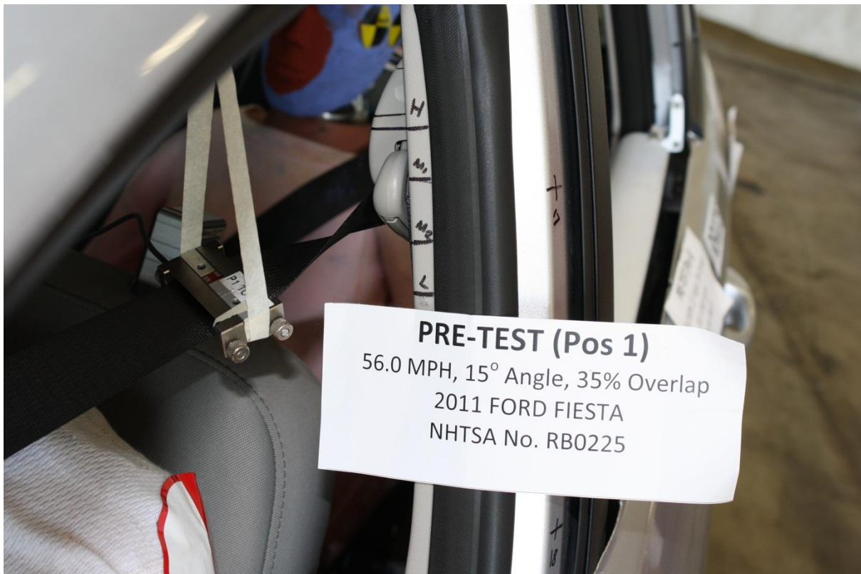
No. 068 Pre-Test Driver Adjustable D-ring
