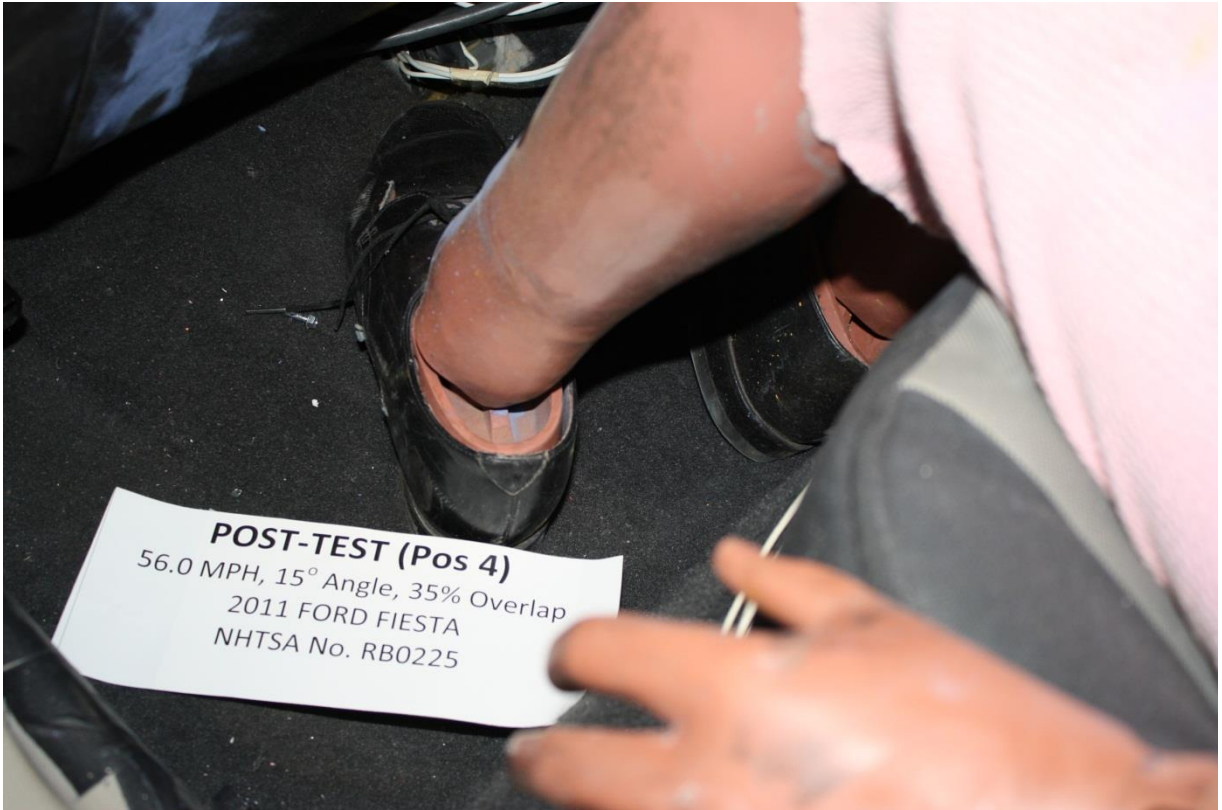
No. 099 Post-Test View of Passenger Dummy Feet
