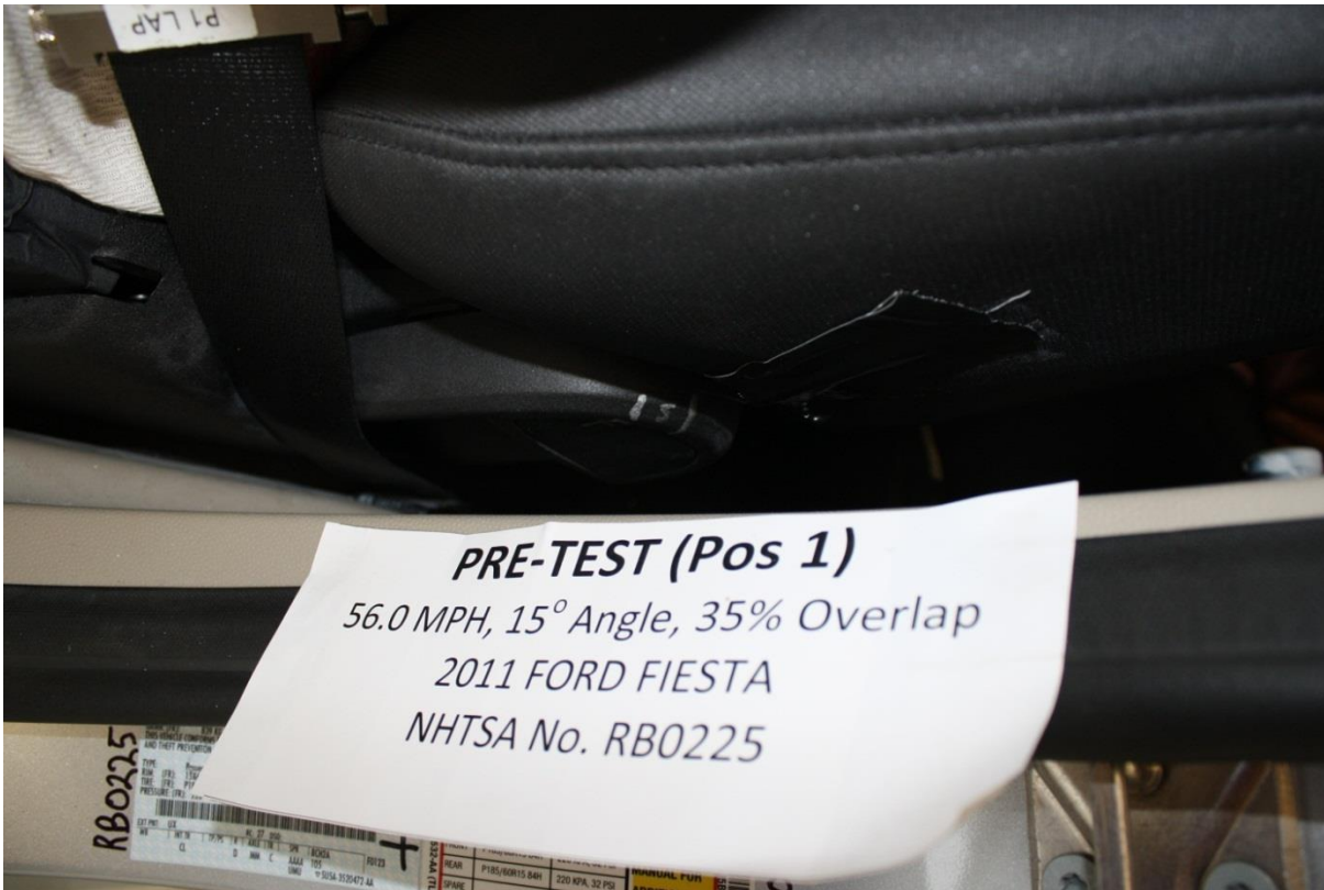
No. 064 Pre-Test Driver Seat Back Position markings
