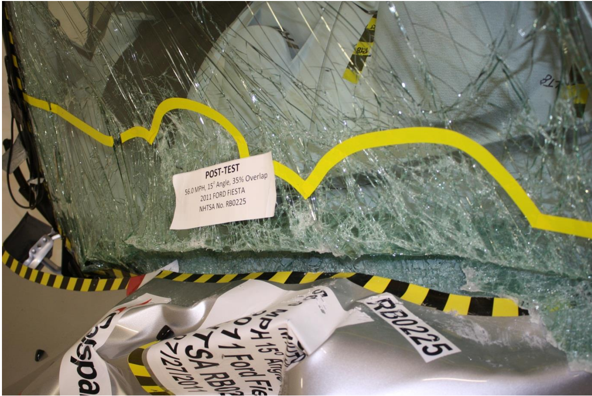
No. 055 Post-Test Driver Dummy Front Windshield View
