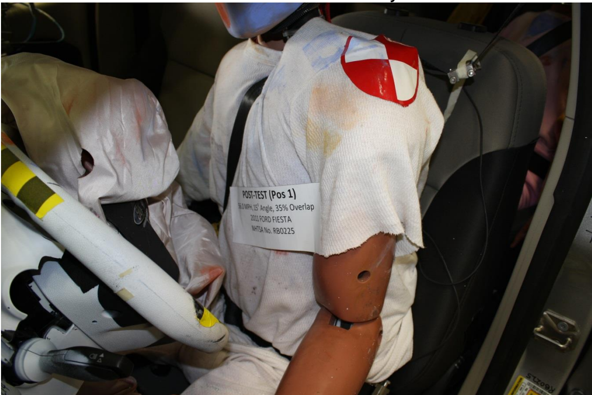
No. 078 Post-Test View of Driver Dummy Abdomen
