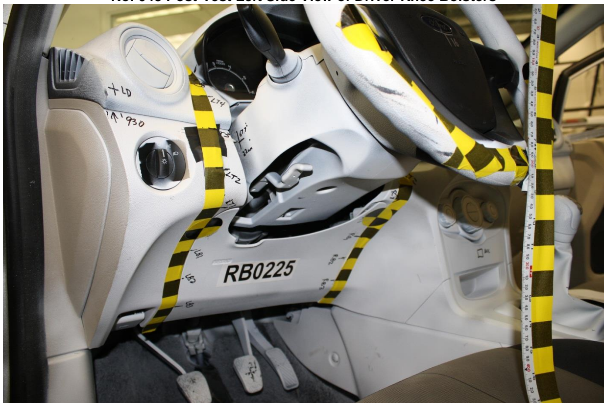
No. 044 Pre-Test Left Side View of Driver Knee Bolsters with panel removed
