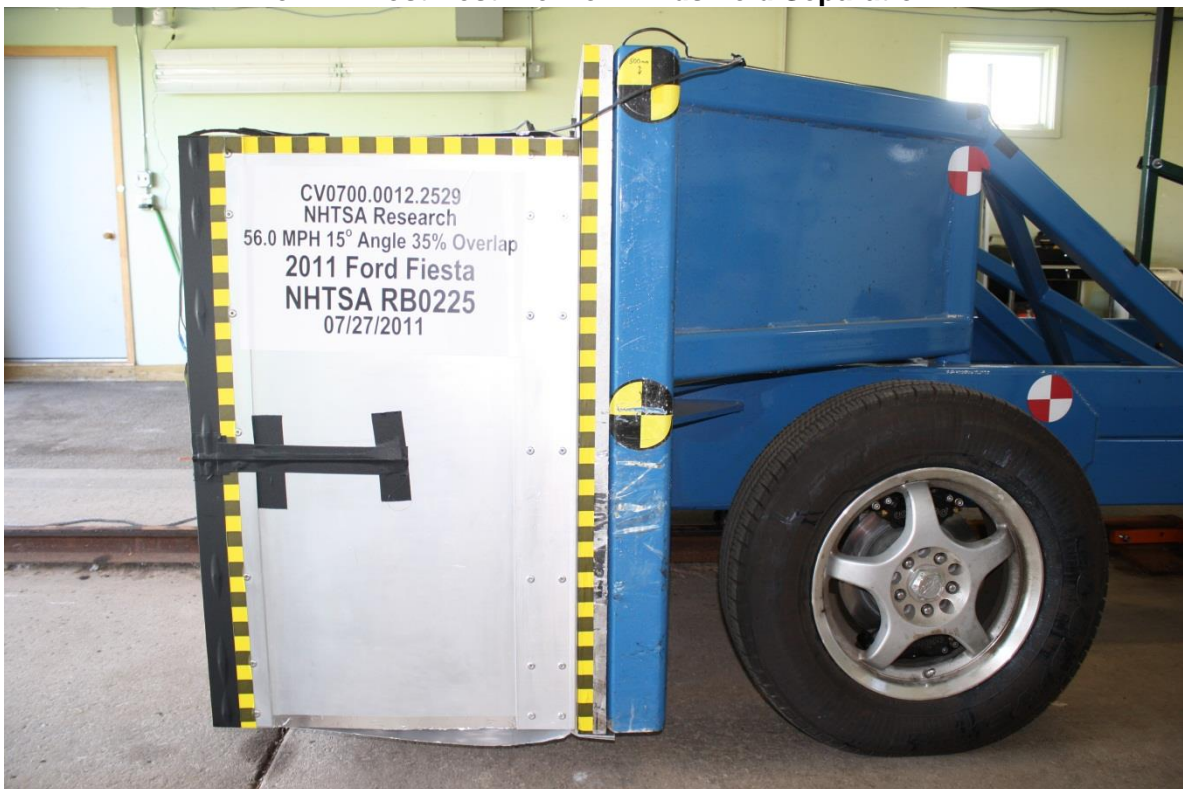
No. 128 Pre-Test Left Side View of RMDB
