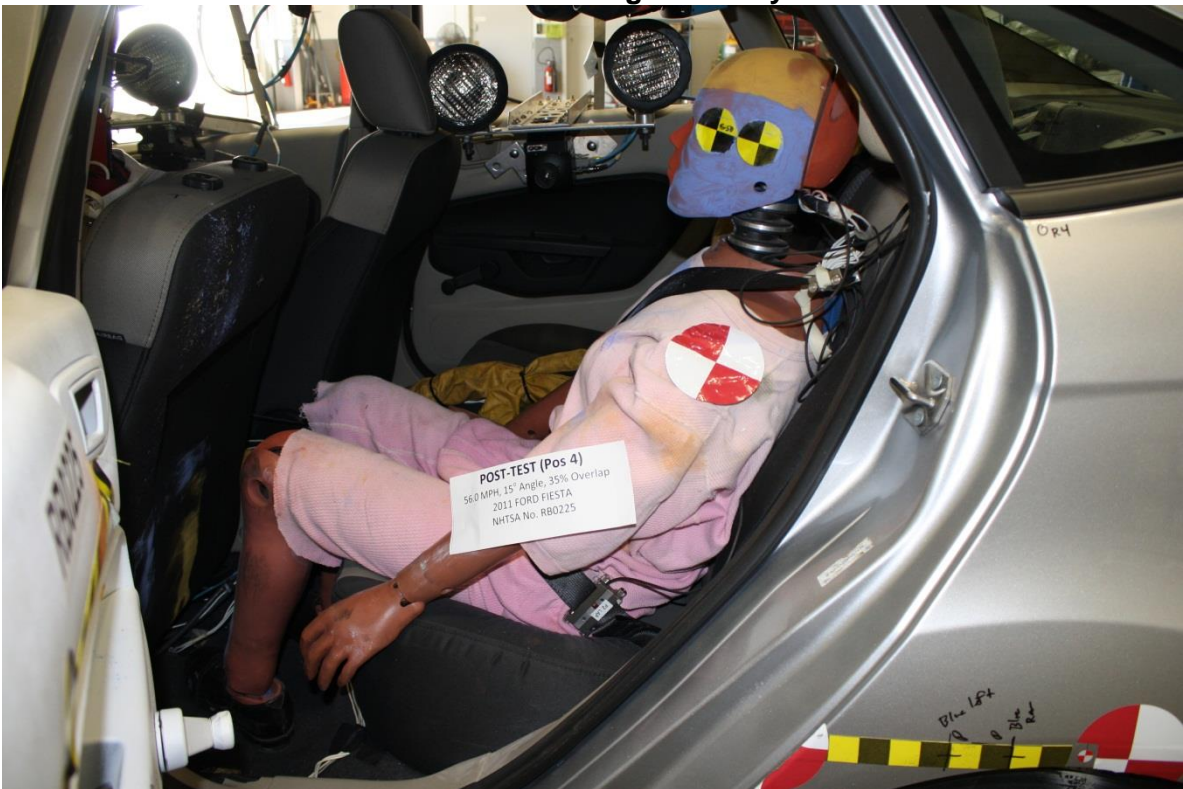
No. 086 Post-Test Left Side Passenger Dummy and Interior View
