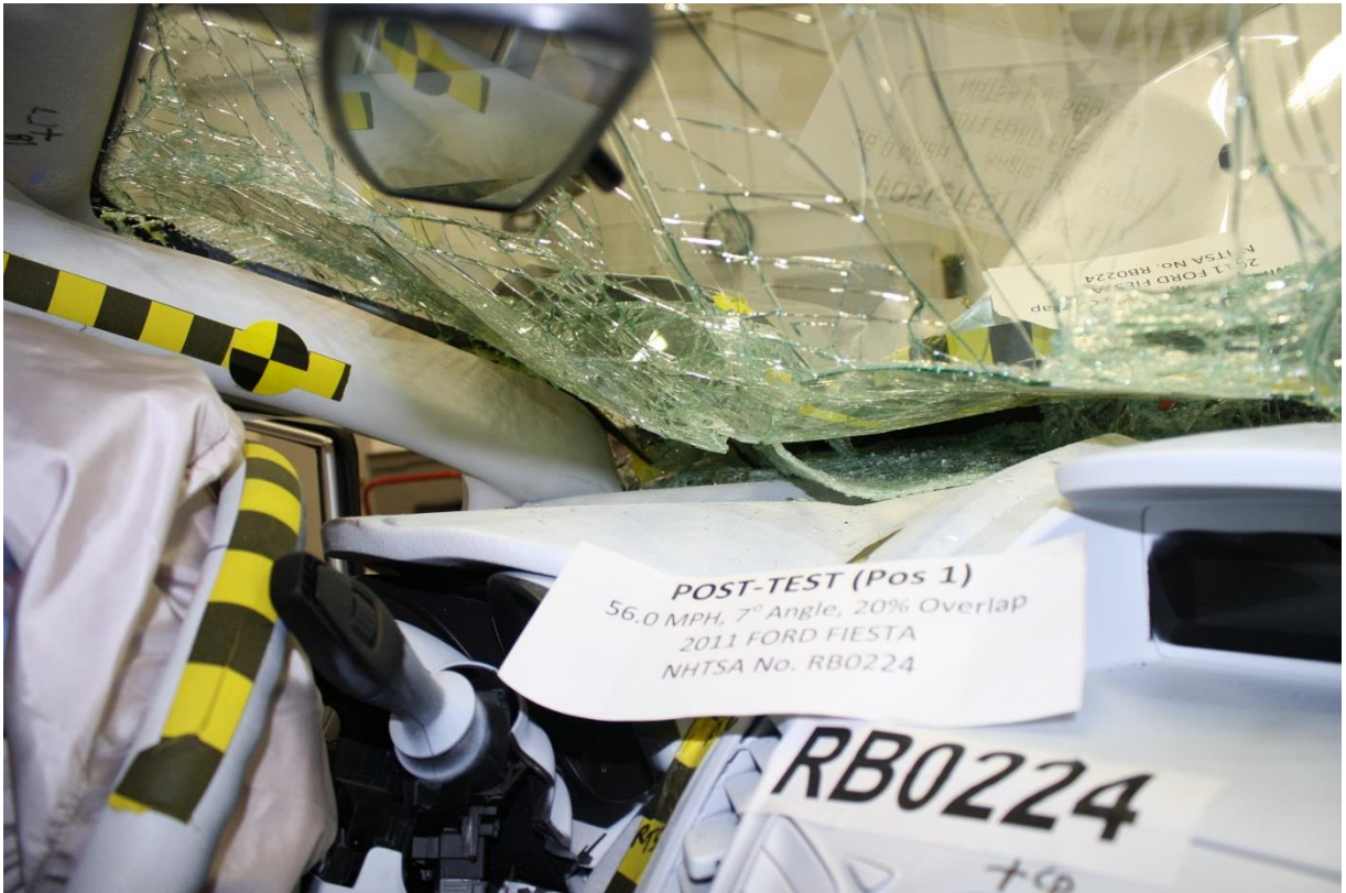
No. 127 Post-Test View of Windshield Separation
