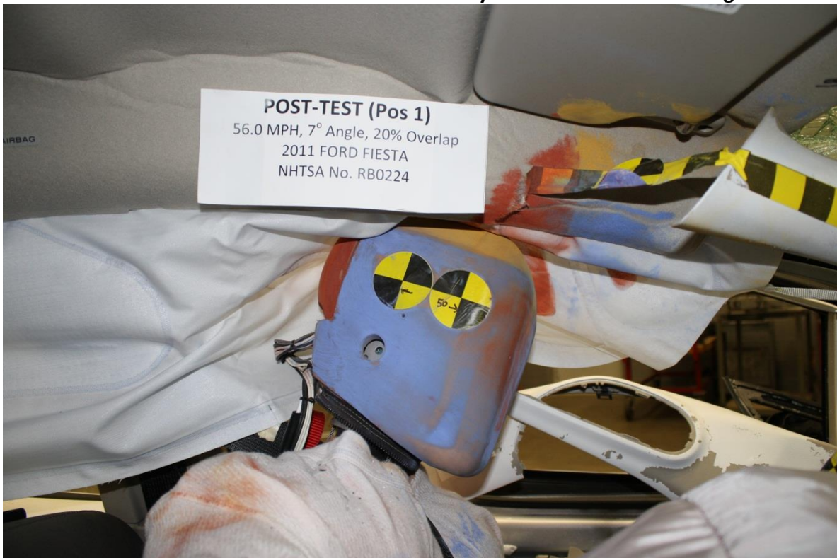
No. 082 Post-Test View of Driver Dummy Head Contact with Vehicle Interior (a, b, c, etc)
