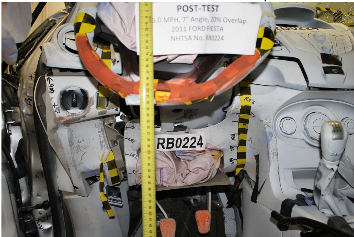
No. 041 Post-Test Overall View of Driver Knee Bolsters with panel removed
