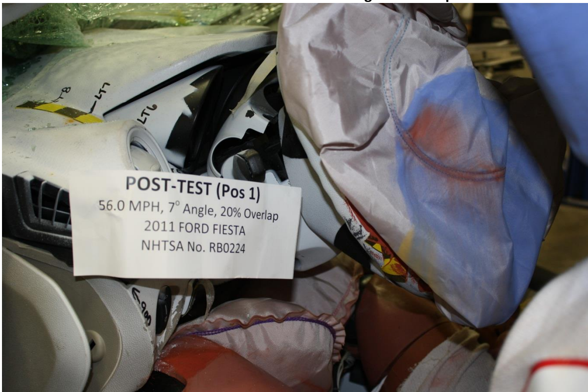
No. 080 Post-Test Left Side View of Steering Wheel set position
