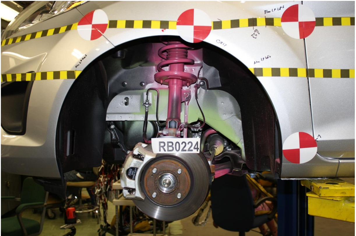
No. 117 Pre-Test Frame Rail with tire removed
