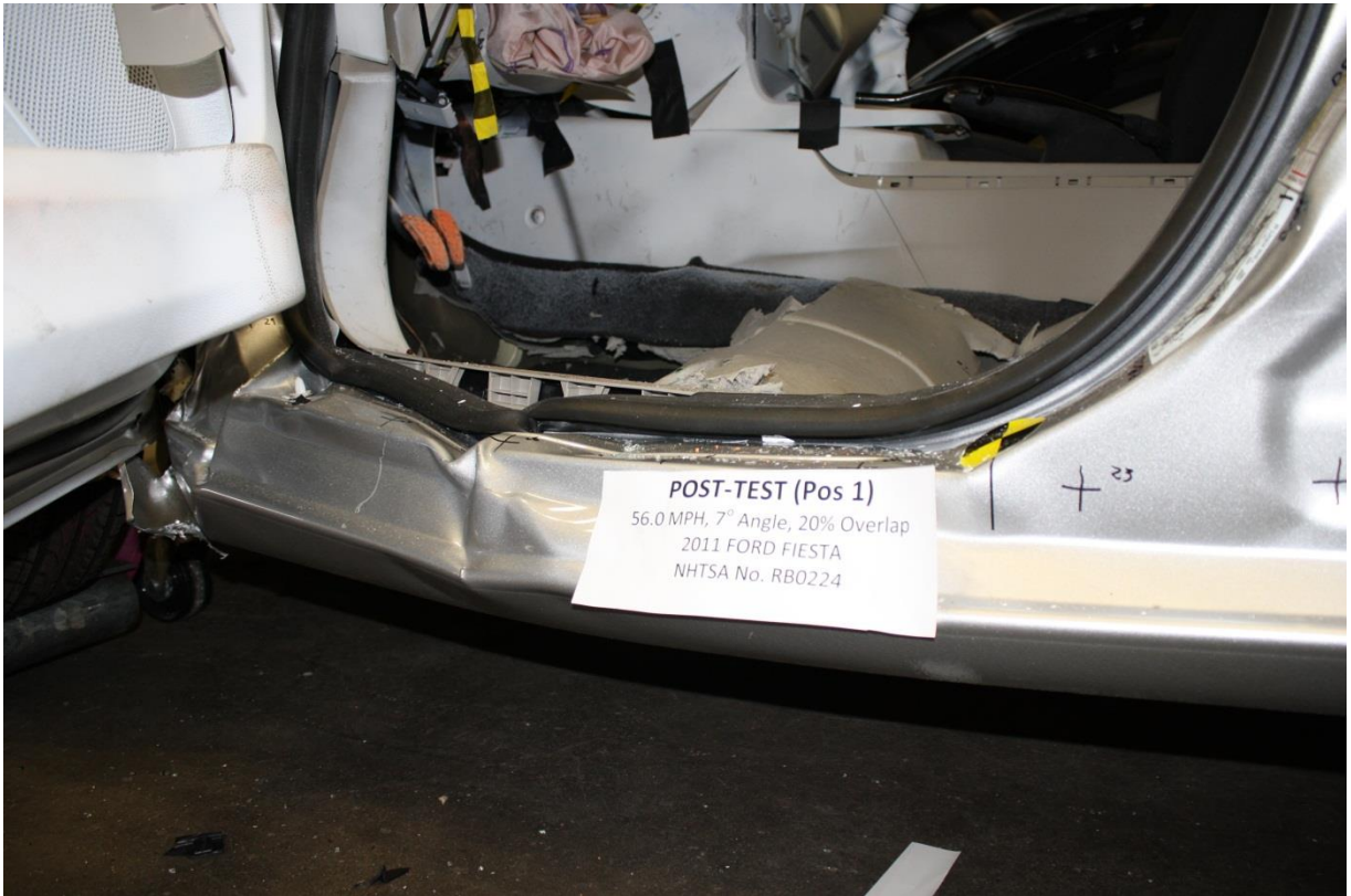
No. 121 Post-Test View of Door Sill with door open
