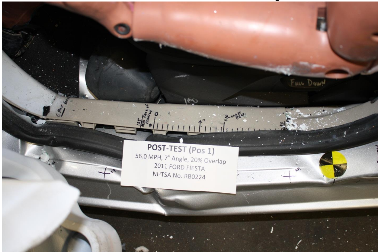
No. 067 Post-Test Driver Seat Fore Aft Markings
