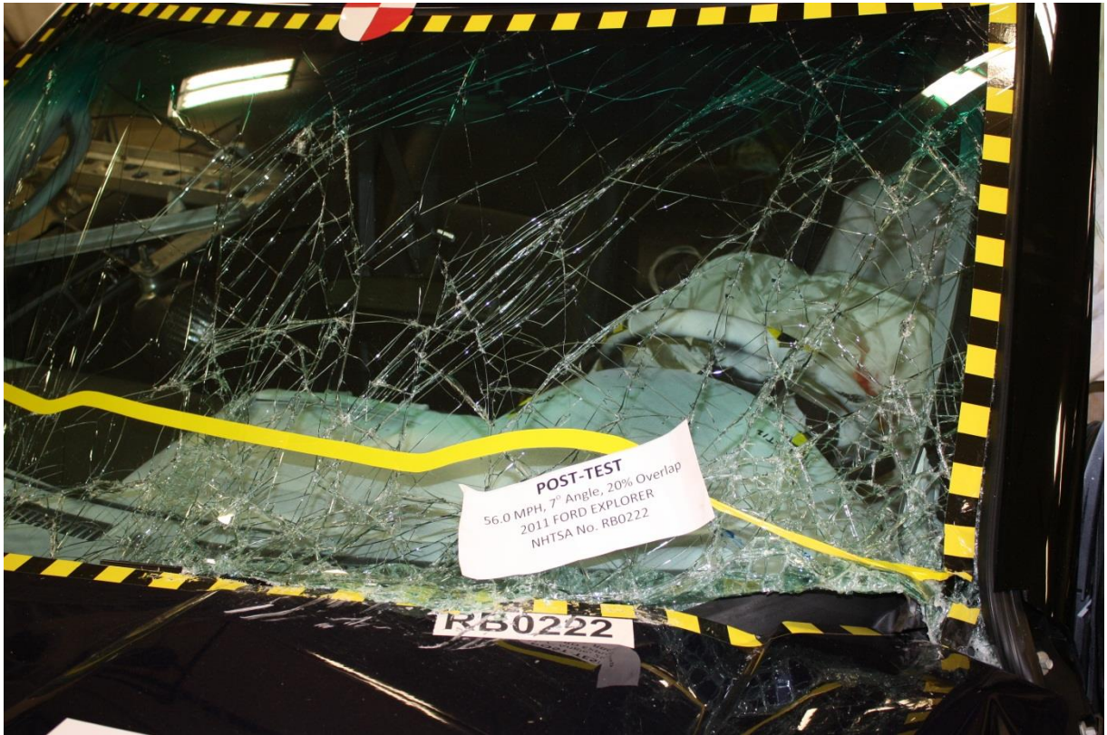
No. 127 Post-Test View of Windshield Separation
