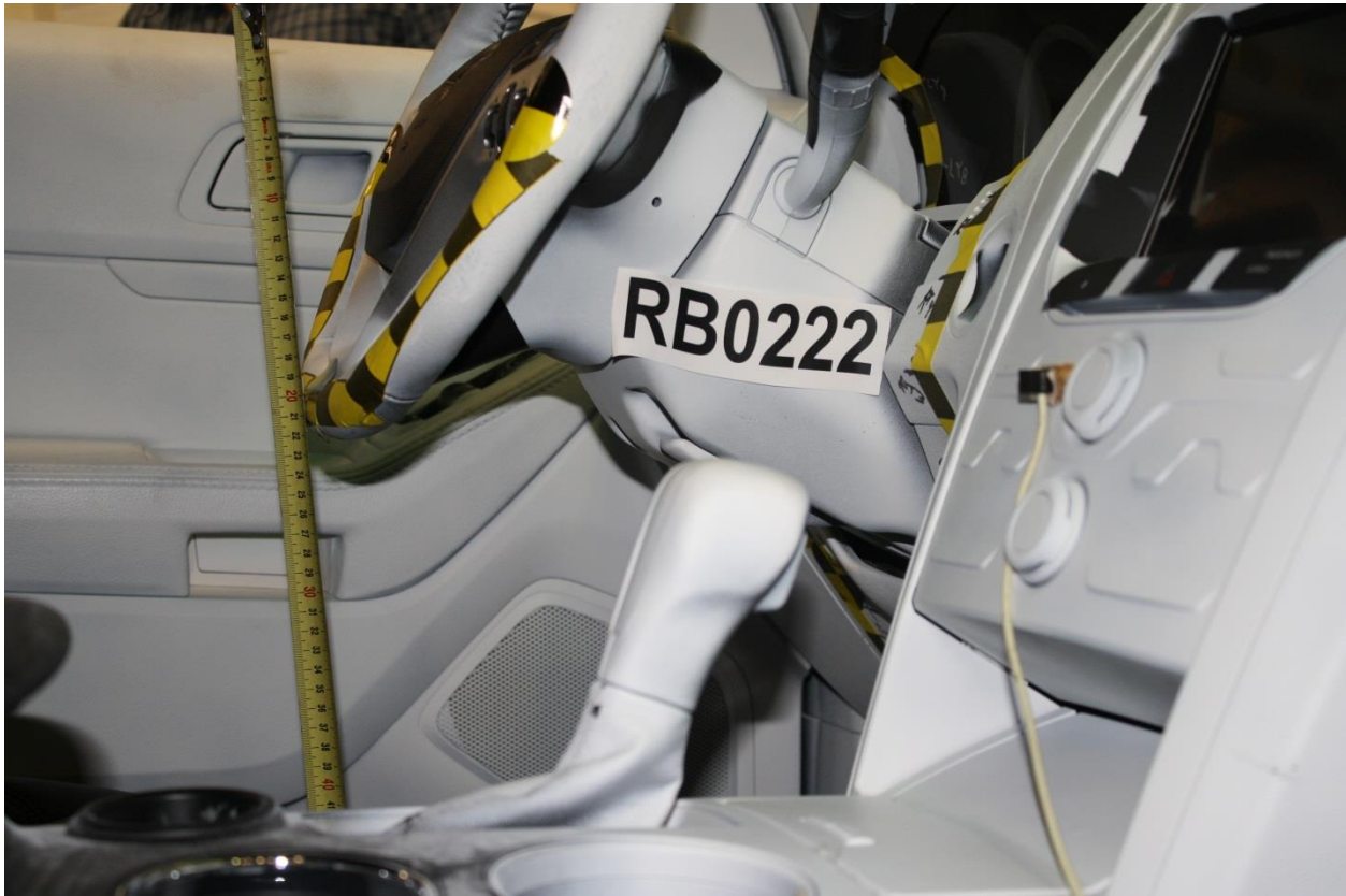
No. 048 Pre-Test Right Side View of Driver Knee Bolster with panel removed
