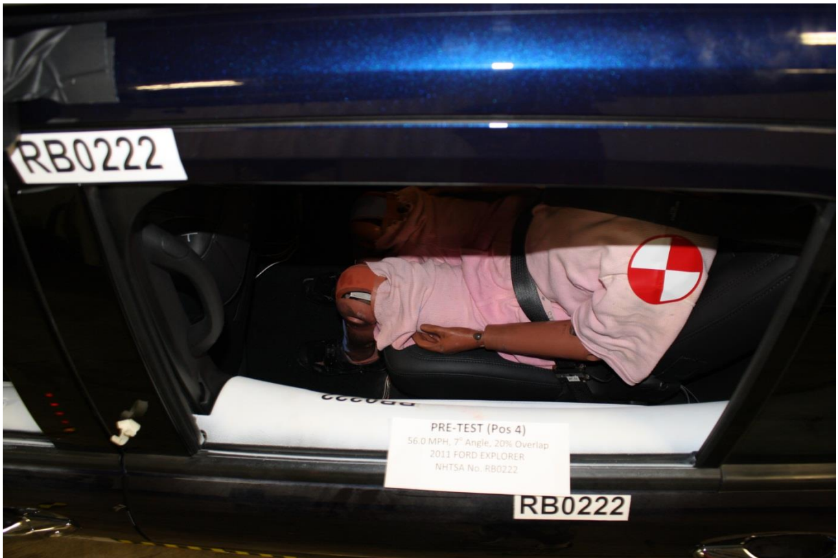
No. 091 Pre-Test View of Passenger Dummy Door Clearance
