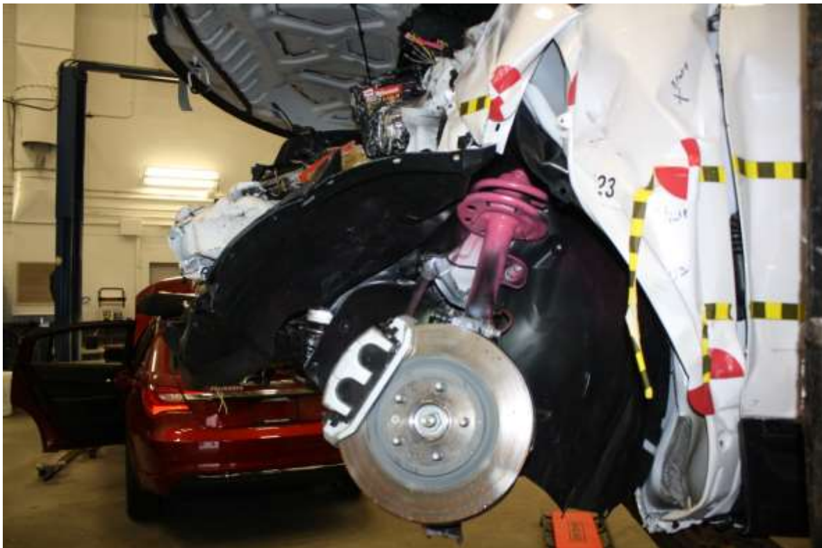
No. 120 Post-Test View of Wheel Well with tire removed
