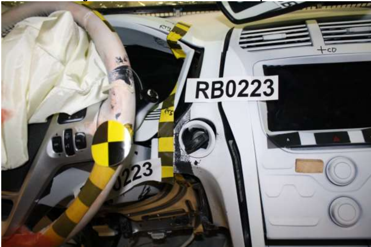
No. 049 Post-test right side view of driver knee bolster with panel removed
