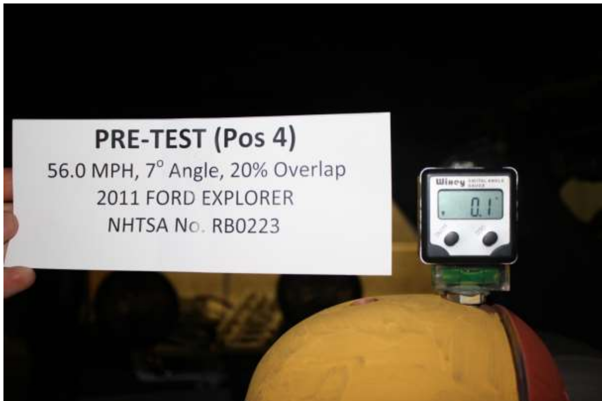
No. 093 Pre-Test Passenger View Showing Head Level (wrong placard)
