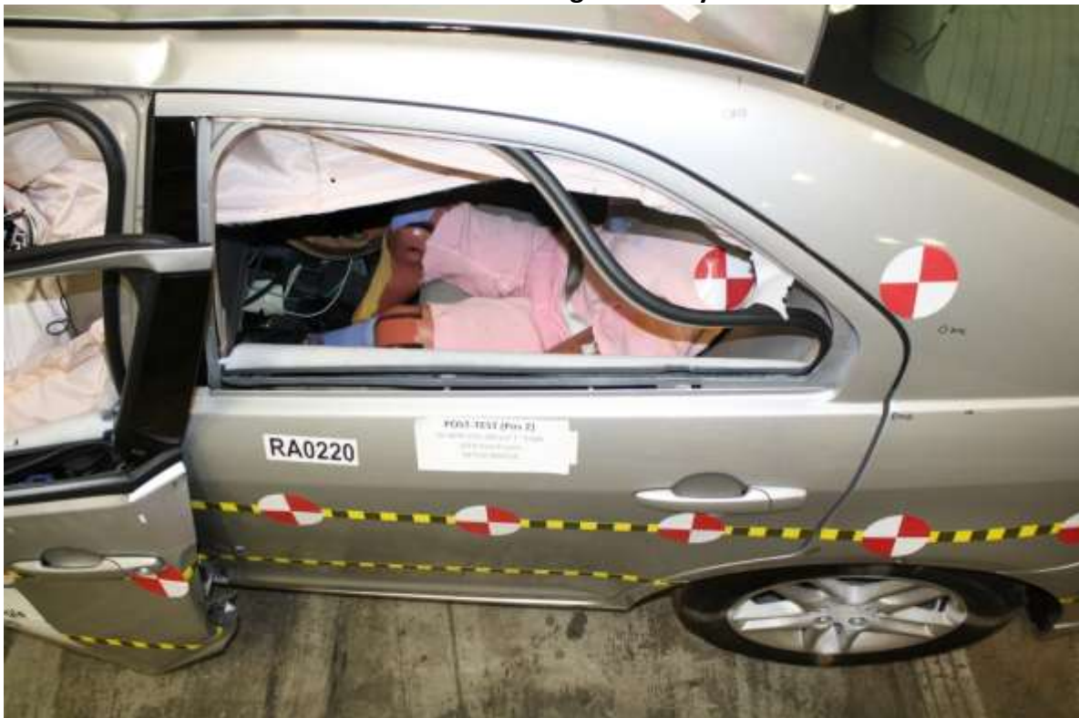
No. 092 Post-Test View of Passenger Dummy Door Clearance
