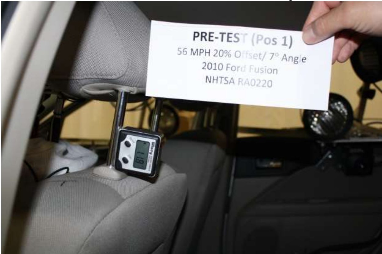
No. 065 Pre-Test Driver Seat Back Position with Level or Inclinometer
