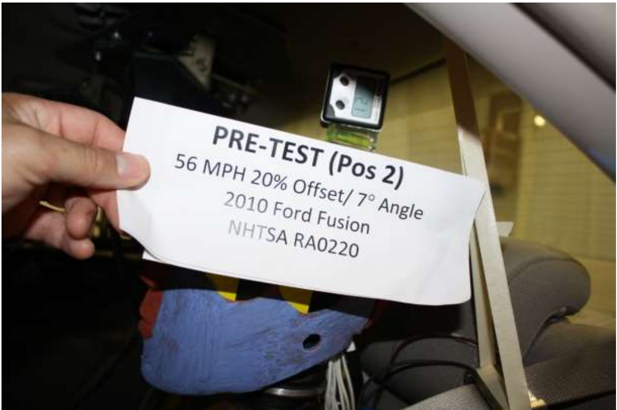
No. 093 Pre-Test Passenger View Showing Head Level
