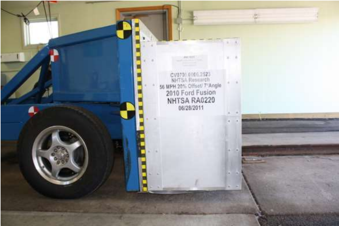
No. 130 Pre-Test Right Side View of RMDB
