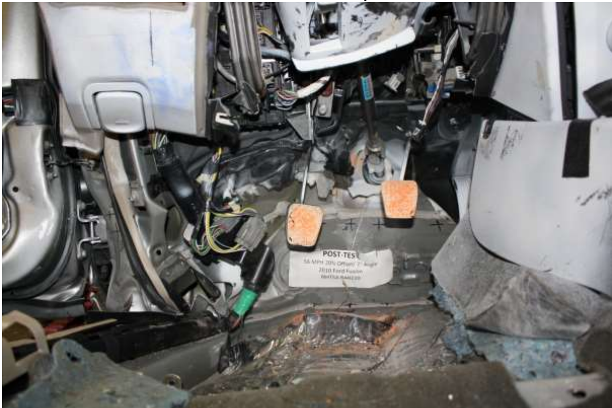
No. 053 Post-Test view of Driver Floor pan at Mid seat level
