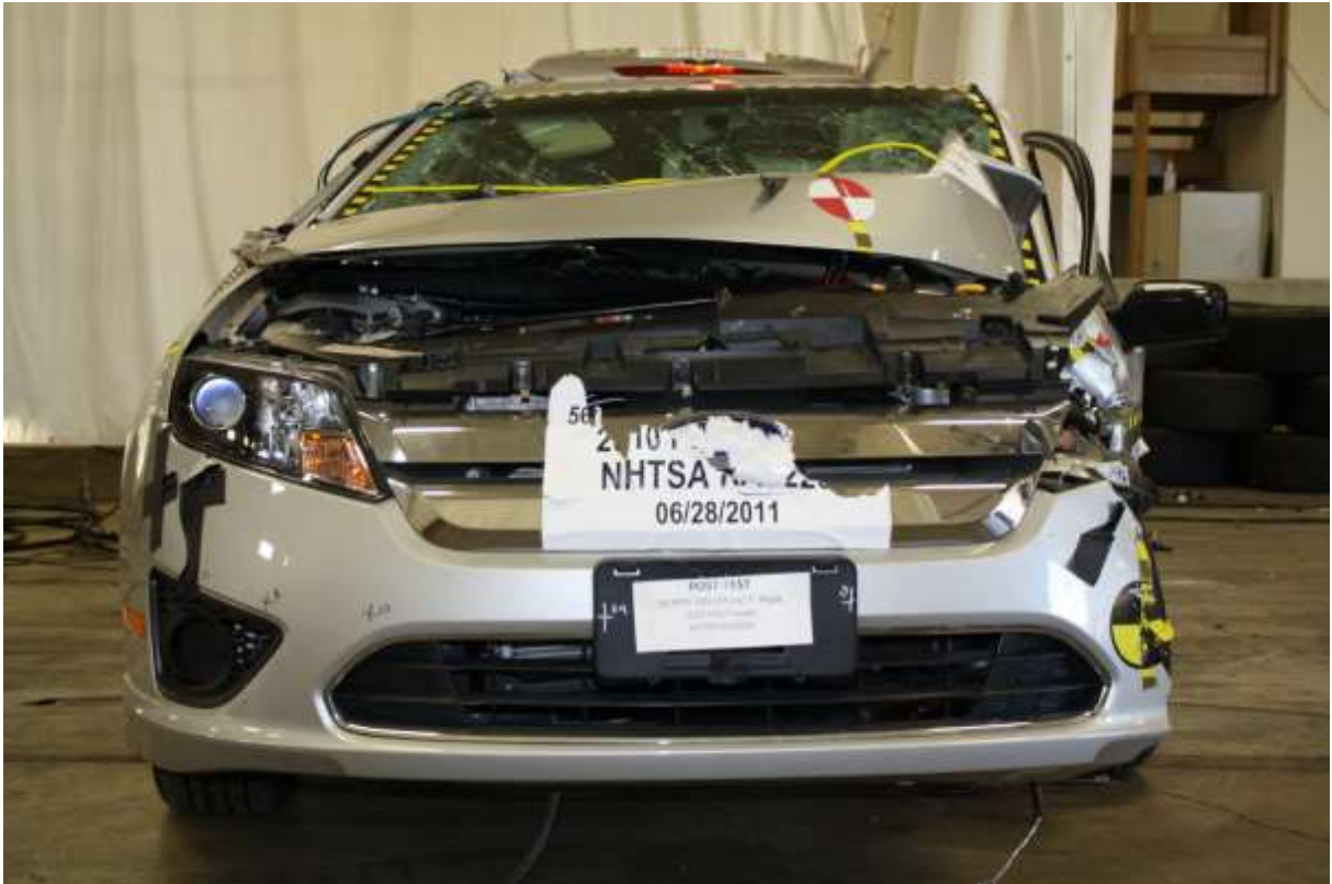
No. 006 Post-Test Front View of Test Vehicle
