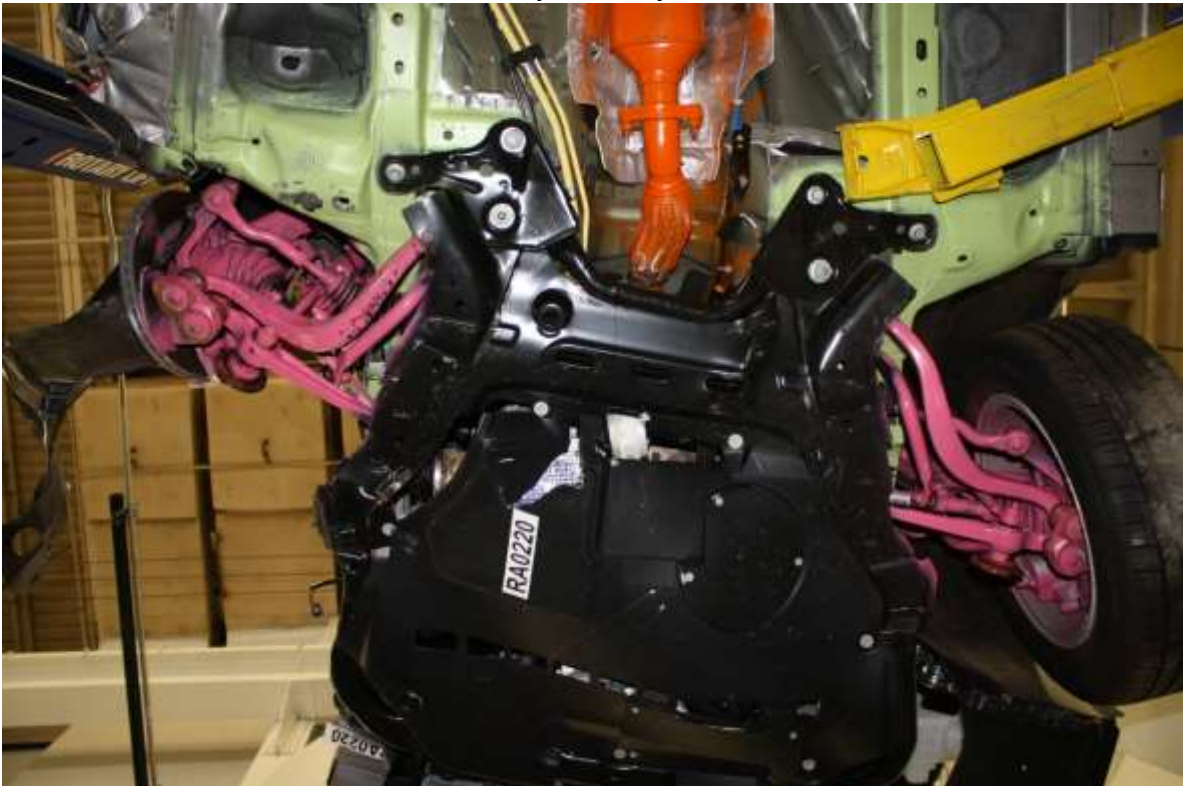
No. 116 Post-Test View of Front Sub-Frame Deformation
