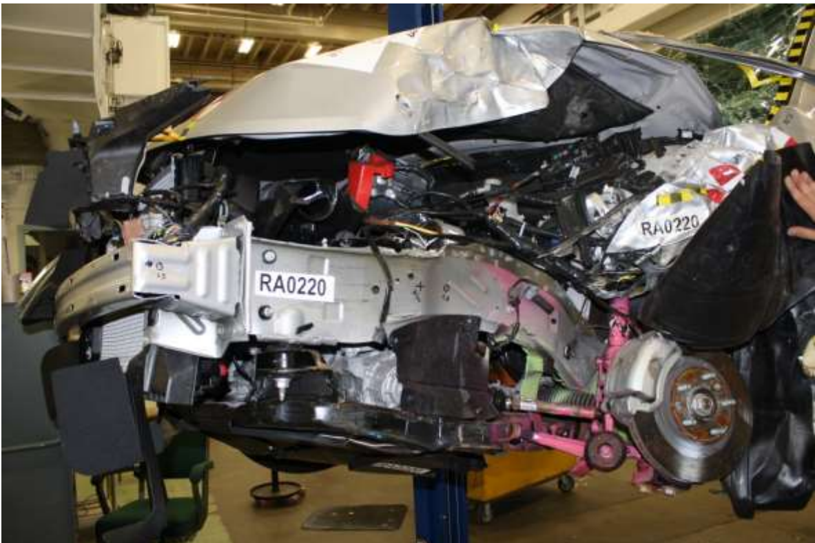
No. 118 Post-Test Frame Rail with tire removed
