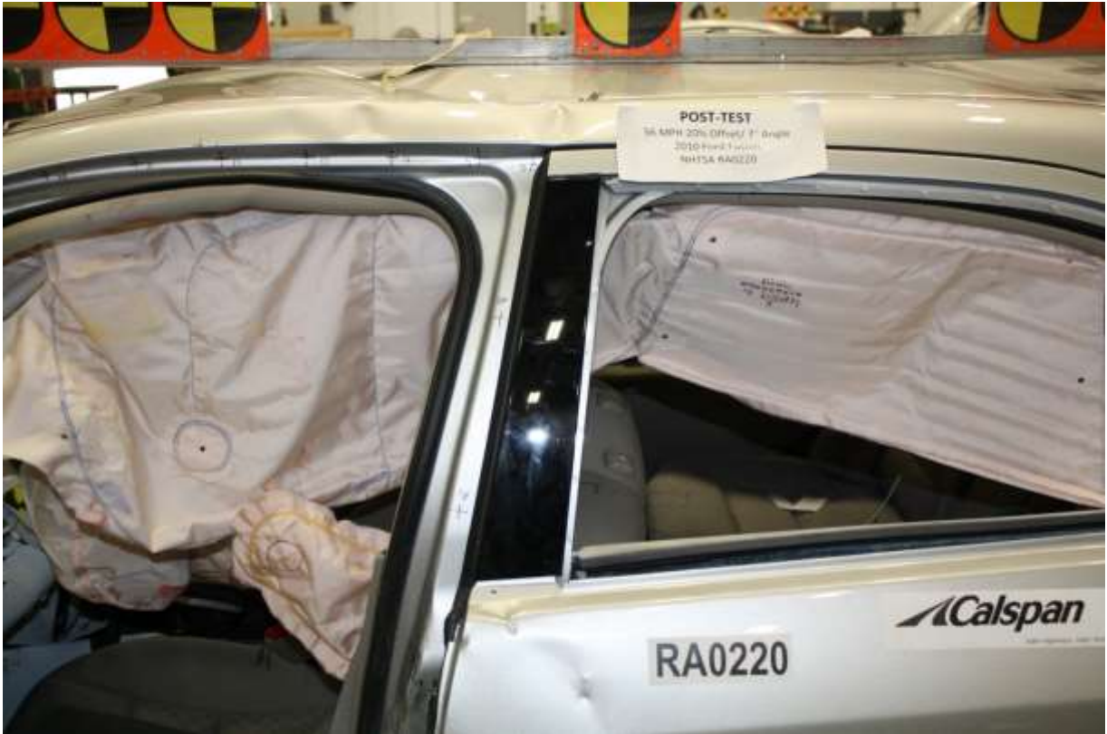
No. 123 Post-Test View of Deformation of B pillar
