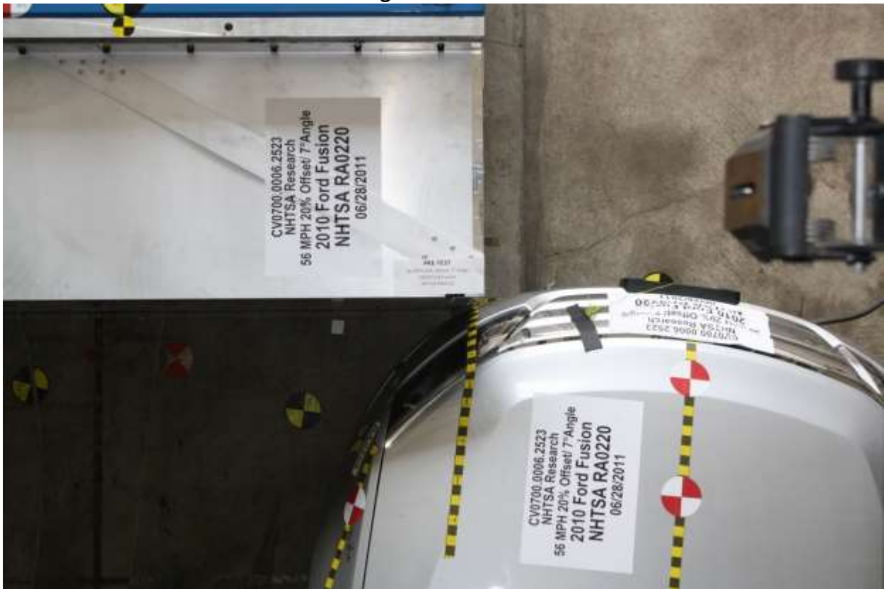
No. 019 Pre-Test Overhead View of RMDB against target vehicle at ideal Impact Point
