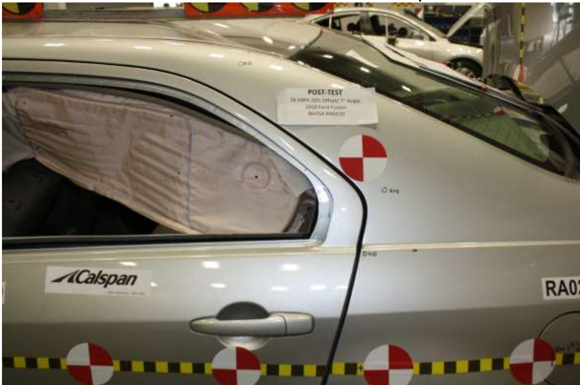
No. 124 Post-Test View of Deformation of C pillar
