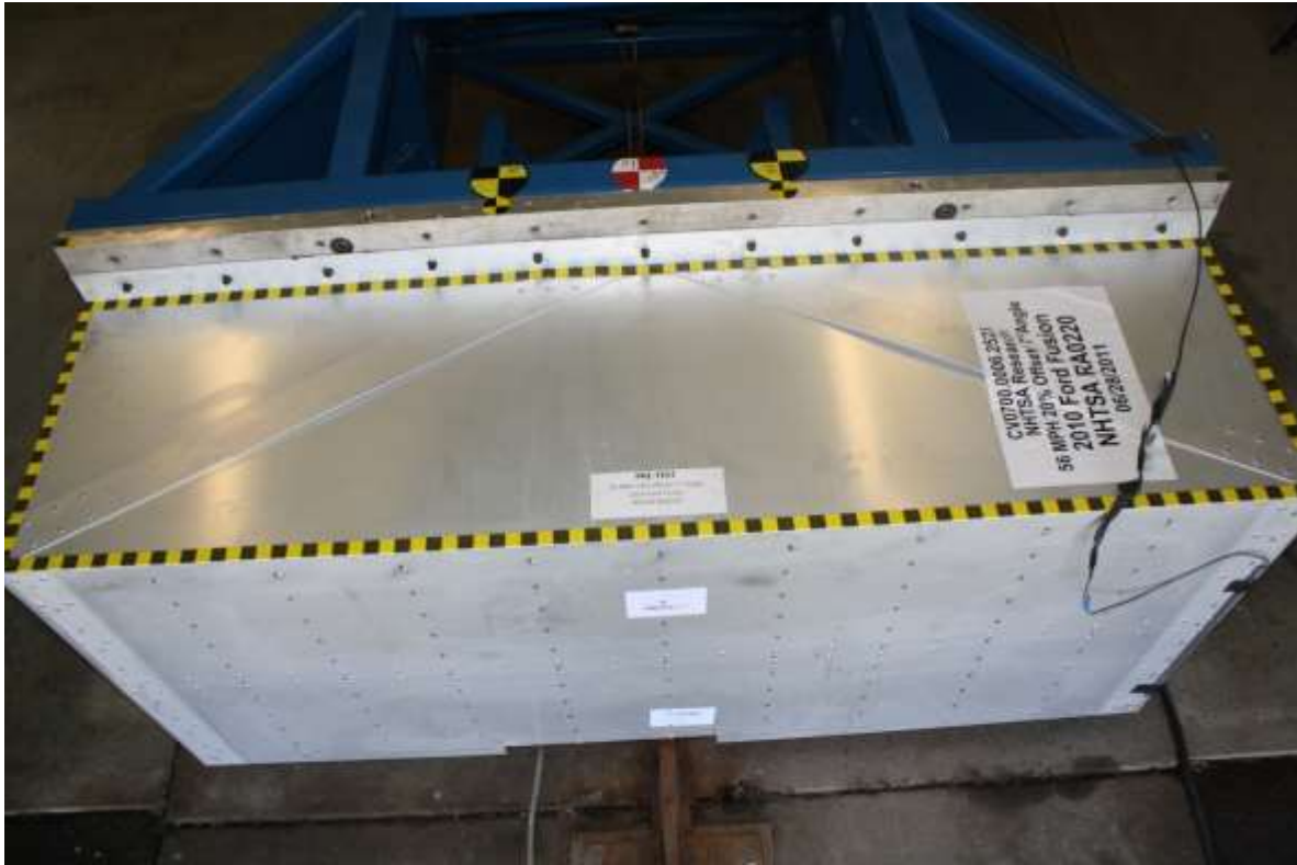
No. 132 Pre-Test Top View of RMDB
