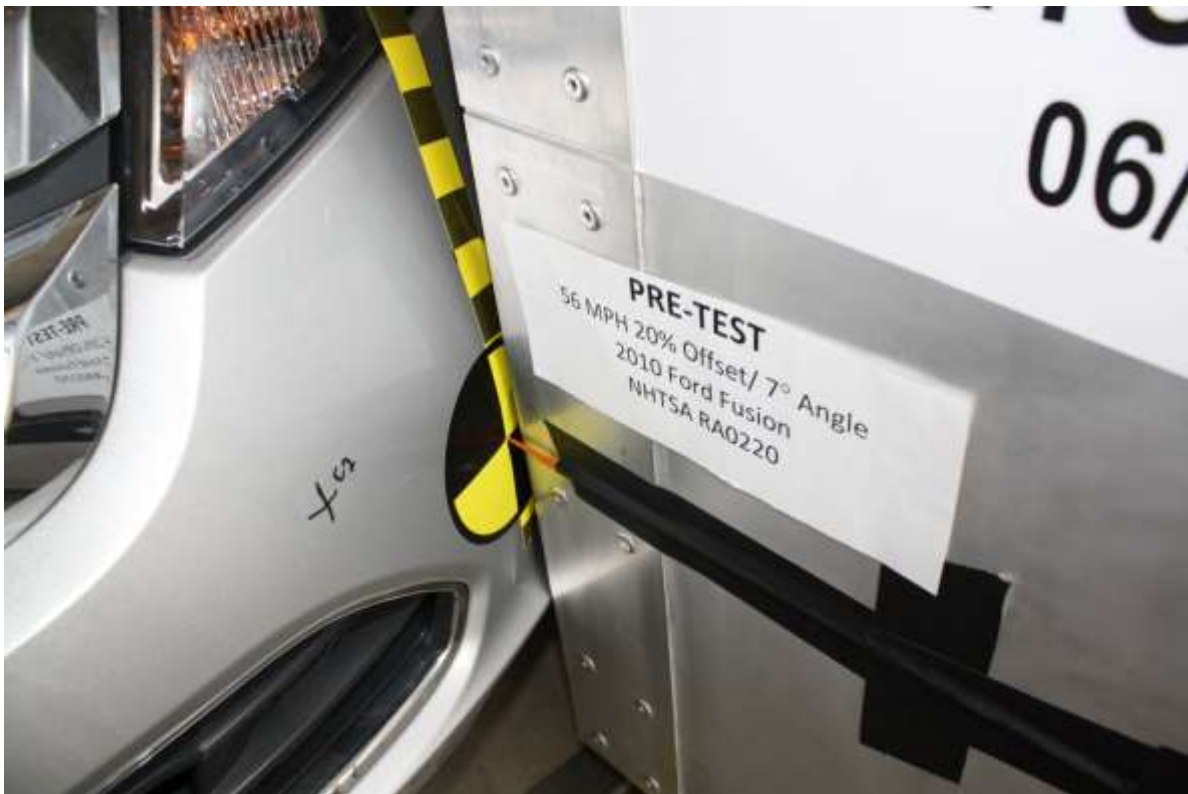
No. 022 Pre-Test Close-up View of Impact Point
