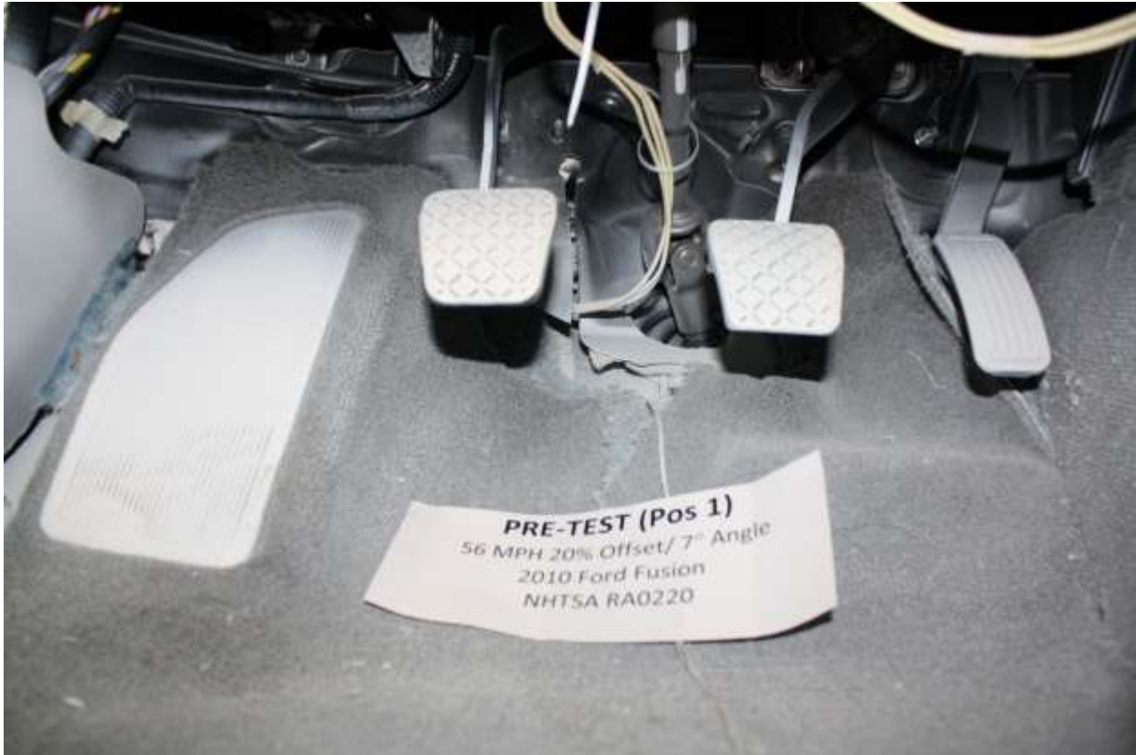
No. 052 Pre-Test View of Driver Floor pan at Mid seat level
