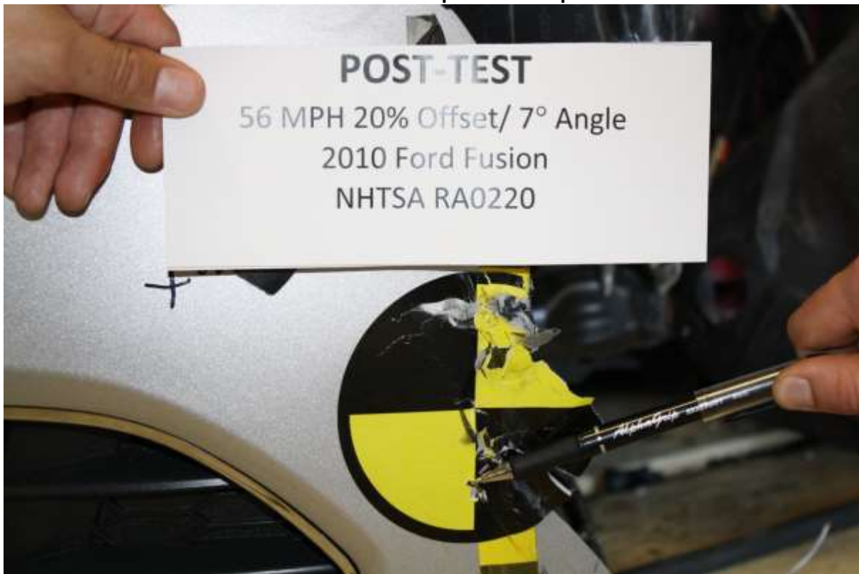
No. 023 Post-Test Close-up View of Impact Point
