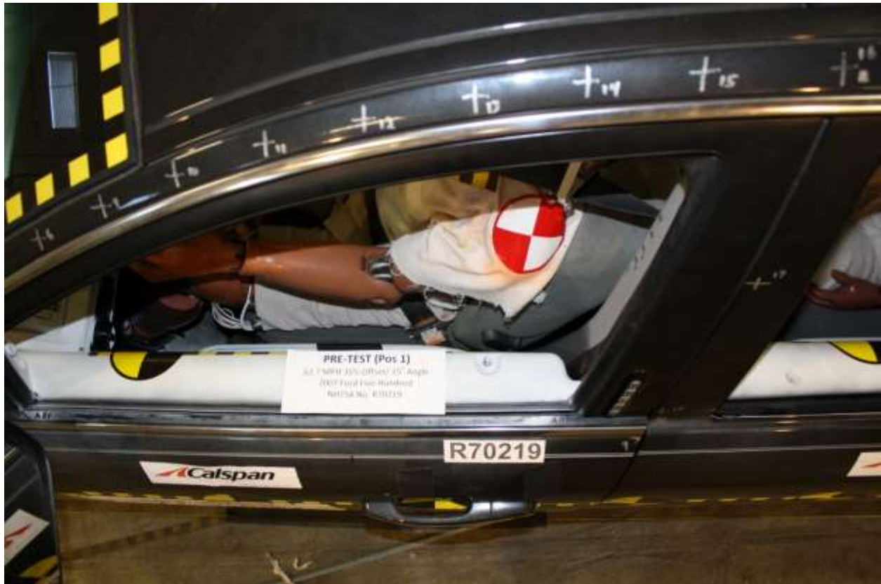
No. 062 Pre-Test View of Driver Dummy Door Clearance
