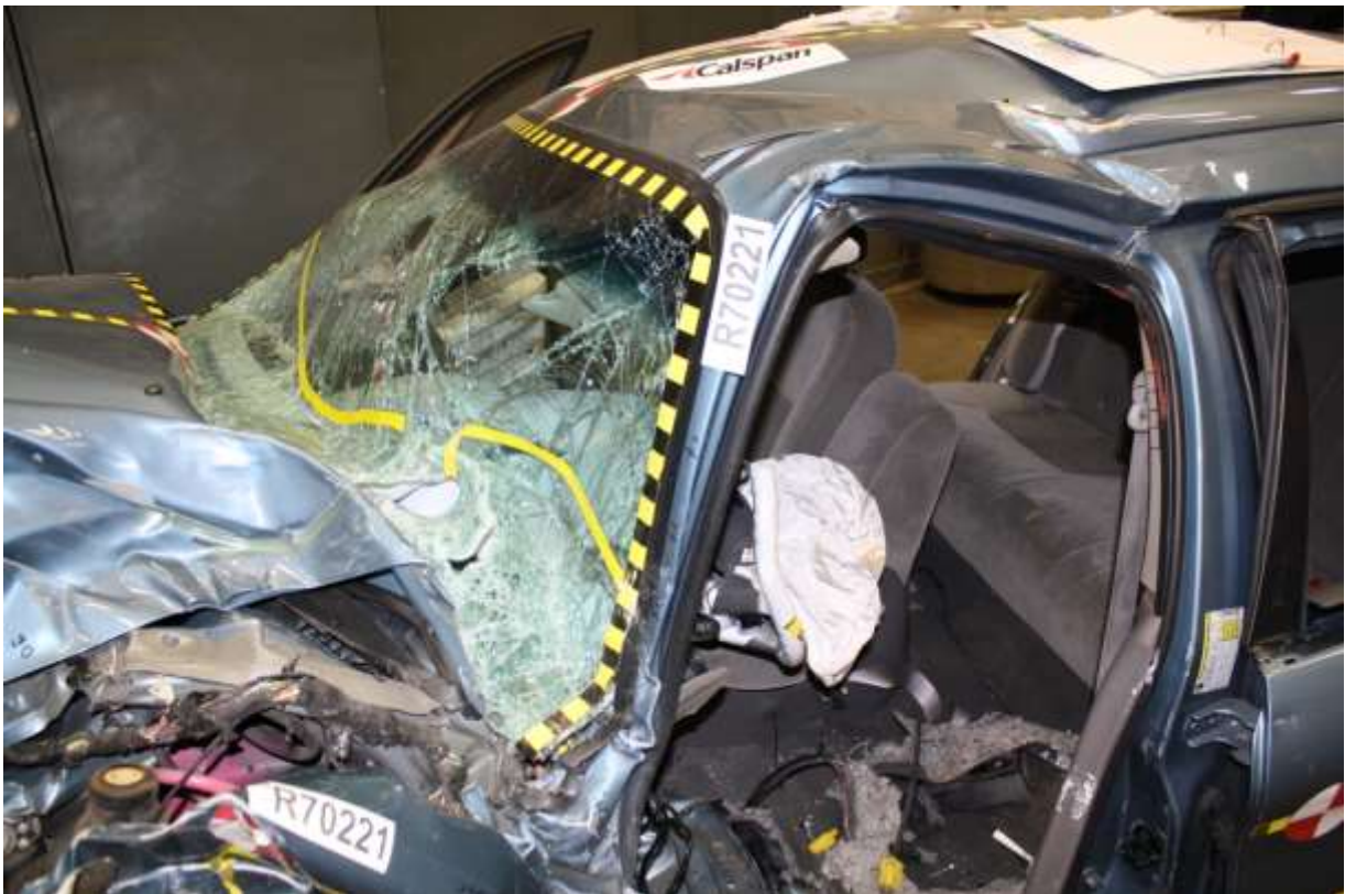
No. 127 Post-Test View of Windshield Separation
