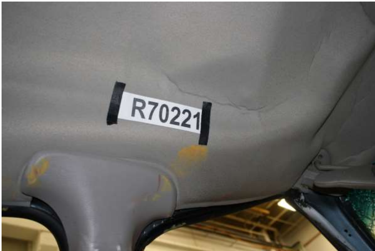
No. 082a Post-Test View of Driver Dummy Head Contact with Vehicle Interior
