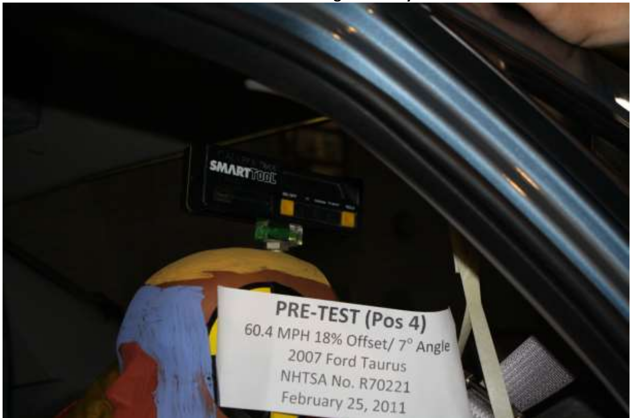
No. 093 Pre-Test Passenger View Showing Head Level
