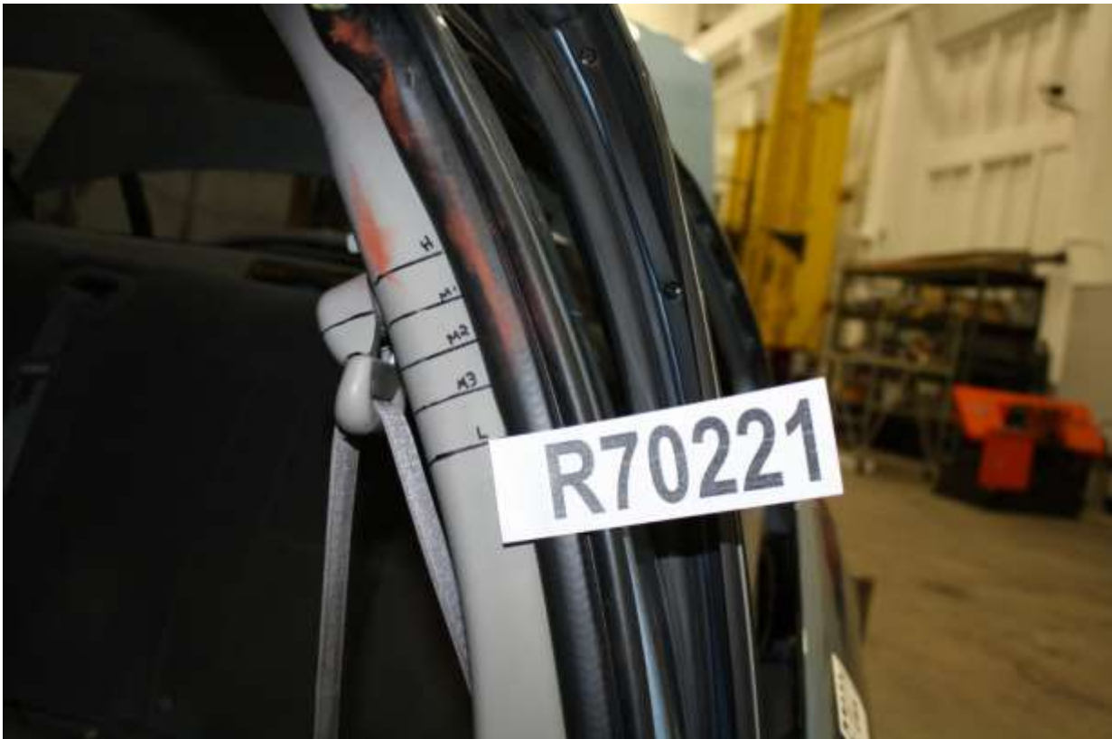
No. 082b Post-Test View of Driver Dummy Head Contact with Vehicle Interior
