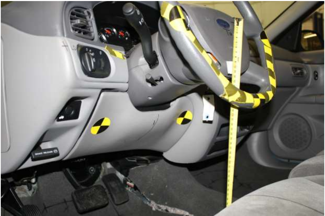
No. 042 Pre-Test Left Side View of Driver Knee Bolsters
