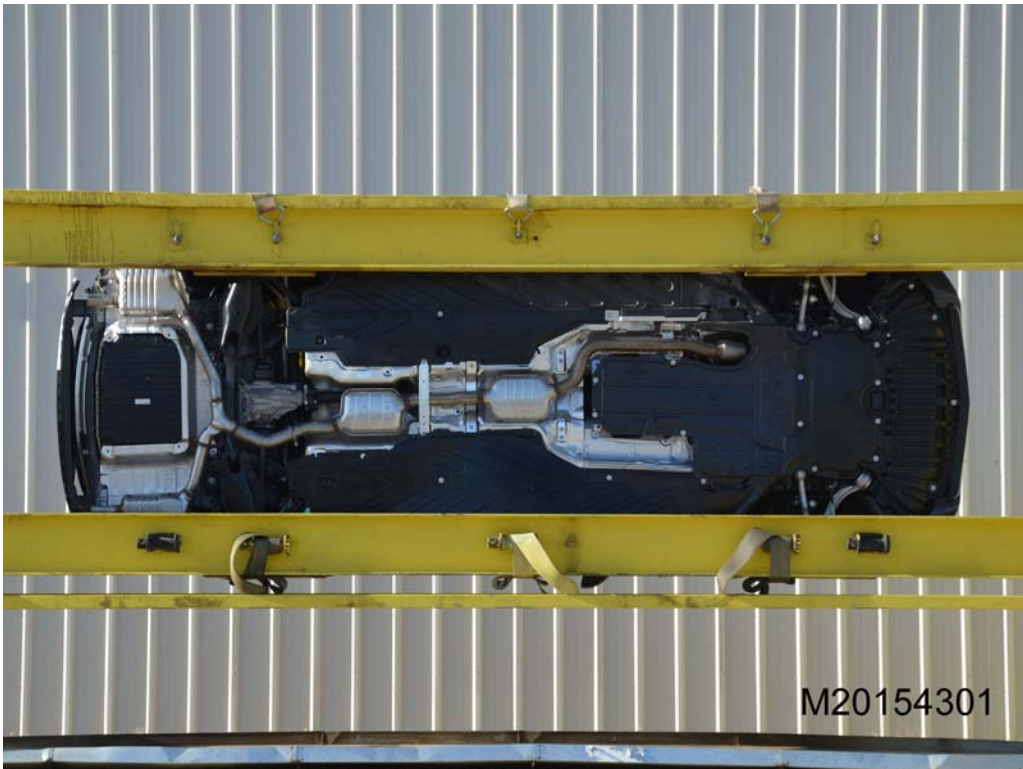
FIGURE 66. FMVSS No. 301 Static Rollover 270 Degrees
