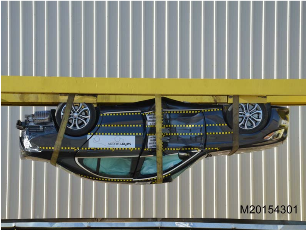
FIGURE 65. FMVSS No. 301 Static Rollover 180 Degrees
