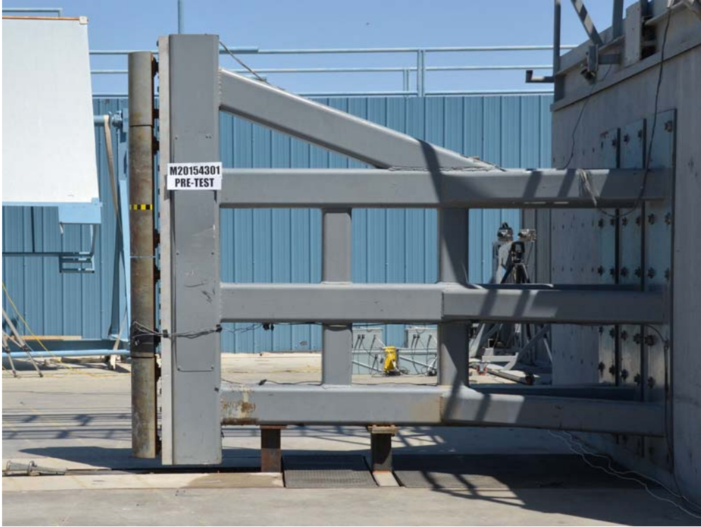
FIGURE 59. Pre-Test Pole Barrier Side View
