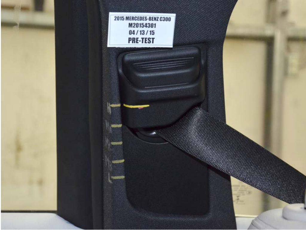
FIGURE 33. Pre-Test View of Belt Anchorage for Dummy
