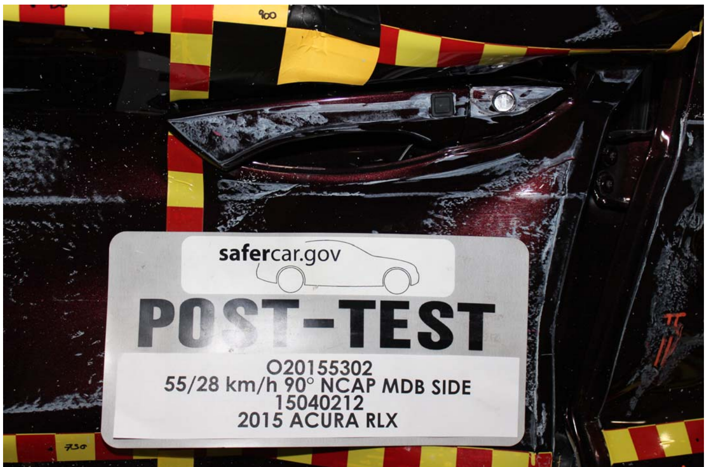
No. 024 - Post-Test Left Rear Door Latch Close-Up
