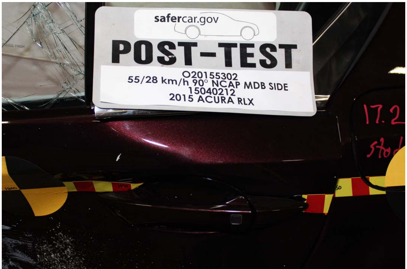
No. 022 - Post-Test Left Front Door Latch Close-Up
