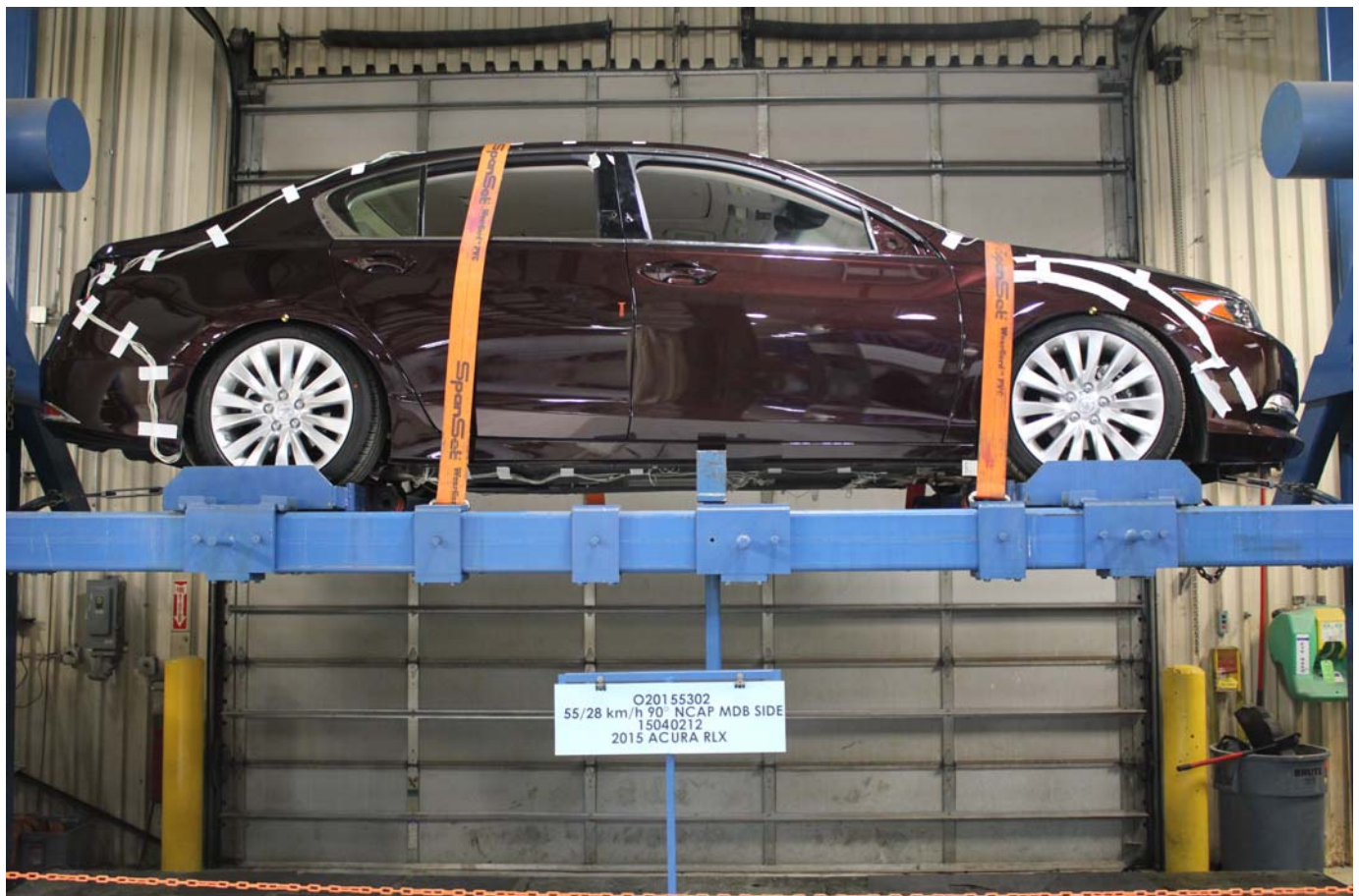
No. 096 - FMVSS No. 301 Static Rollover 0 Degrees
