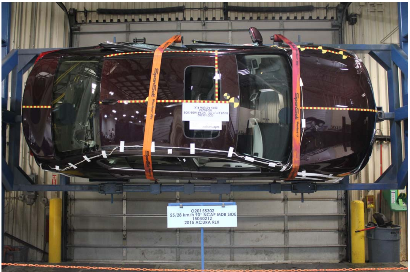
No. 099 - FMVSS No. 301 Static Rollover 270 Degrees
