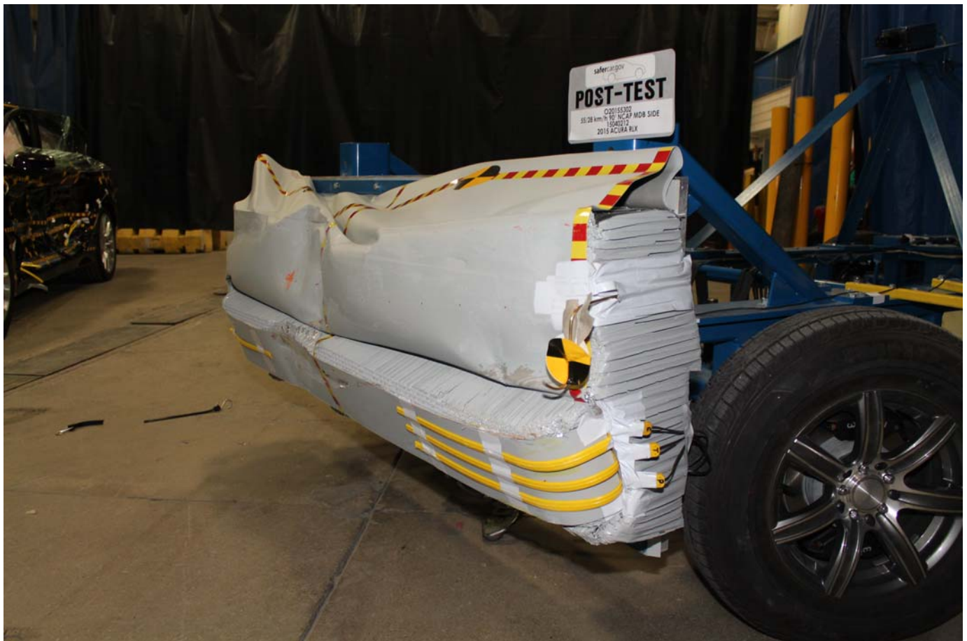
No. 089 - Post-Test Left Side View of MDB Impactor Face
