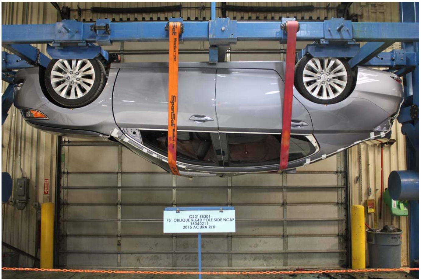
No. 065 - FMVSS No. 301 Static Rollover 180 Degrees
