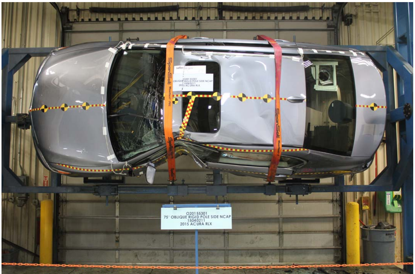
No. 064 - FMVSS No. 301 Static Rollover 90 Degrees
