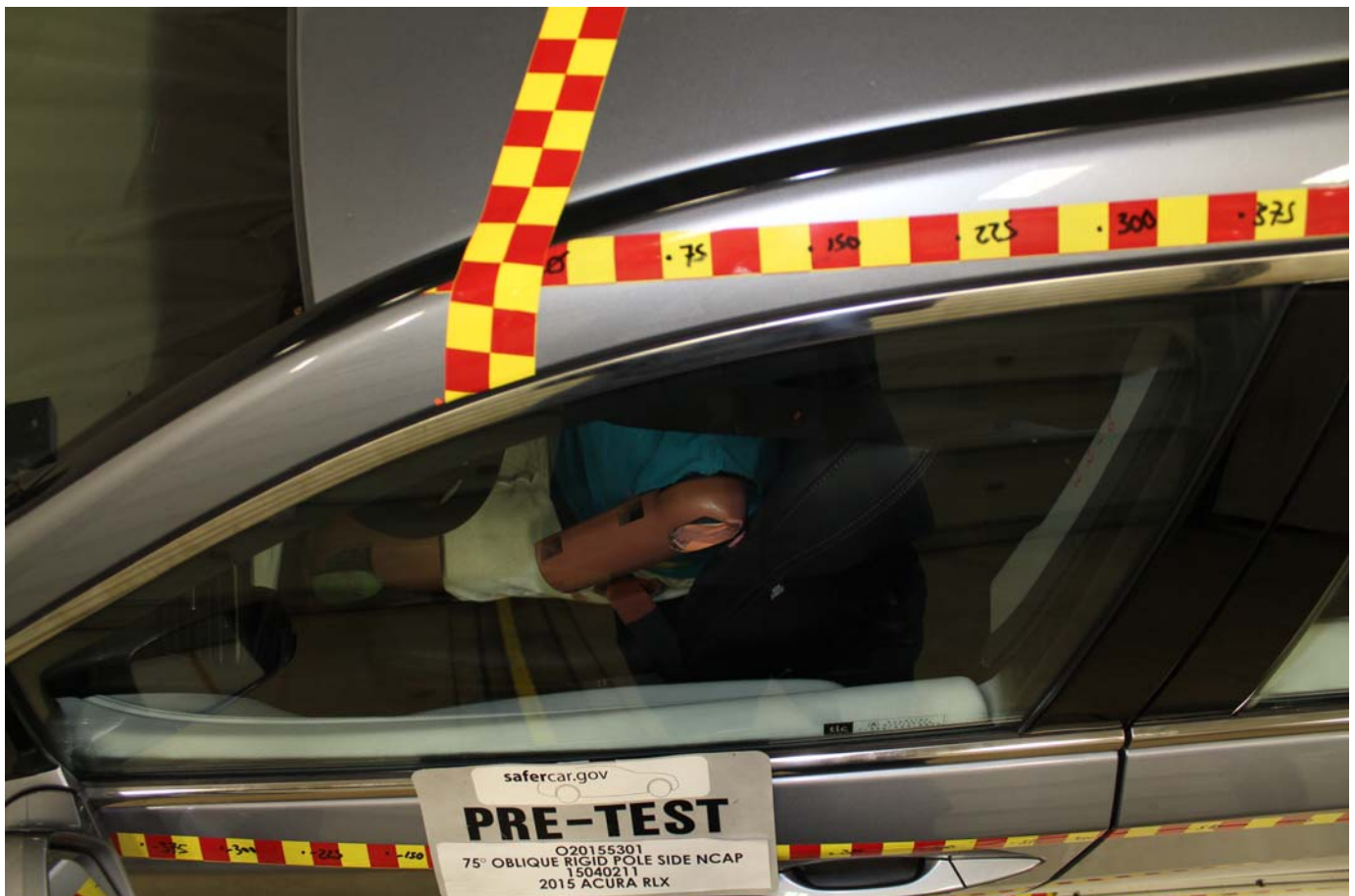
No. 040 - Pre-Test Dummy and Door Clearance View
