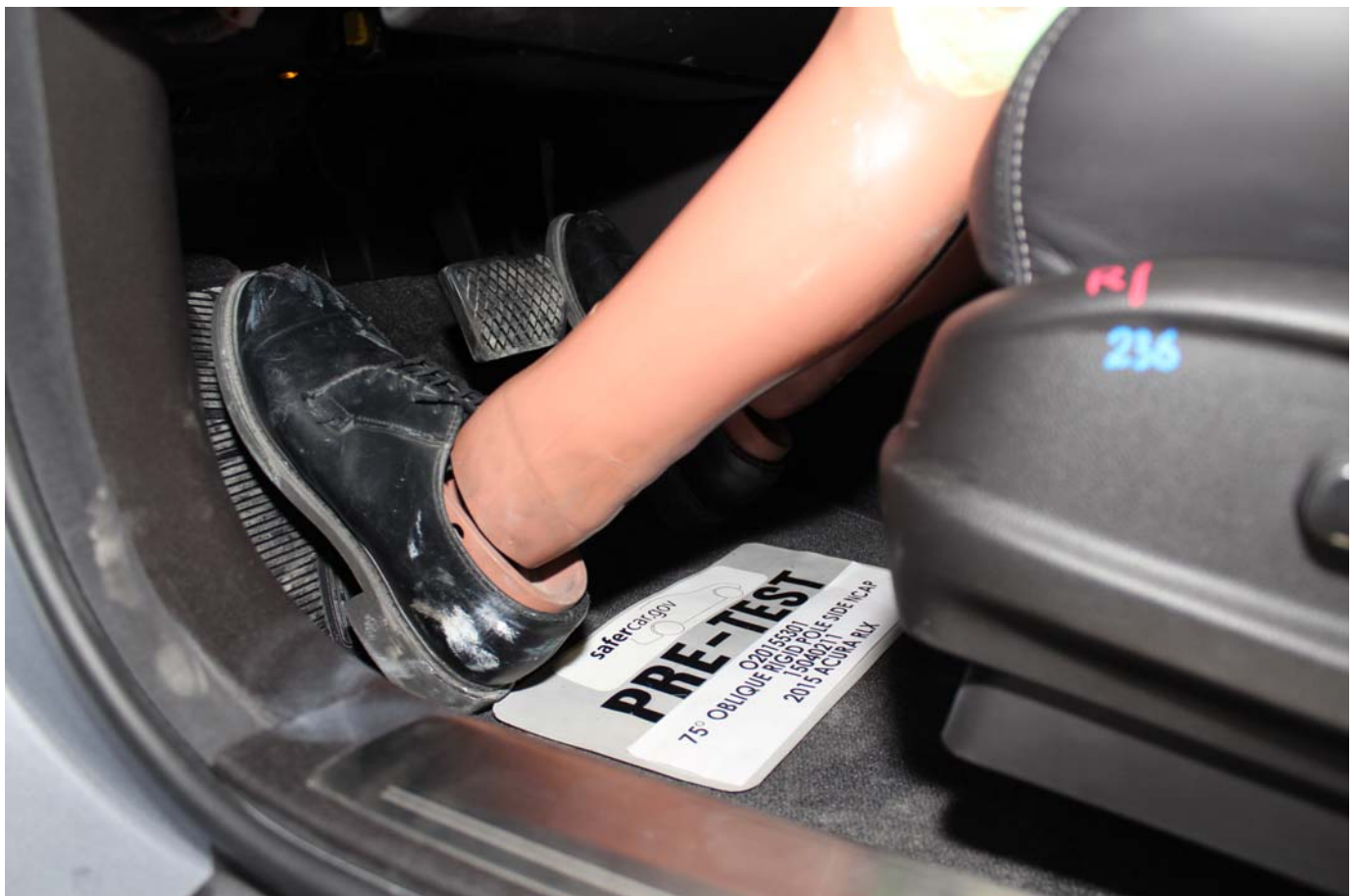
No. 032 - Pre-Test Placement of Dummy's Feet
