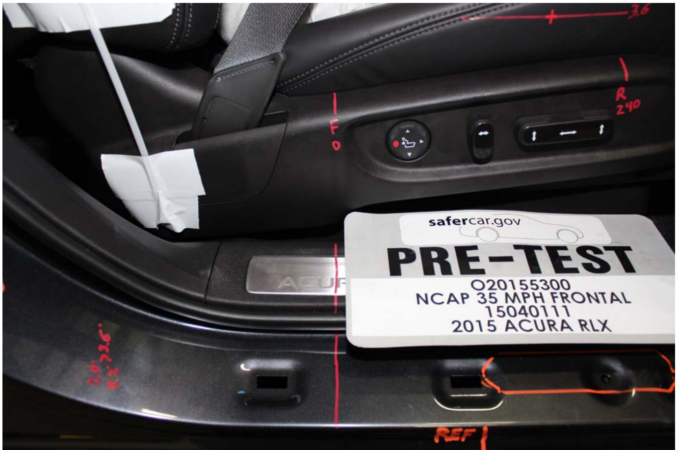
No. 061 - Pre-Test Passenger's Seat Fore-Aft Markings
