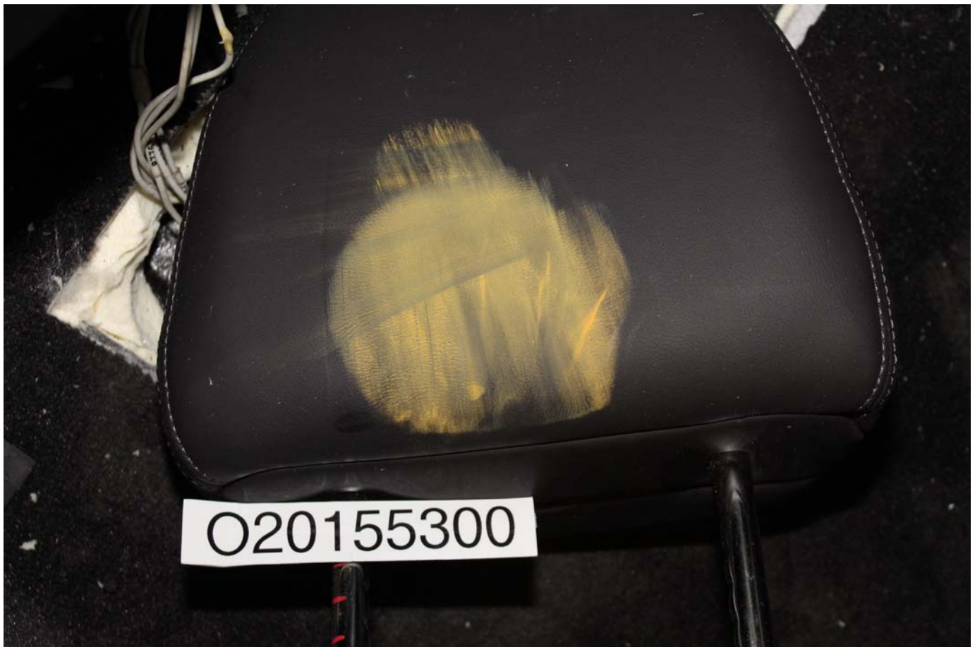
No. 073 - Post-Test Passenger Dummy Contact with Headrest
