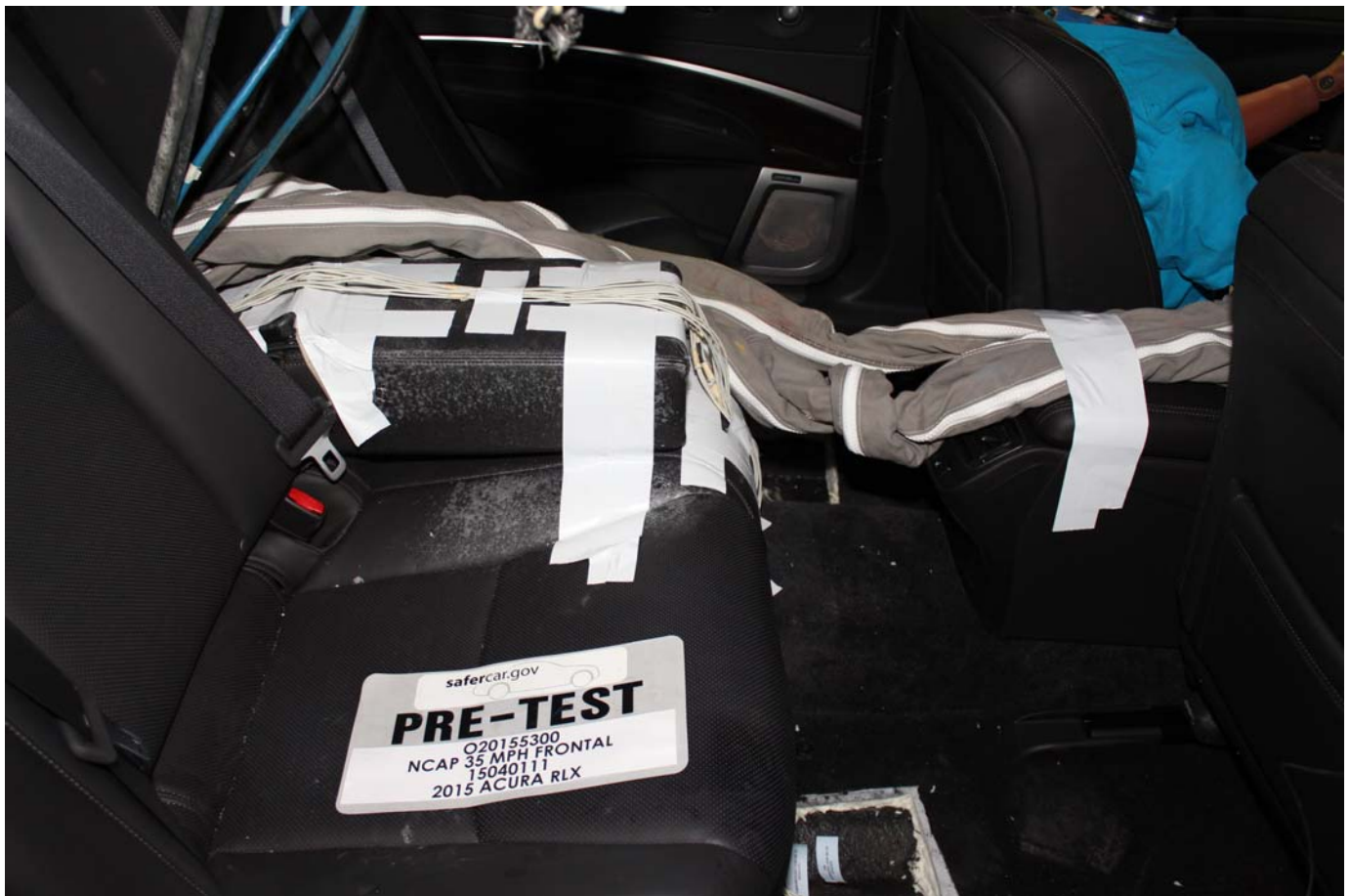
No. 031 - Pre-Test Dummy Cable Routing
