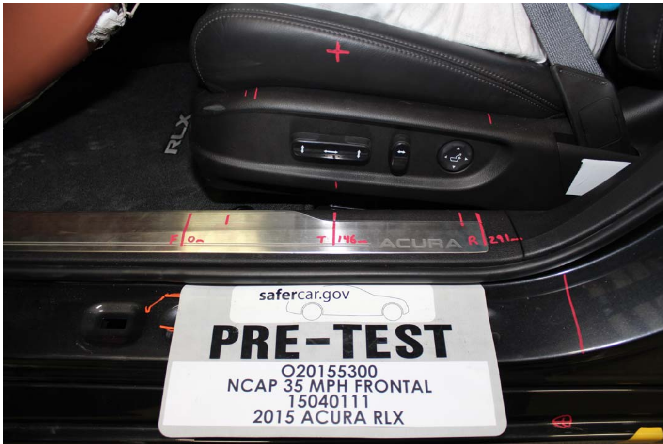
No. 039 - Pre-Test Driver's Seat Fore-Aft Markings
