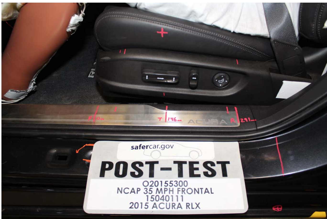
No. 040 - Post-Test Driver's Seat Fore-Aft Markings
