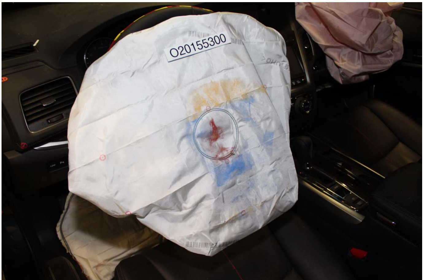
No. 050 - Post-Test Driver Dummy Contact with Airbag
