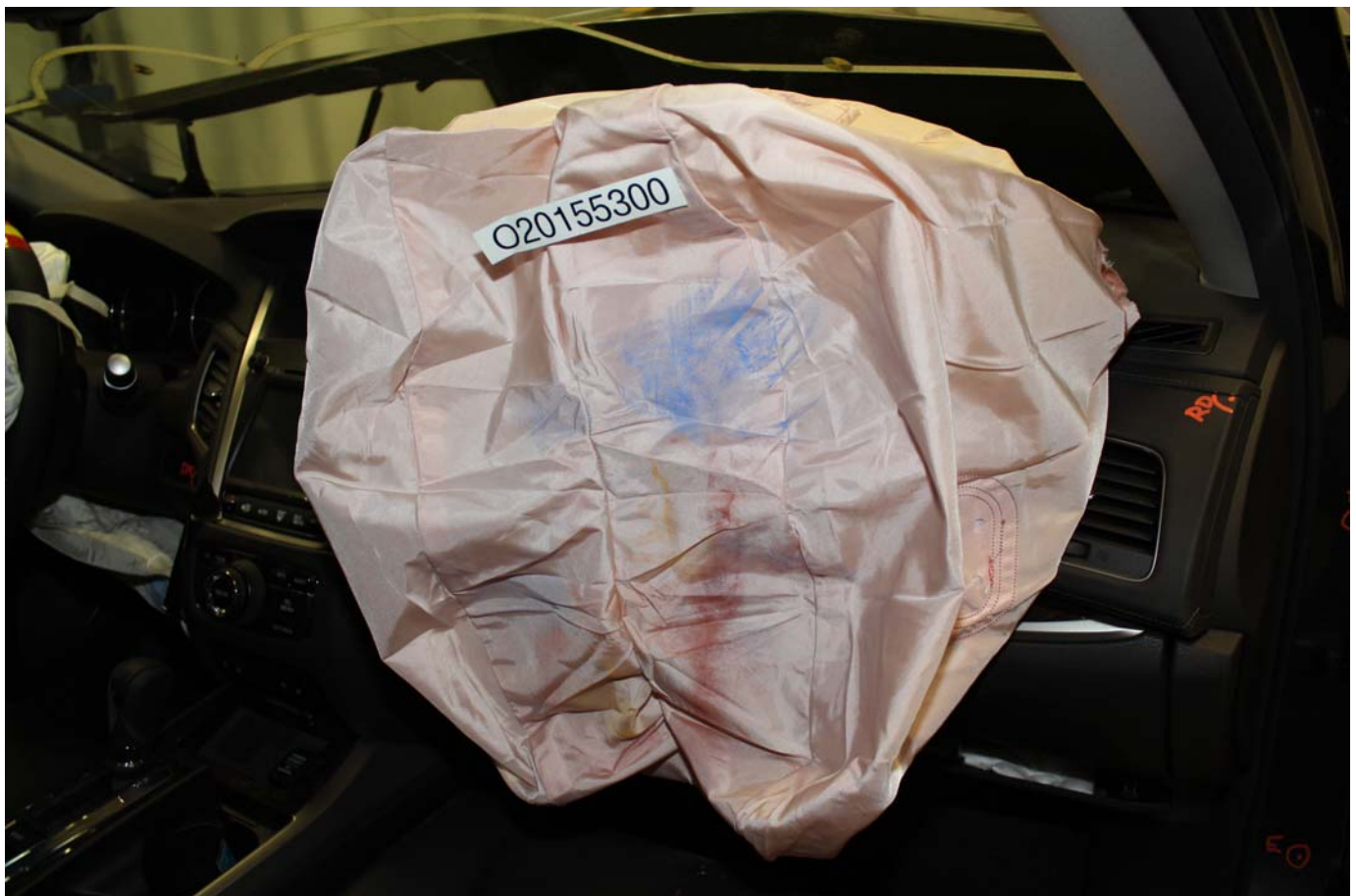
No. 072 - Post-Test Passenger Dummy Contact with Airbag
