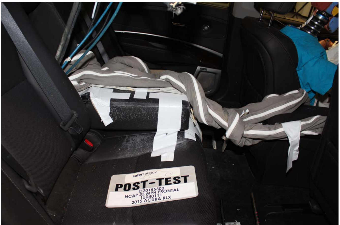
No. 032 - Post-Test Dummy Cable Routing
