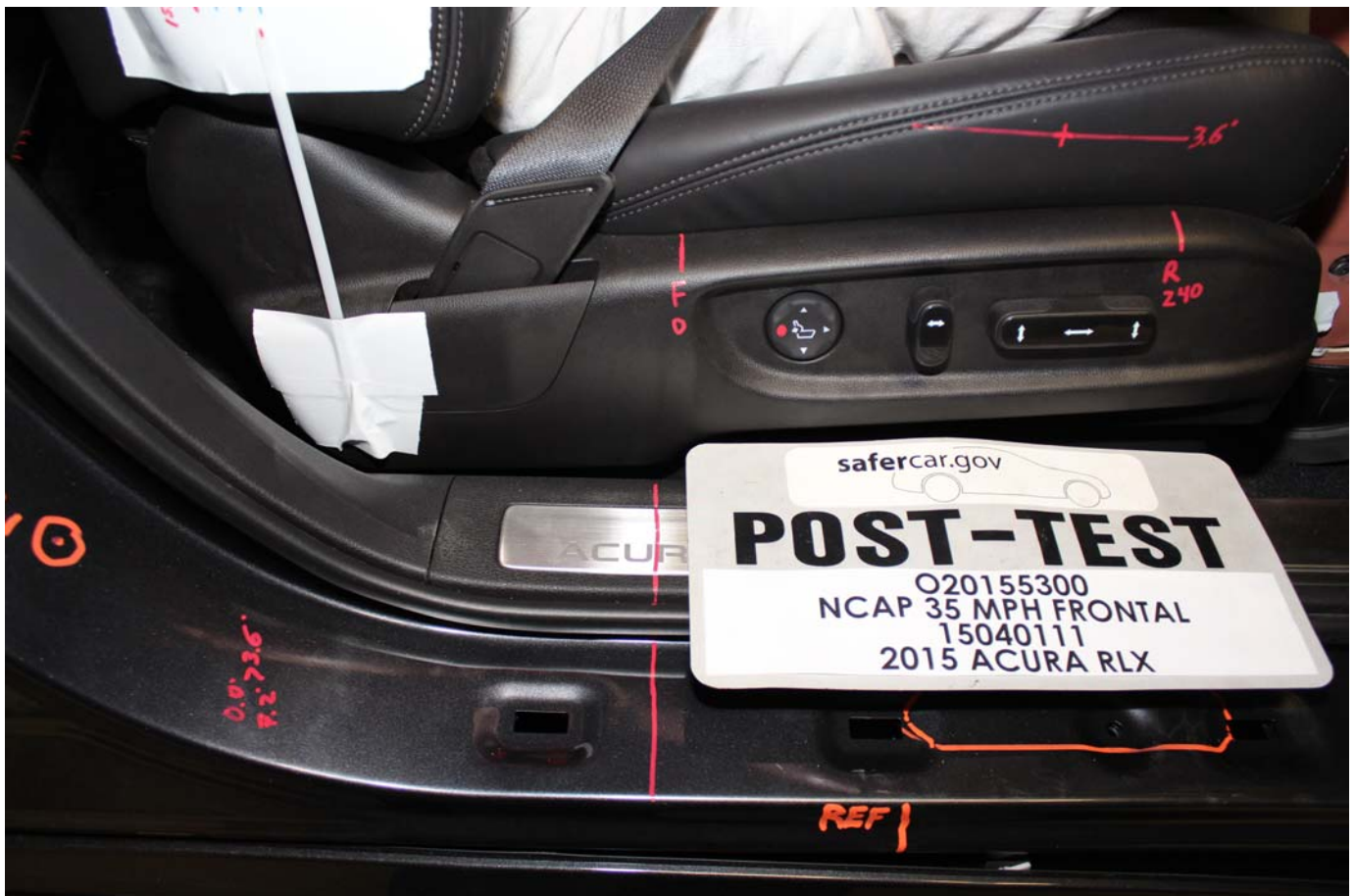
No. 062 - Post-Test Passenger's Seat Fore-Aft Markings
