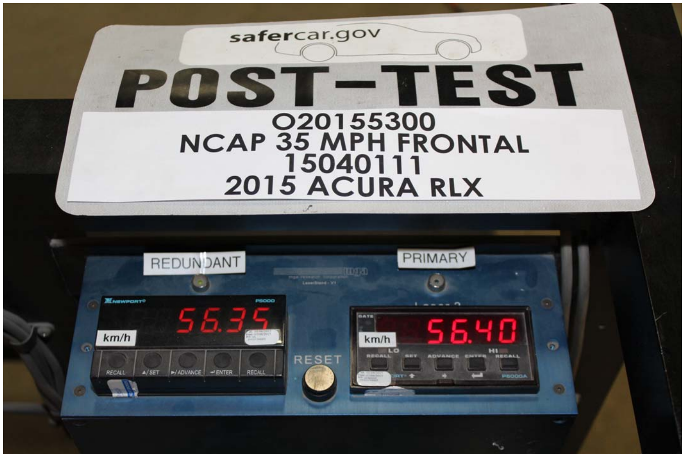
No. 077 - Post-Test Speed Trap Read-Out
