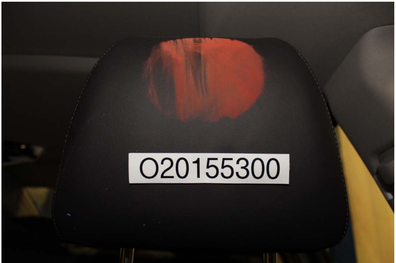
No. 051 - Post-Test Driver Dummy Contact with Headrest
