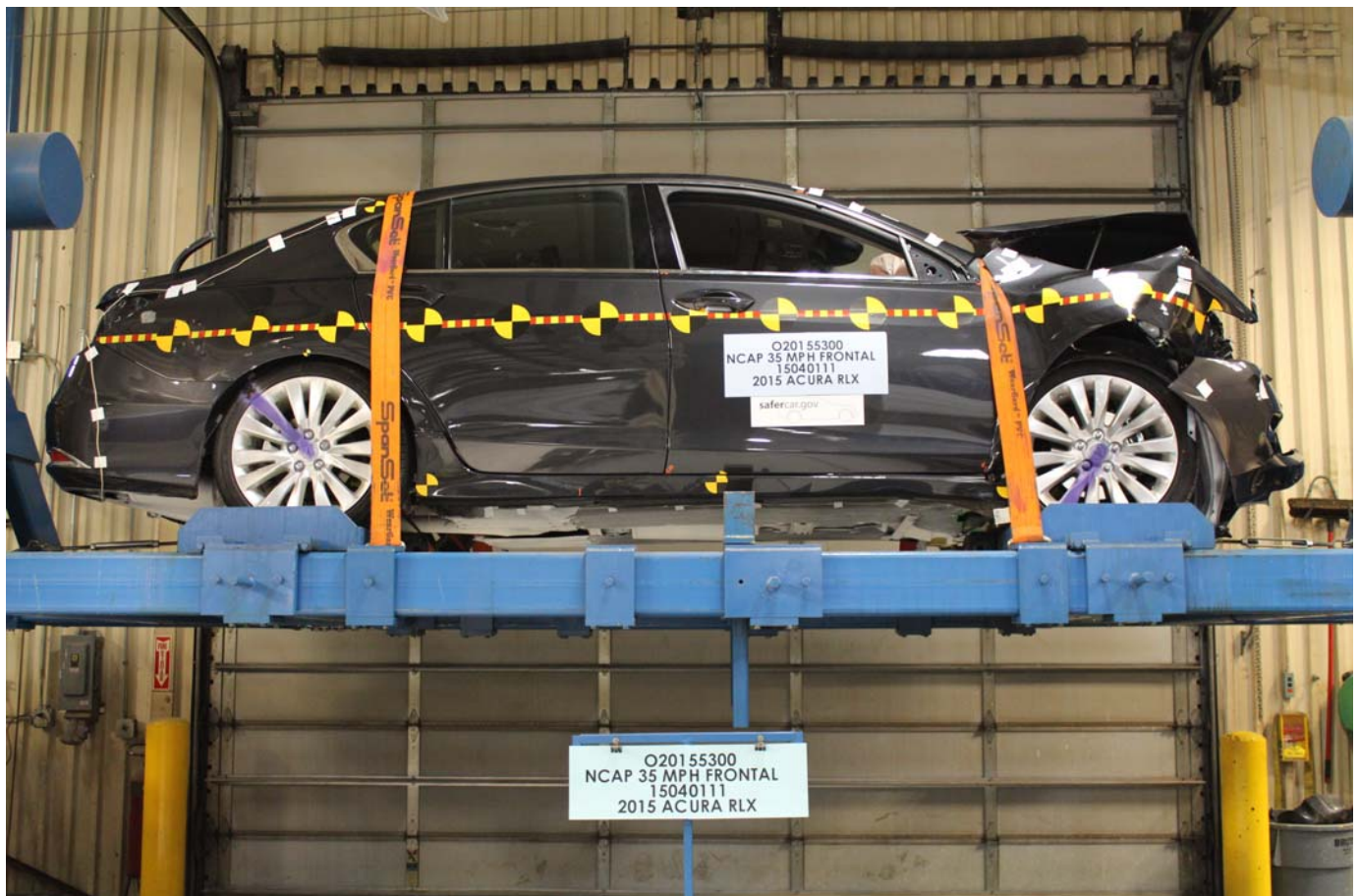
No. 078 - Vehicle at 0 Degree on Static Rollover Device
