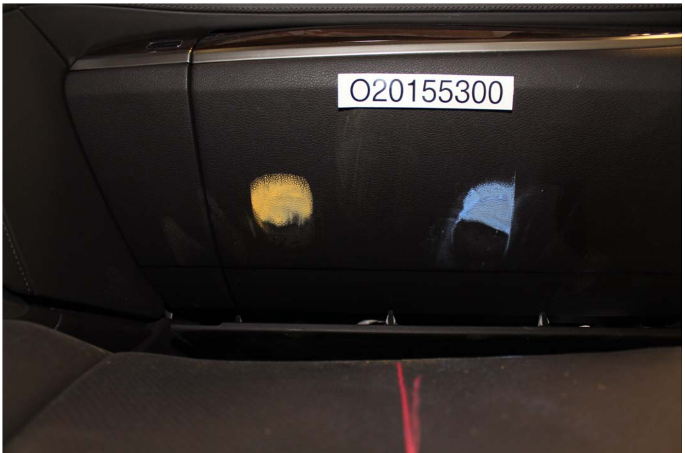
No. 074 - Post-Test Passenger Dummy Contact with Glovebox
