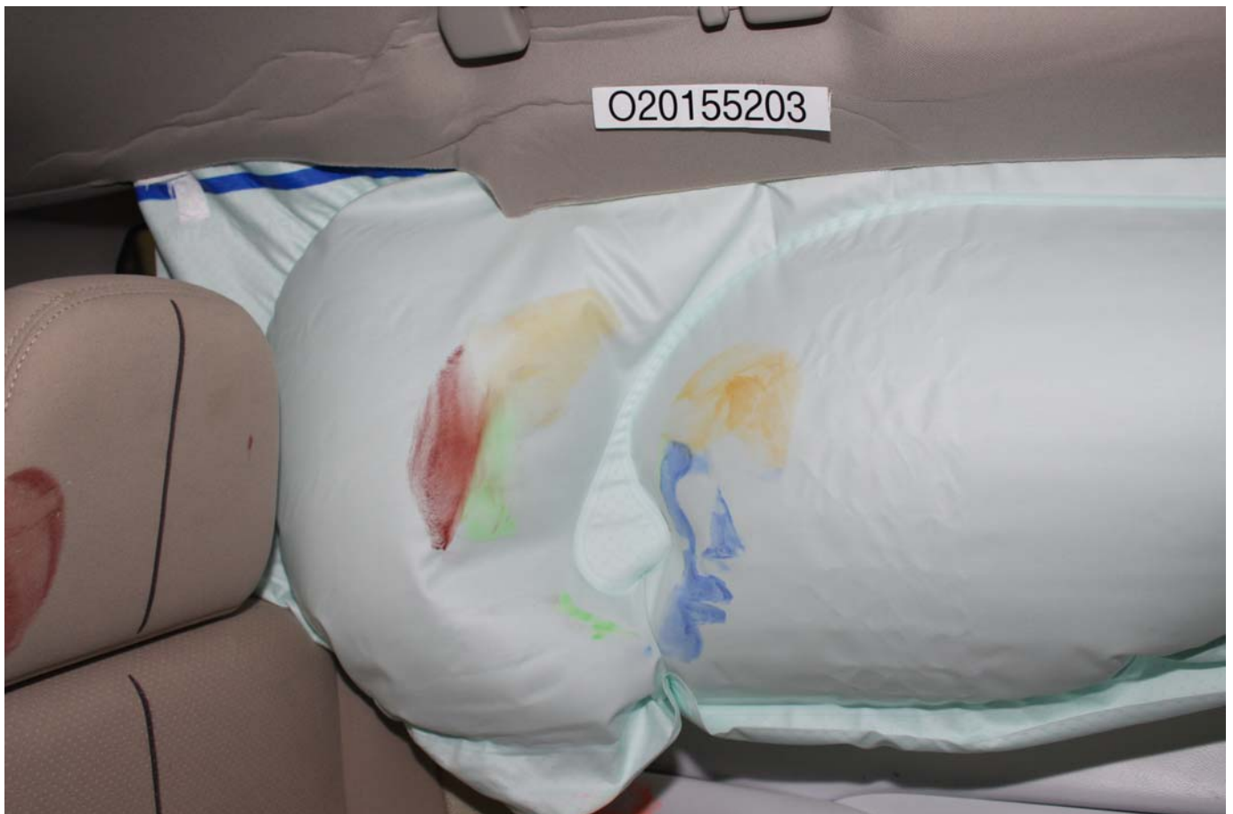
No. 076 - Post-Test Rear Passenger Dummy Close-up Head Contact with Side Airbag View
