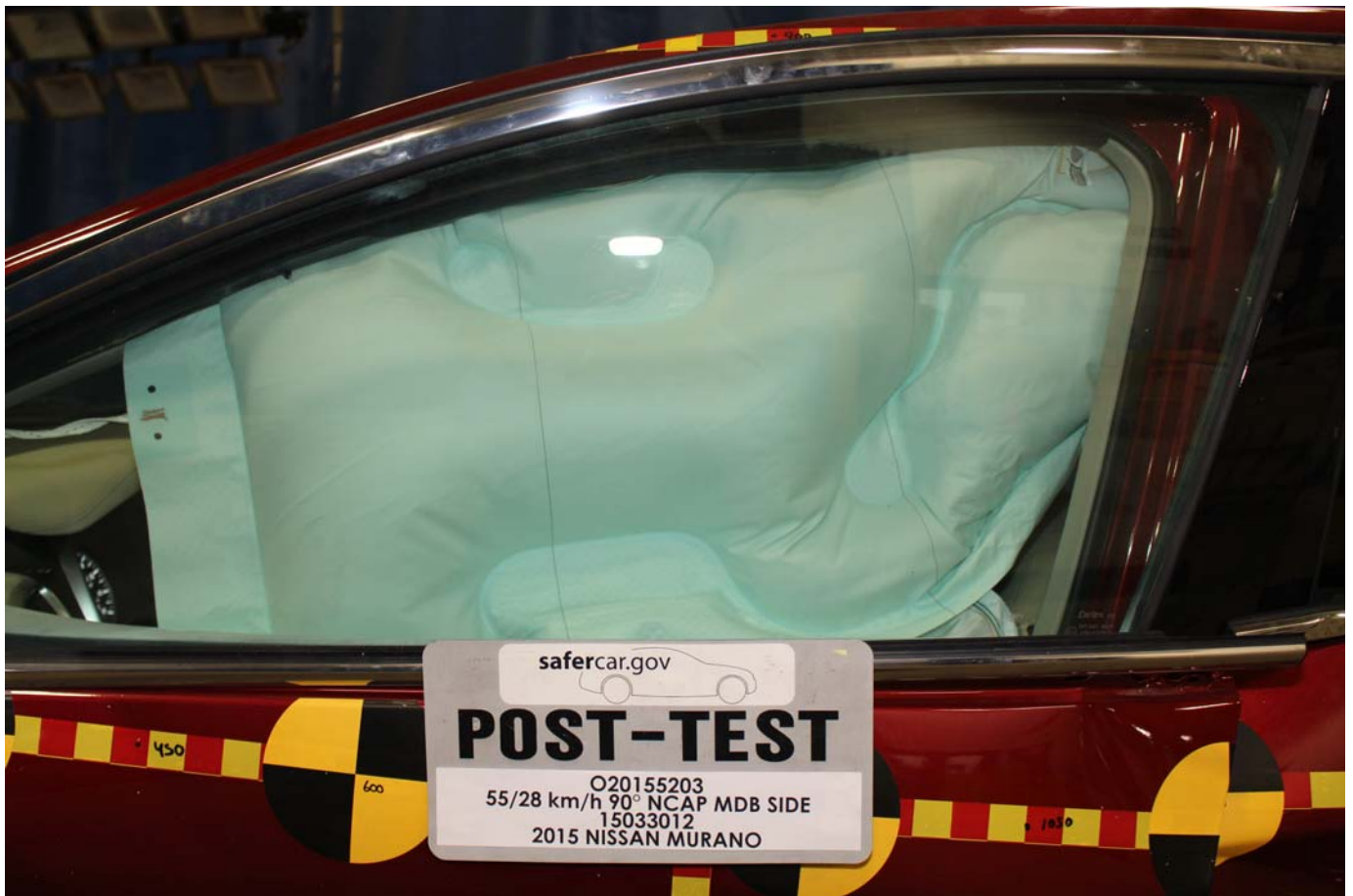
No. 029 - Post-Test Left Side View of Driver Dummy Shoulder and Door Top View
