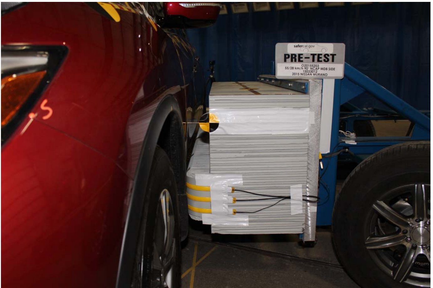
No. 017 - Pre-Test Left Side View of MDB Positioned Against Side of Test Vehicle
