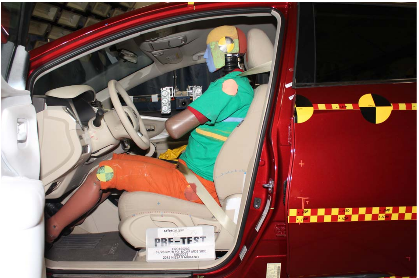
No. 027 - Pre-Test Left Side View of Driver Dummy Showing Belt and Chalking
