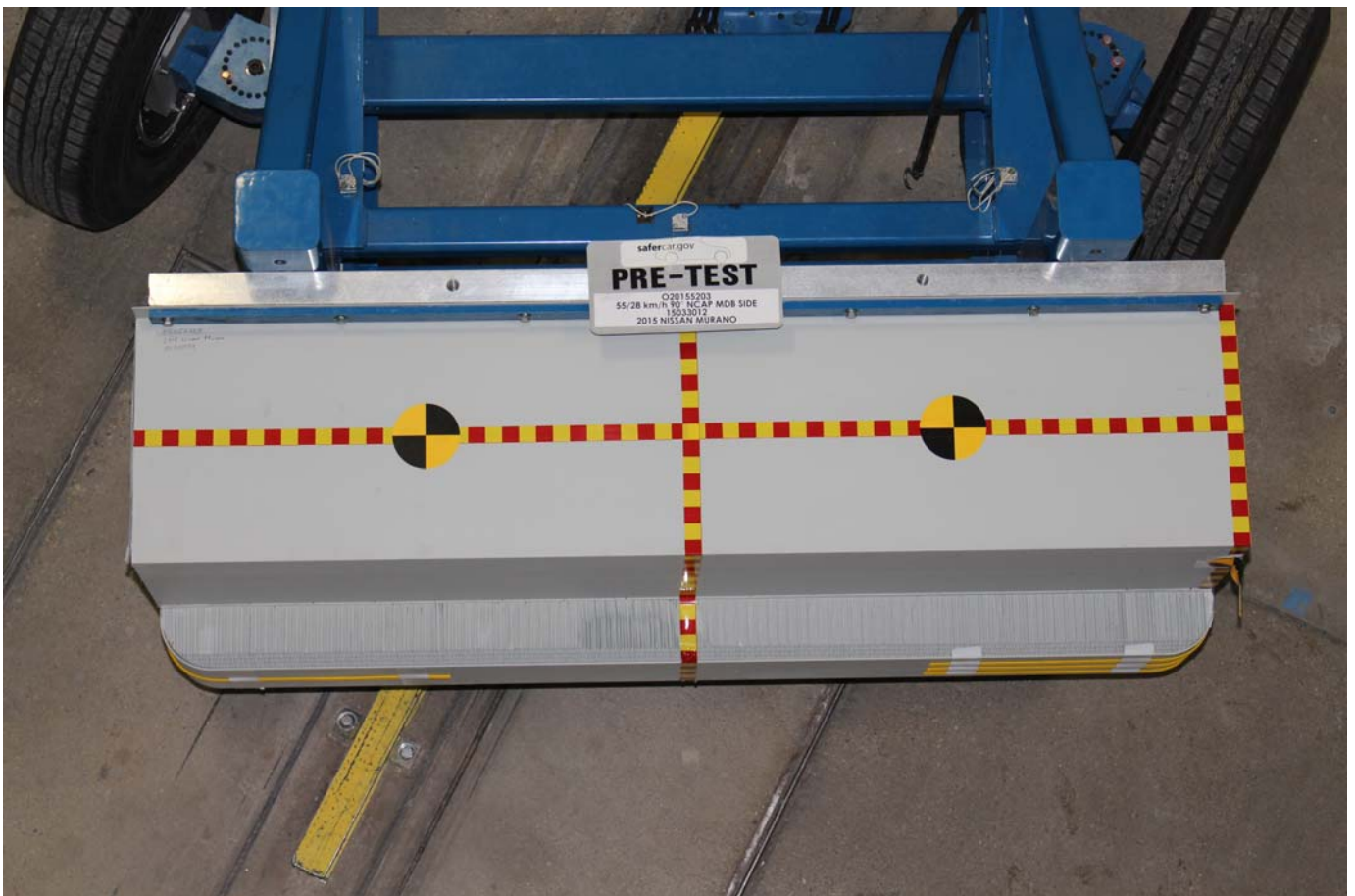
No. 086 - Pre-Test Top View of MDB Impactor Face
