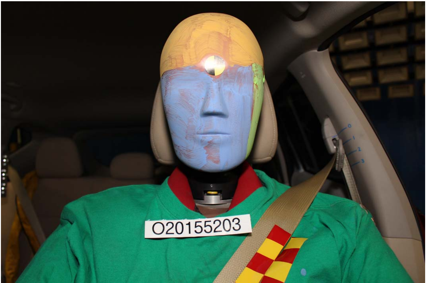
No. 031 - Pre-Test Frontal View of Driver Dummy Head and Shoulders in Relation to Head Restraint
