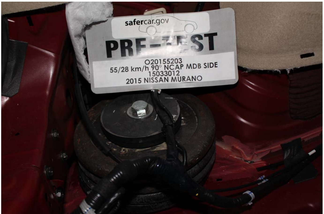
No. 094 - Pre-Test Ballast View
