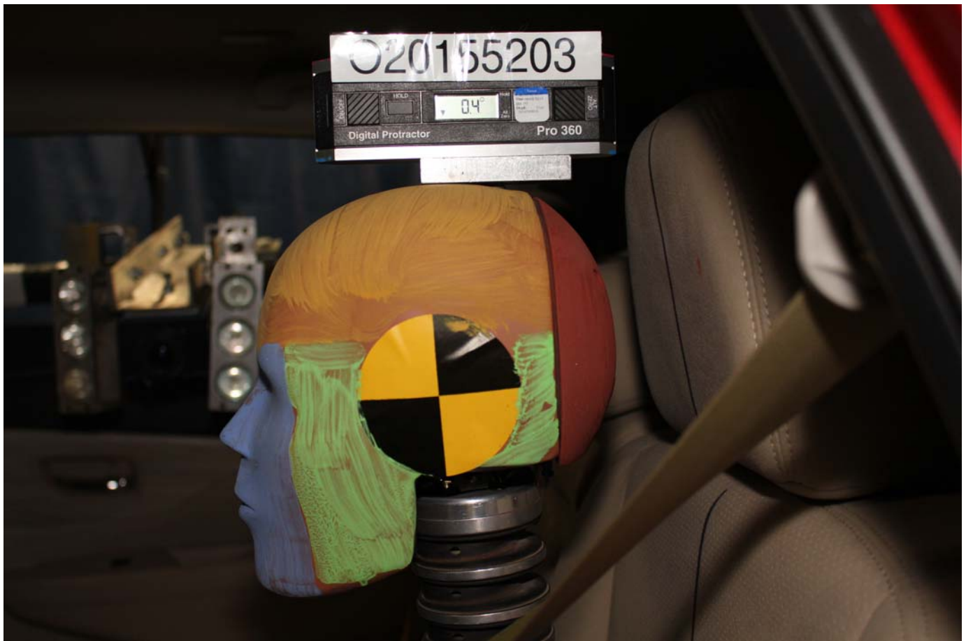
No. 063 - Pre-Test View of Rear Passenger Dummy's Head Showing Dummy's Head is Level
