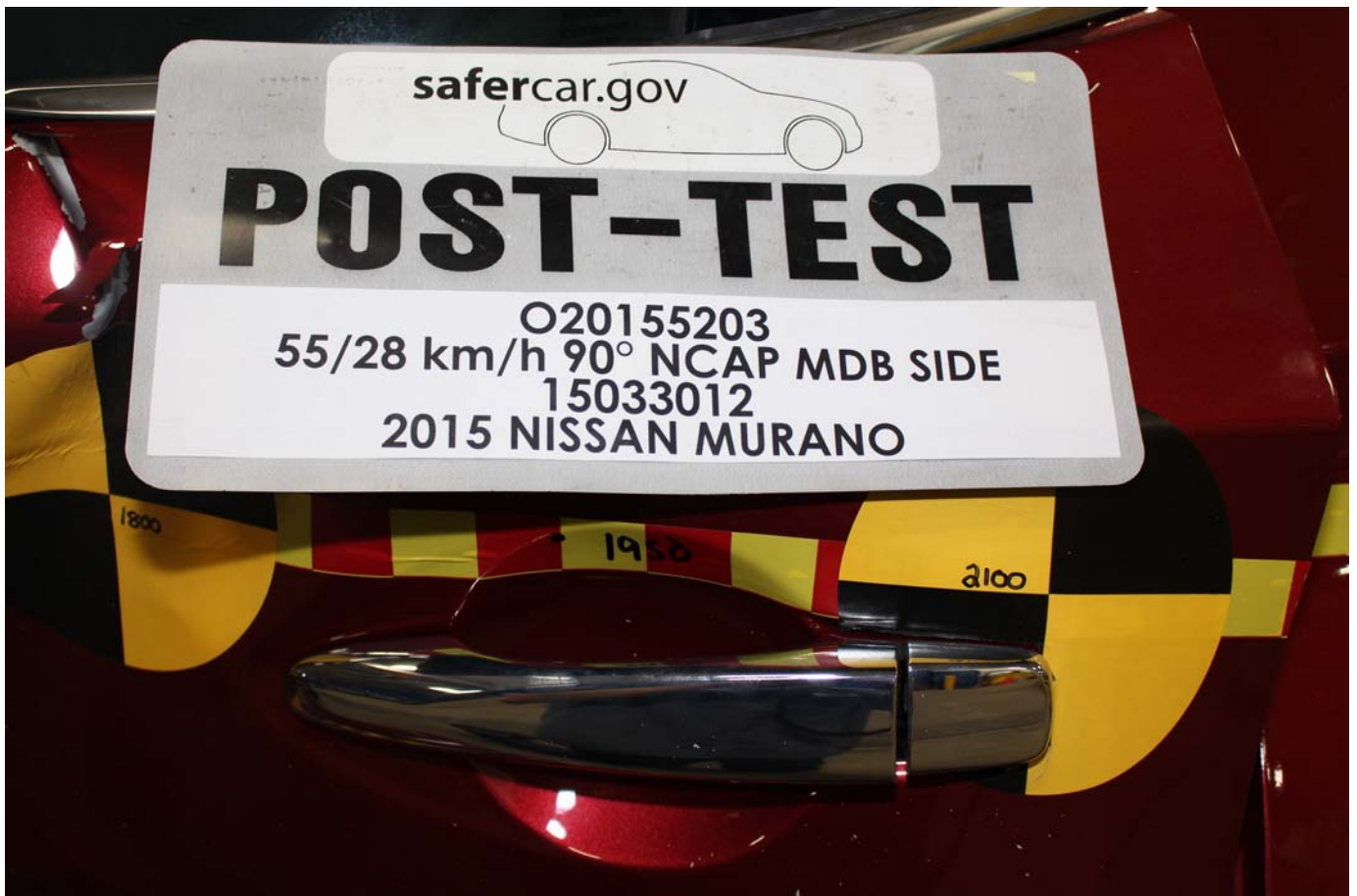
No. 024 - Post-Test Left Rear Door Latch Close-Up
