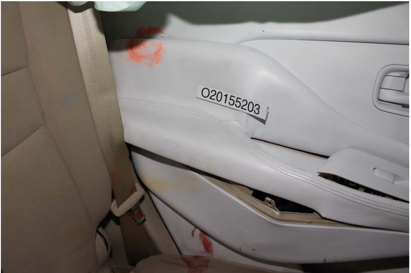
No. 077 - Post-Test Rear Passenger Dummy Close-up Torso Contact with Vehicle Interior View
