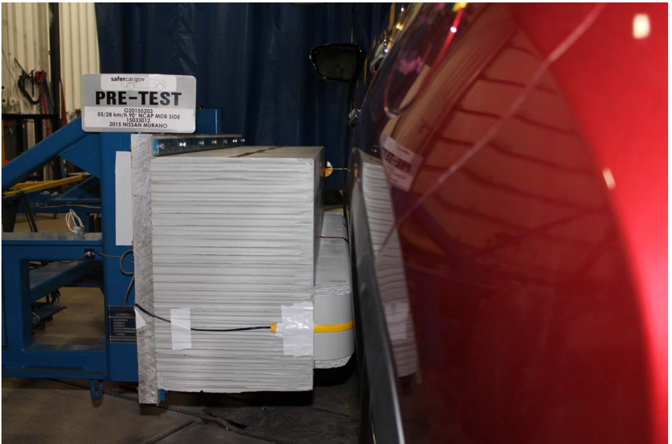
No. 018 - Pre-Test Right Side View of MDB Positioned Against Side of Test Vehicle
