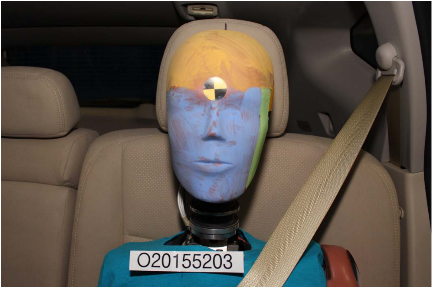
No. 059 - Pre-Test Frontal View of Rear Passenger Dummy Head and Shoulders in Relation to Head Restraint
