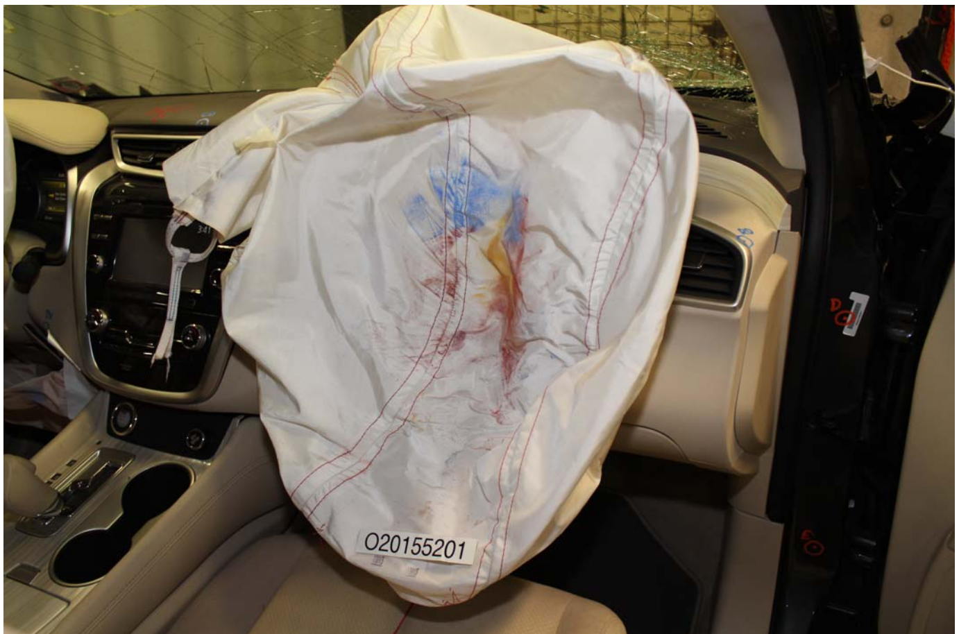
No. 072 - Post-Test Passenger Dummy Contact with Airbag
