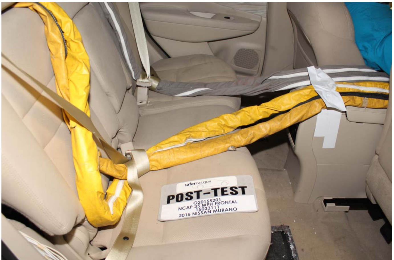
No. 032 - Post-Test Dummy Cable Routing
