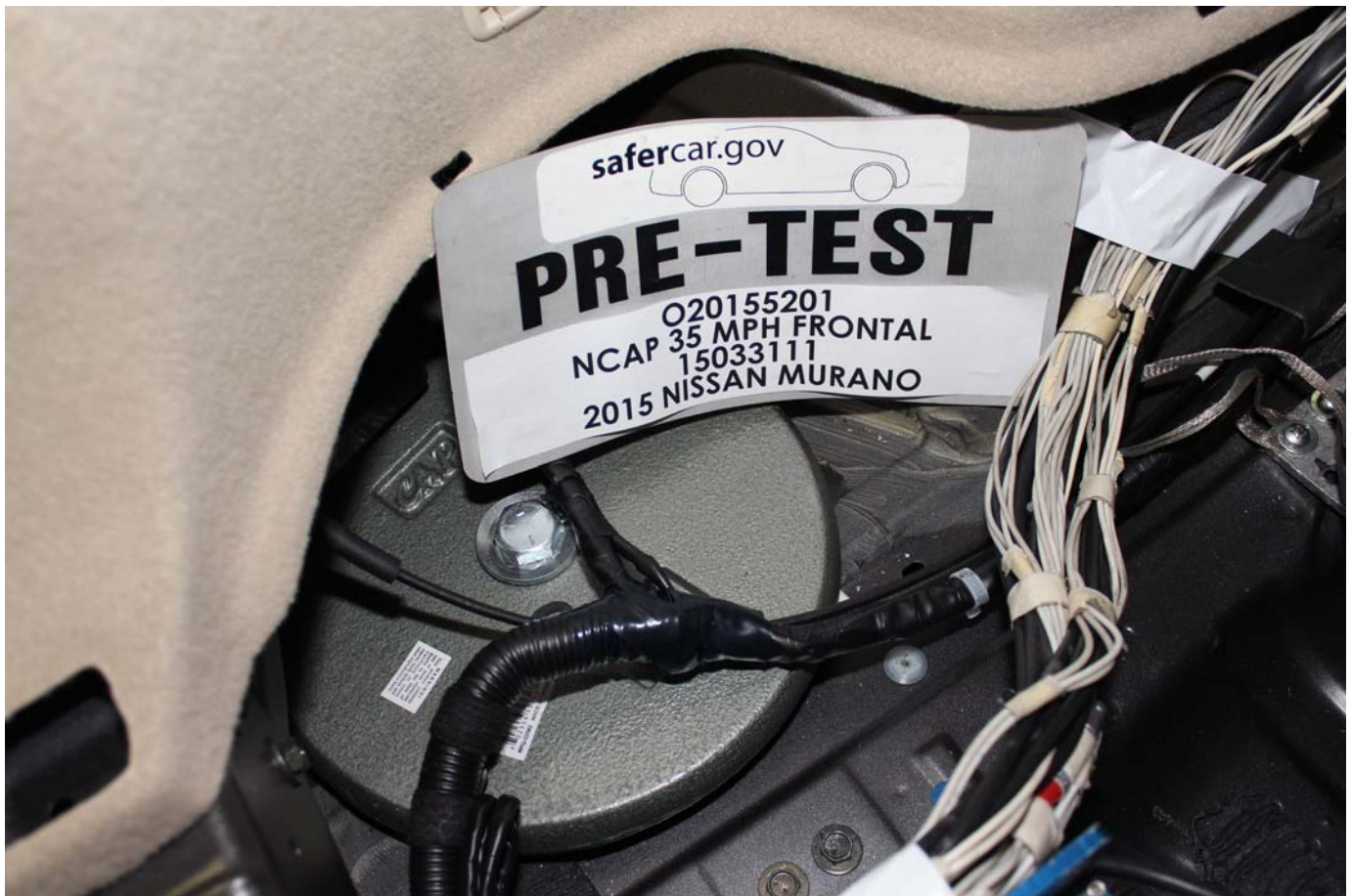
No. 075 - Ballast Installed in Vehicle
