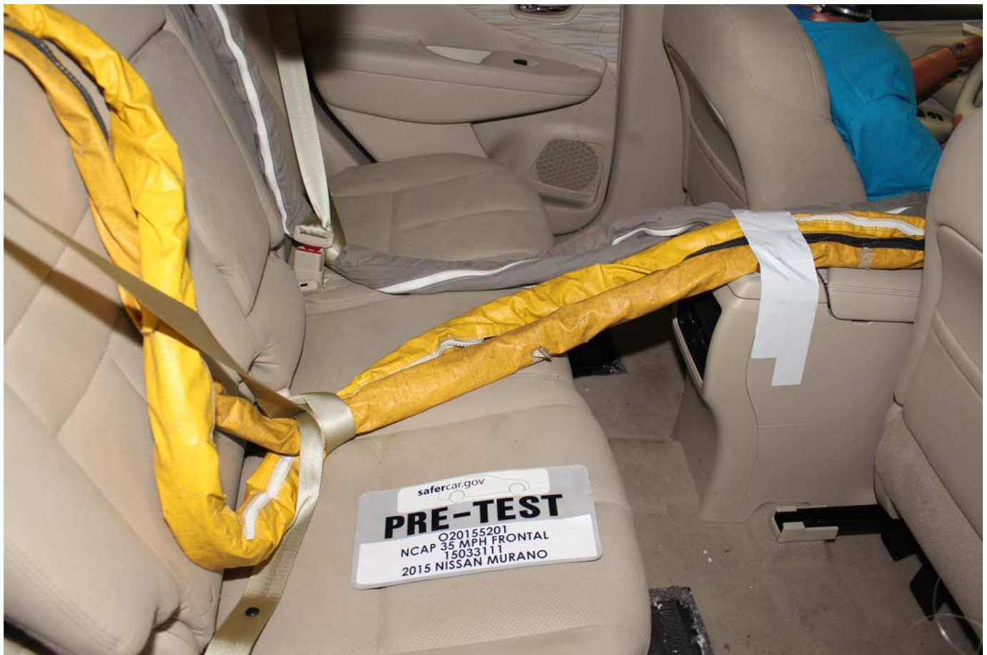
No. 031 - Pre-Test Dummy Cable Routing
