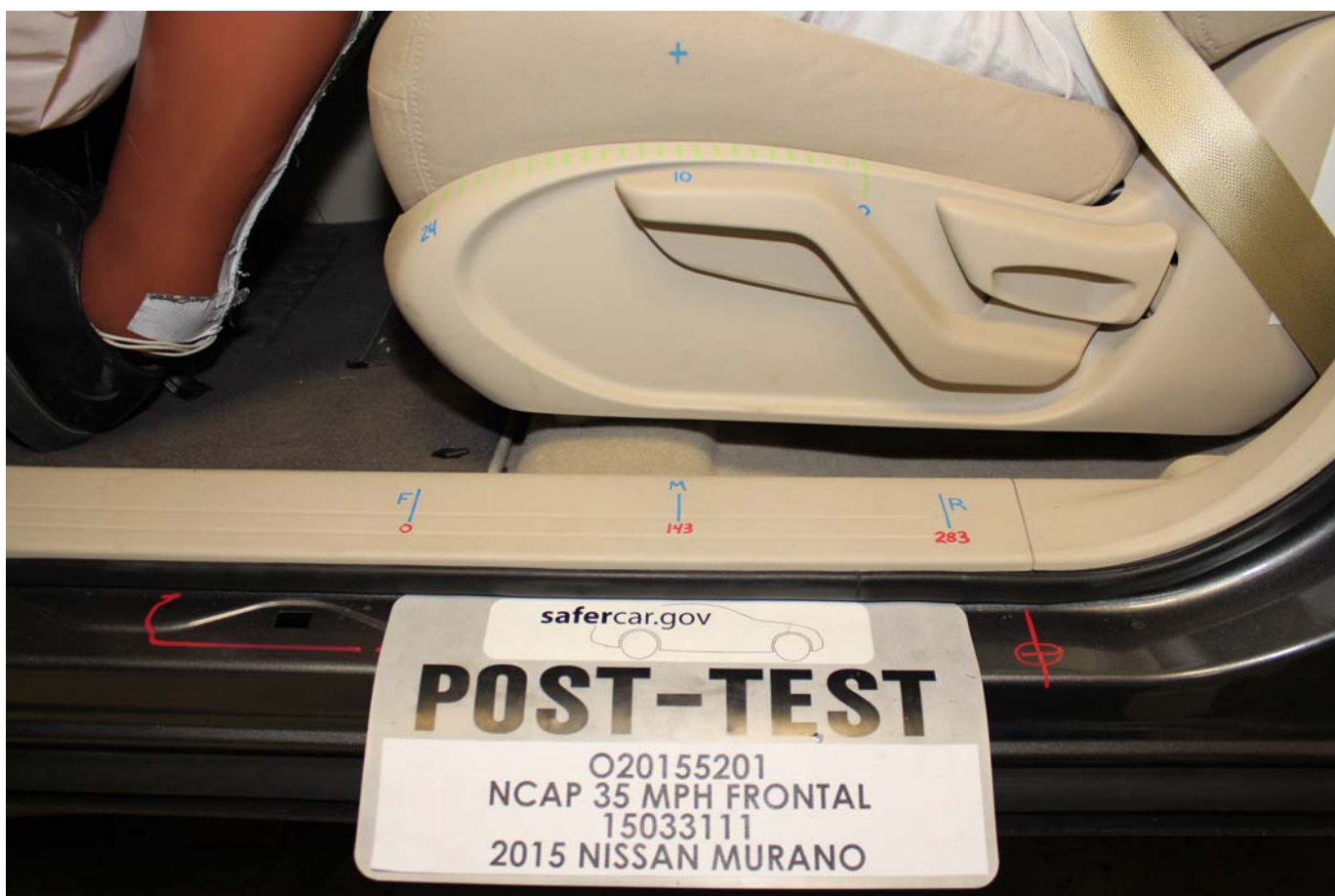
No. 040 - Post-Test Driver's Seat Fore-Aft Markings
