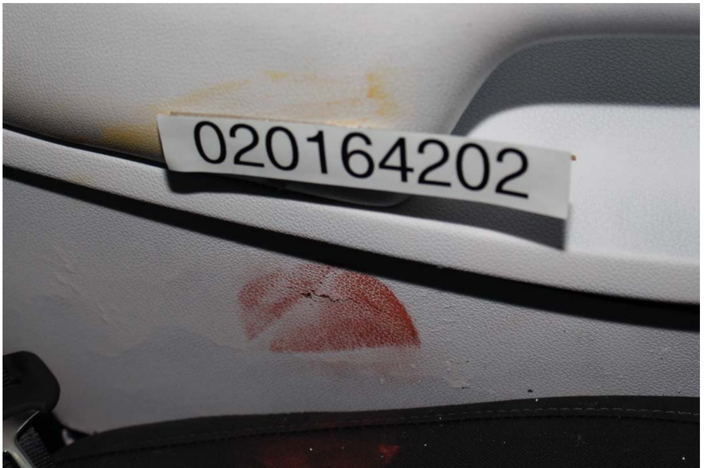
No. 079 - Post-Test Rear Passenger Dummy Close-up Pelvis Contact with Vehicle Interior View
