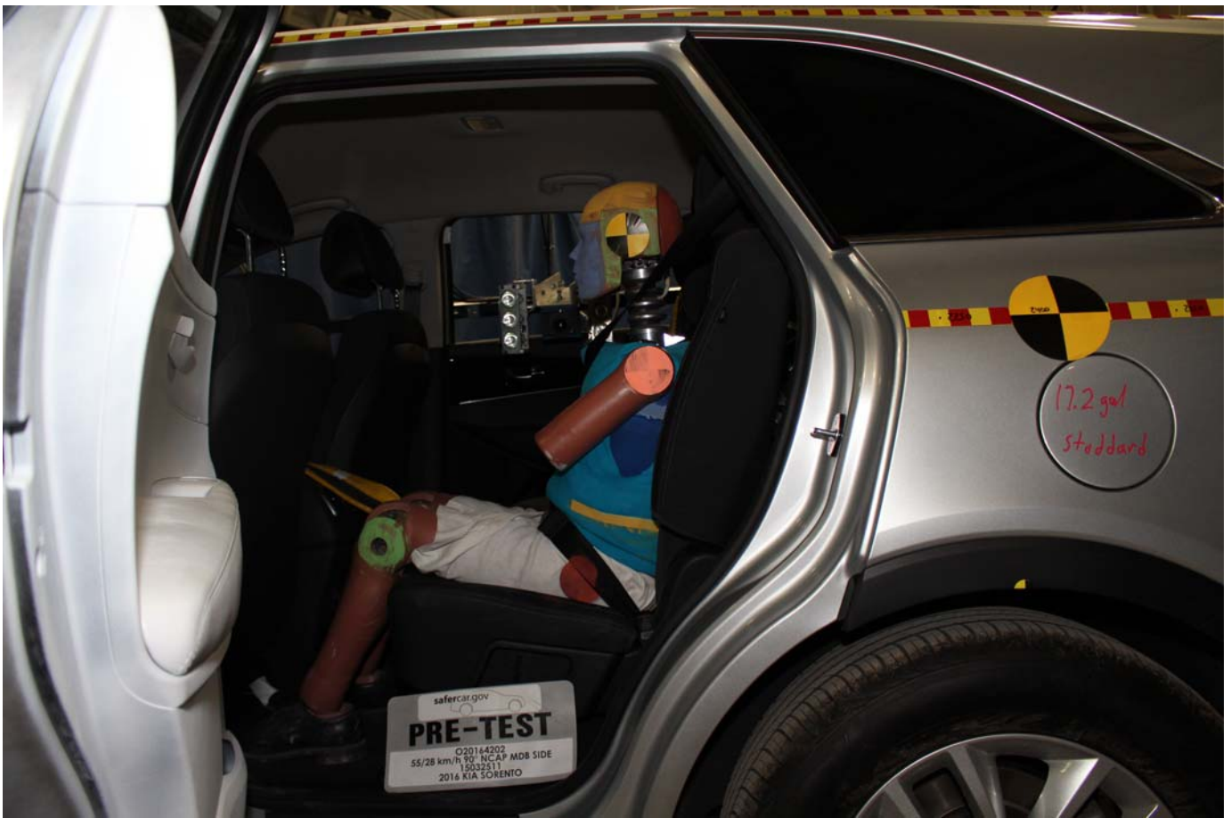
No. 055 - Pre-Test Left Side View of Rear Passenger Dummy Showing Belt and Chalking
