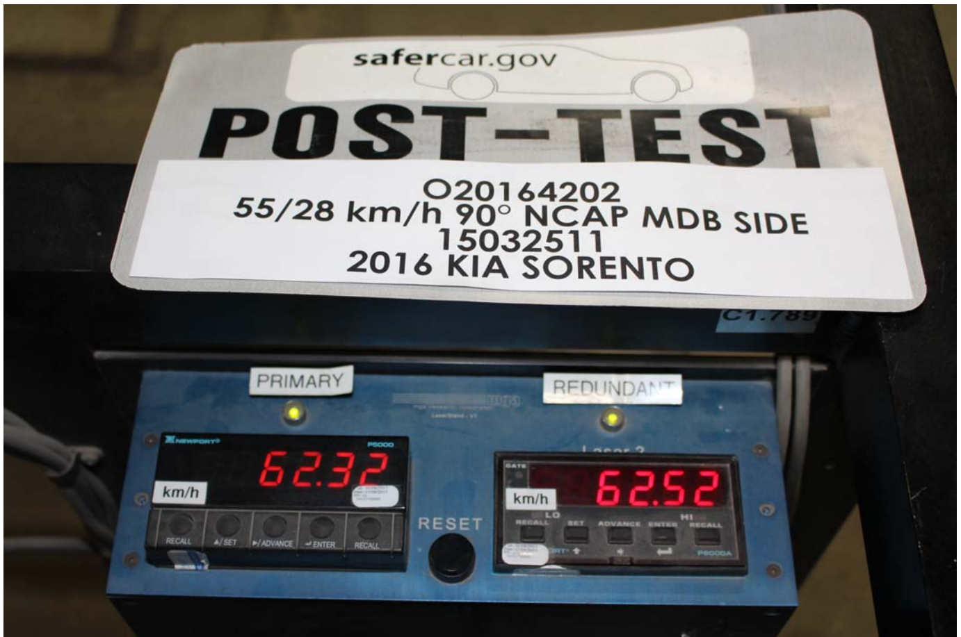
No. 095 - Post-Test Primary and Redundant Speed Trap Read-Out
