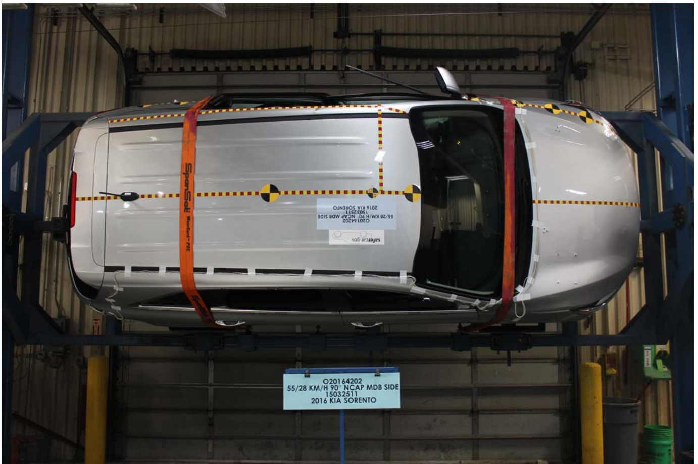
No. 099 - FMVSS No. 301 Static Rollover 270 Degrees
