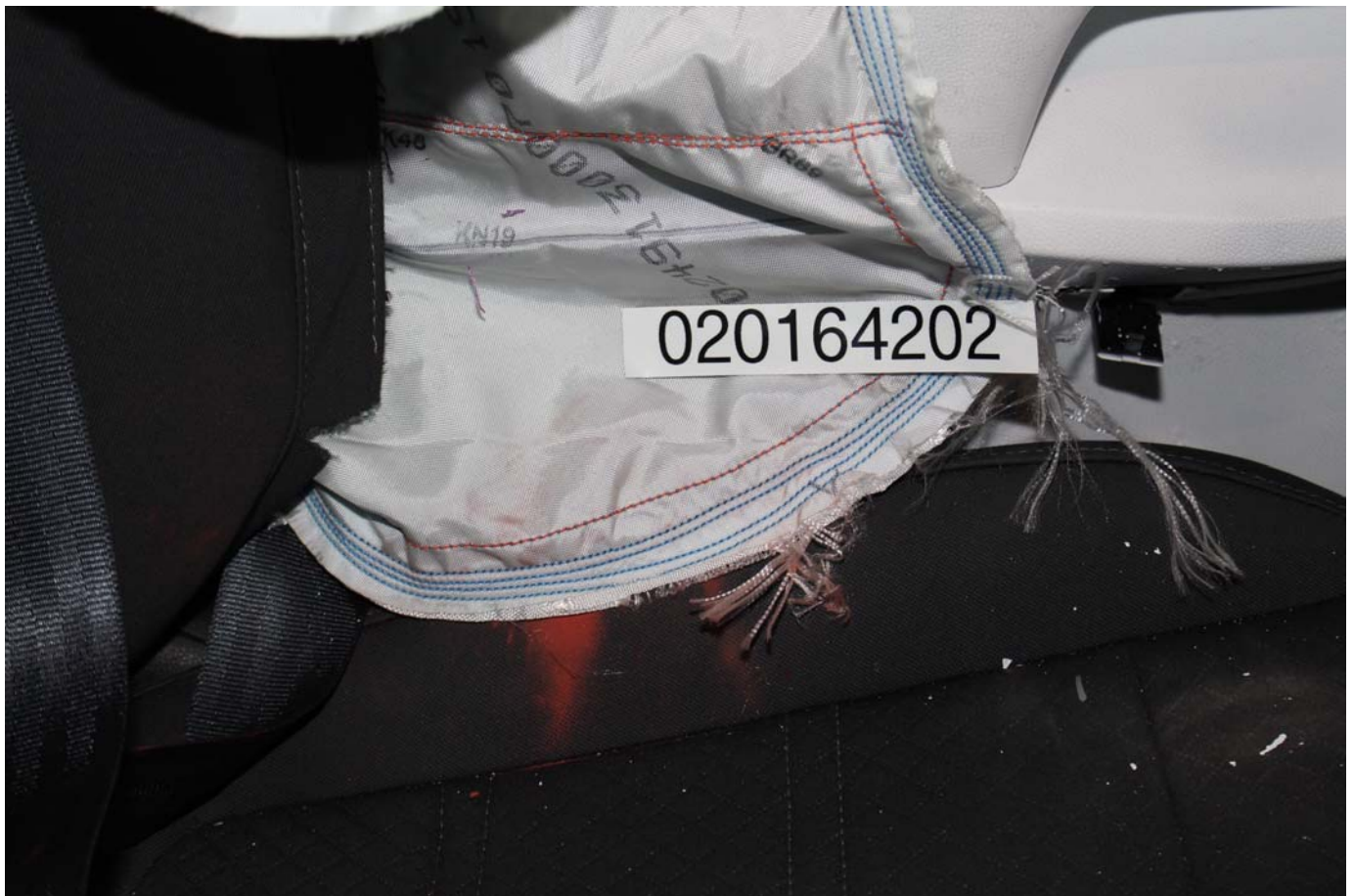
No. 053 - Post-Test Driver Dummy Close-up Pelvis Contact with Side Airbag View
