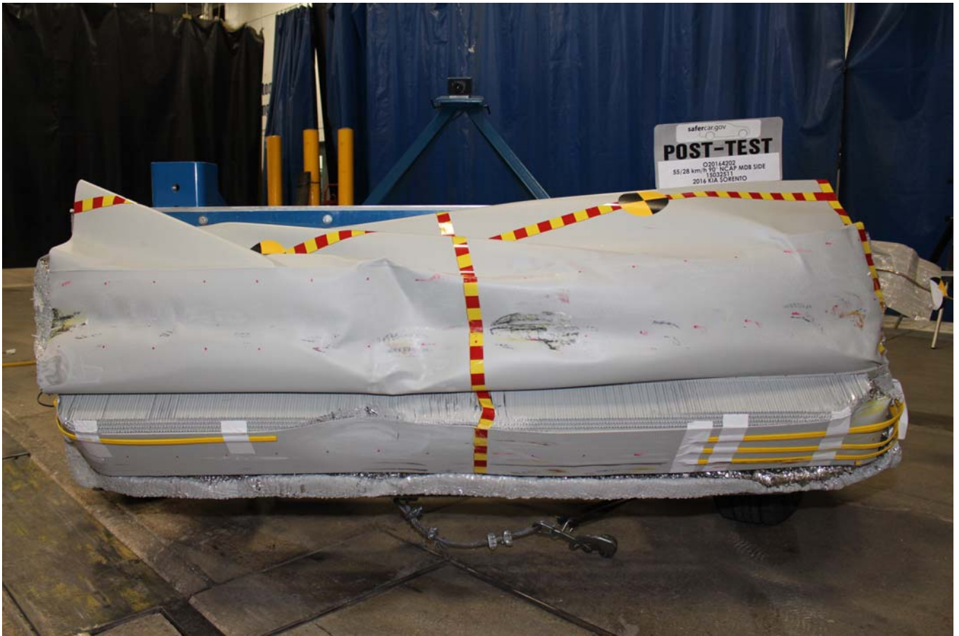
No. 085 - Post-Test Front View of MDB Impactor Face
