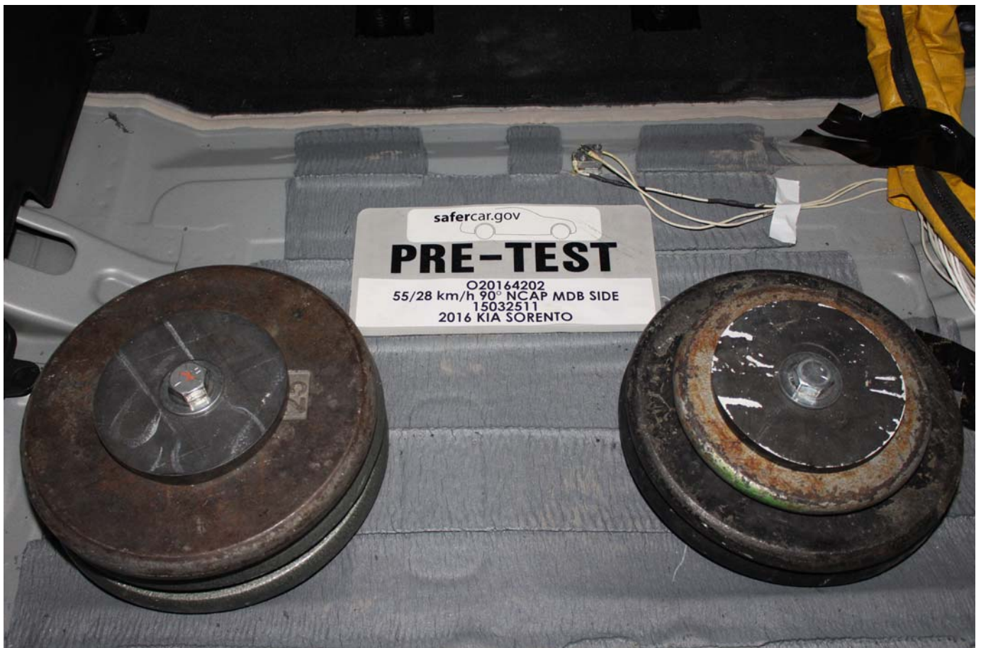
No. 094 - Pre-Test Ballast View
