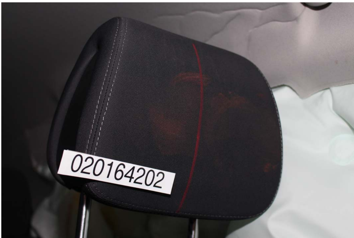
No. 048 - Post-Test Driver Dummy Close-up Head Contact with Vehicle Interior View
