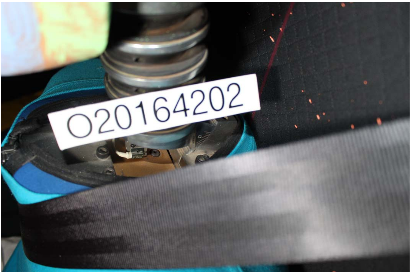
No. 062 - Pre-Test View of Rear Passenger Dummy's Neck Showing Position of Adjustable Neck Bracket
