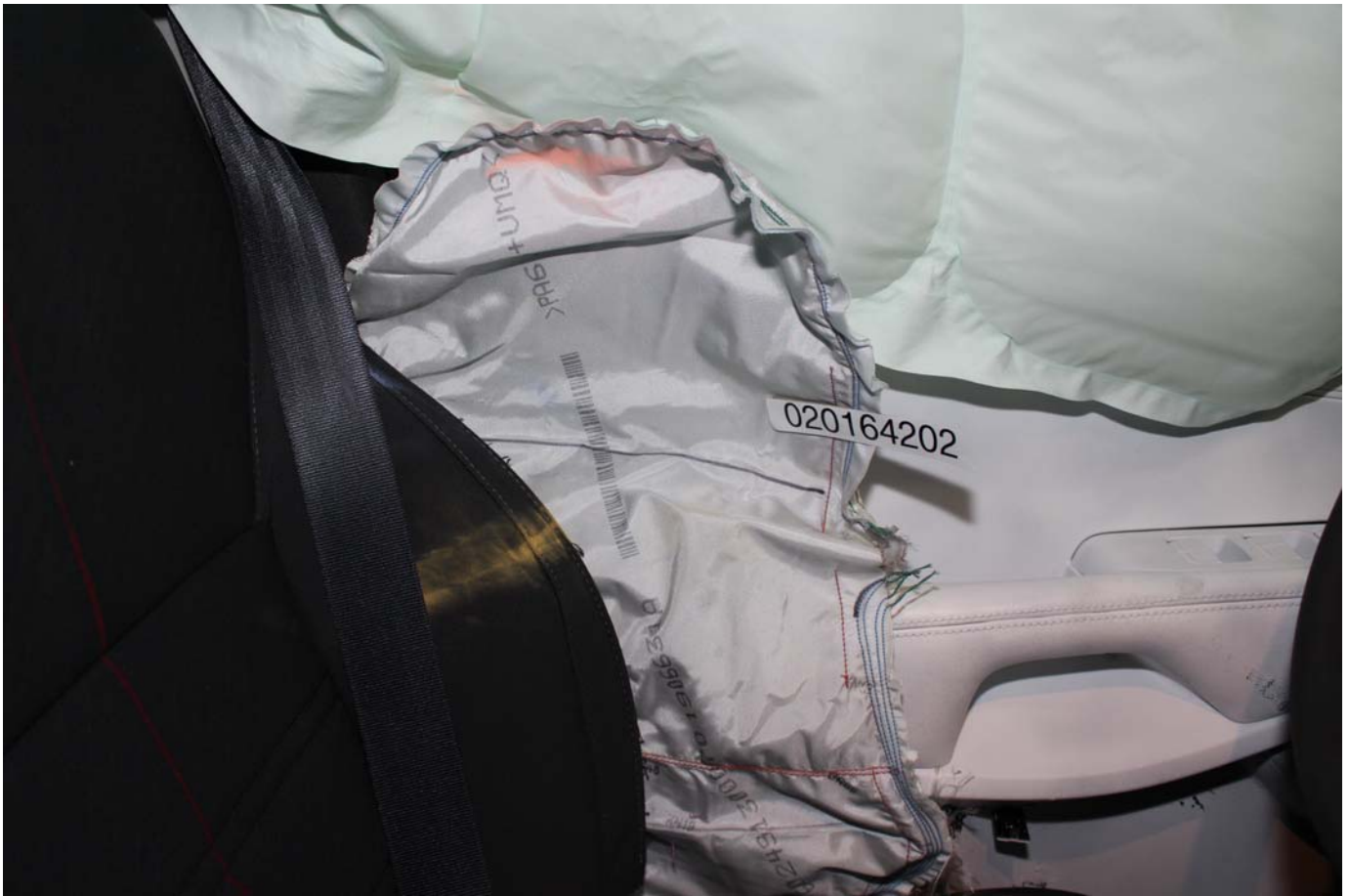
No. 051 - Post-Test Driver Dummy Close-up Torso Contact with Side Airbag View
