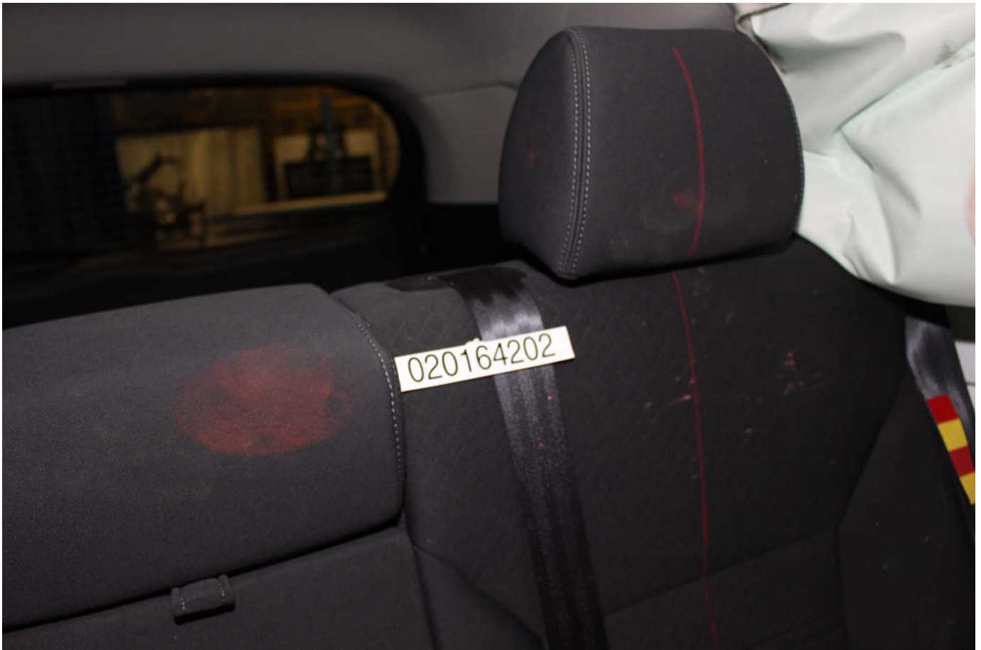
No. 075 - Post-Test Rear Passenger Dummy Close-up Head Contact with Vehicle Interior View
