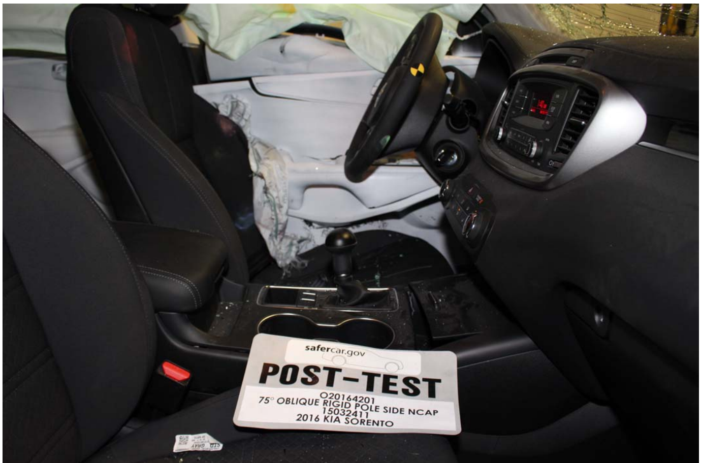
No. 072 - Post-Test View of Shattered Vehicle Inner Door Panel
