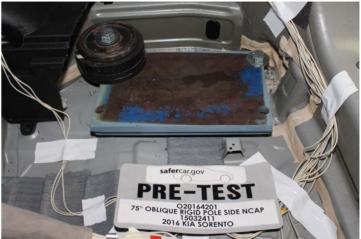
No. 061 - Pre-Test Ballast View
