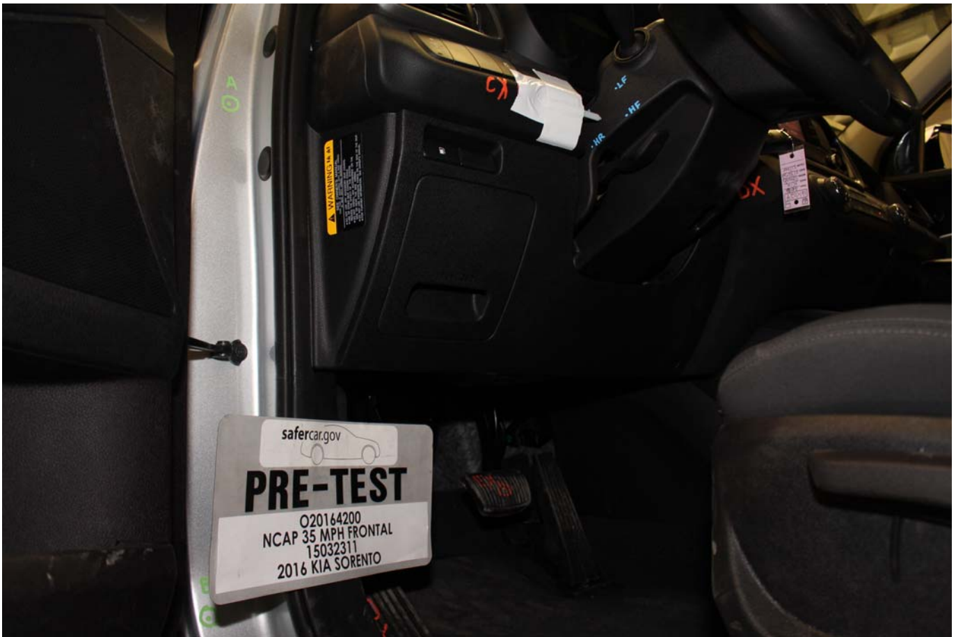
Photo No. 041. - Pre-Test Driver's Side Knee Bolster (without dummy)
