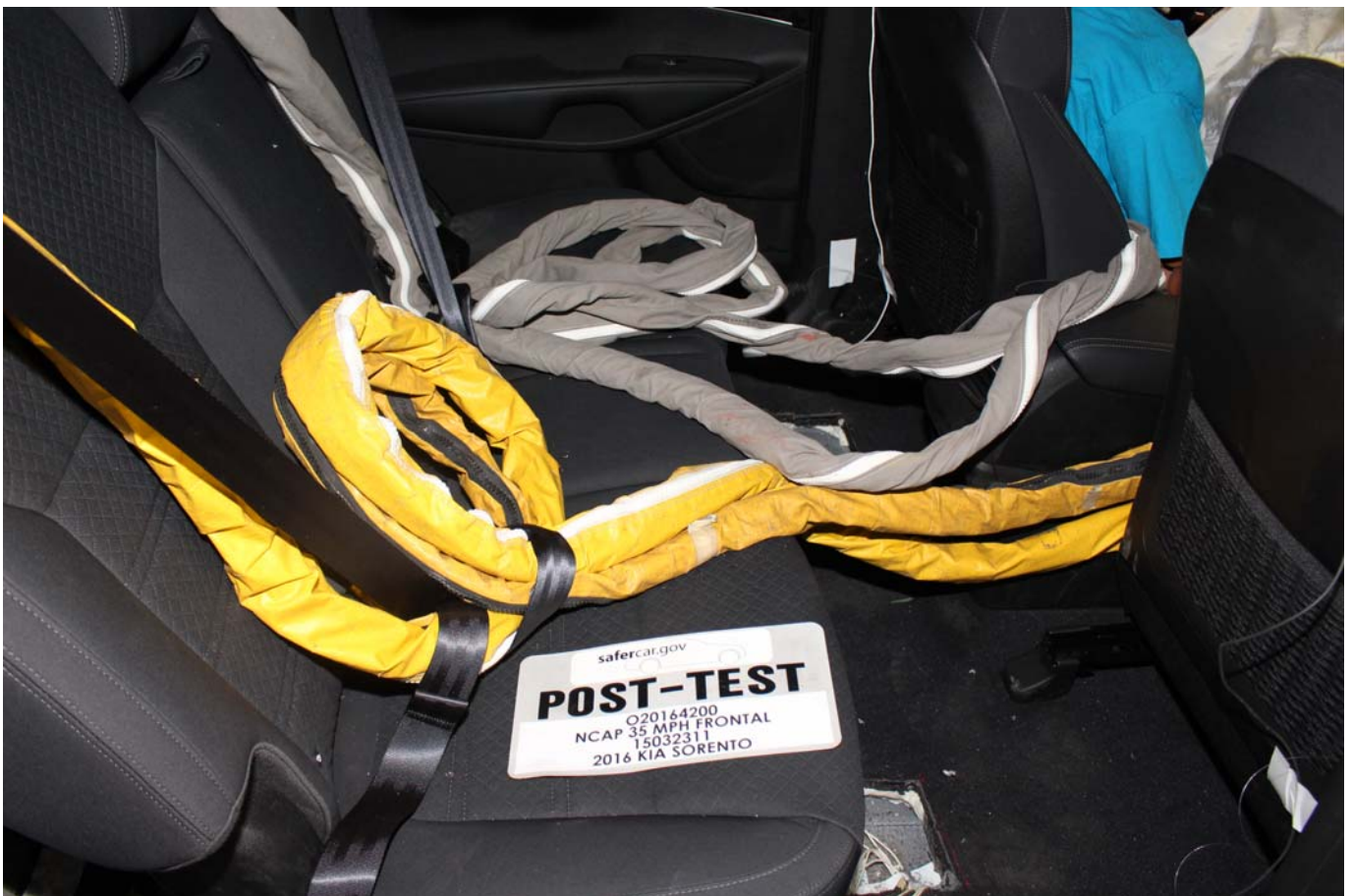
Photo No. 028. - Post-Test Dummy Cable Routing
