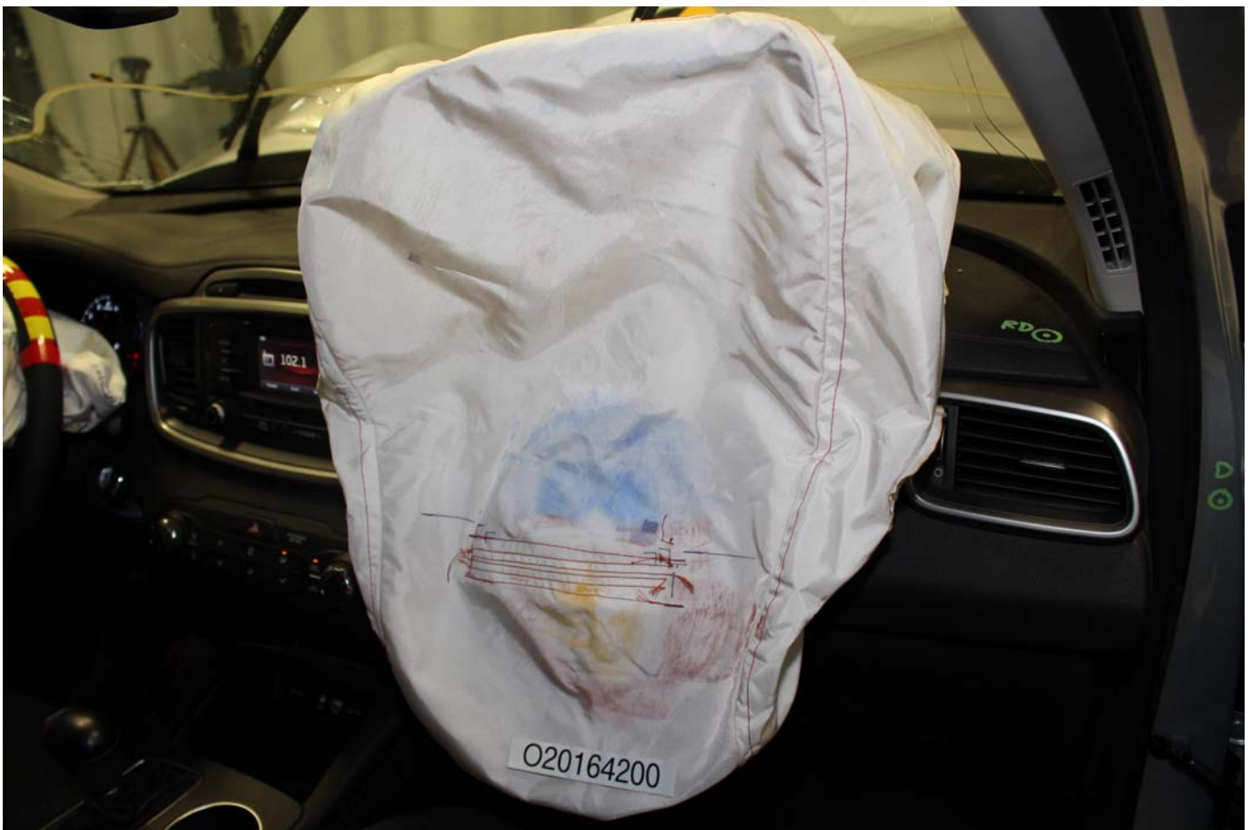
Photo No. 067. - Post-Test Passenger Dummy Contact with Airbag
