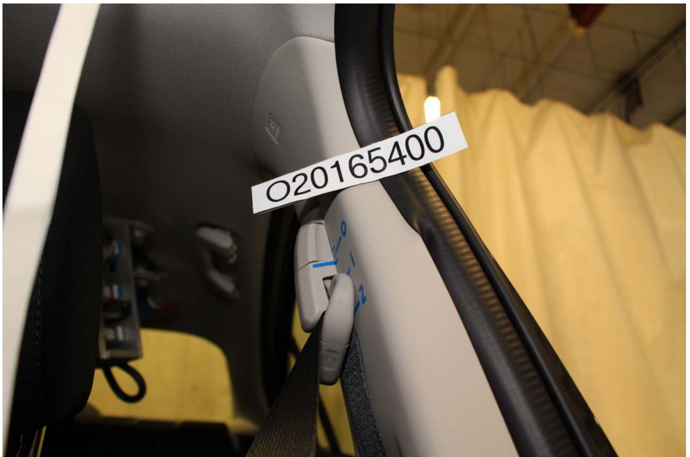
No. 042 Post-Test View of Belt Anchorage for Driver Dummy
