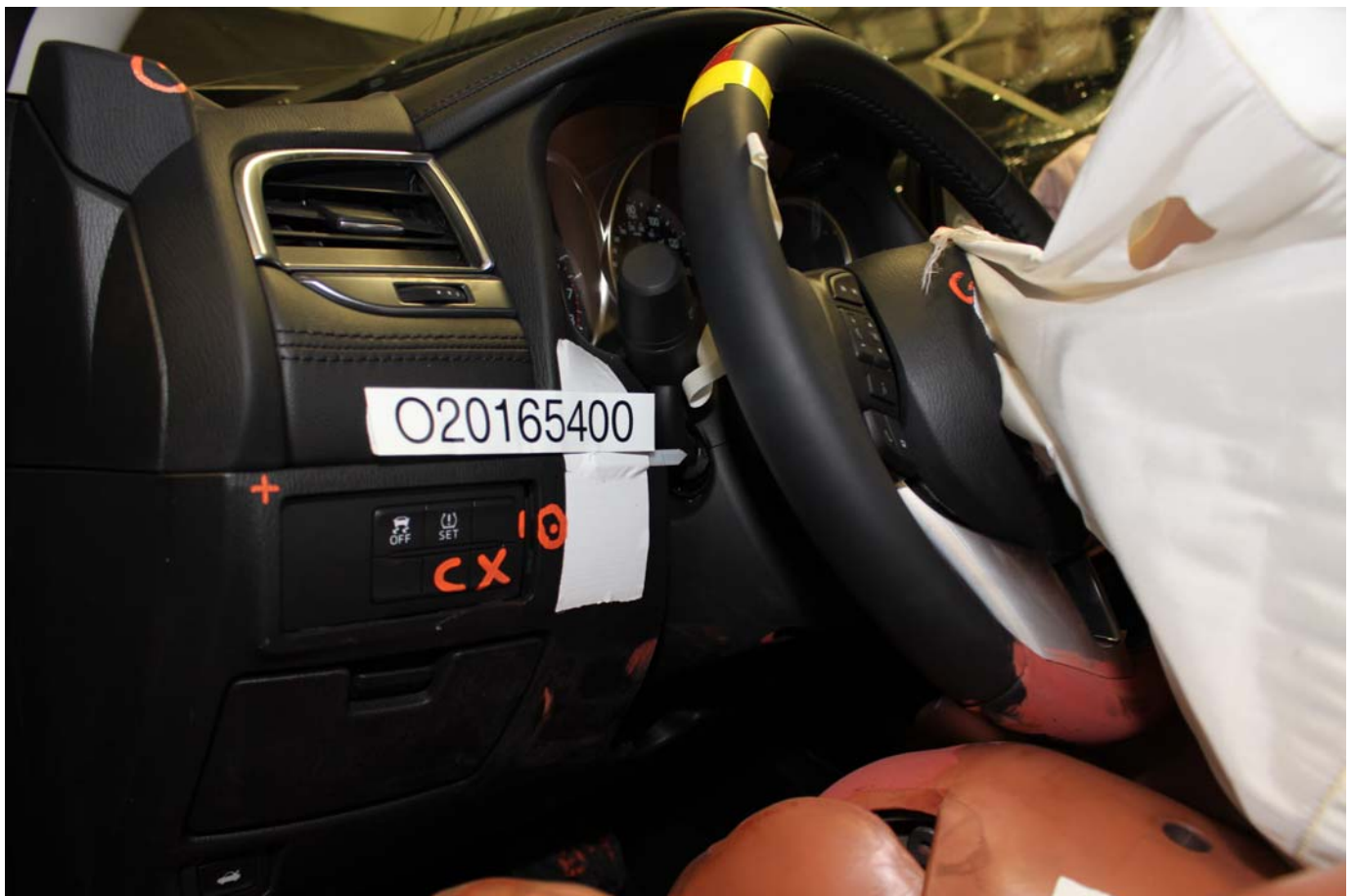
No. 054 Post-Test View of the Steering Wheel
