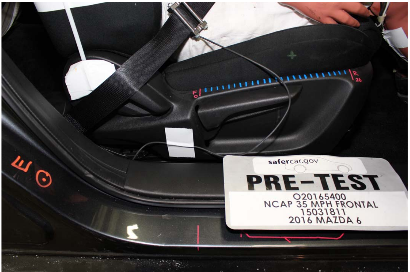
No. 061 Pre-Test Passenger's Seat Fore-Aft Markings
