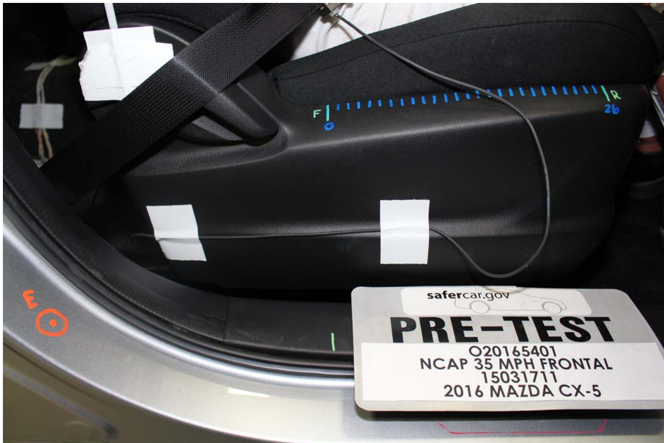
No. 061 Pre-Test Passenger's Seat Fore-Aft Markings
