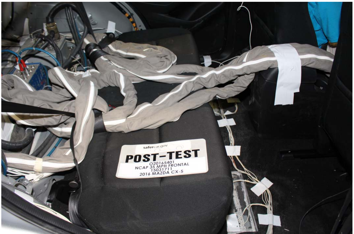
No. 032 Post-Test Dummy Cable Routing
