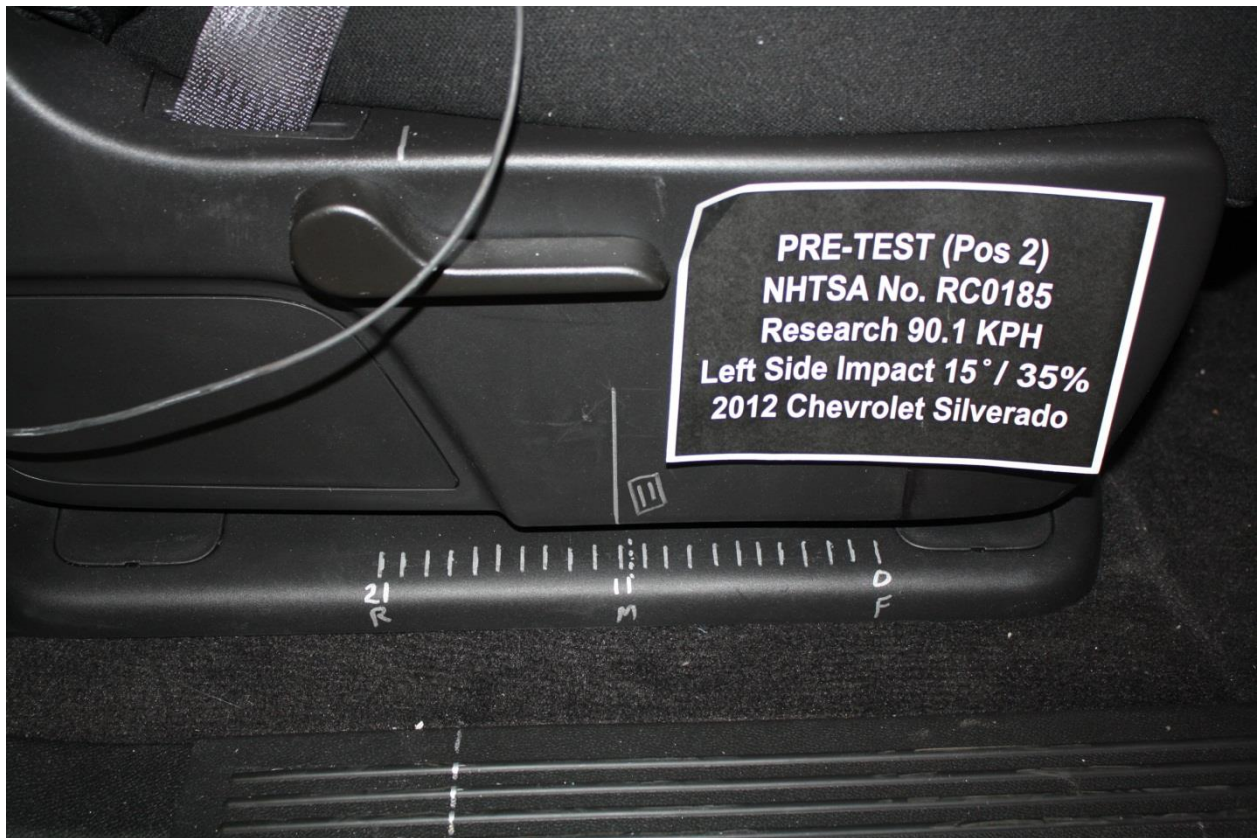
No. 106 Pre-Test Passenger Seat Fore-Aft Markings
