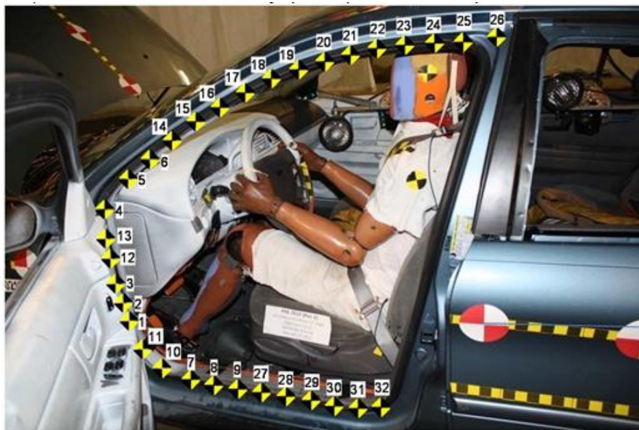
Figure 25: Driver Door Measurements
