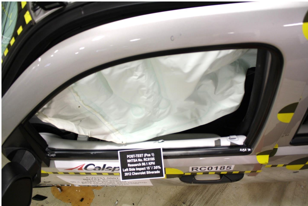
No. 061 Post-Test View of Driver Door Clearance
