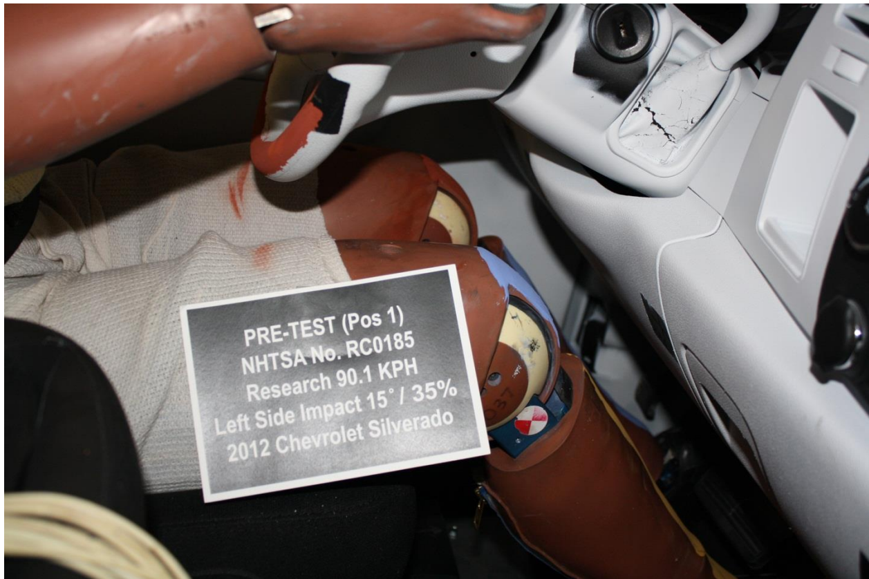
No. 071 Pre-Test View of Driver Right Knee and Bolster
