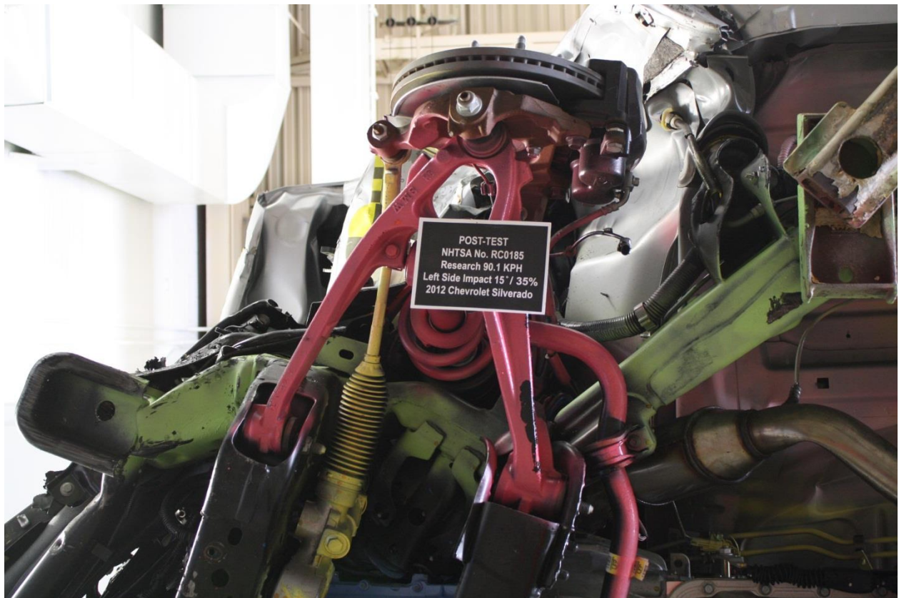
No. 141 Post-Test Frame Rail with tire removed
