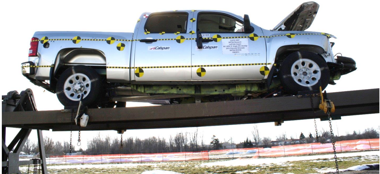
No. 184 Vehicle at 360 Degrees on Static Rollover Device
