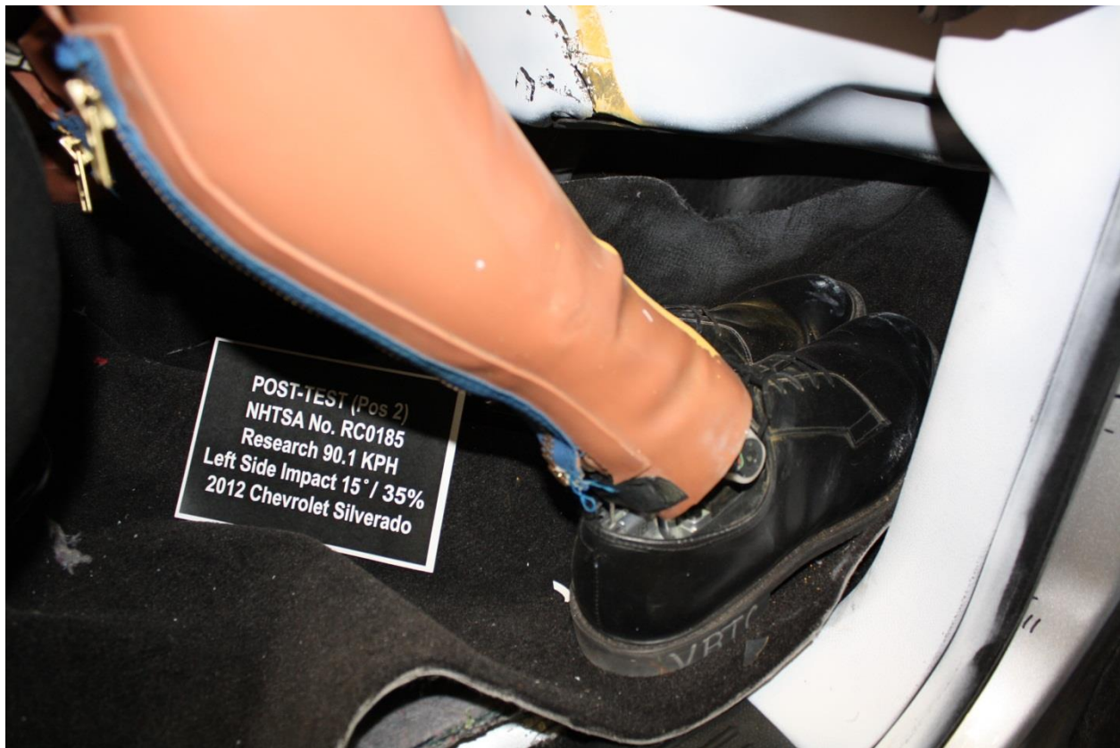
No. 113 Post-Test View of Passenger Feet
