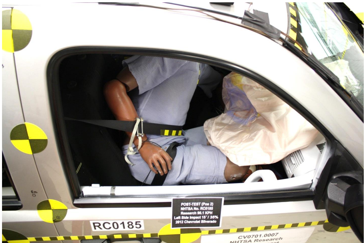
No. 105 Post-Test View of Passenger Door Clearance
