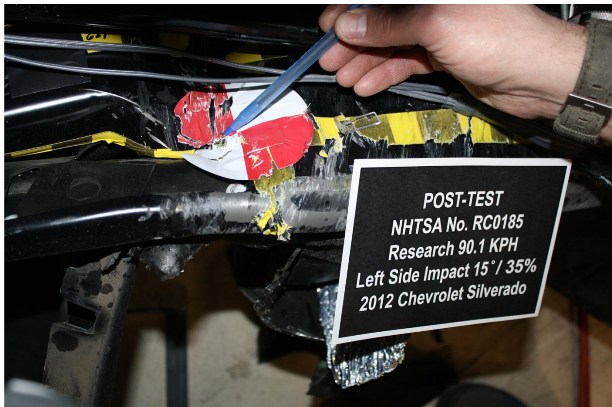
No. 026 Post-Test Close-up View of Impact Point
