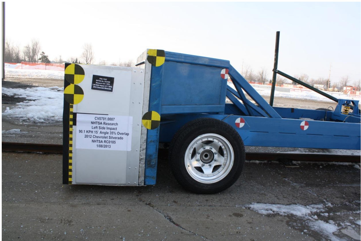
No. 162 Pre-Test Left Side View of RMDB
