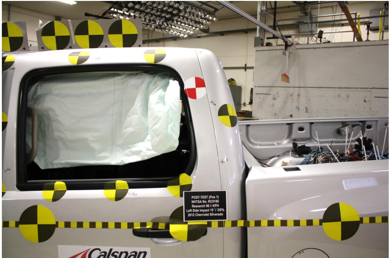
No. 158 Post-Test View of Deformation of C pillar-Struck Side
