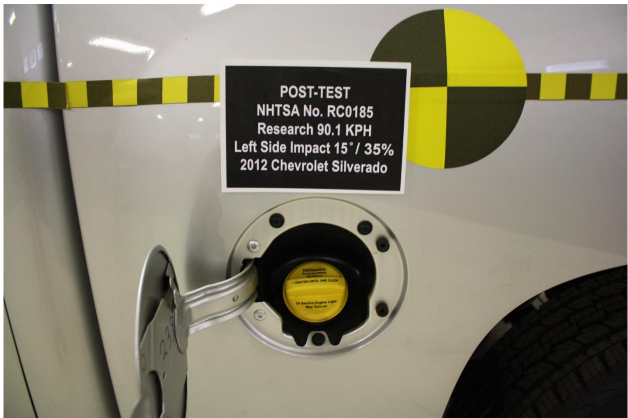
No. 126 Post-Test View of Fuel Filler Cap
