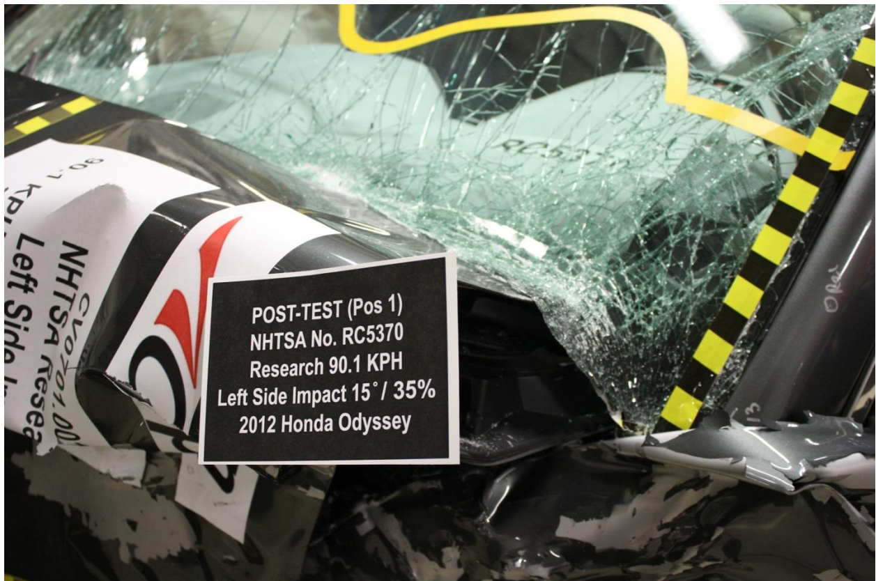
No. 161 Post-Test View of Windshield Separation
