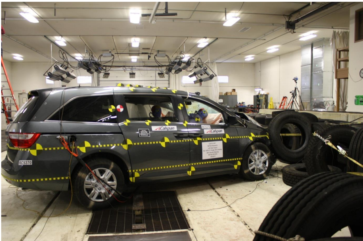
No. 179 Post-Test RMDB & Vehicle, Front View
