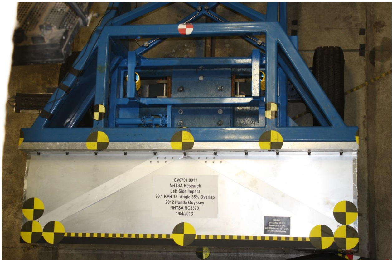
No. 166 Pre-Test Top View of RMDB
