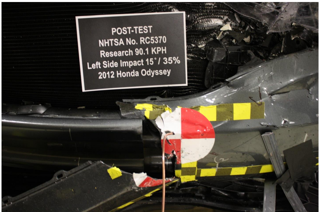
No. 026 Post-Test Close-up View of Impact Point
