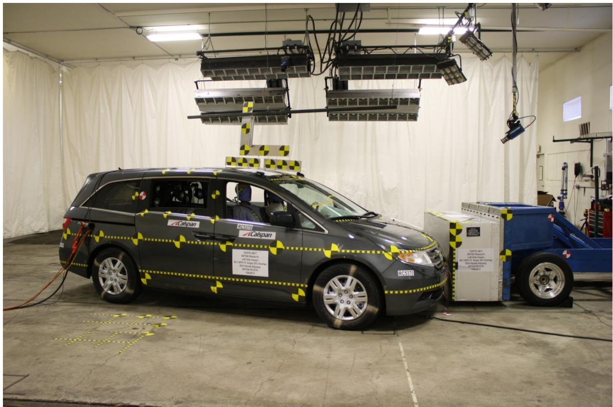
No. 172 Pre-Test RMDB & Vehicle, Left Side
