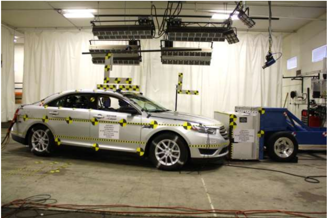
No. 023 Pre-Test Left Side View of RMDB against target vehicle at ideal Impact Point
