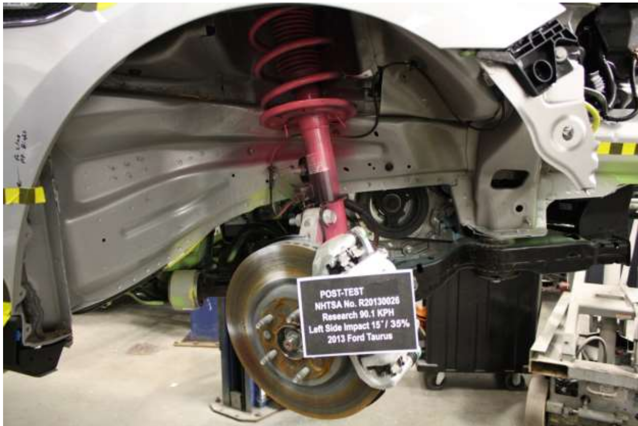
No. 150 Post-Test Side View of Front Passenger Wheel Well w/ Tire Removed
