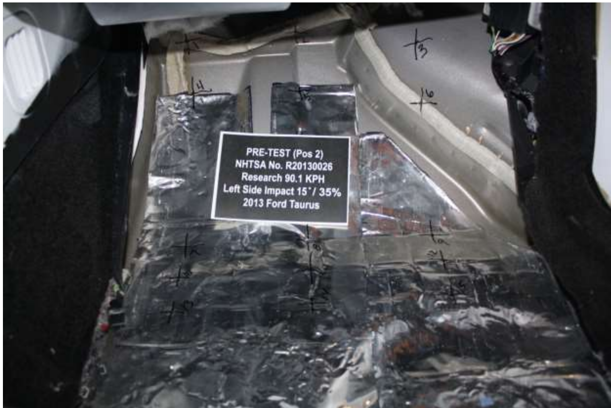
No. 094 Pre-Test View of Passenger Floor pan at Mid seat level, without carpet
