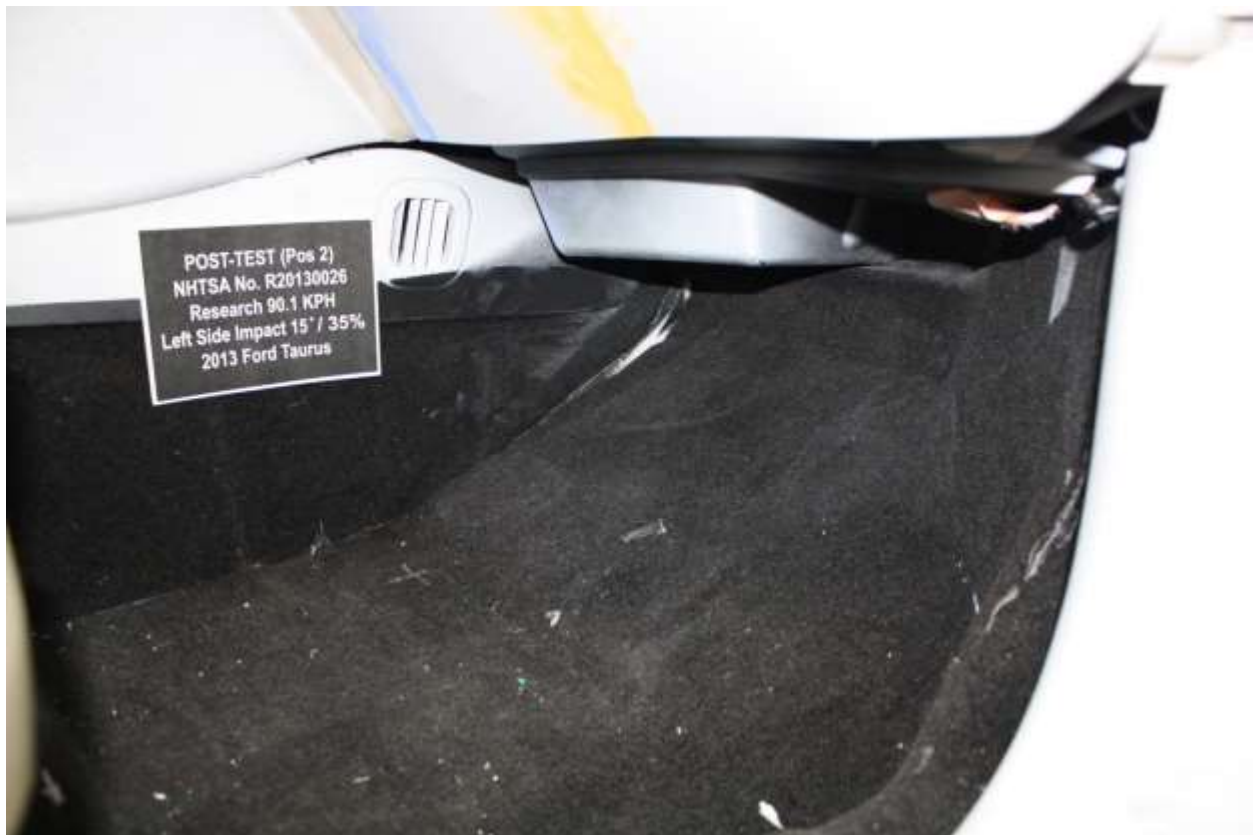
No. 089 Post-Test View of Passenger Floor pan at Left sill level, w/carpet
