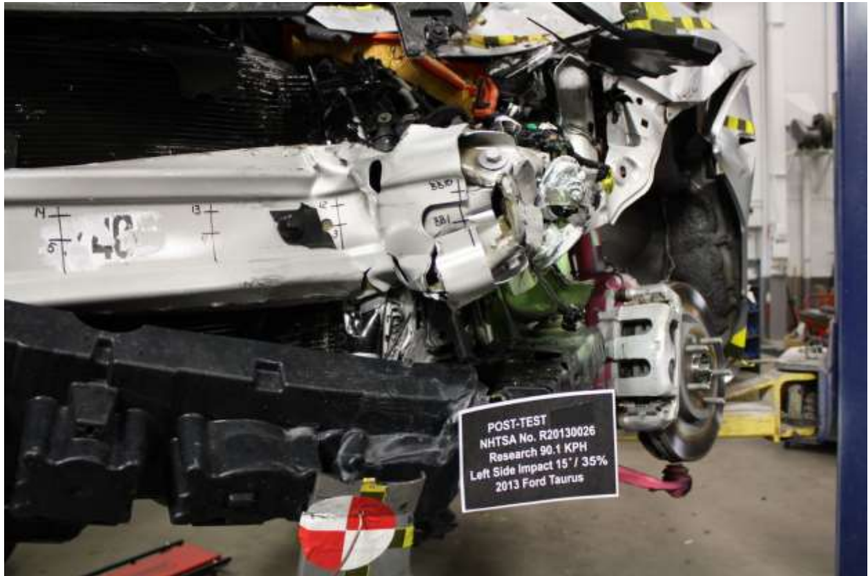
No. 144 Post-Test Side View of Front Driver Wheel Well w/ Tire Removed
