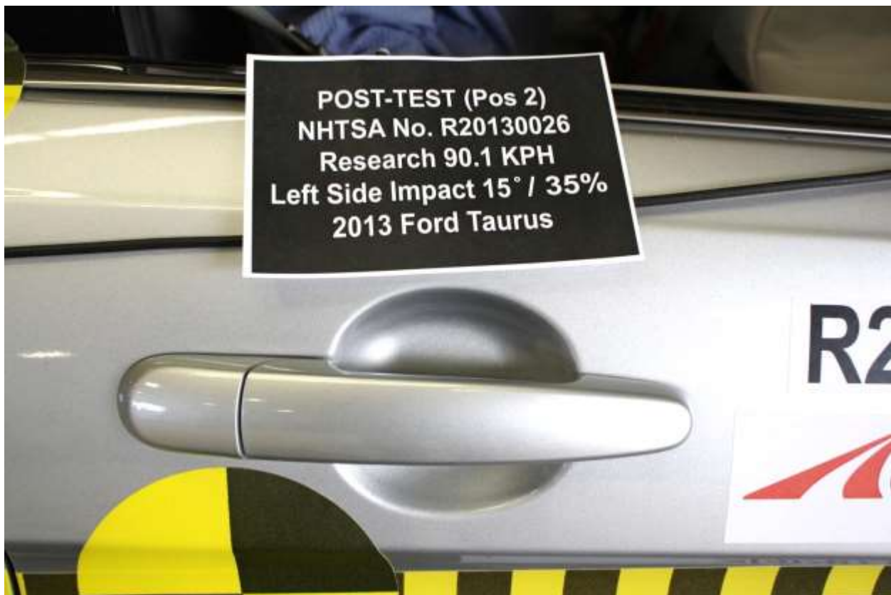
No. 031 Post-Test Close-up View of Passenger Door Latch
