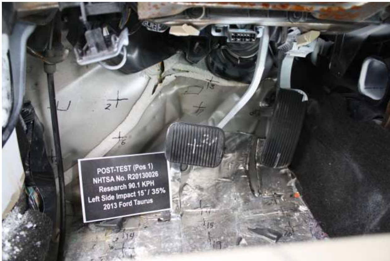
No. 051 Post-Test view of Driver Floor pan at Mid seat level, w/o carpet
