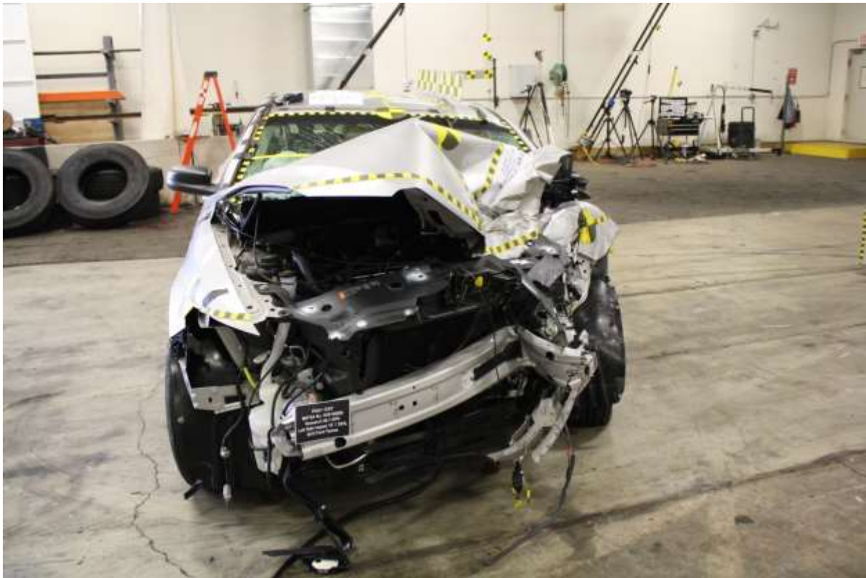
No. 006 Post-Test Front View of Test Vehicle
