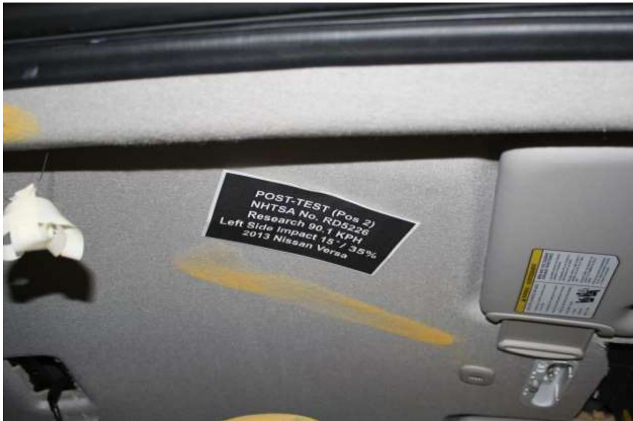
No. 121b Post-Test View of Passenger Head contact with Interior
