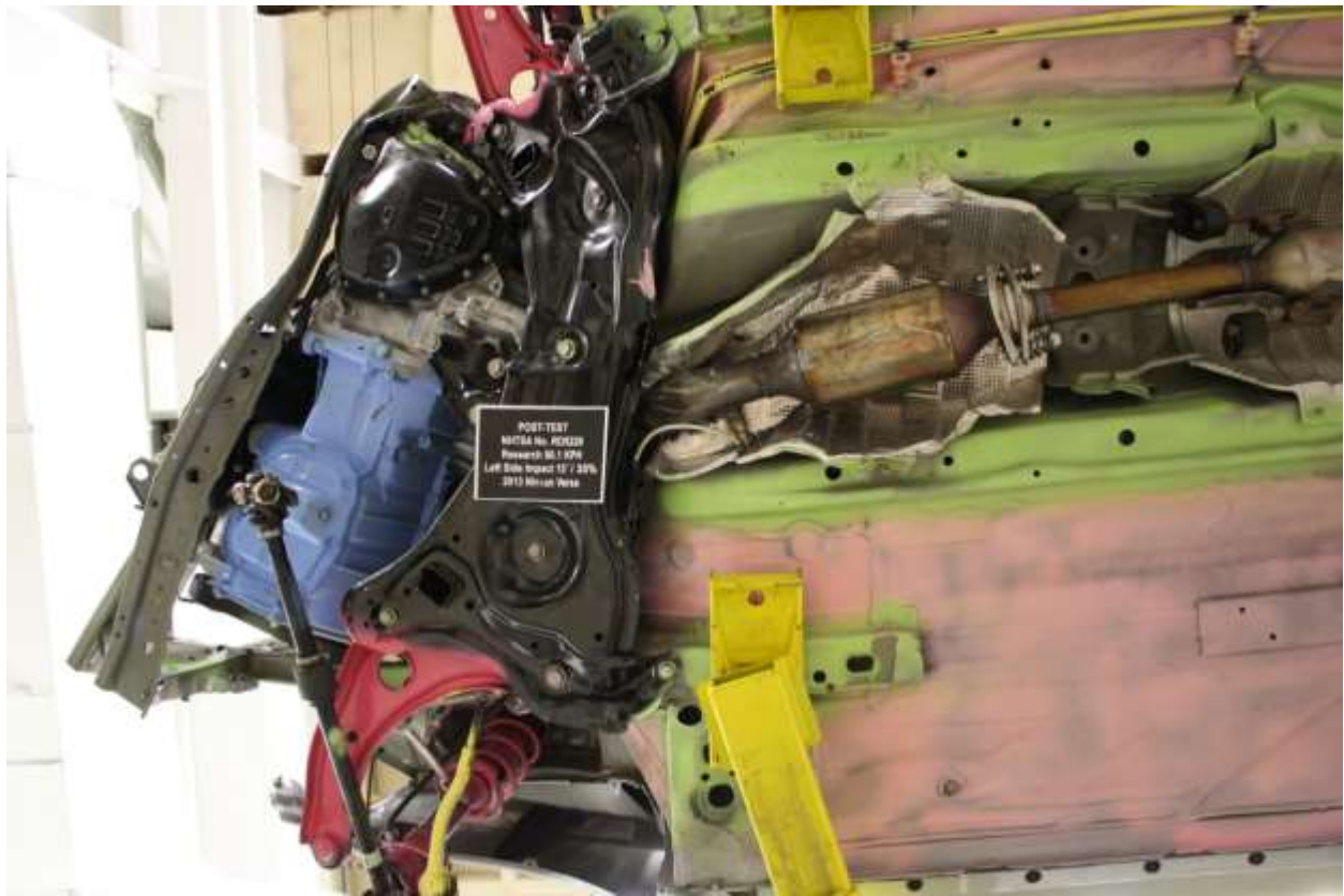
No. 139 Post-Test View of Front Sub-Frame Deformation
