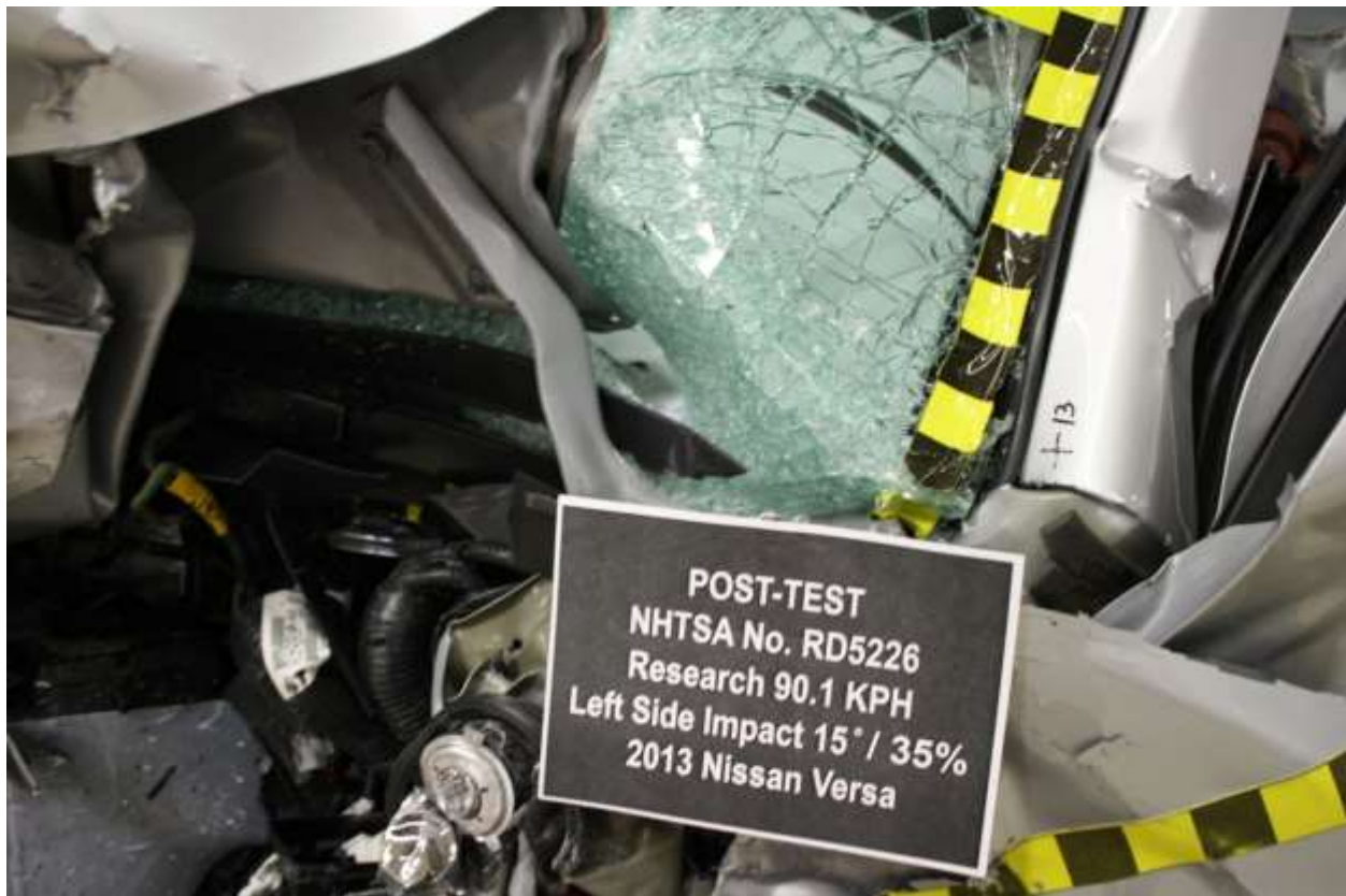
No. 161 Post-Test View of Windshield Separation
