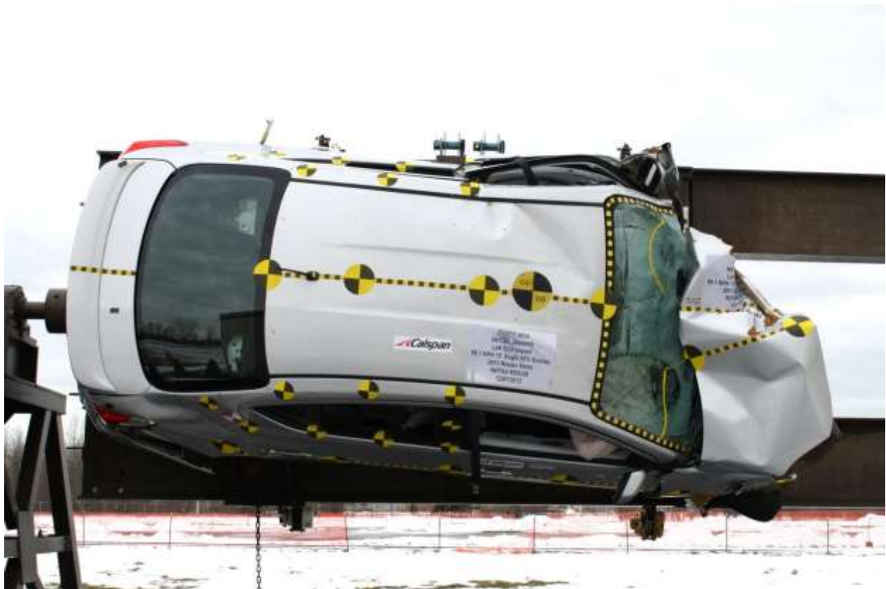
No. 183 Vehicle at 270 Degrees on Static Rollover Device
