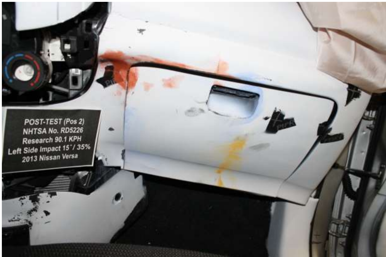
No. 122 Post-Test Passenger Contact With Glovebox
