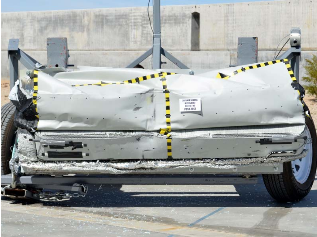
FIGURE 85. Post-Test Front View of MDB Impactor Face
