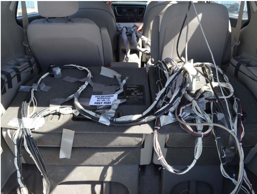
FIGURE 28. Post-Test Dummy Cable Routing
