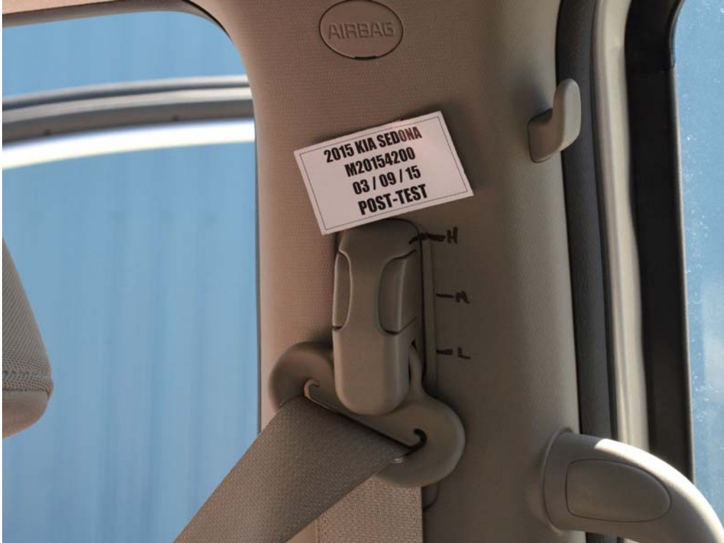
FIGURE 59. Post-Test View of Belt Anchorage for Passenger Dummy
