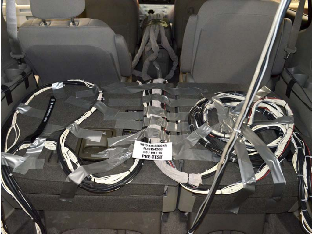
FIGURE 27. Pre-Test Dummy Cable Routing
