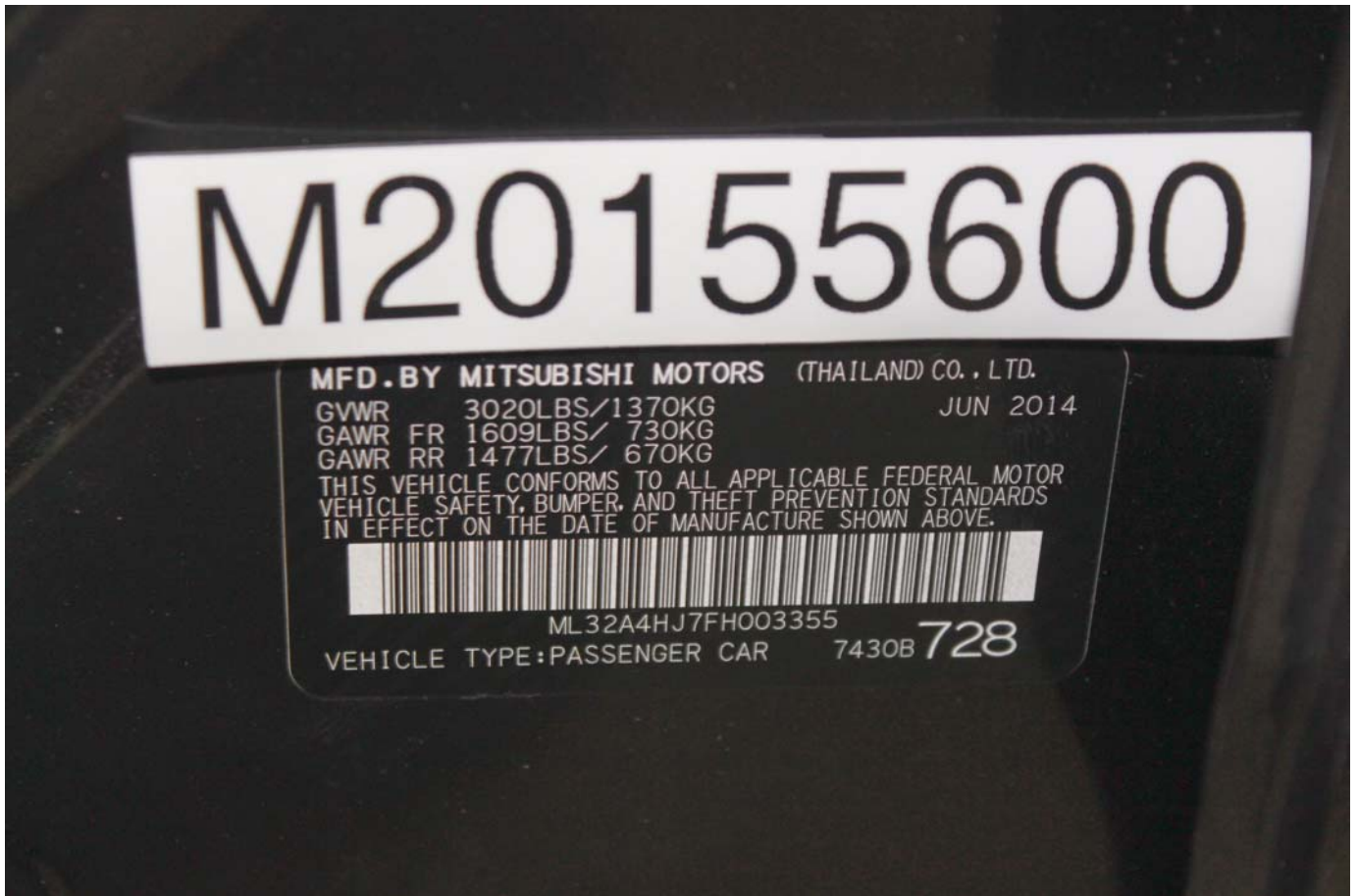
Photo No. 2 - Vehicle Certification Placard
