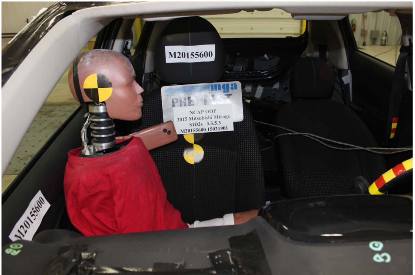
Photo No. 13 - Pre-Test SID-II's Dummy Front View
