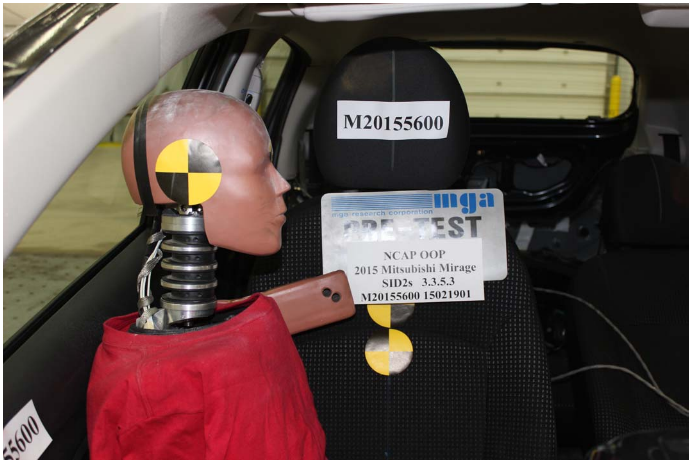
Photo No. 15 - Pre-Test SID-IIs Dummy Front Closeup View
