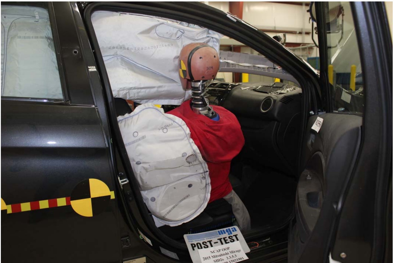
Photo No. 21 - Post-Test SID-IIs Dummy Right Side View (Door Open)
