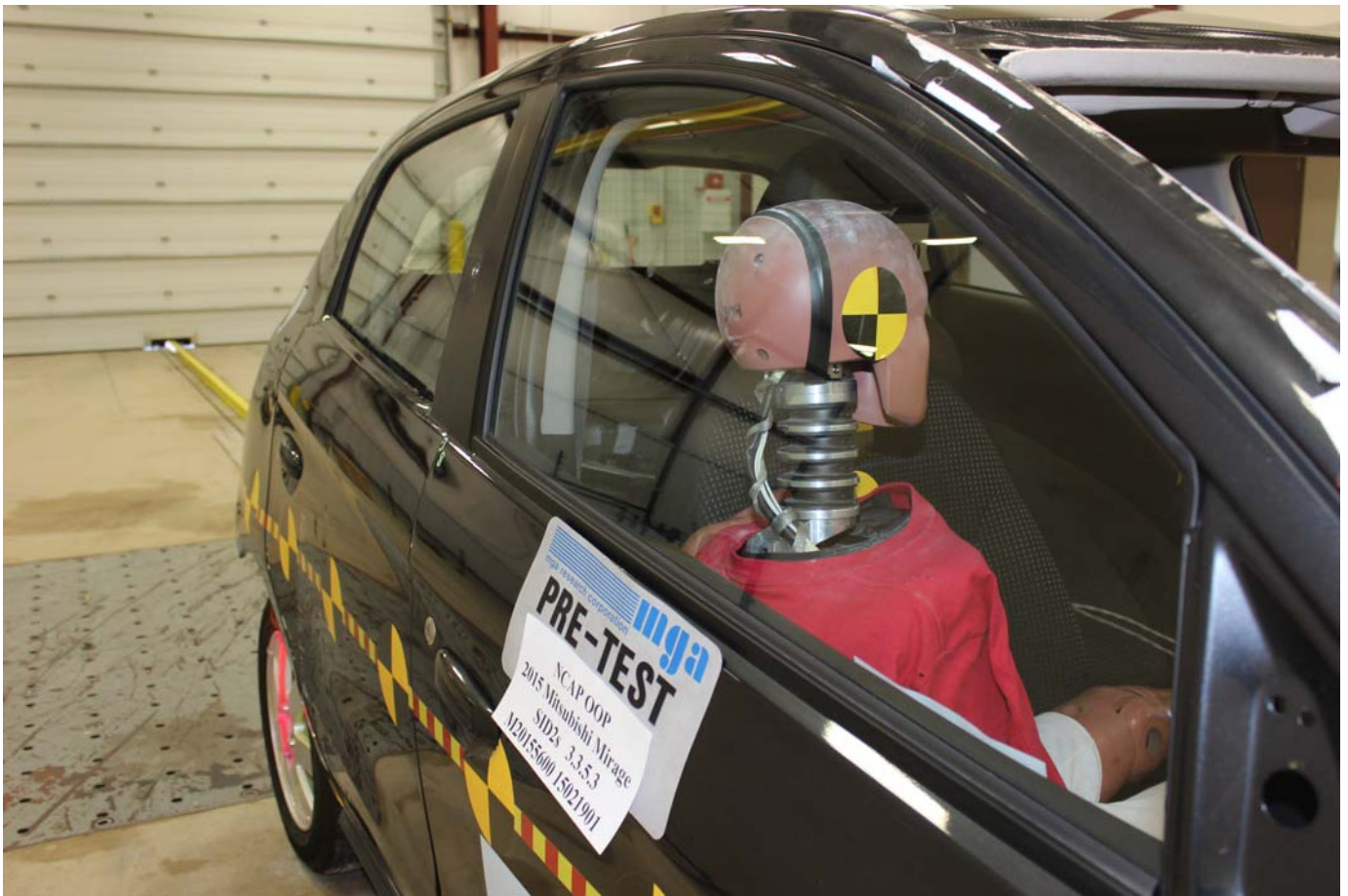
Photo No. 17 - Pre-Test SID-IIs Dummy Right ¾ Front View
