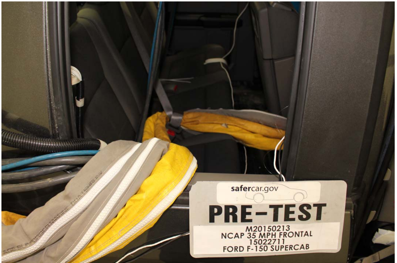
No. 031 Pre-Test Dummy Cable Routing
