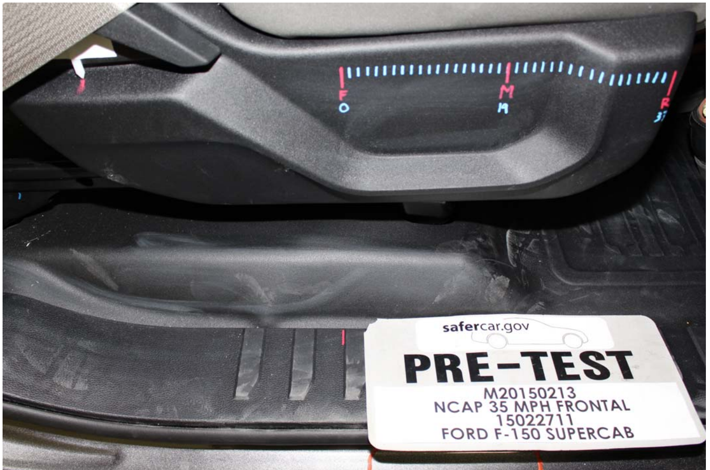
No. 061 Pre-Test Passenger's Seat Fore-Aft Markings
