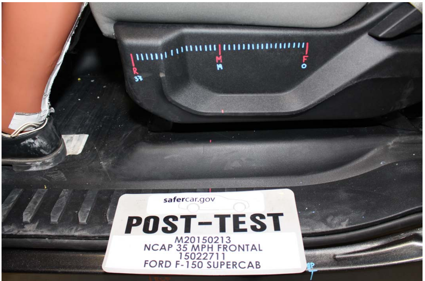
No. 040 Post-Test Driver's Seat Fore-Aft Markings
