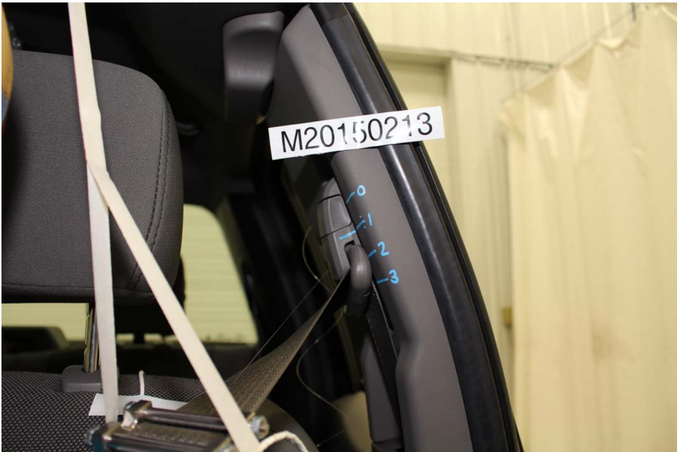
No. 041 Pre-Test View of Belt Anchorage for Driver Dummy
