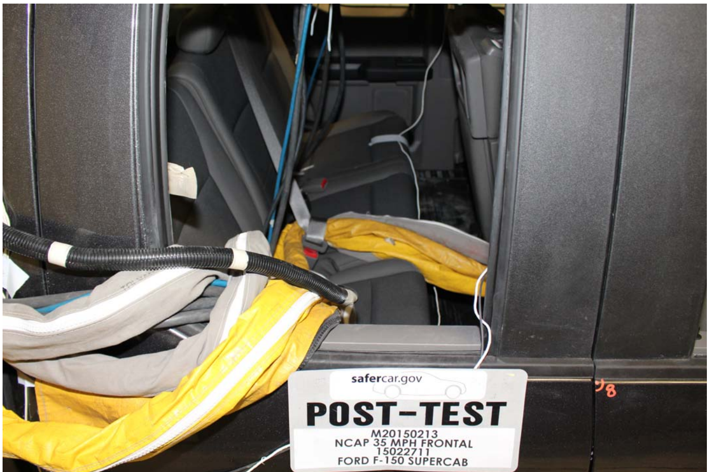
No. 032 Post-Test Dummy Cable Routing
