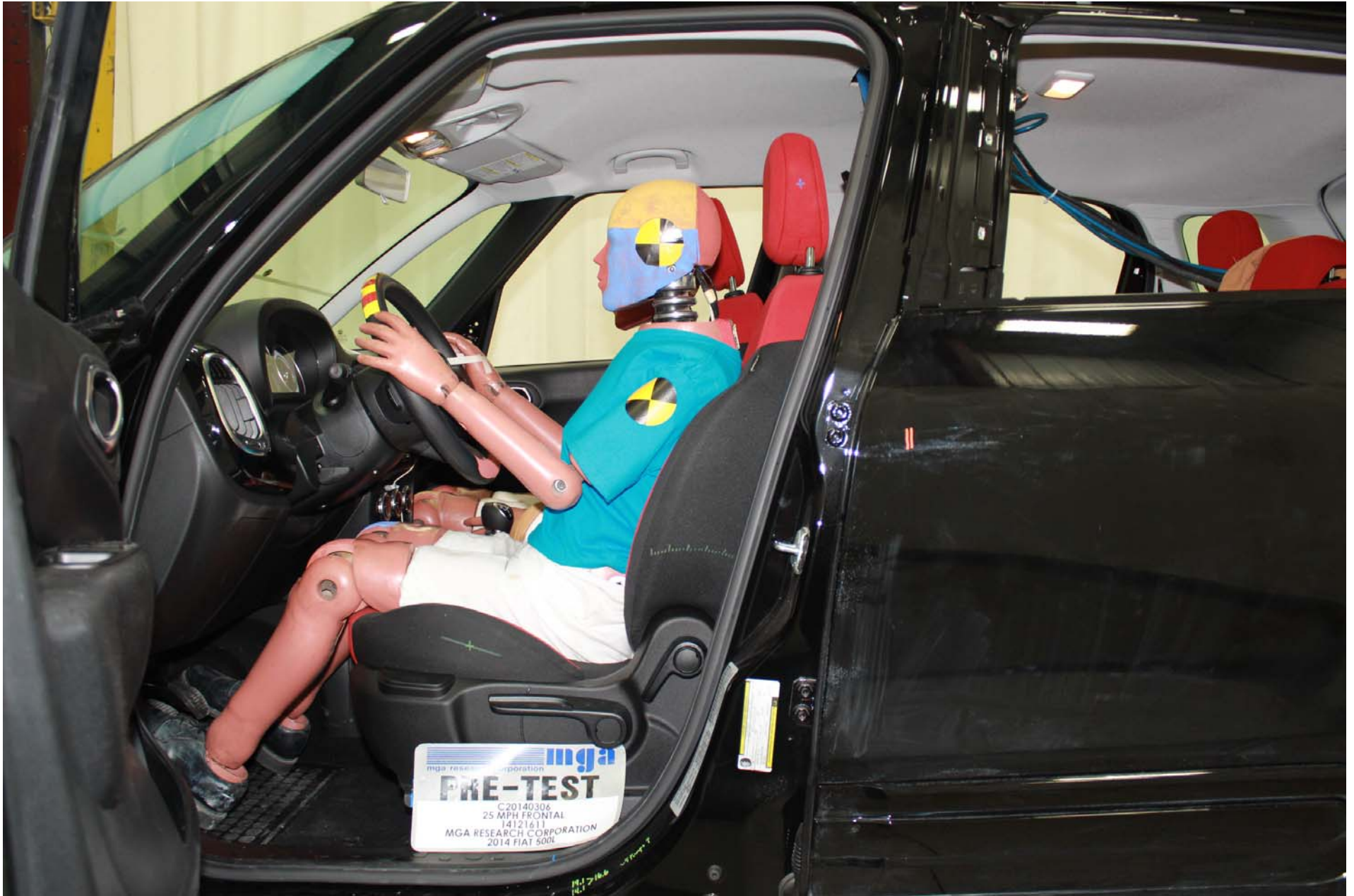
Photo No. 37 - Pre-Test Driver Dummy Position Left Side View (door open)
