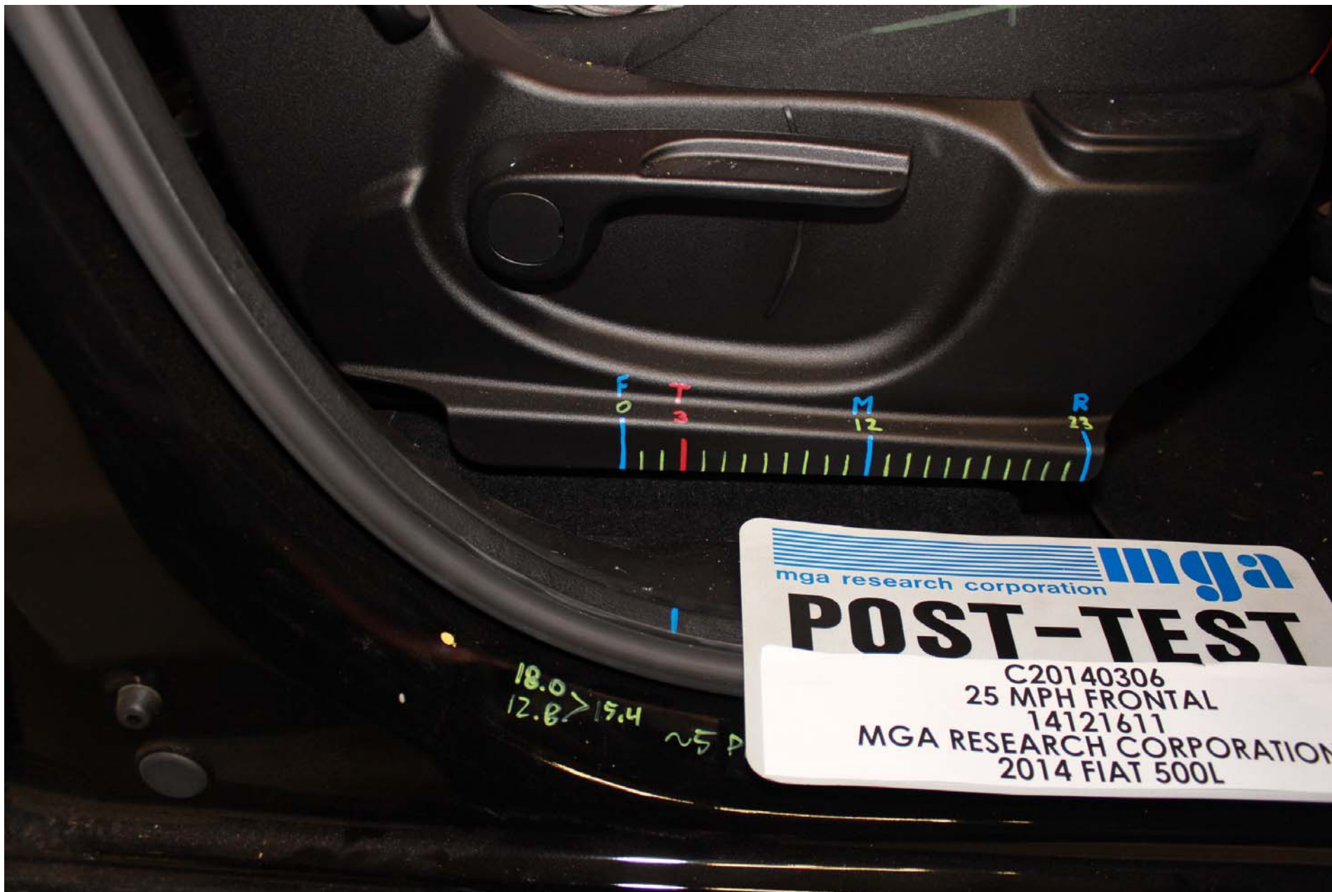
Photo No. 54 - Post-Test Passenger Dummy Seat Position
