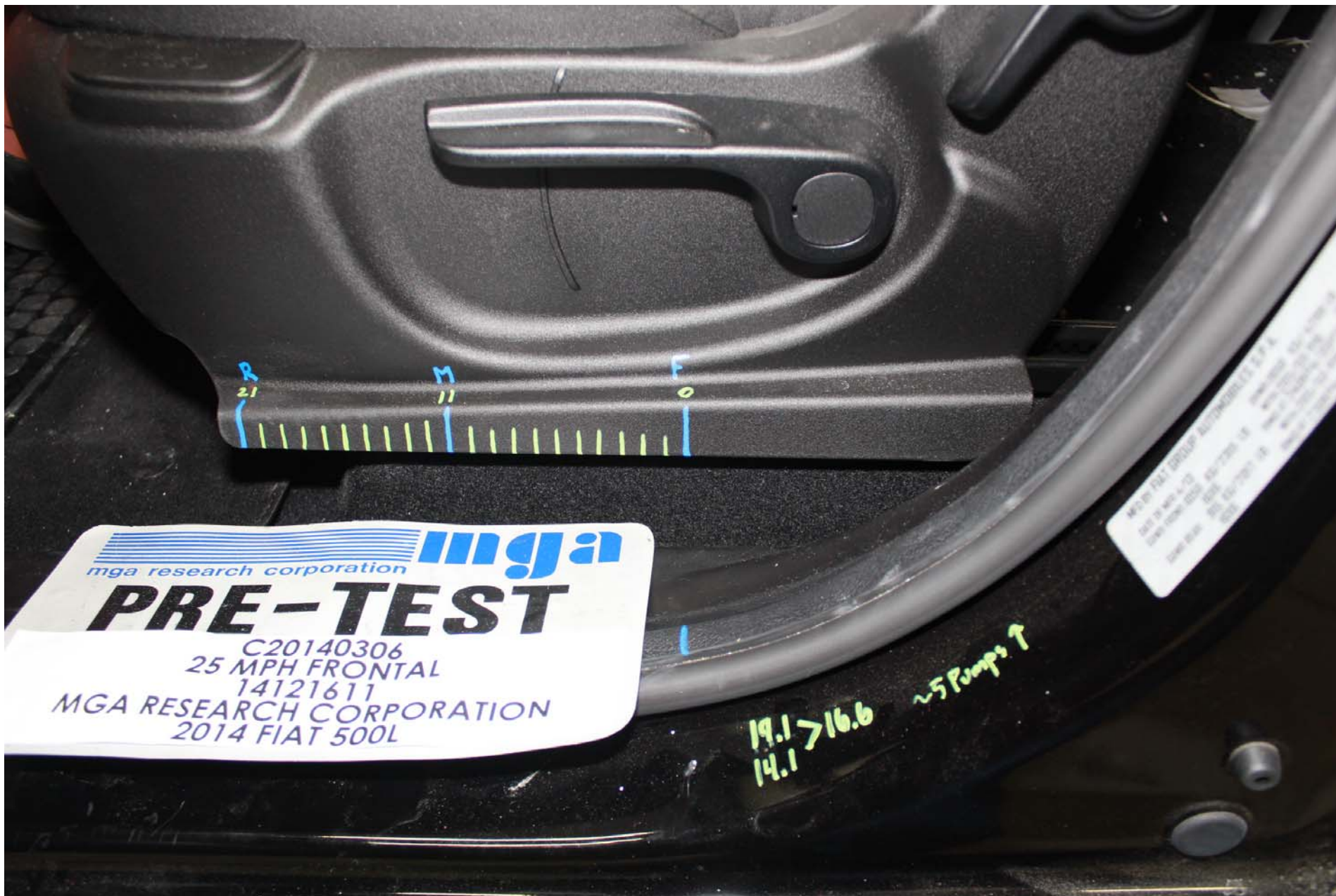
Photo No. 39 - Pre-Test Driver Dummy Seat Position
