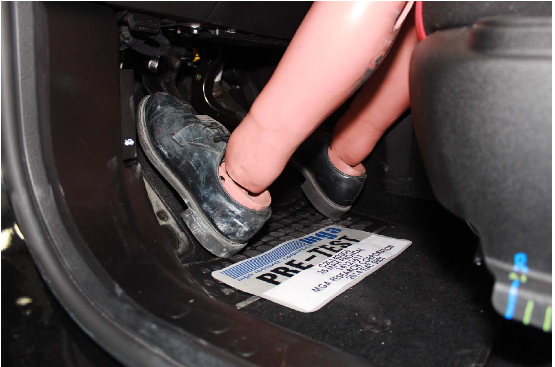
Photo No. 41 - Pre-Test Driver Dummy Feet Position
