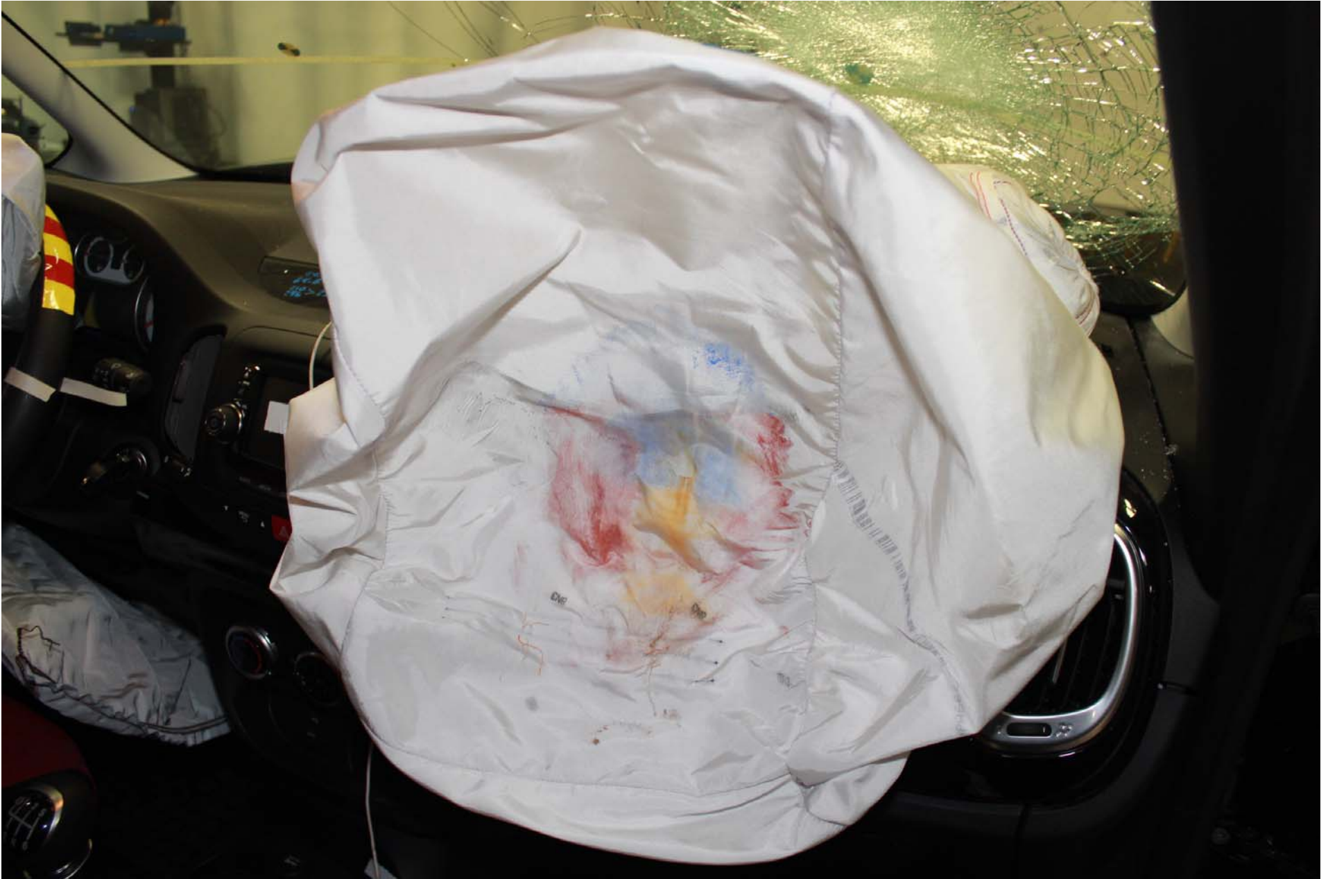
Photo No. 59 - Post-Test Passenger Dummy Airbag Contact
