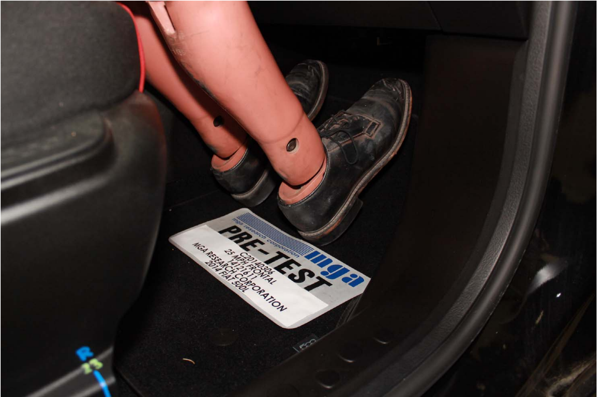
Photo No. 55 - Pre-Test Passenger Dummy Feet Position
