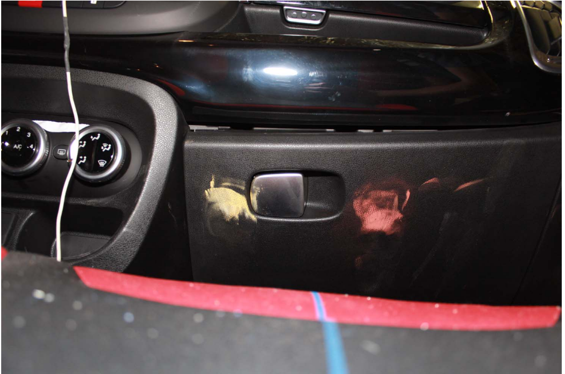
Photo No. 60 - Post-Test Passenger Dummy Knee Contact (glove box)
