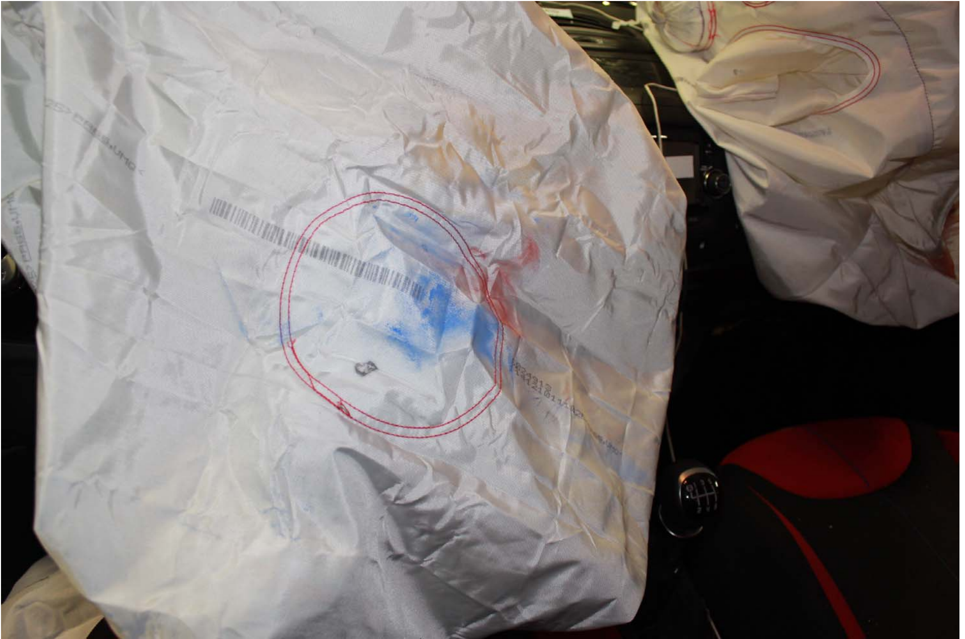
Photo No. 45 - Post-Test Driver Dummy Airbag Contact
