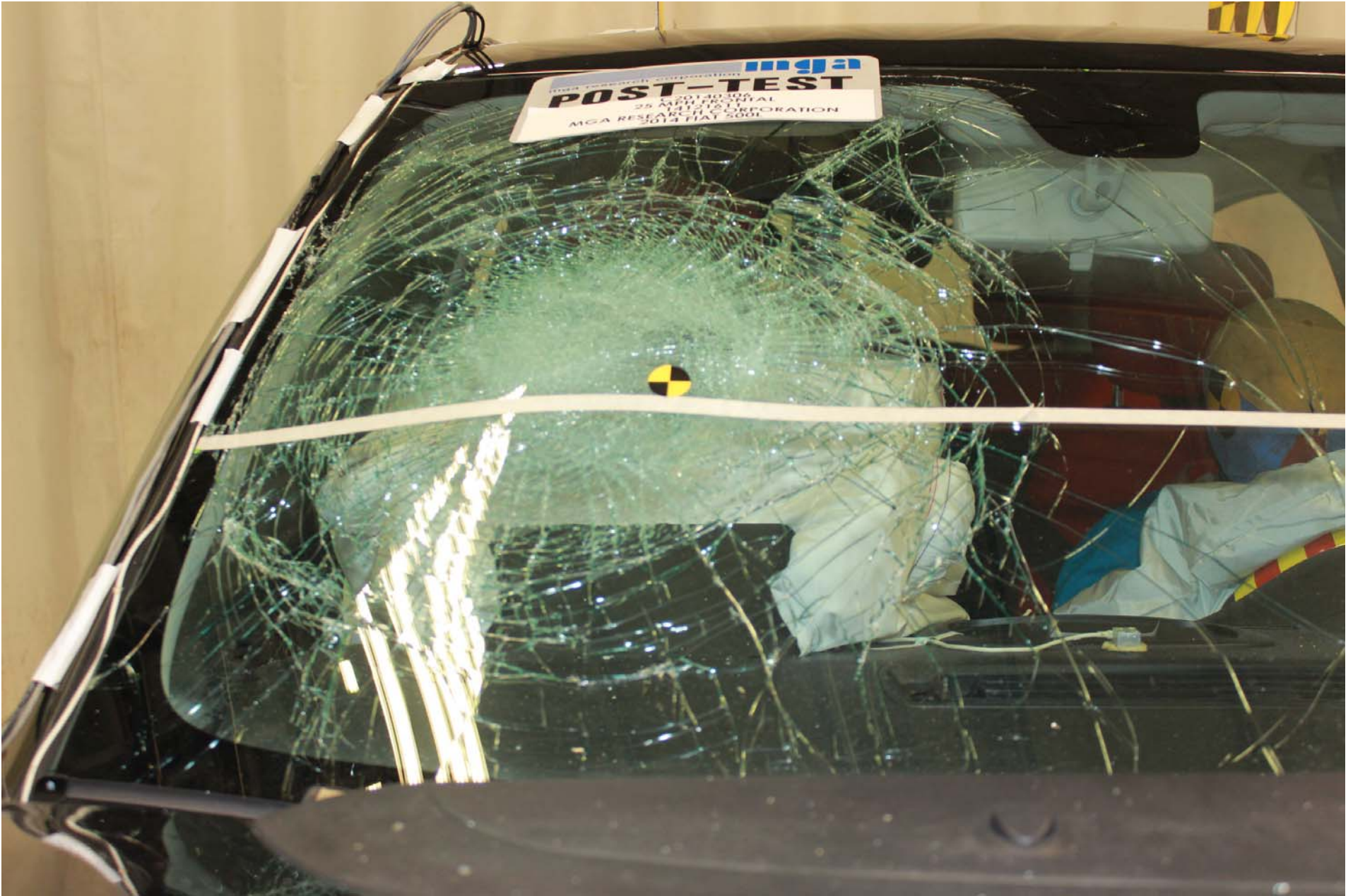
Photo No. 48 - Post-Test Passenger Dummy Front View (head position)
