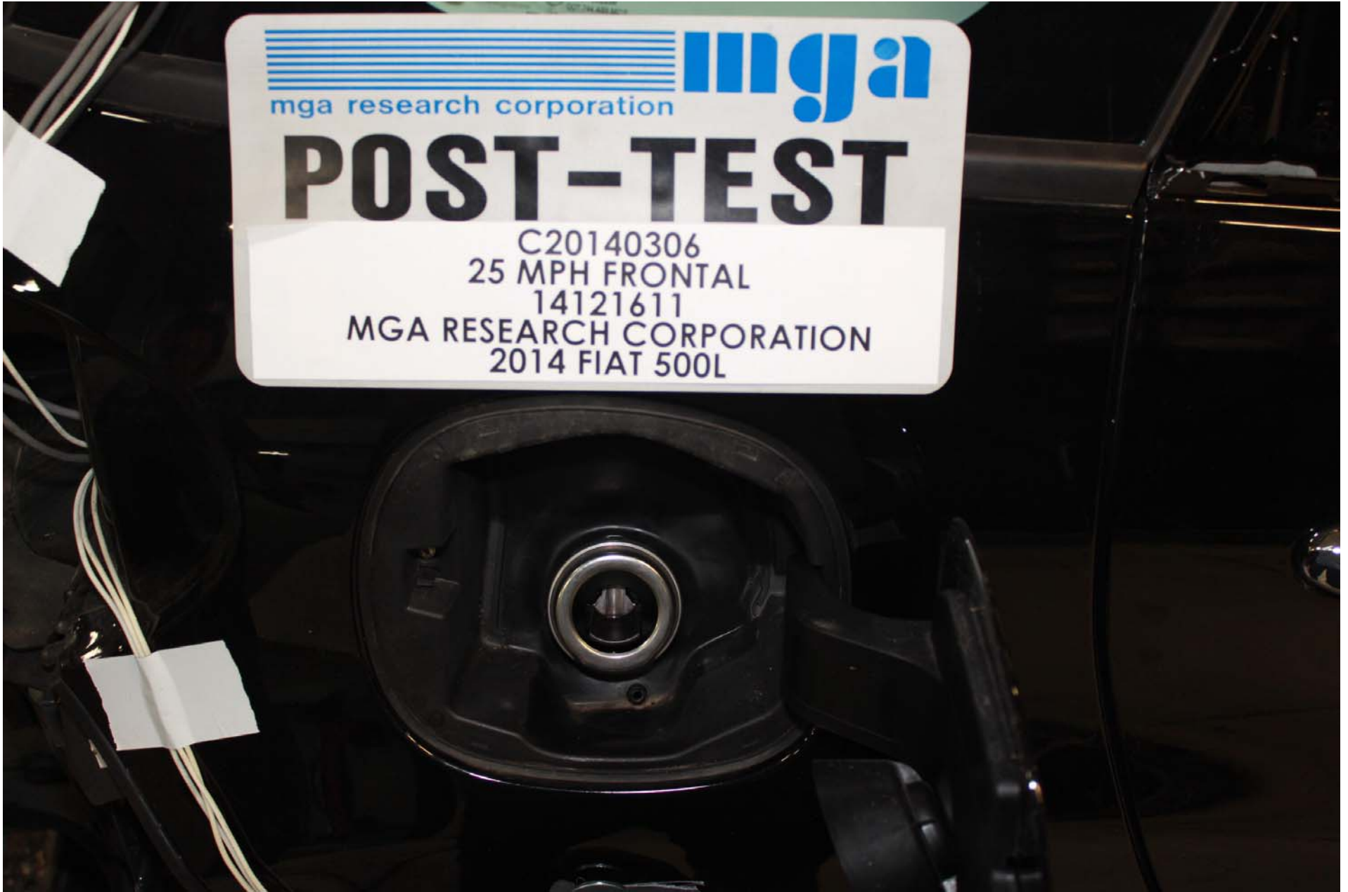
Photo No. 24 - Post-Test Fuel Filler Cap View
