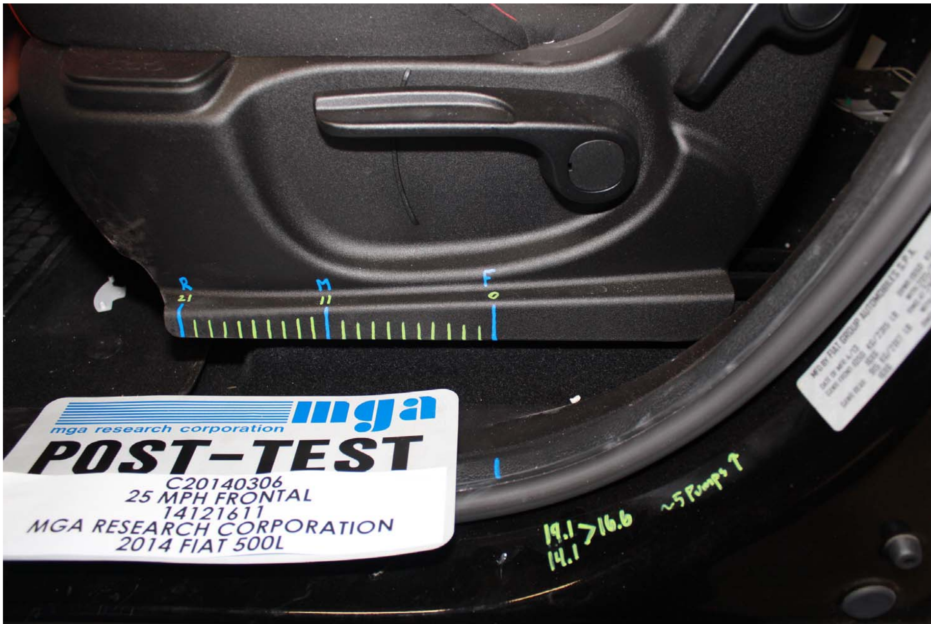
Photo No. 40 - Post-Test Driver Dummy Seat Position
