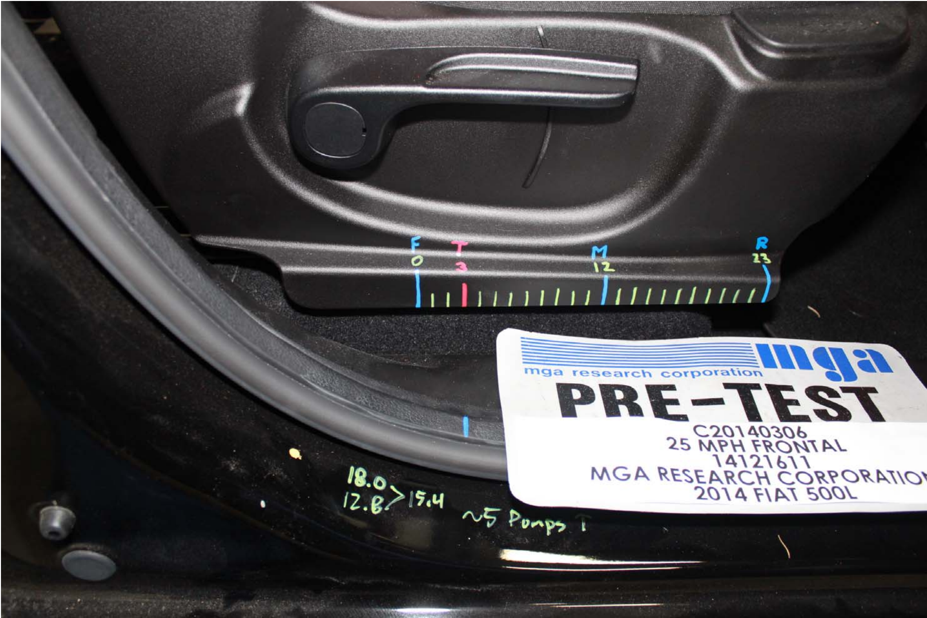
Photo No. 53 - Pre-Test Passenger Dummy Seat Position
