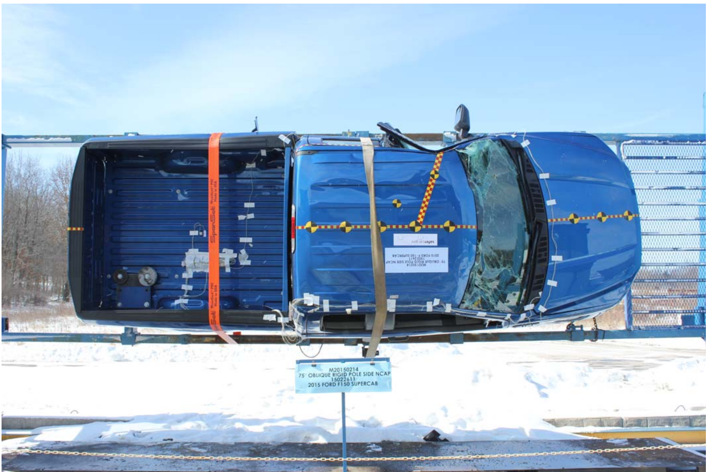
No. 066 FMVSS No. 301 Static Rollover 270 Degrees
