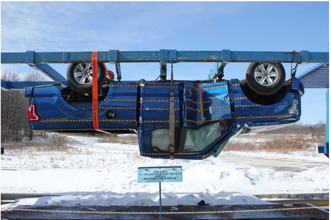
No. 065 FMVSS No. 301 Static Rollover 180 Degrees
