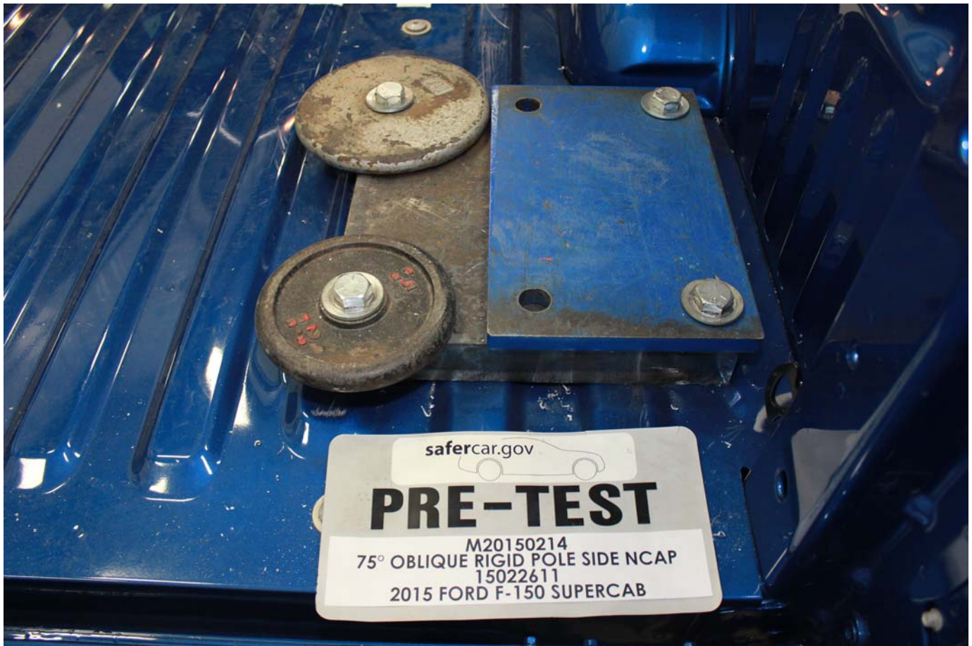
No. 061 Pre-Test Ballast View
