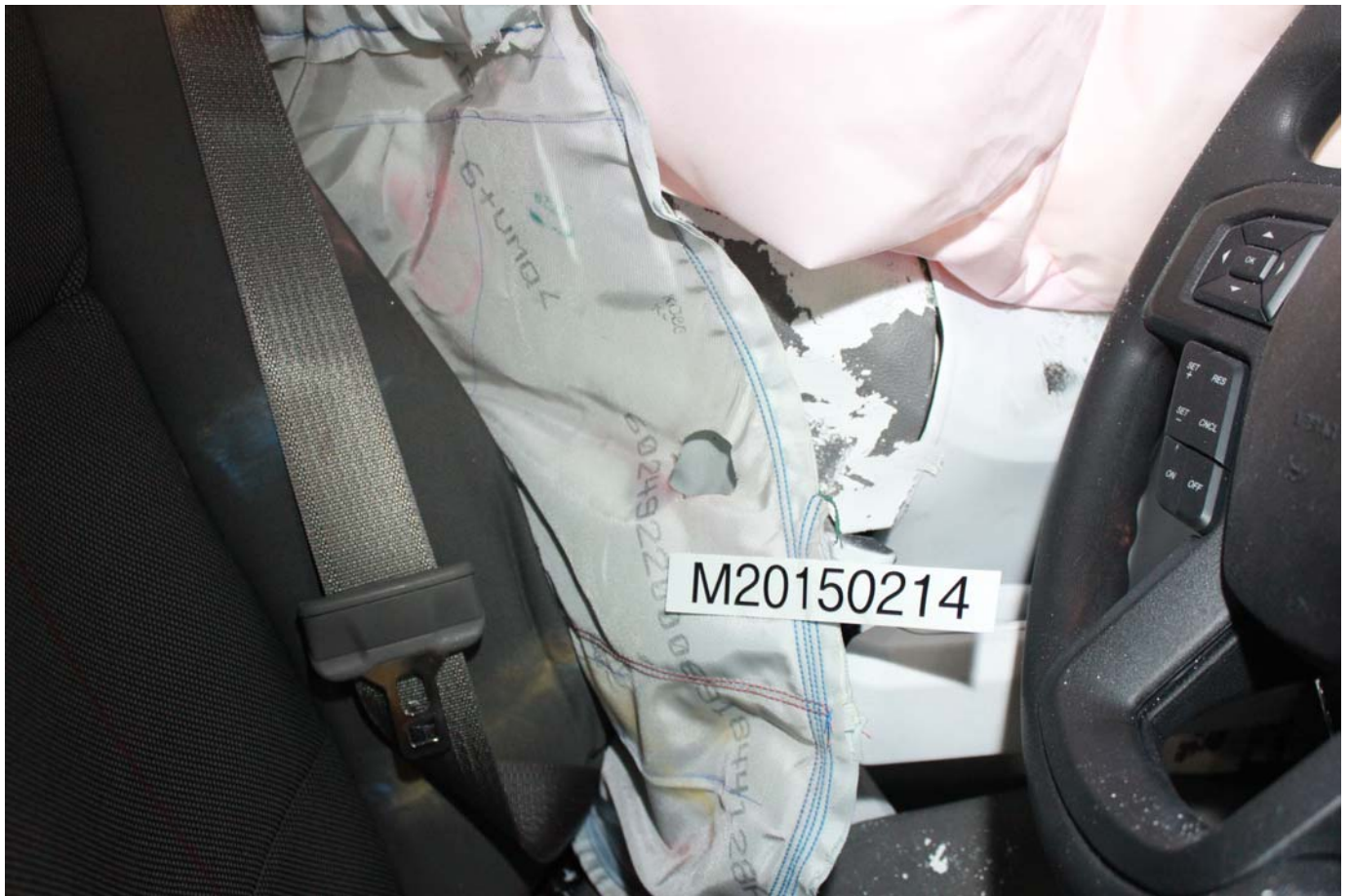
No. 049 Post-Test Dummy Close-Up Torso Contact with Side Air Bag View
