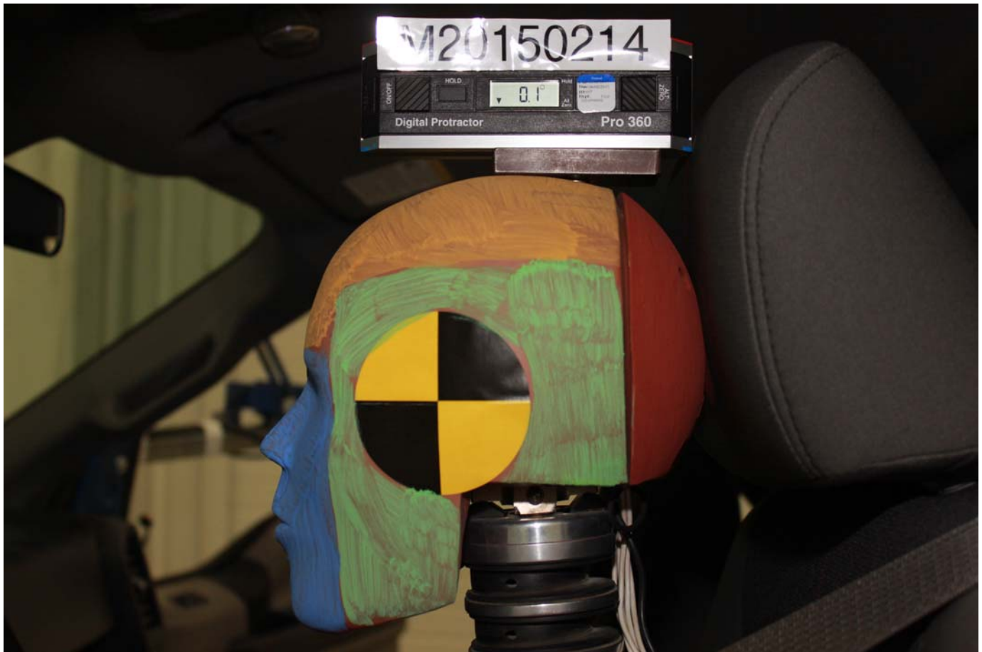
No. 031 Pre-Test Left Side View of Dummy's Head Showing Dummy's Head is Level
