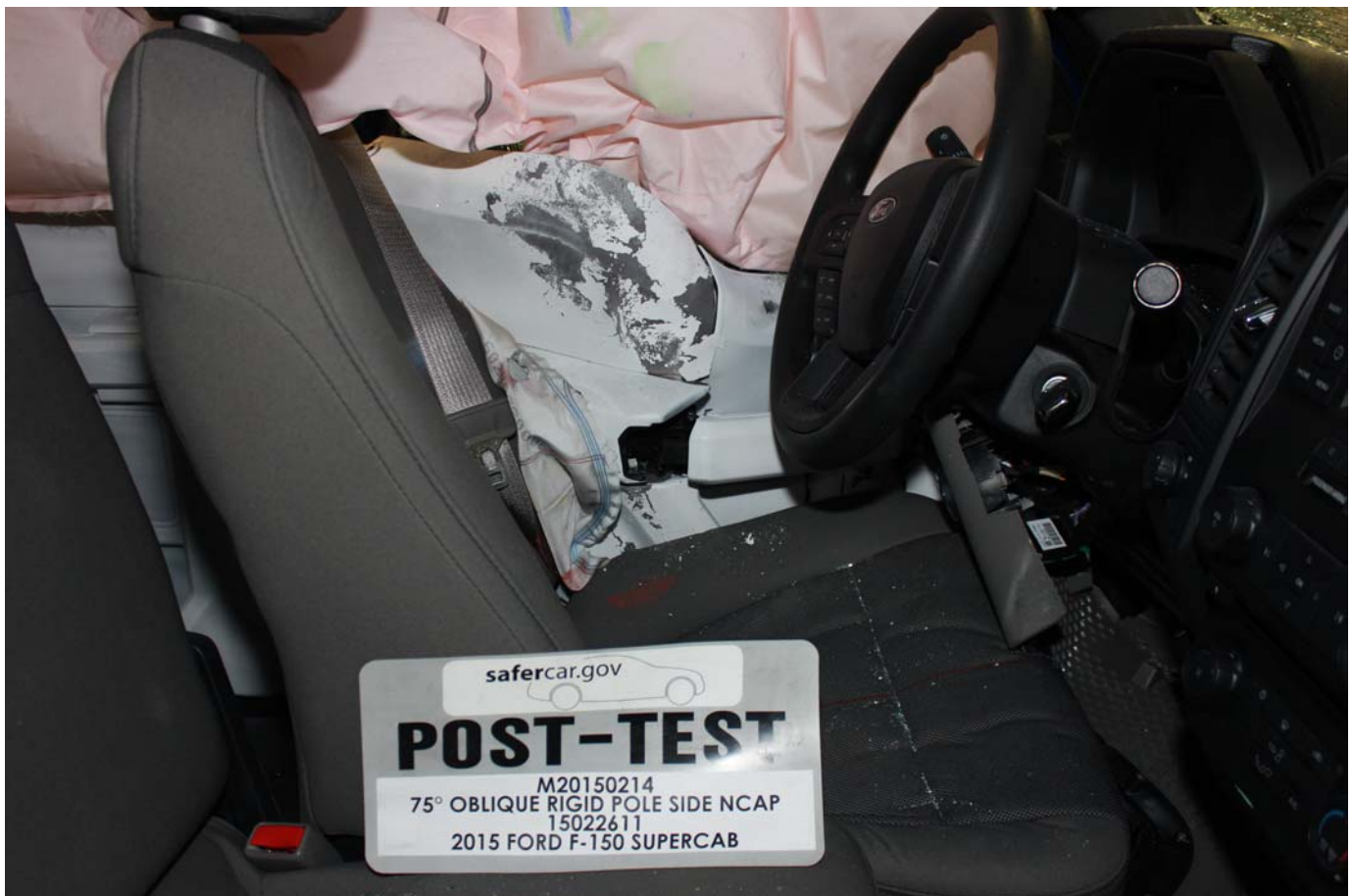
No. 071 Post-Test View of Shattered Vehicle Inner Door Panel
