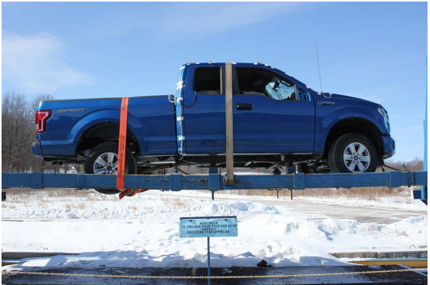
No. 067 FMVSS No. 301 Static Rollover 360 Degrees
