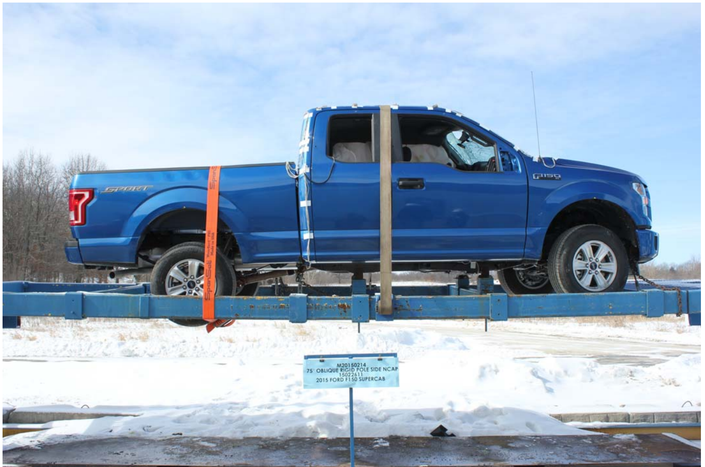
No. 063 FMVSS No. 301 Static Rollover 0 Degrees
