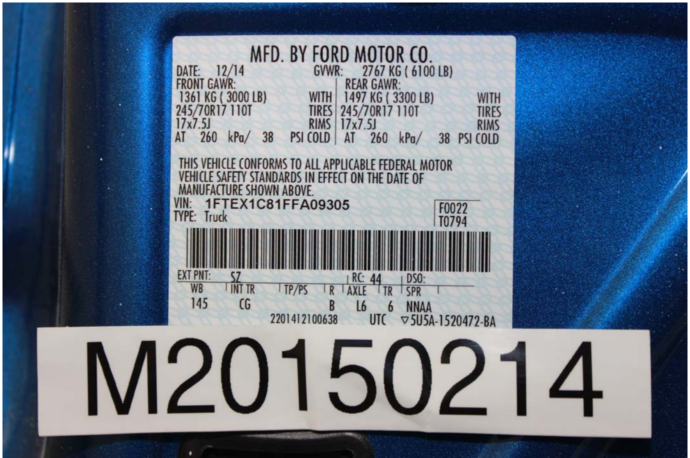
No. 055 Close-Up View of Vehicle's Certification Label
