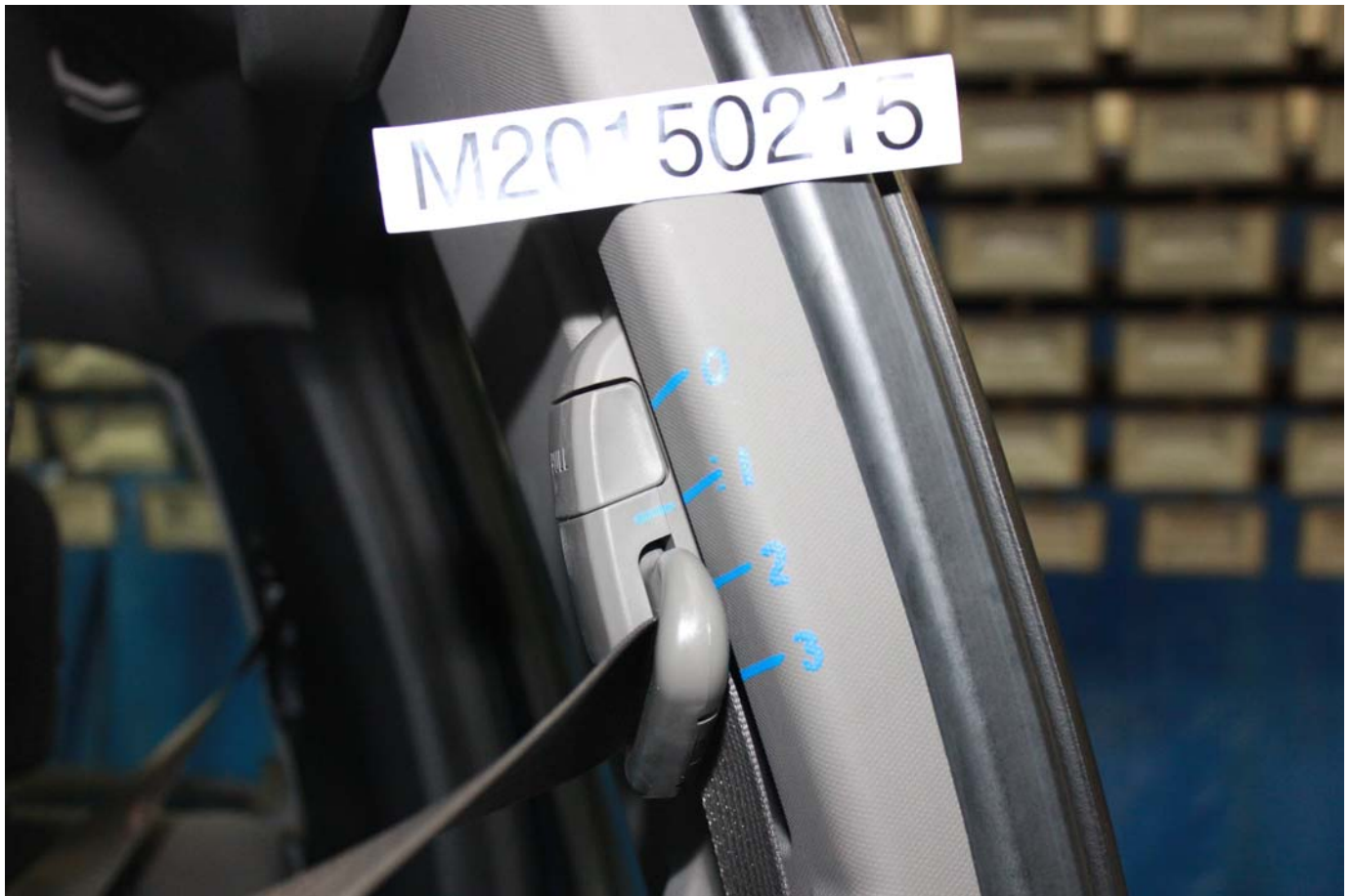
No. 035 Pre-Test View of Belt Anchorage for Driver Dummy
