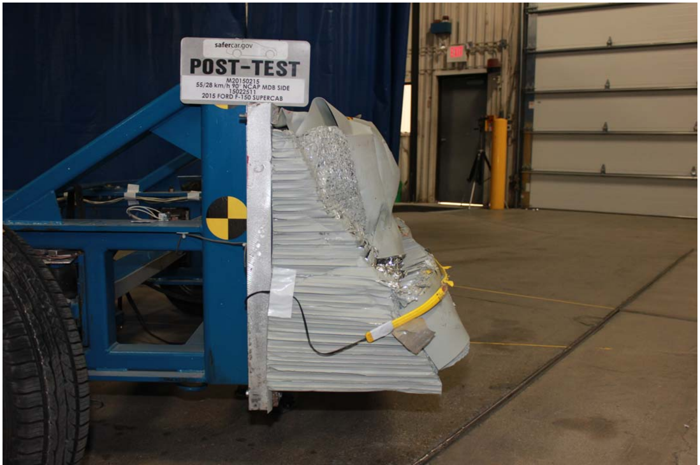
No. 091 Post-Test Right Side View of MDB Impactor Face
