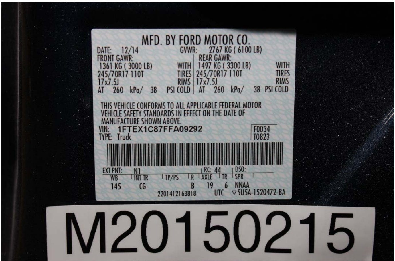
No. 092 Close-Up View of Vehicle's Certification Label
