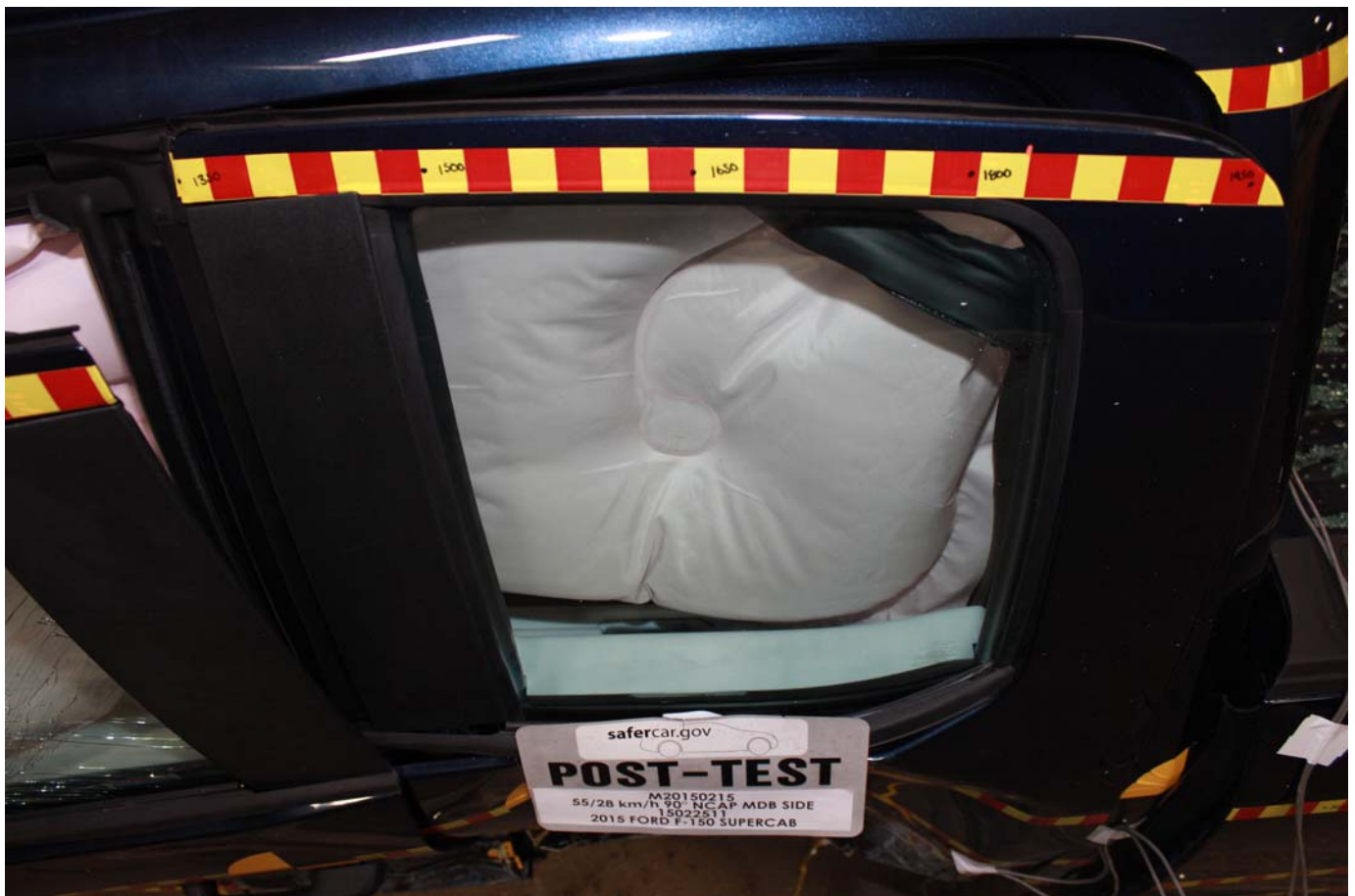
No. 070 Post-Test Rear Passenger Dummy and Door Clearance View
