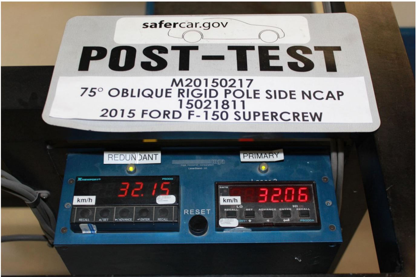
Post-Test Primary and Redundant Speed Trap Read-Out
