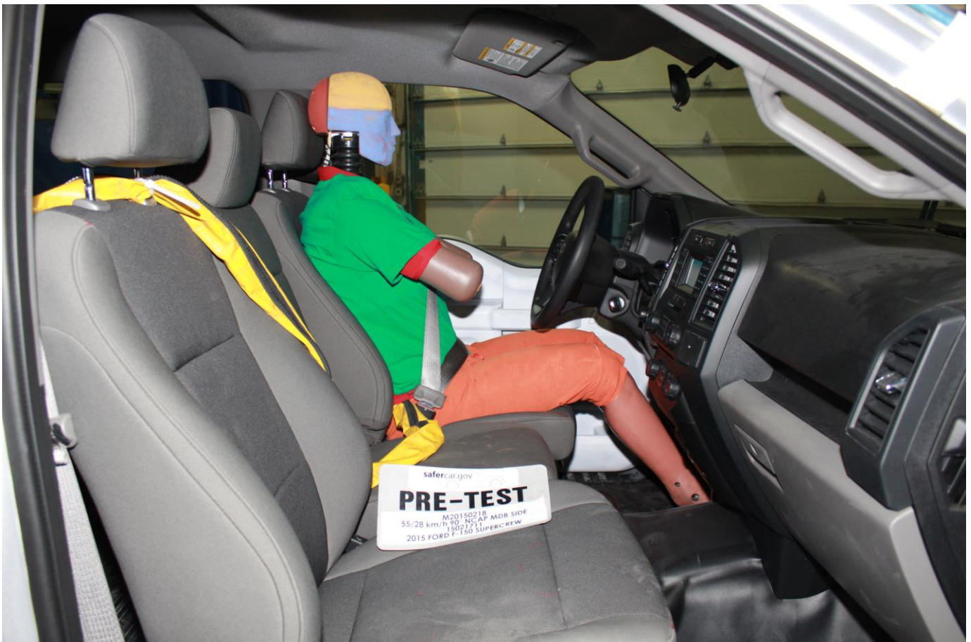
Pre-Test Right Side View of Driver Dummy and Front Seat of Occupant Compartment
