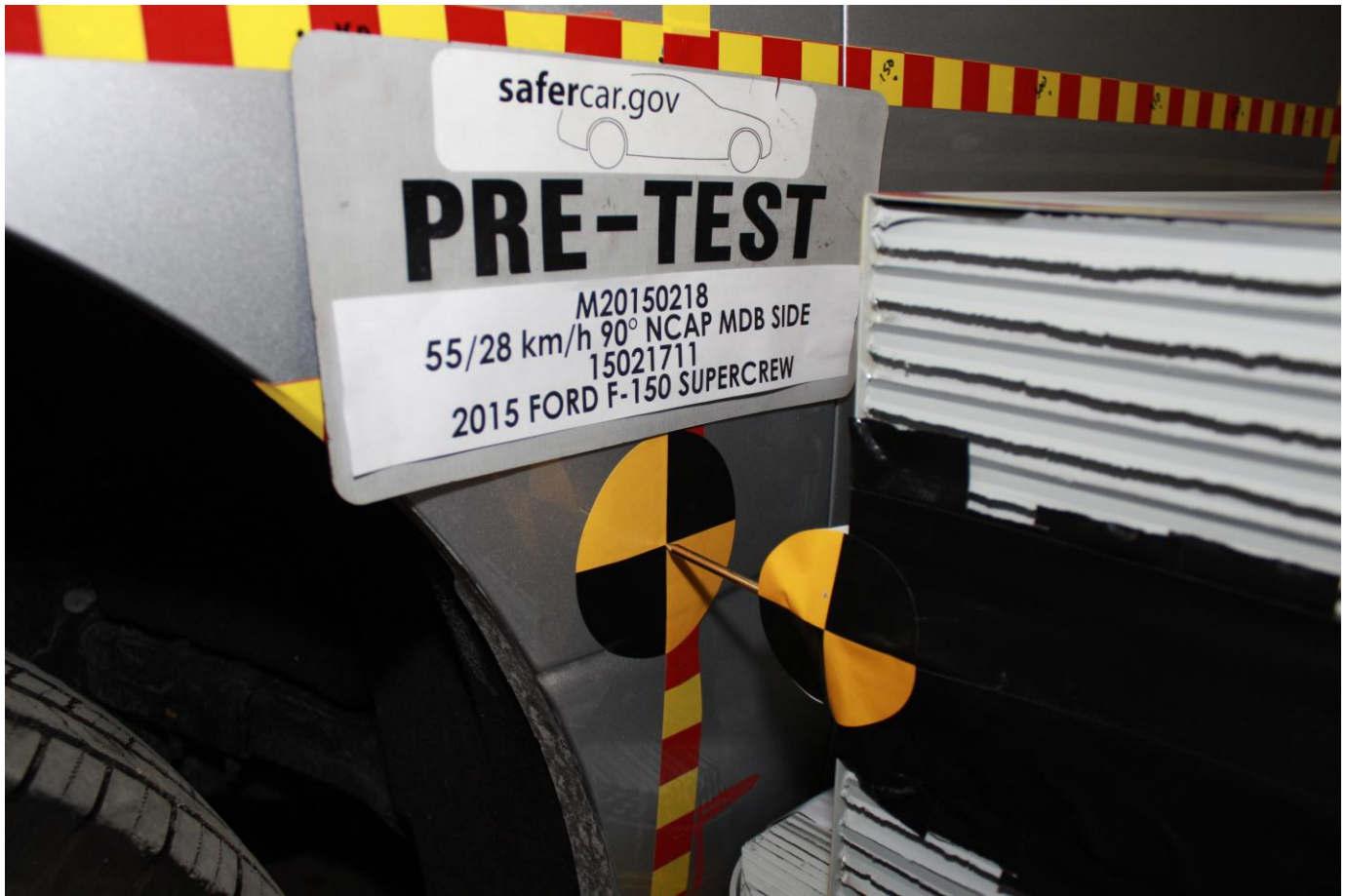
Pre-Test Close-Up View of Impact Point Target
