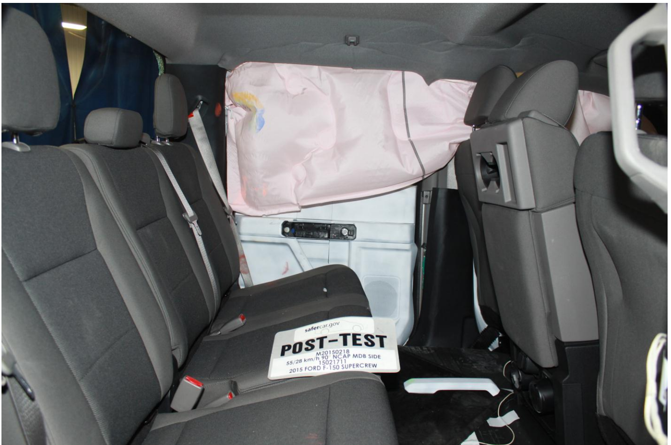
Post-Test Rear Passenger Inner Door Panel View
