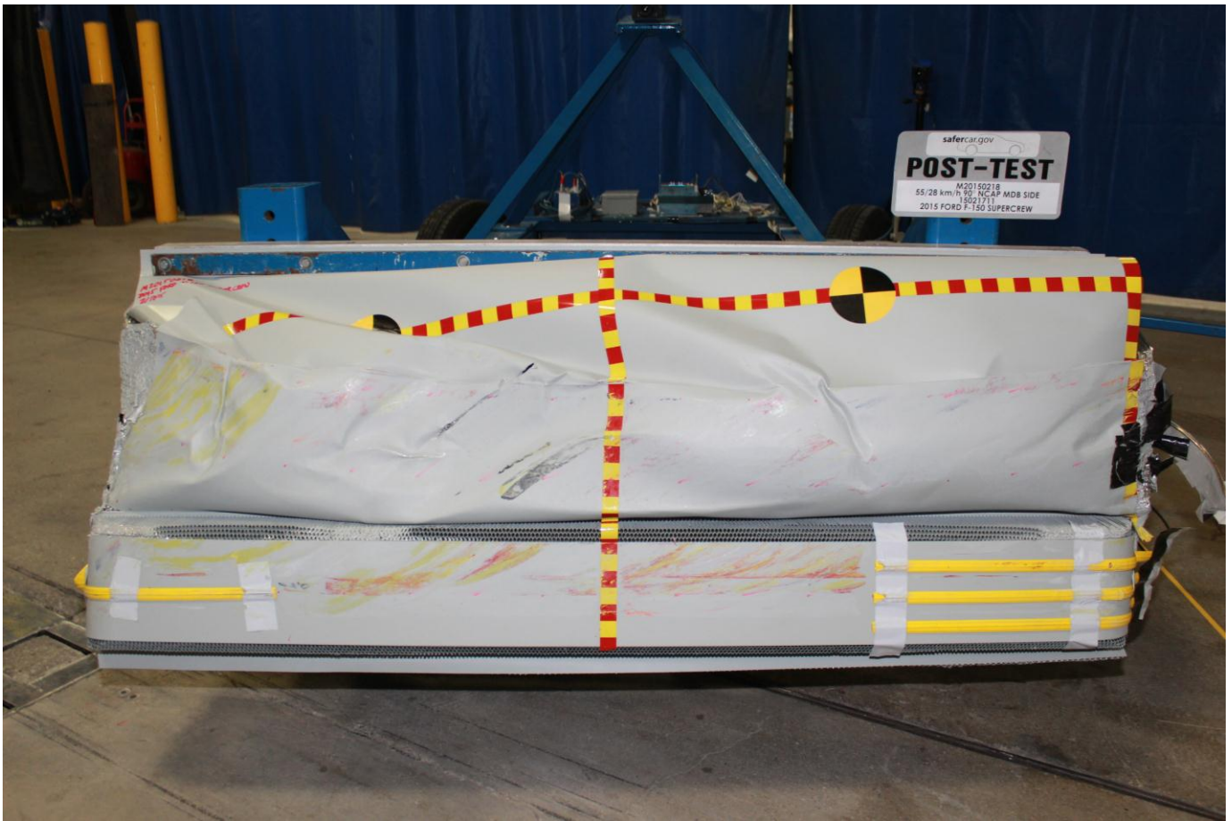
Post-Test Front View of MDB Impactor Face
