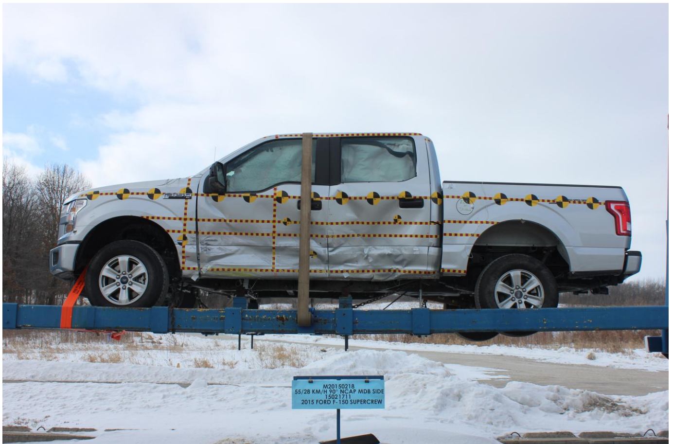
FMVSS No. 301 Static Rollover 360 Degrees
