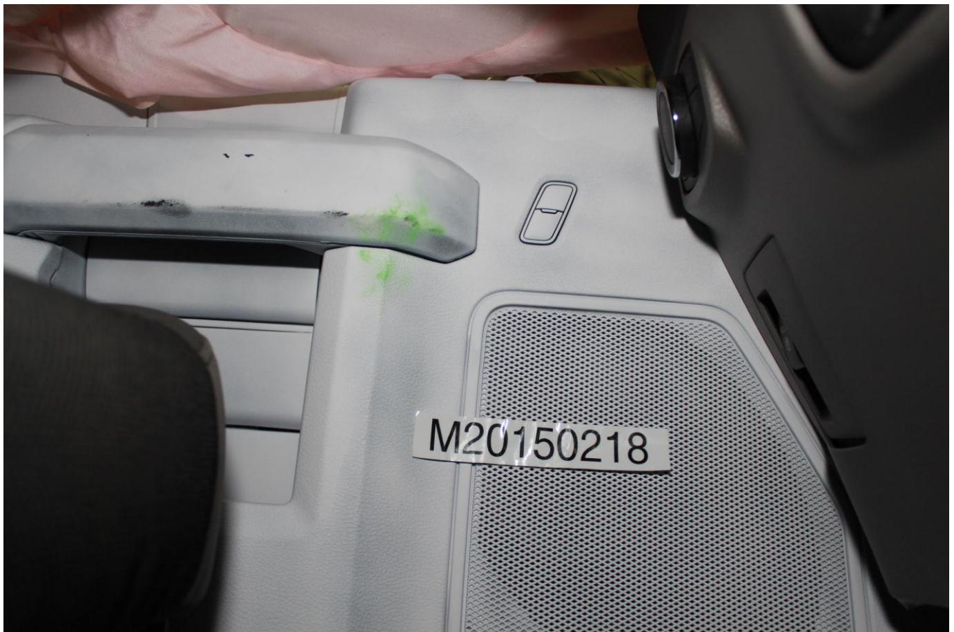
Post-Test Driver Dummy Close-up Knee Contact View
