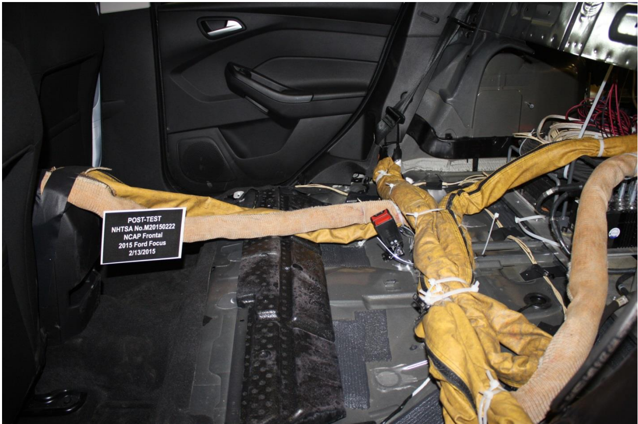
Figure A-28: Post-Test Dummy Cable Routing
