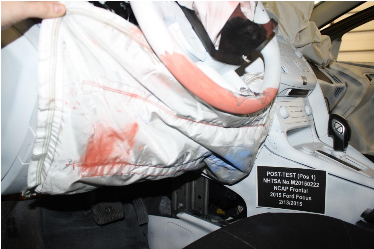
Figure A-42: Post-Test Driver's Side Knee Bolster
