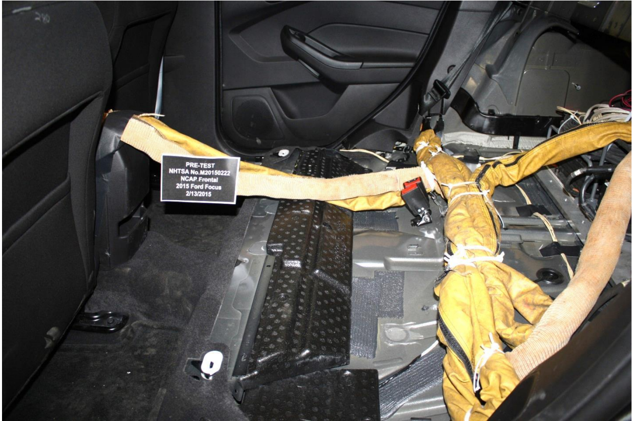
Figure A-27: Pre-Test Dummy Cable Routing
