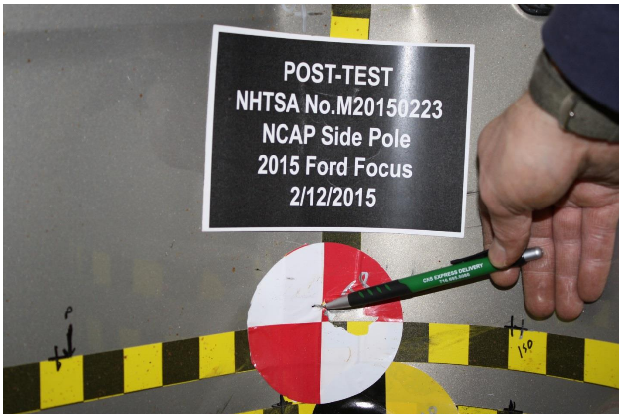
Figure A-20: Post-Test Close-Up View of Impact Point Target Showing Impact Location
