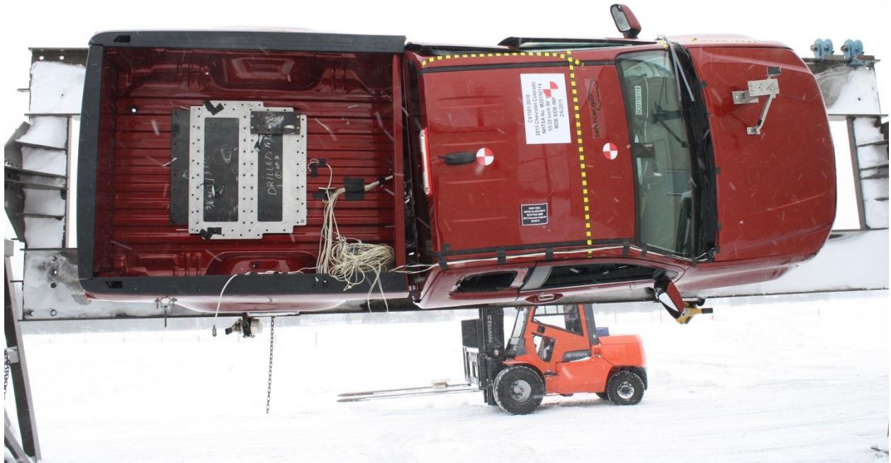
Figure A-99: FMVSS No. 301 Static Rollover 270 Degrees
