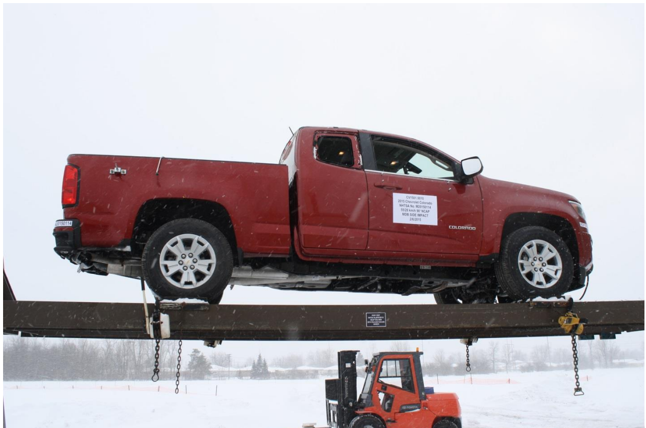
Figure A-100: FMVSS No. 301 Static Rollover 360 Degrees
