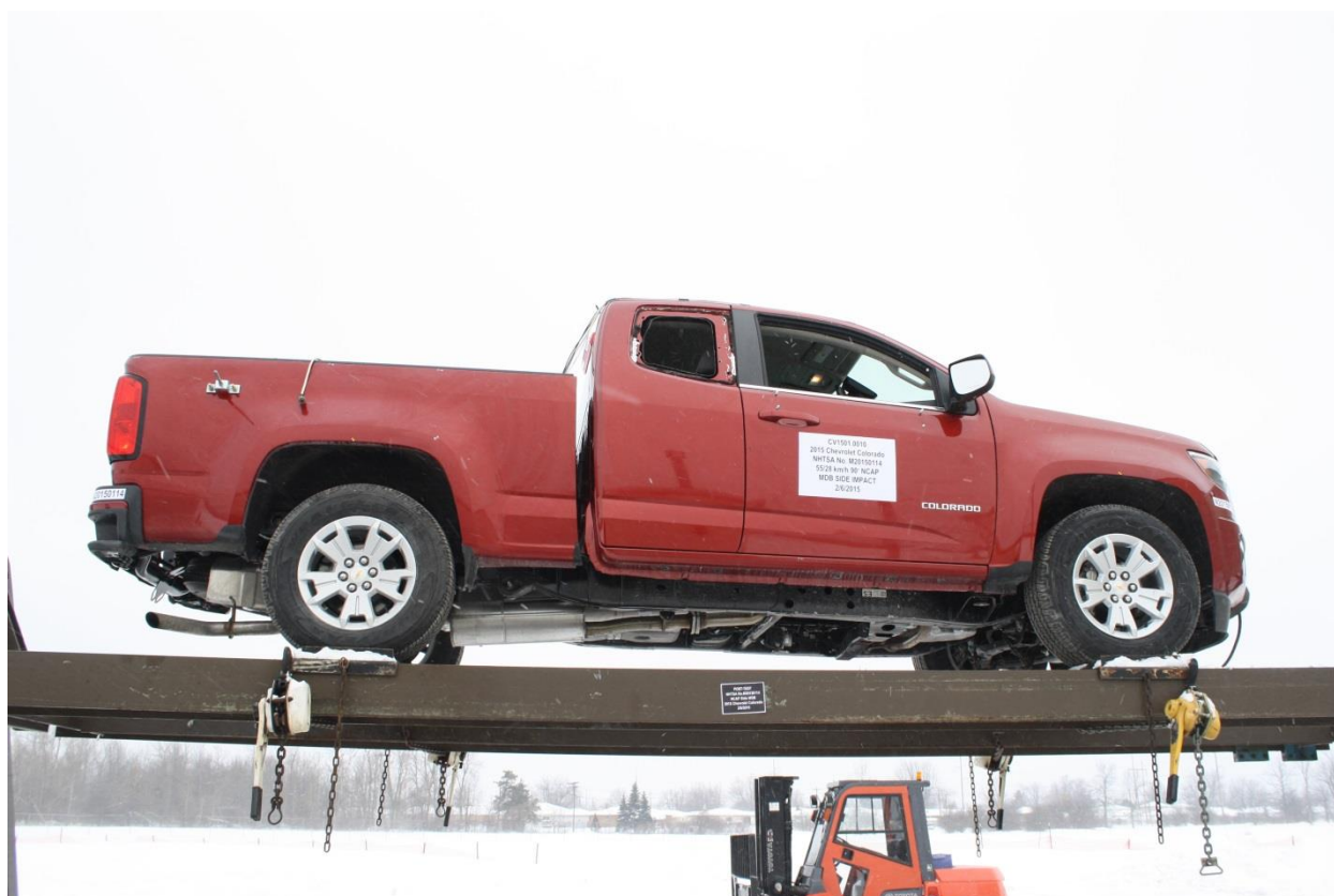
Figure A-96: FMVSS No. 301 Static Rollover 0 Degrees
