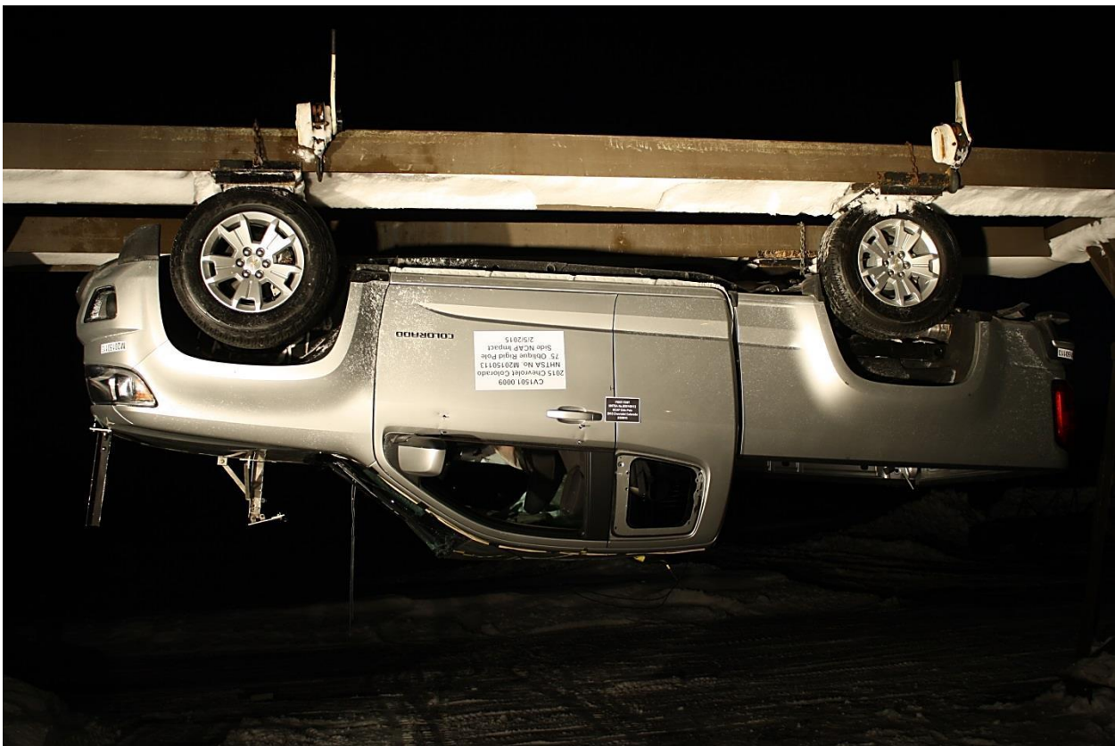
Figure A-65: FMVSS No. 301 Static Rollover 180 Degrees
