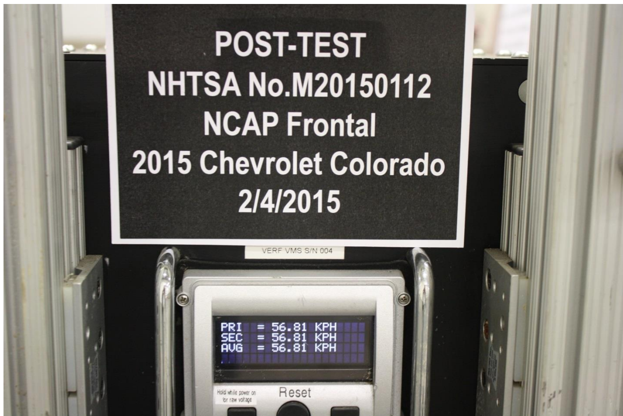
Figure A-71: Post-Test Speed Trap Read-Out
