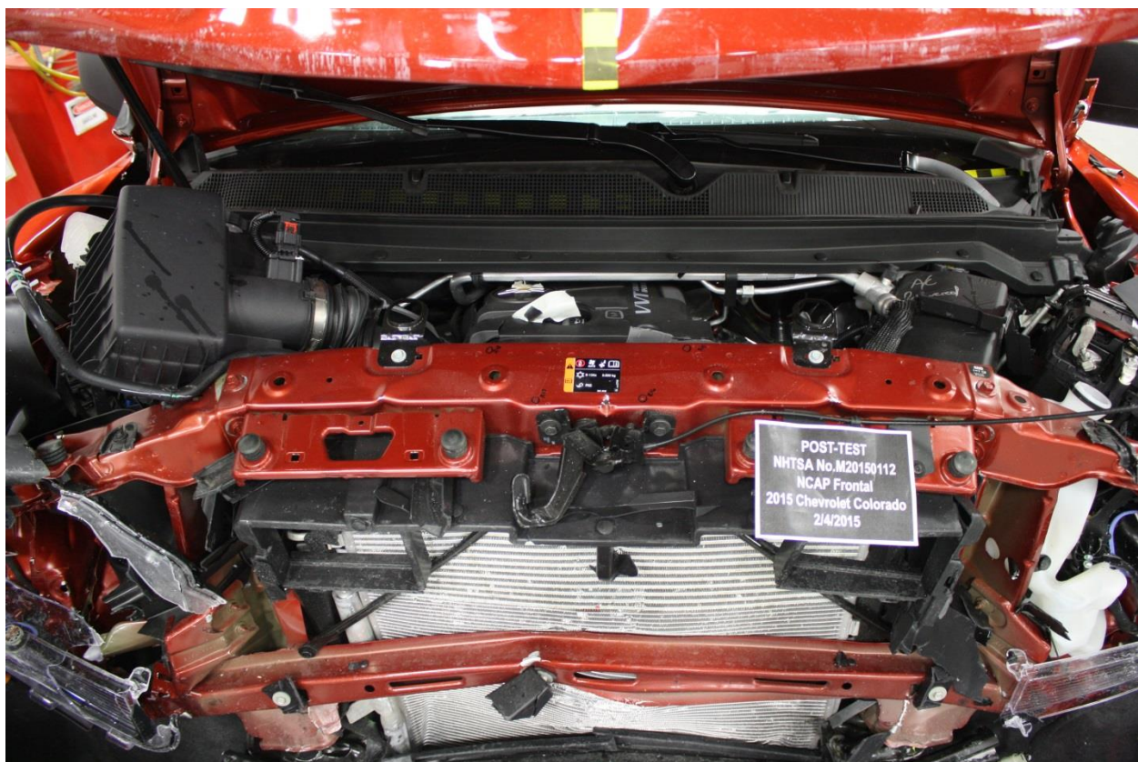
Figure A-20: Post-Test Engine Compartment View
