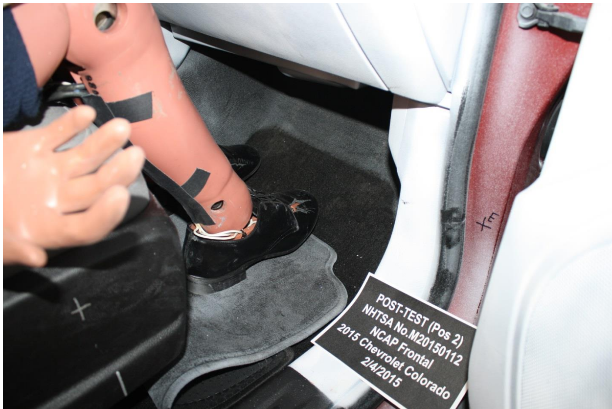
Figure A-61: Post-Test Passenger Dummy Feet
