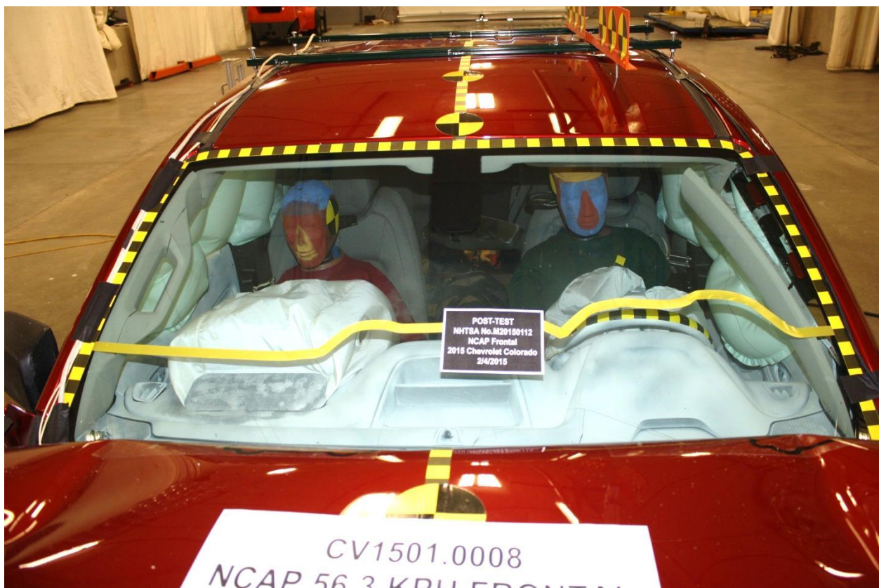
Figure A-18: Post-Test Windshield View
