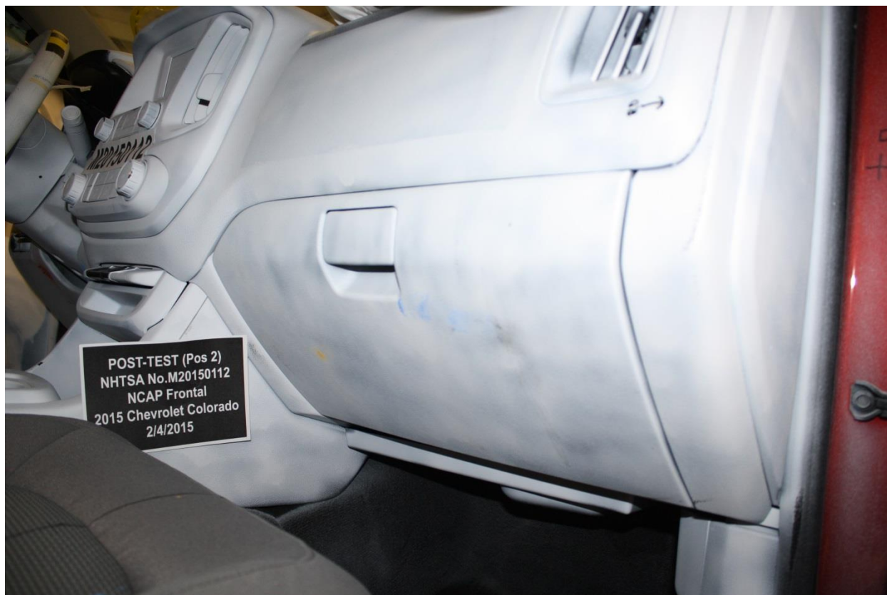
Figure A-63: Post-Test Passenger's Side Knee Bolster
