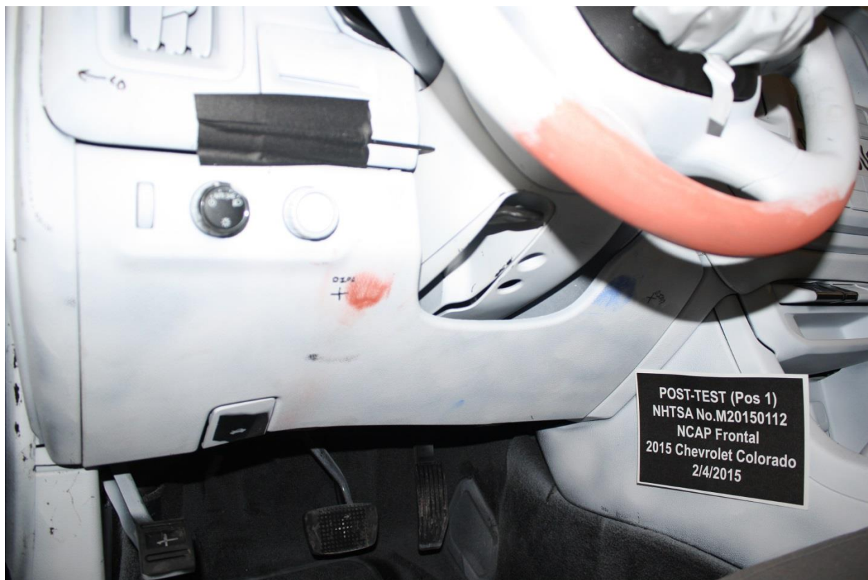
Figure A-42: Post-Test Driver's Side Knee Bolster
