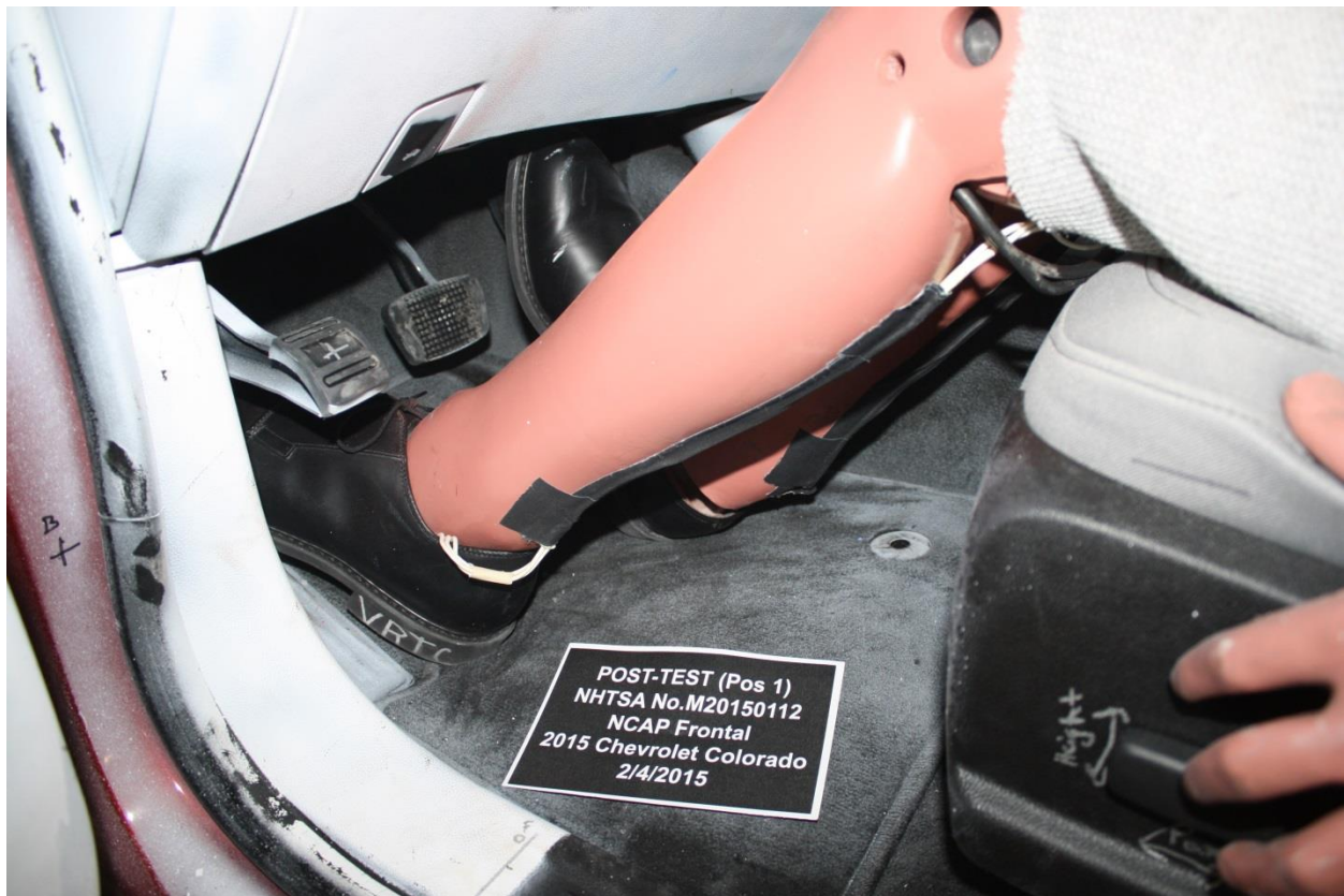
Figure A-40: Post-Test Driver Dummy Feet
