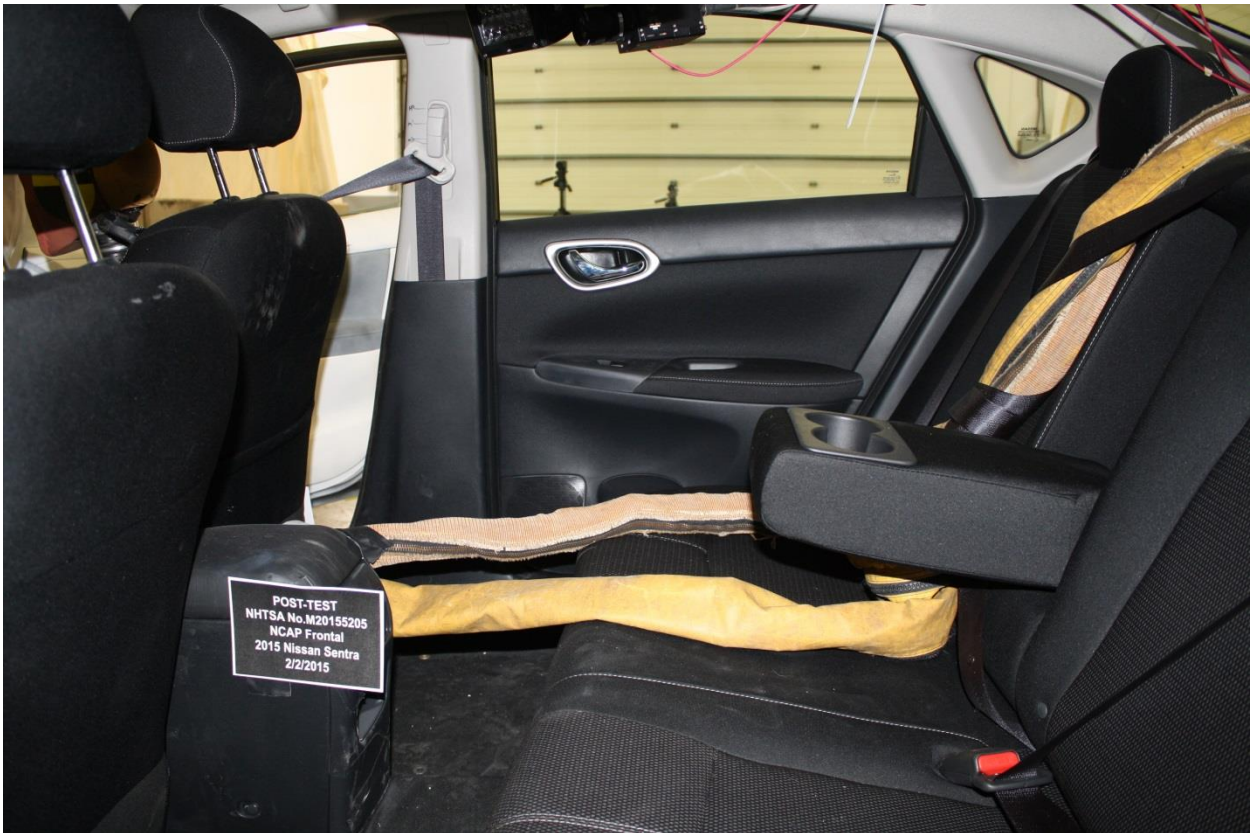
Figure A-28: Post-Test Dummy Cable Routing
