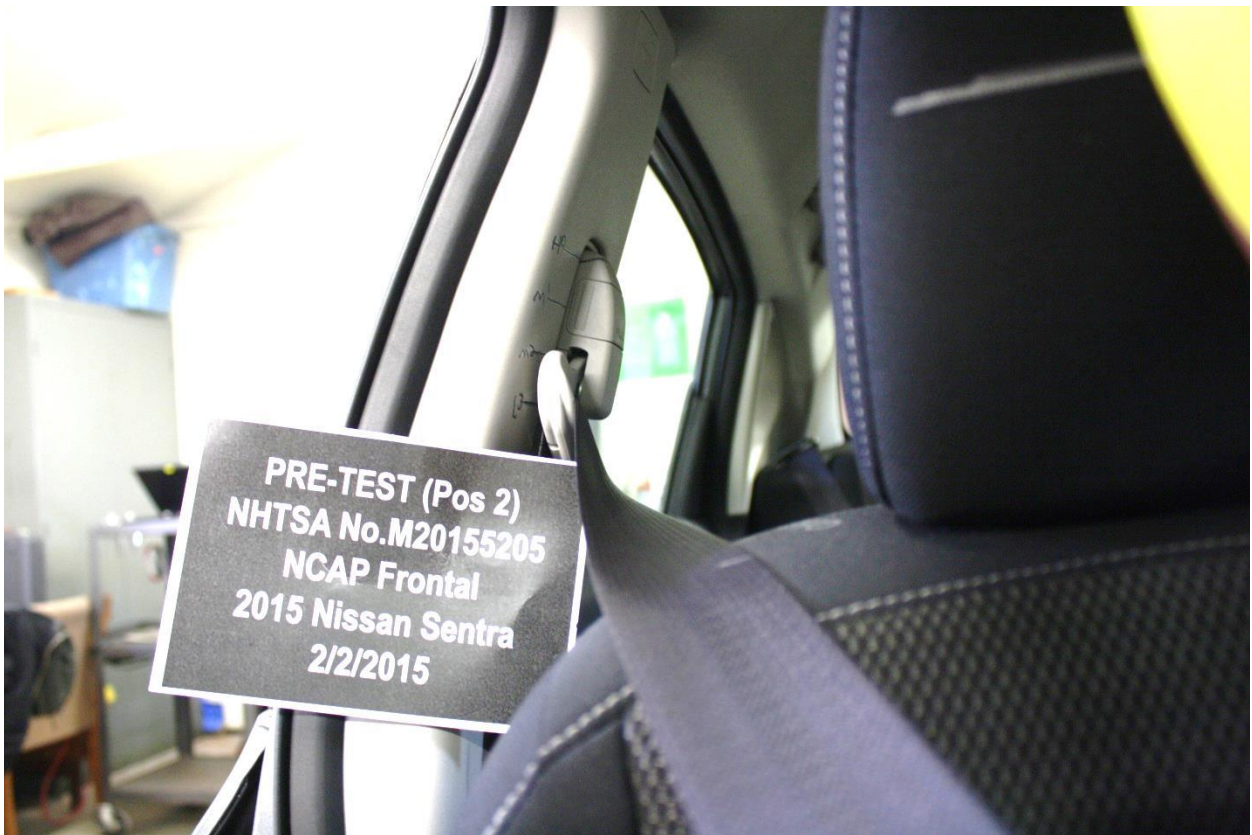
Figure A-58: Pre-Test View of Belt Anchorage for Passenger Dummy
