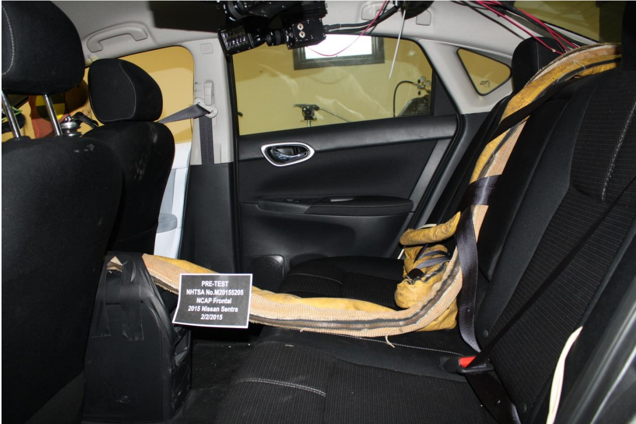
Figure A-27: Pre-Test Dummy Cable Routing
