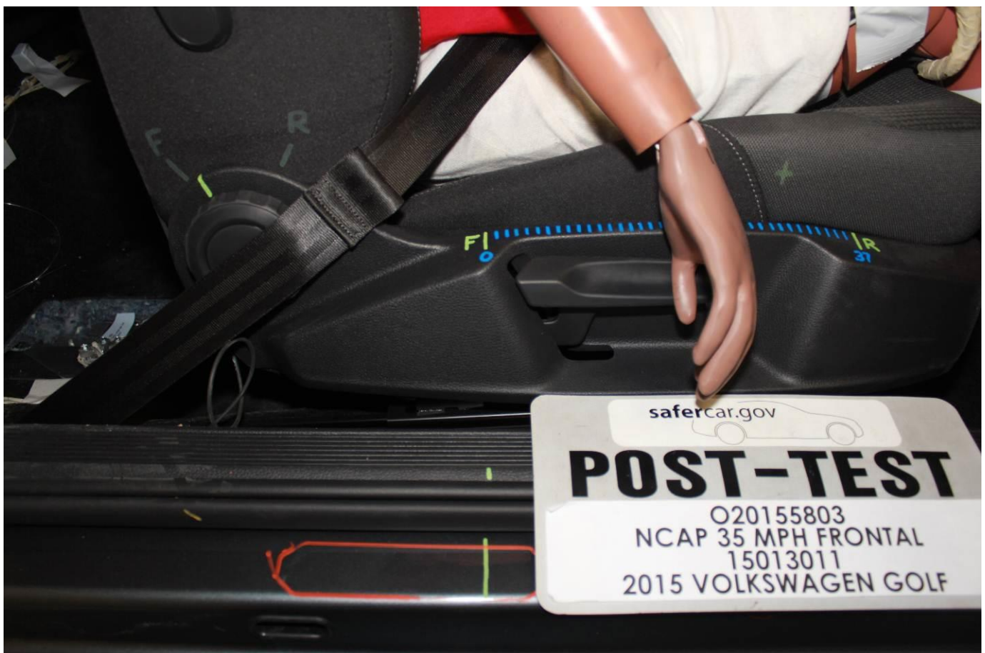
Post-Test Passenger's Seat Fore-Aft Markings
