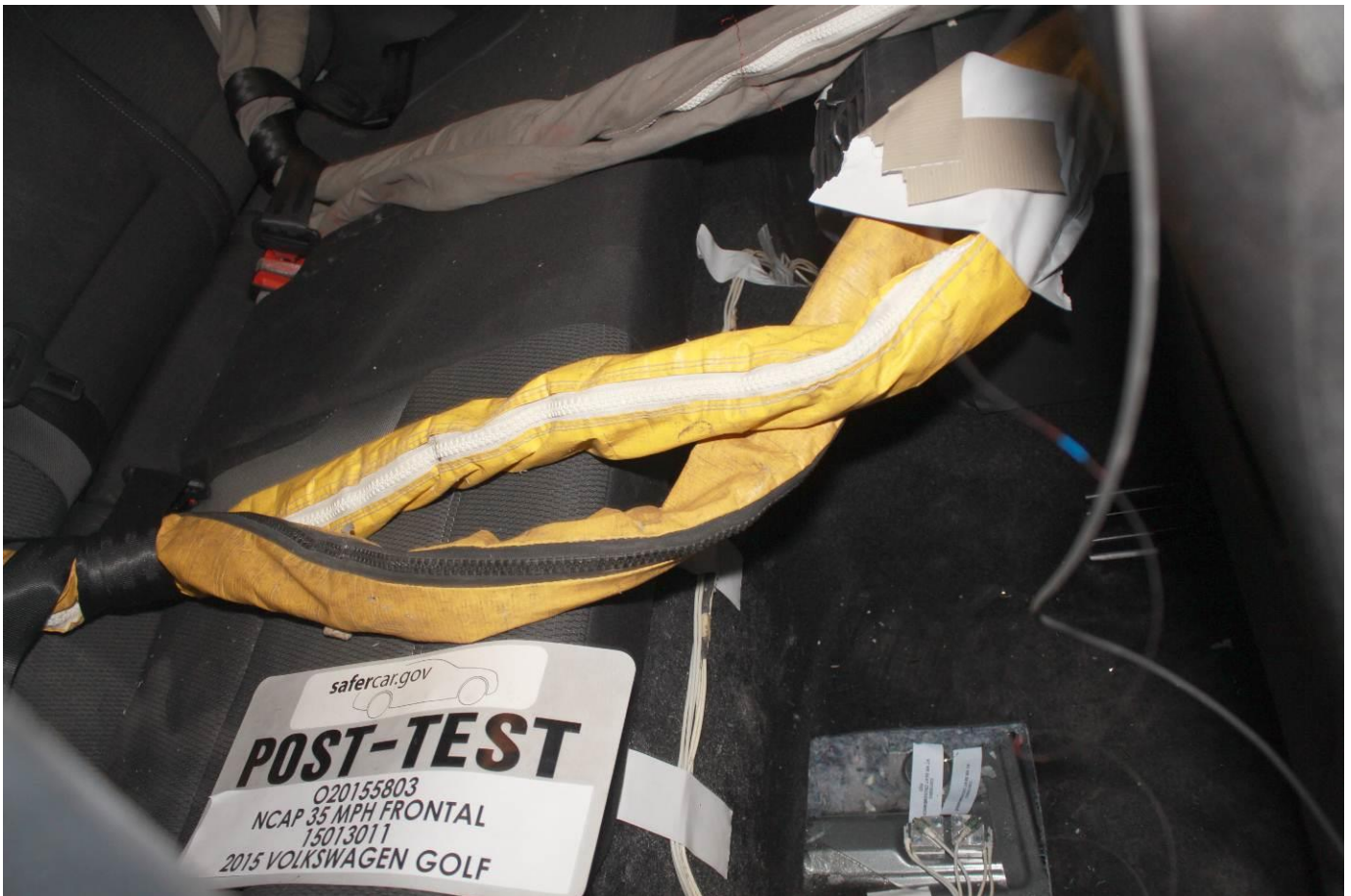
Post-Test Dummy Cable Routing
