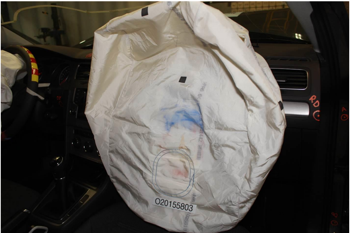
Post-Test Passenger Dummy Contact with Airbag
