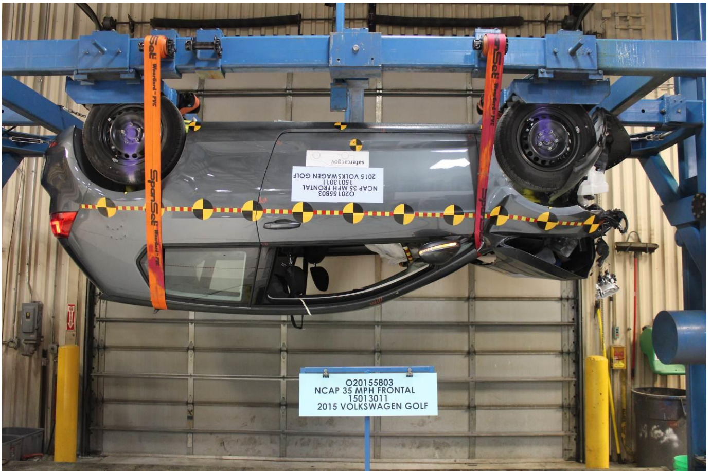
Vehicle at 180 Degrees on Static Rollover Device
