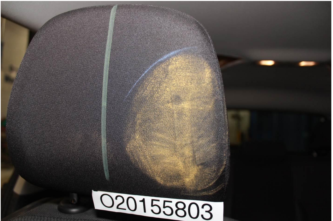
Post-Test Passenger Dummy Contact with Headrest
