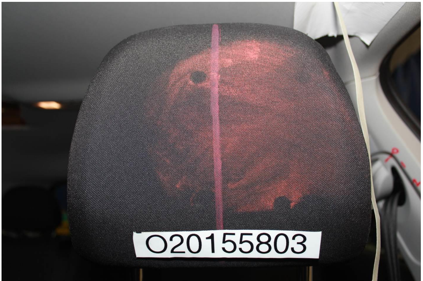
Post-Test Driver Dummy Contact with Headrest
