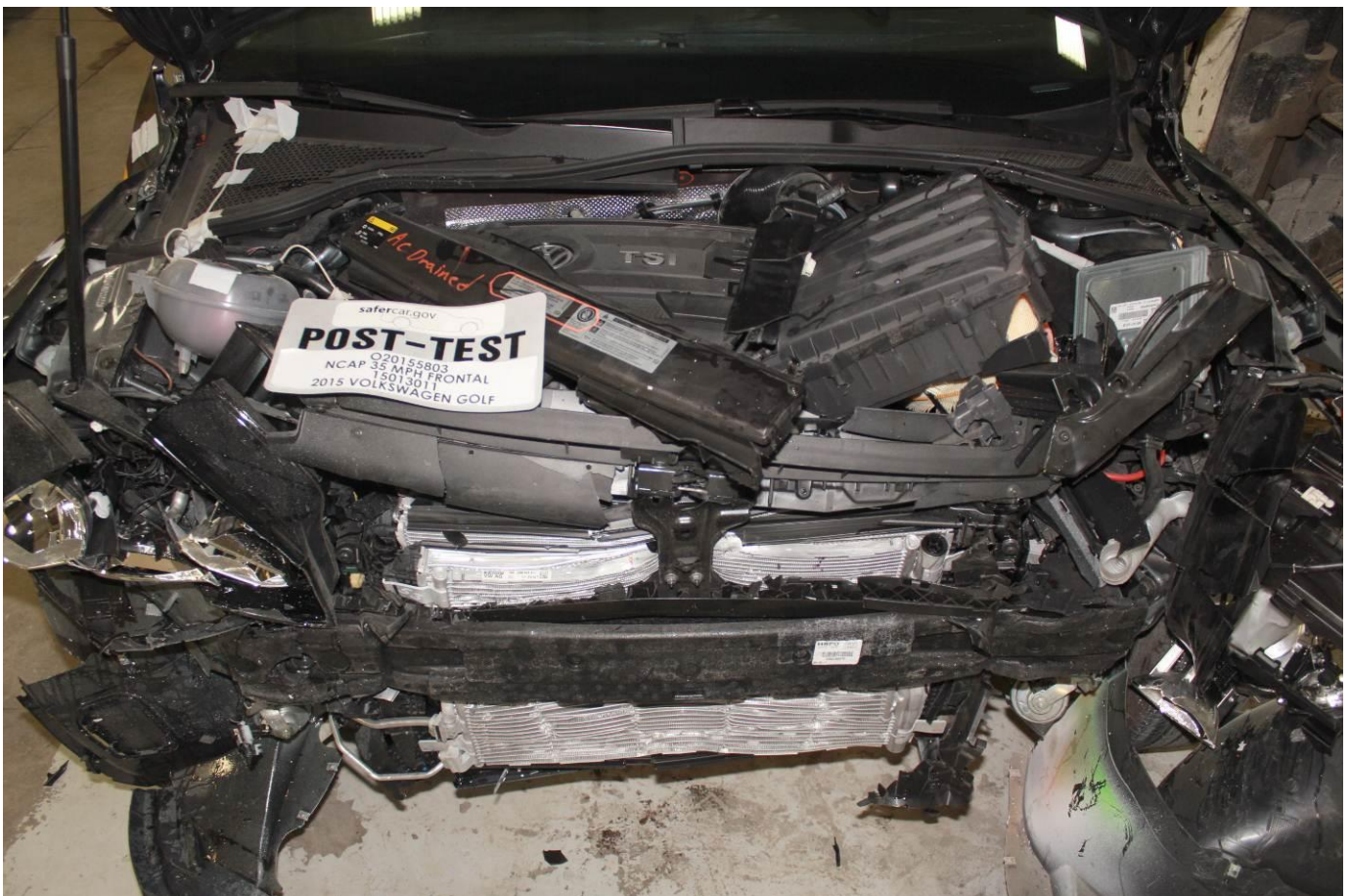
Post-Test Engine Compartment View
