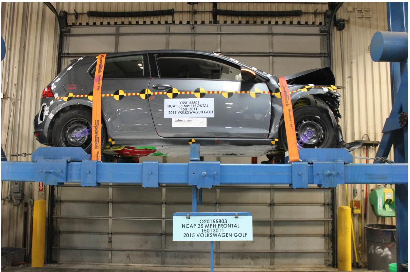
Vehicle at 360 Degrees on Static Rollover Device
