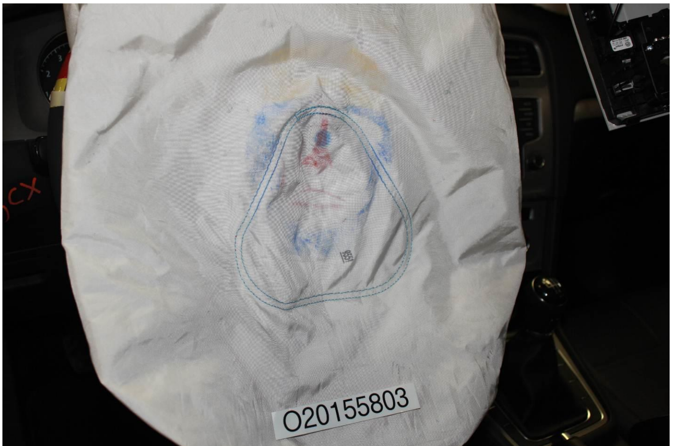
Post-Test Driver Dummy Contact with Airbag
