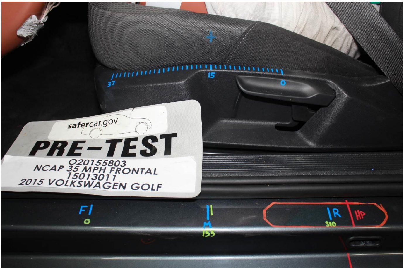
Pre-Test Driver's Seat Fore-Aft Markings
