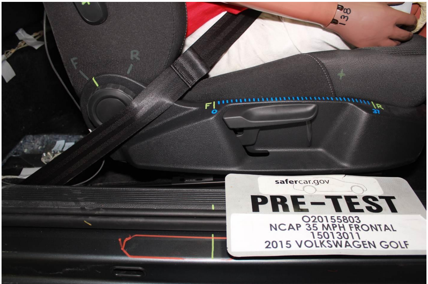
Pre-Test Passenger's Seat Fore-Aft Markings
