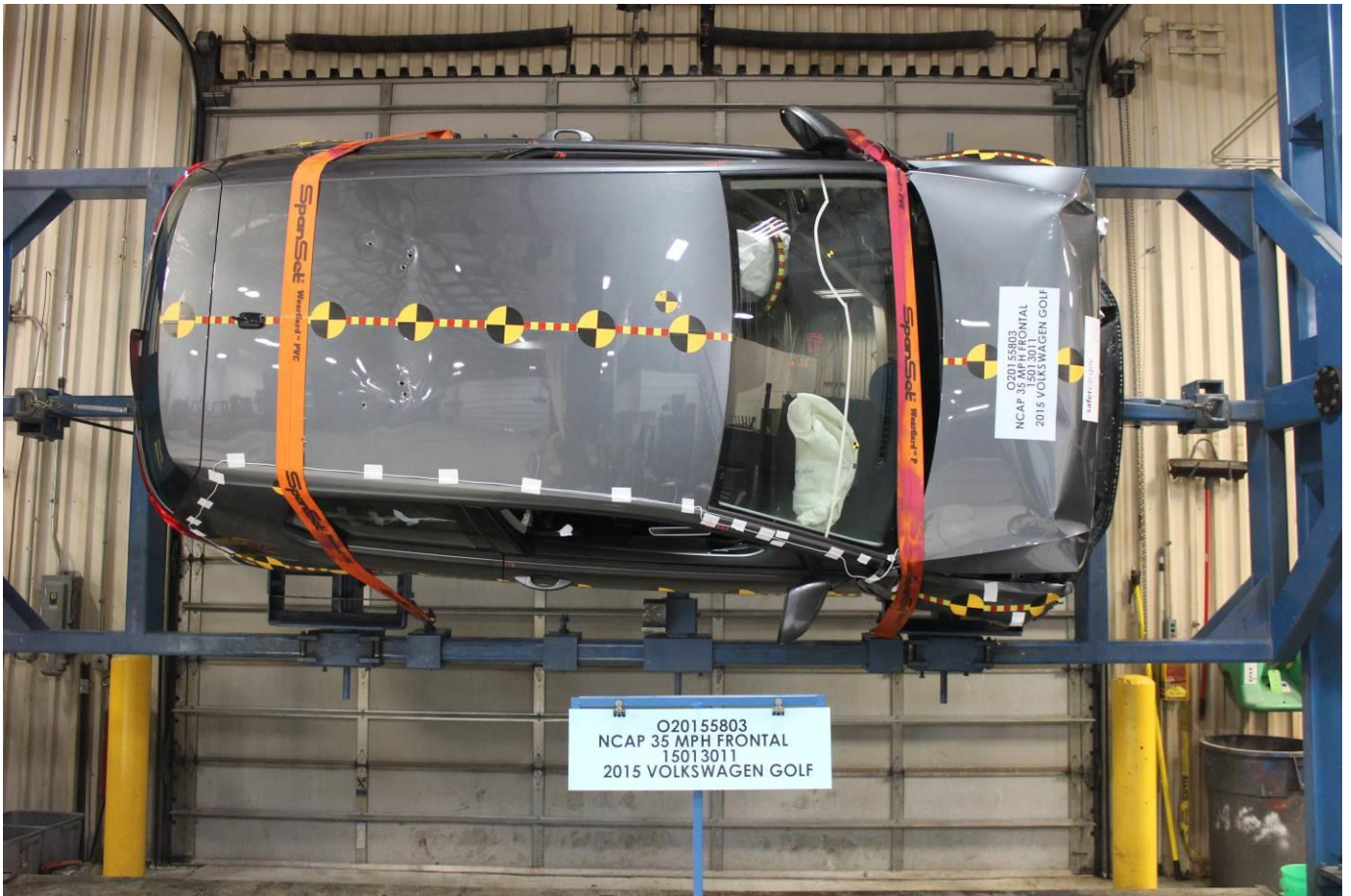
Vehicle at 90 Degrees on Static Rollover Device
