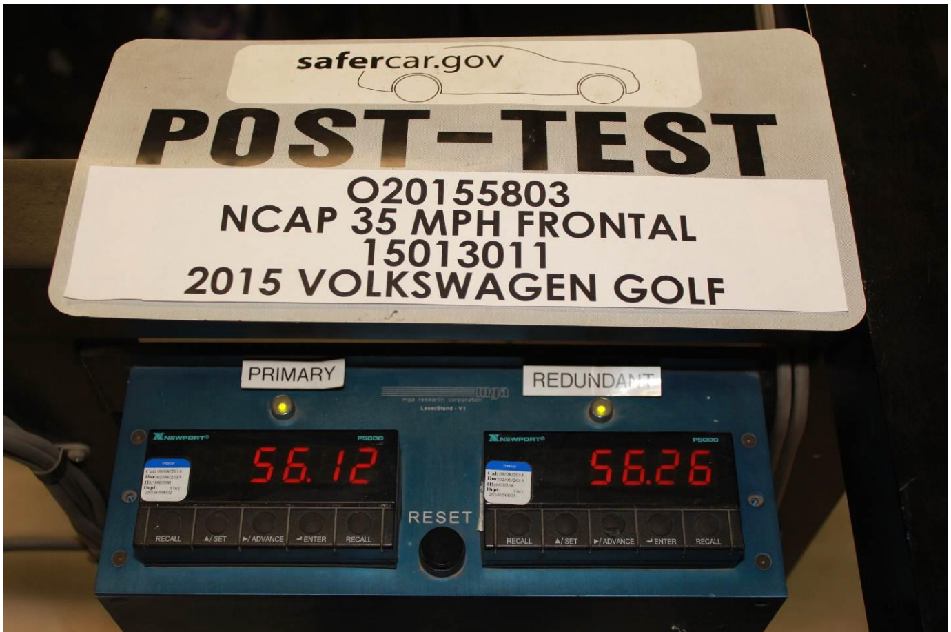
Post-Test Speed Trap Read-Out
