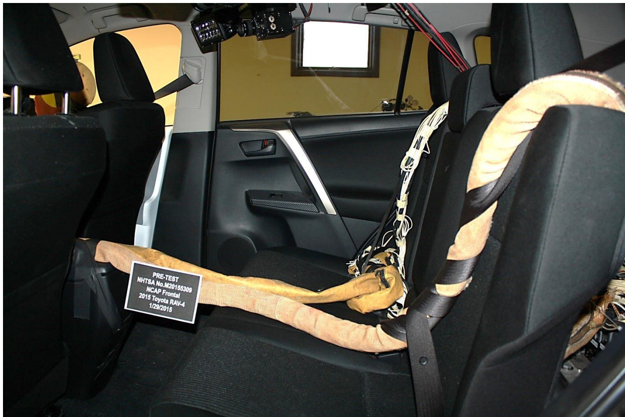
Figure A-27: Pre-Test Dummy Cable Routing
