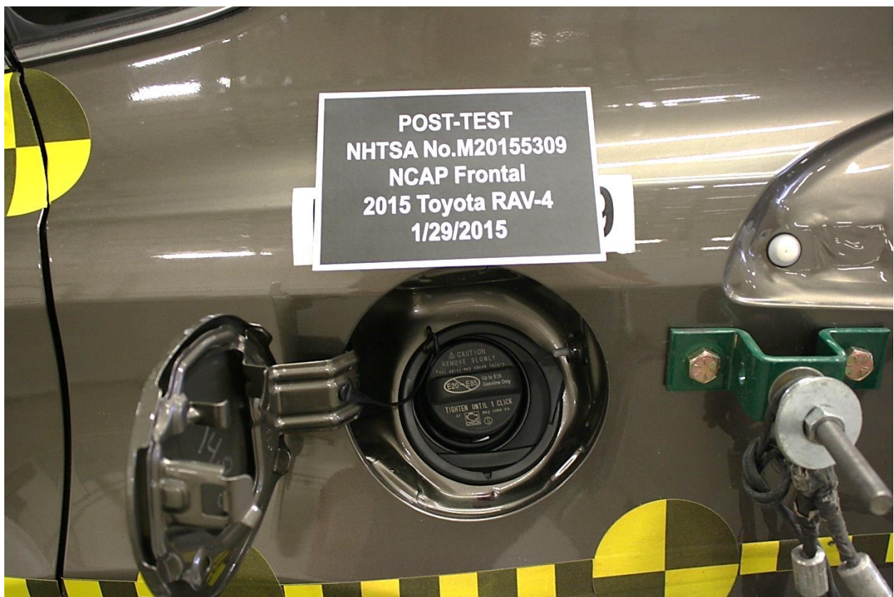
Figure A-22: Post-Test Fuel Filler Cap View
