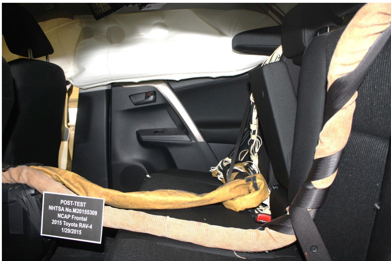
Figure A-28: Post-Test Dummy Cable Routing
