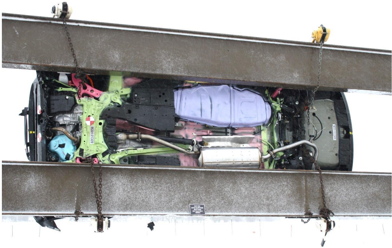
Figure A-75: Vehicle at 270° on Static Rollover Device
