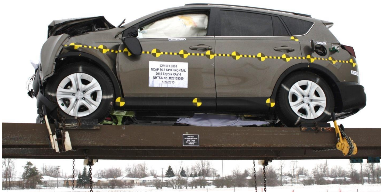
Figure A-76: Vehicle at 360° on Static Rollover Device
