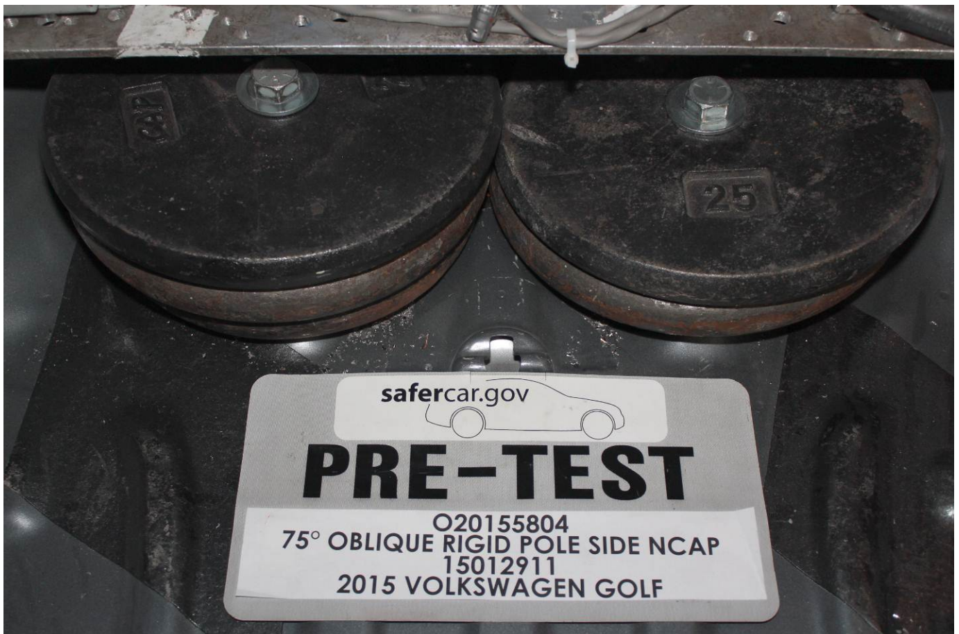
Pre-Test Ballast View
