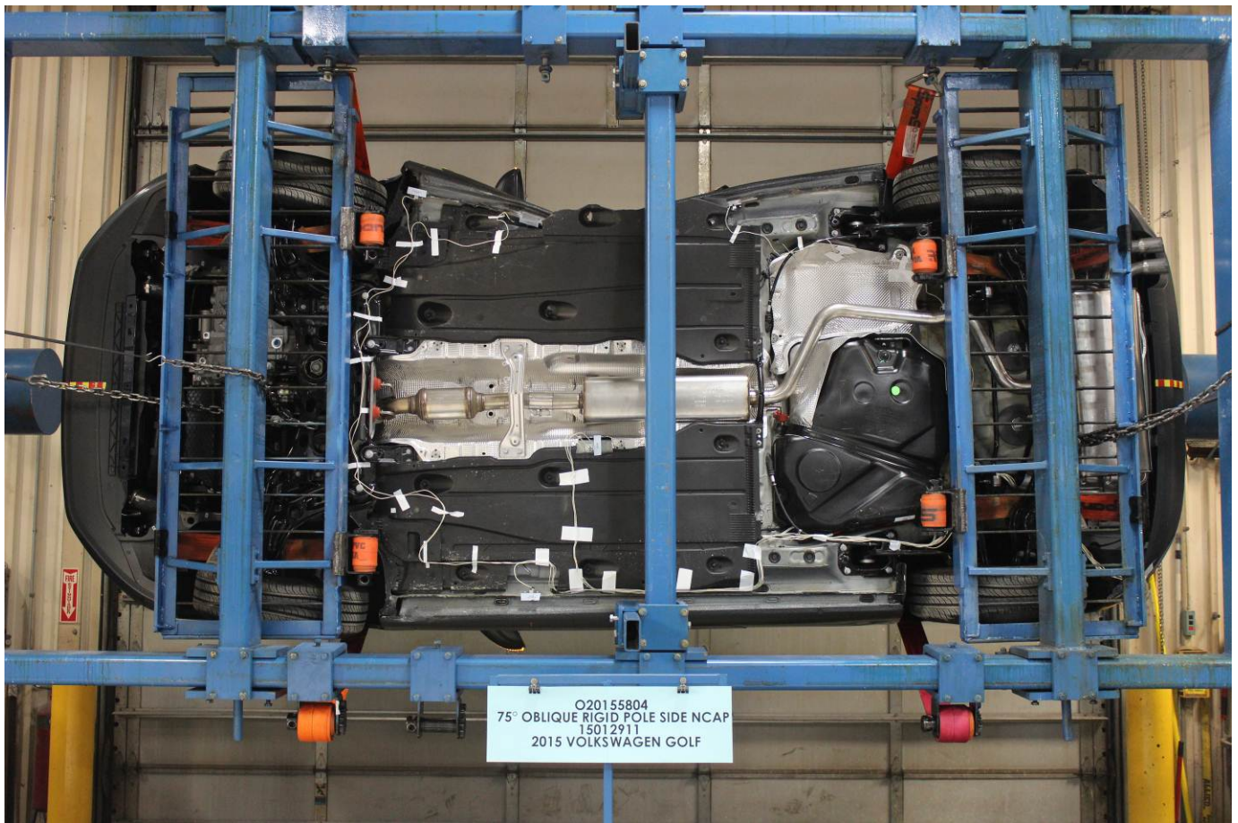
FMVSS No. 301 Static Rollover 90 Degrees
