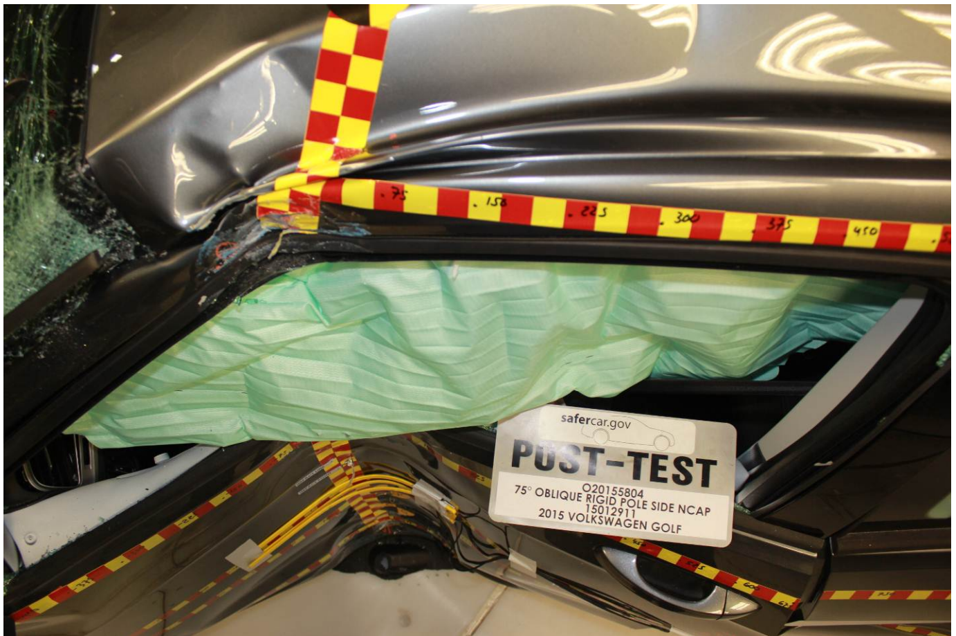
Post-Test Dummy and Door Clearance View
