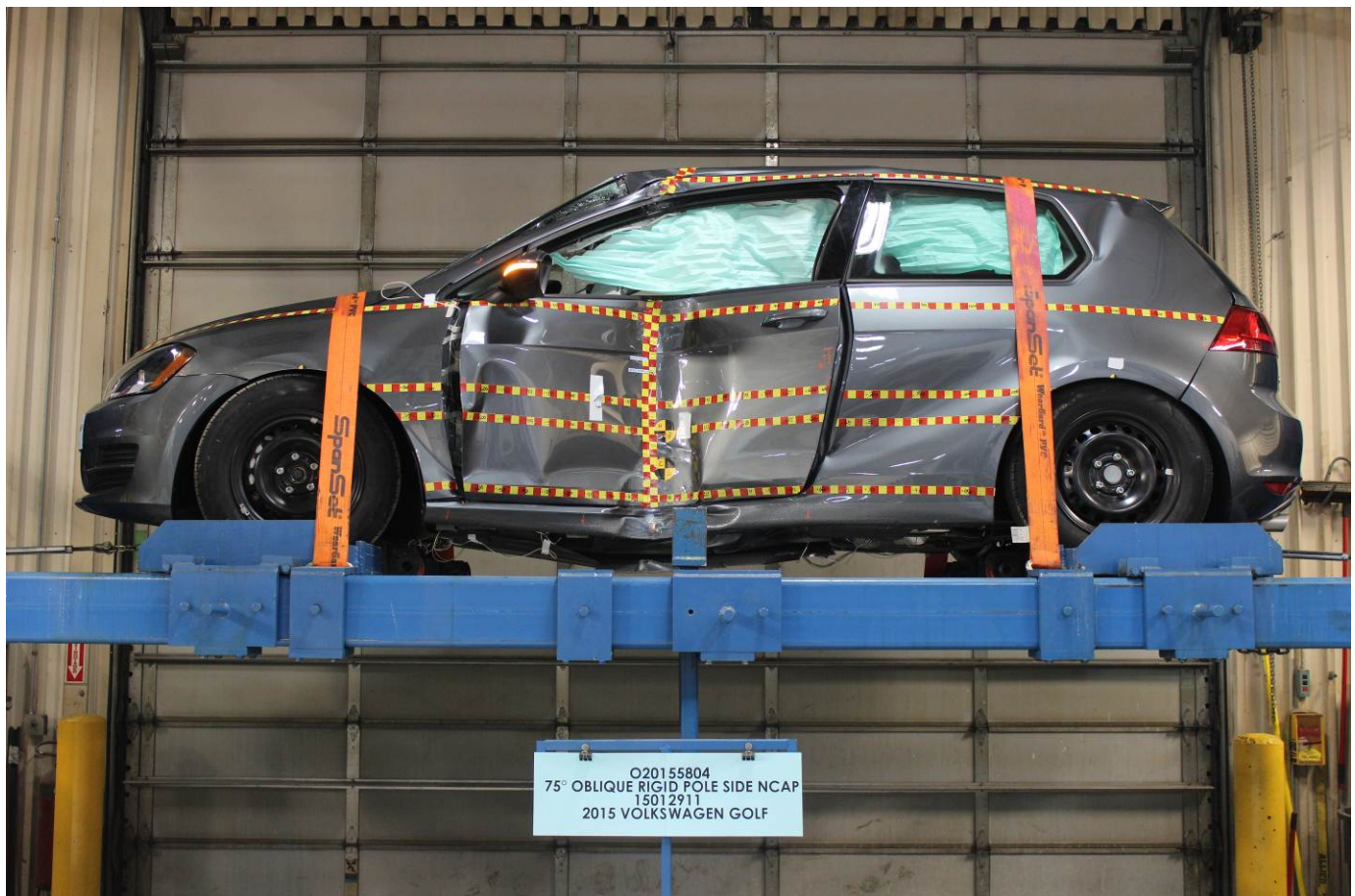
FMVSS No. 301 Static Rollover 0 Degrees
