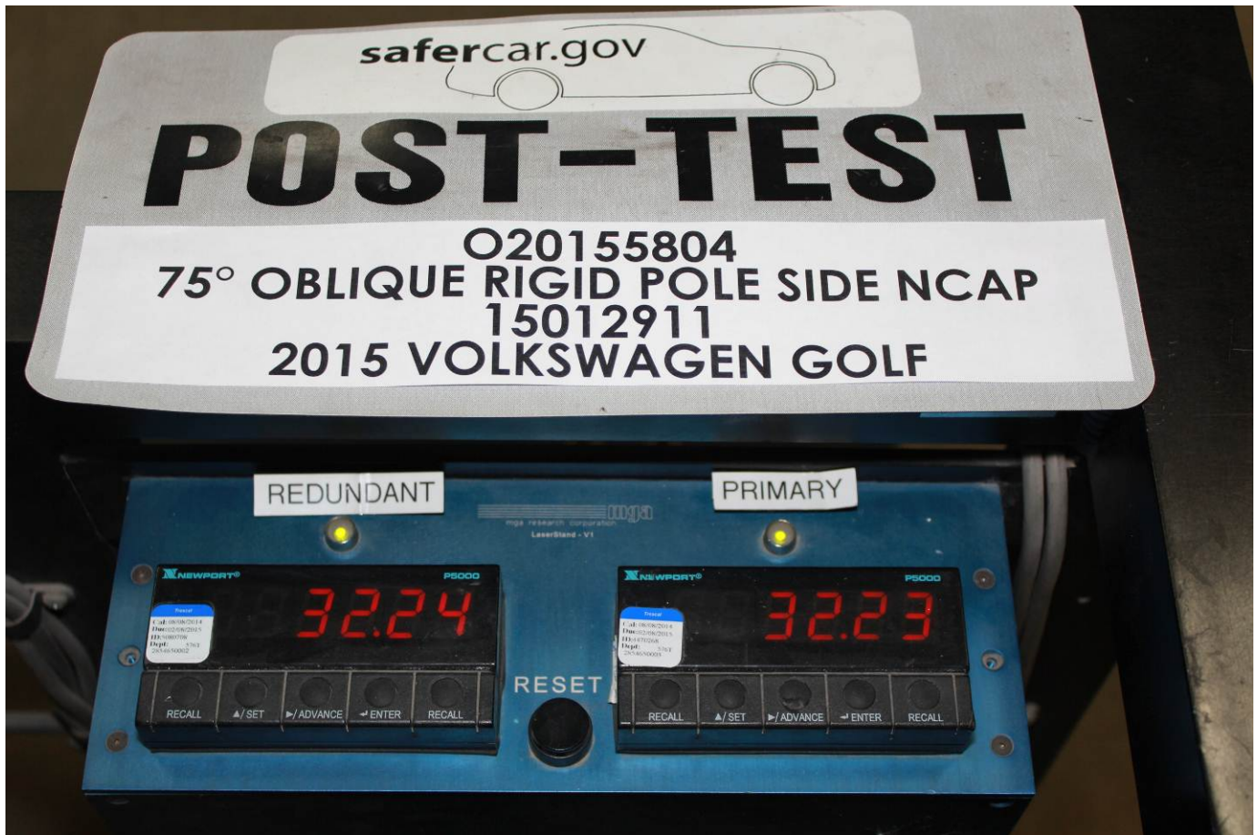
Post-Test Primary and Redundant Speed Trap Read-Out
