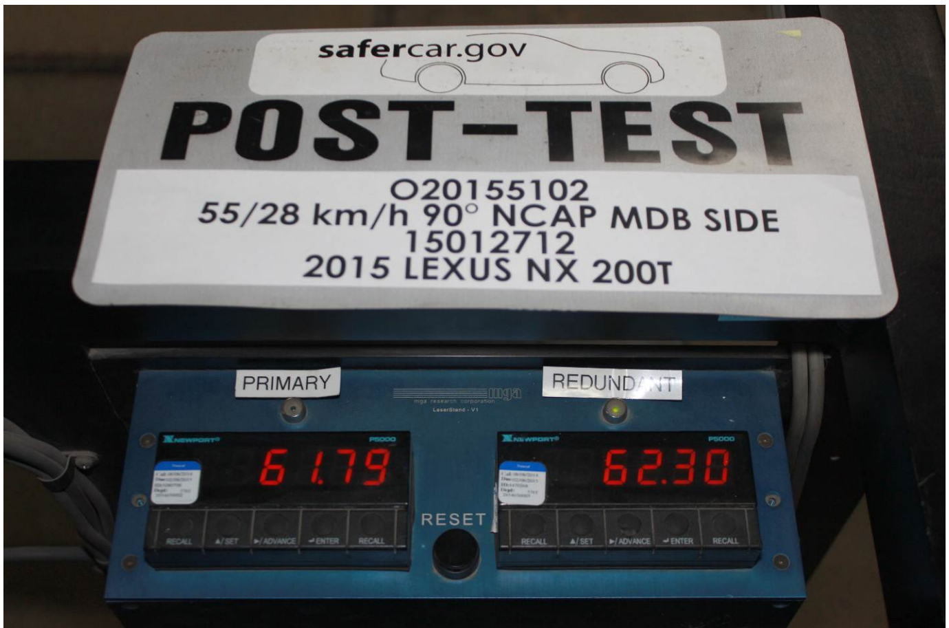
Post-Test Primary and Redundant Speed Trap Read-Out
