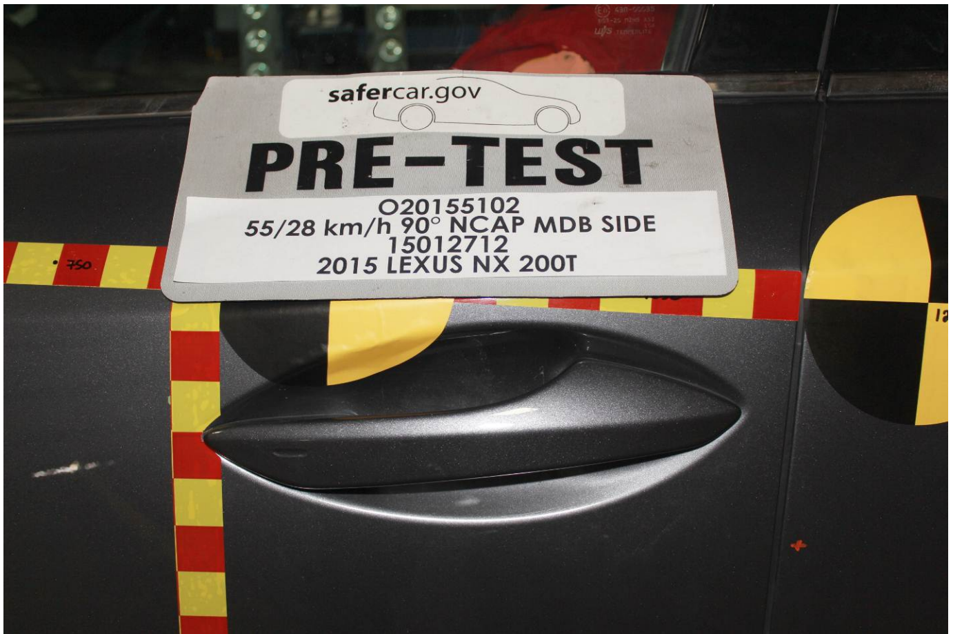
Pre-Test Left Front Door Latch Close-Up
