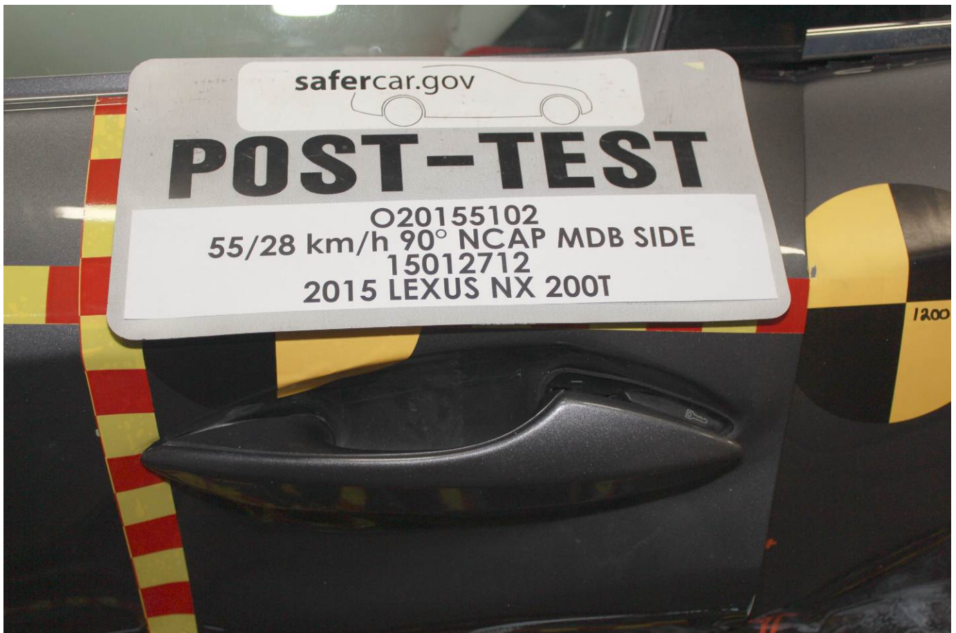
Post-Test Left Front Door Latch Close-Up
