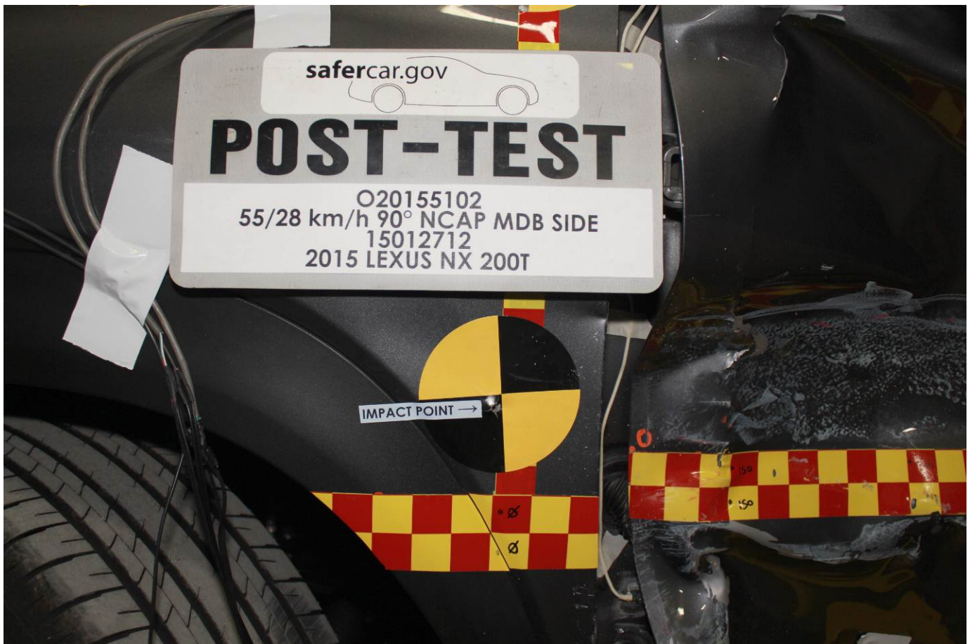
Post-Test Close-Up View of Impact Point Target
