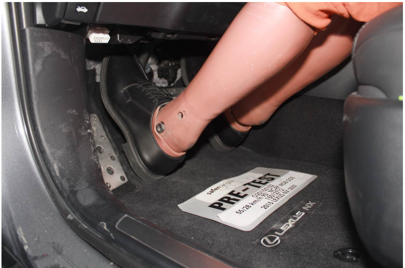
Pre-Test Placement of Driver Dummy's Feet
