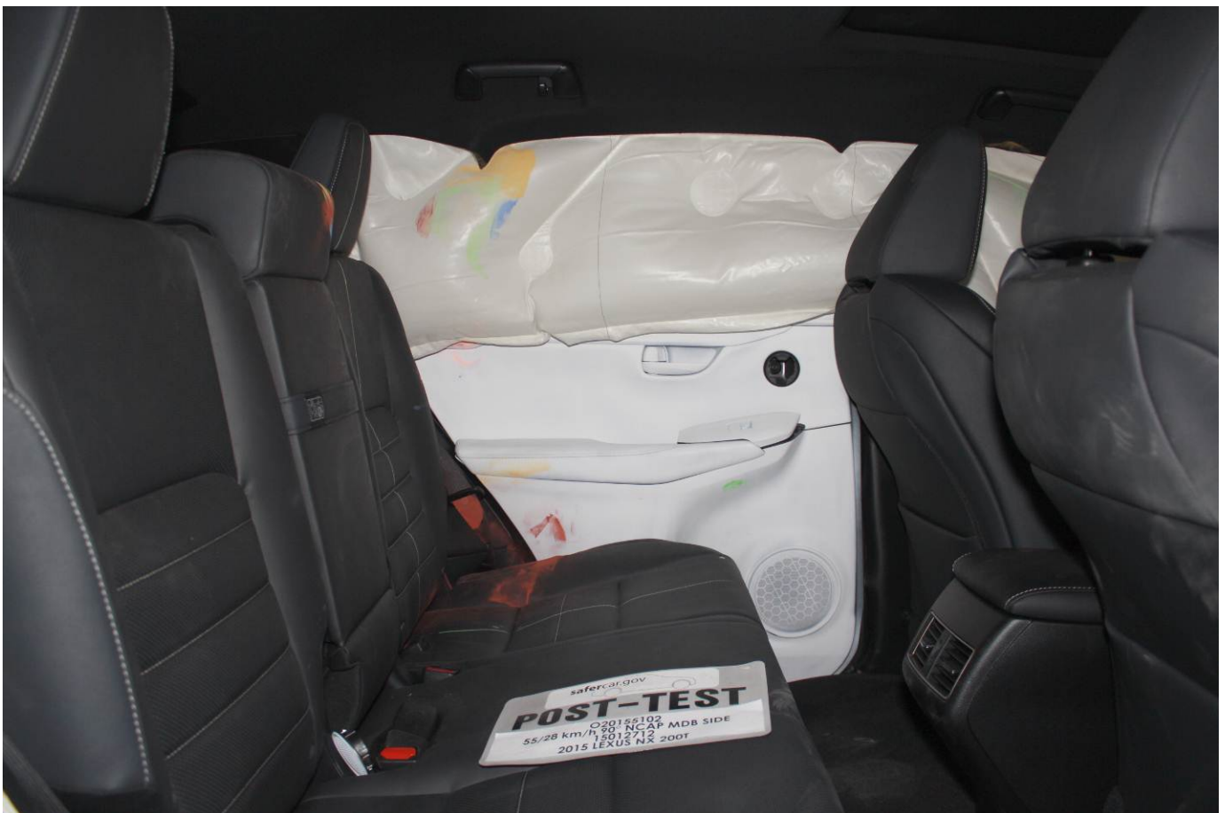
Post-Test Rear Passenger Inner Door Panel View
