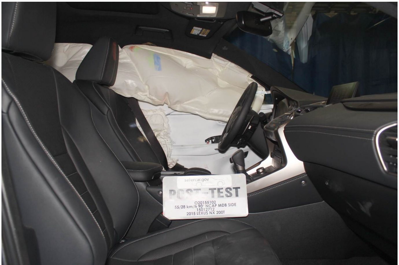
Post-Test Driver Inner Door Panel View
