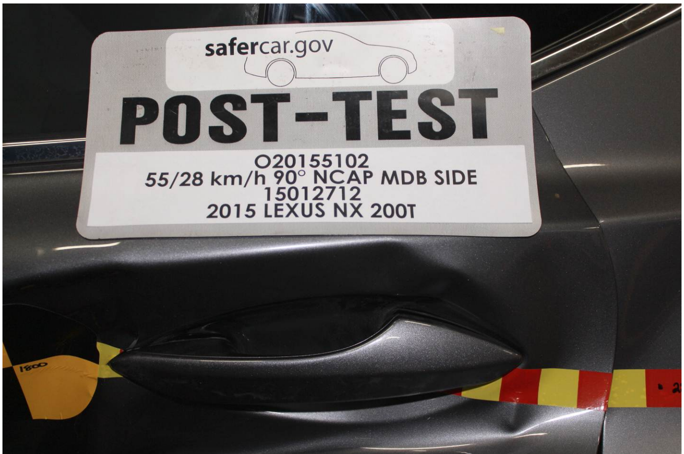
Post-Test Left Rear Door Latch Close-Up
