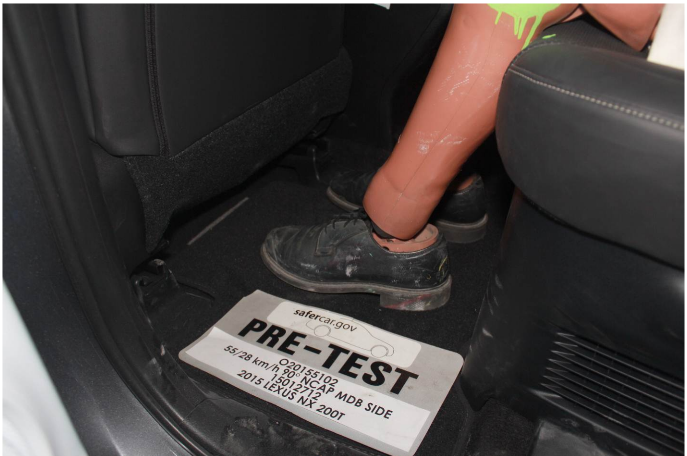
Pre-Test Placement of Rear Passenger Dummy's Feet
