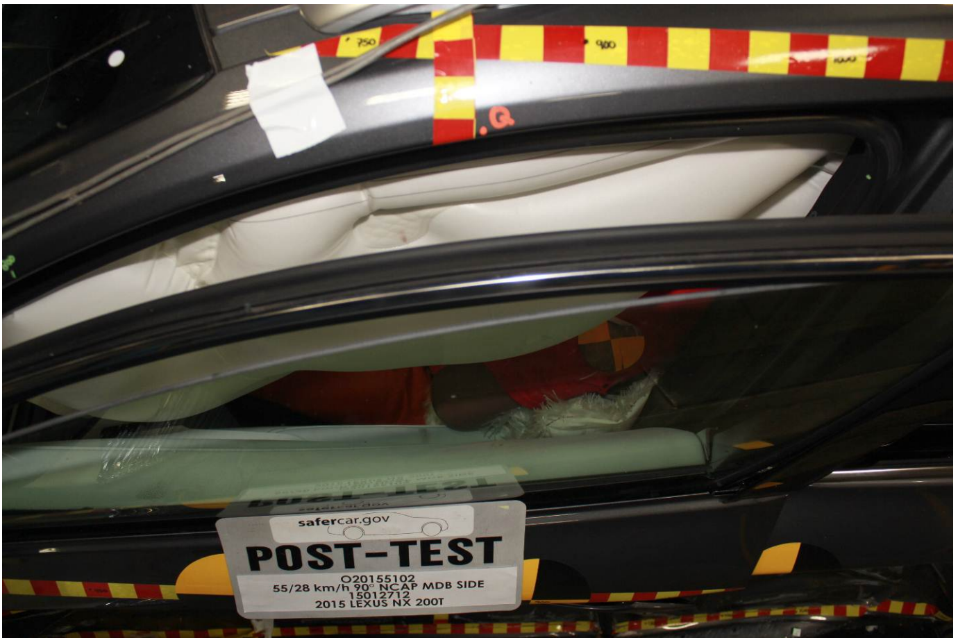
Post-Test Driver Dummy and Door Clearance View
