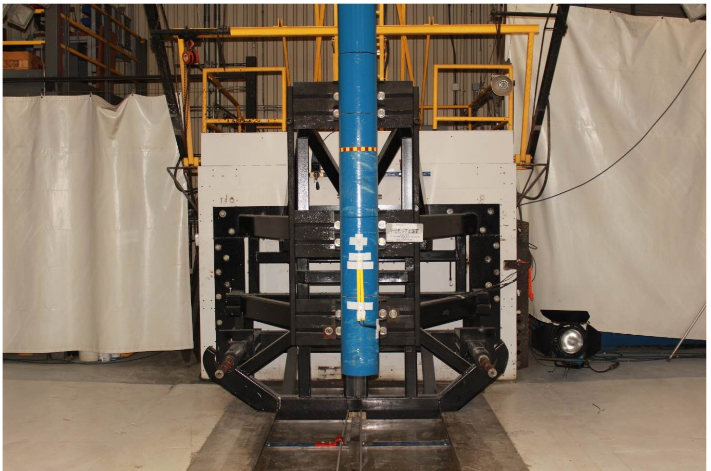
Pre-Test Pole Barrier Front View
