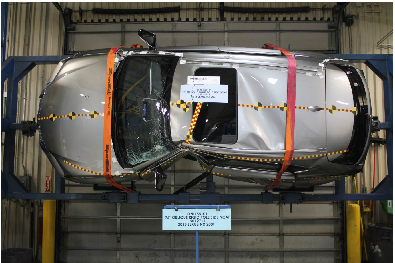
FMVSS No. 301 Static Rollover 90 Degrees
