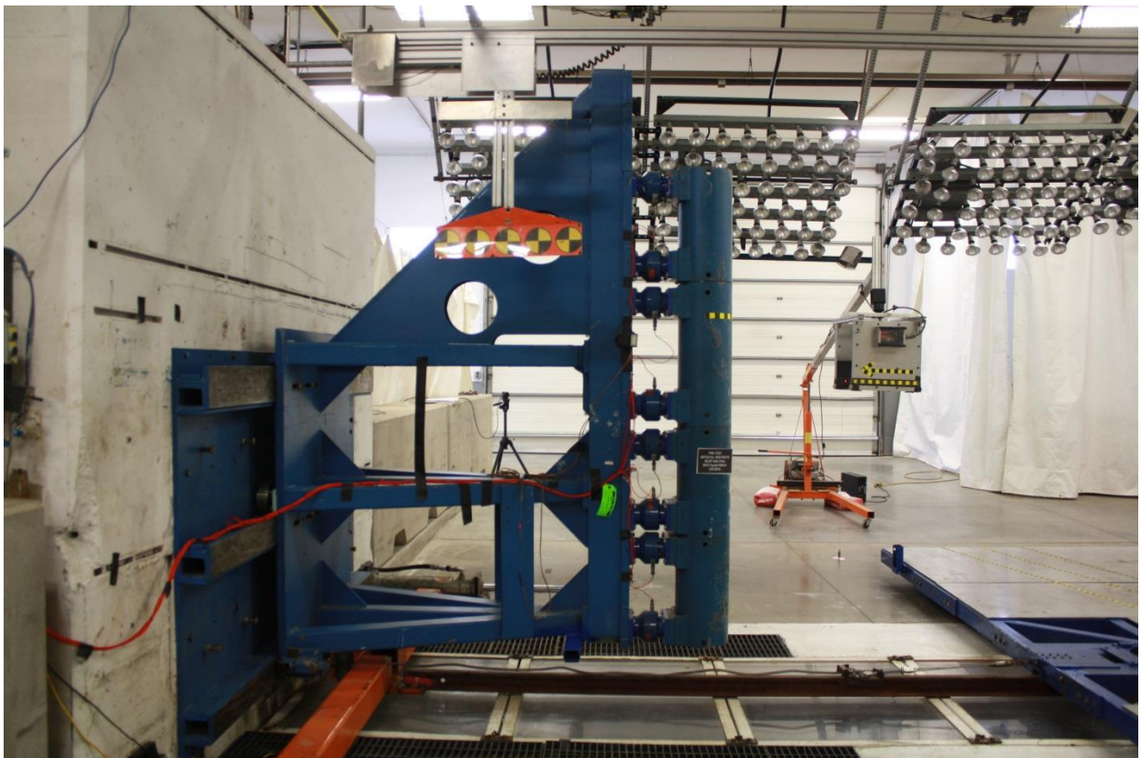
Figure A-59: Pre-Test Pole Barrier Side View
