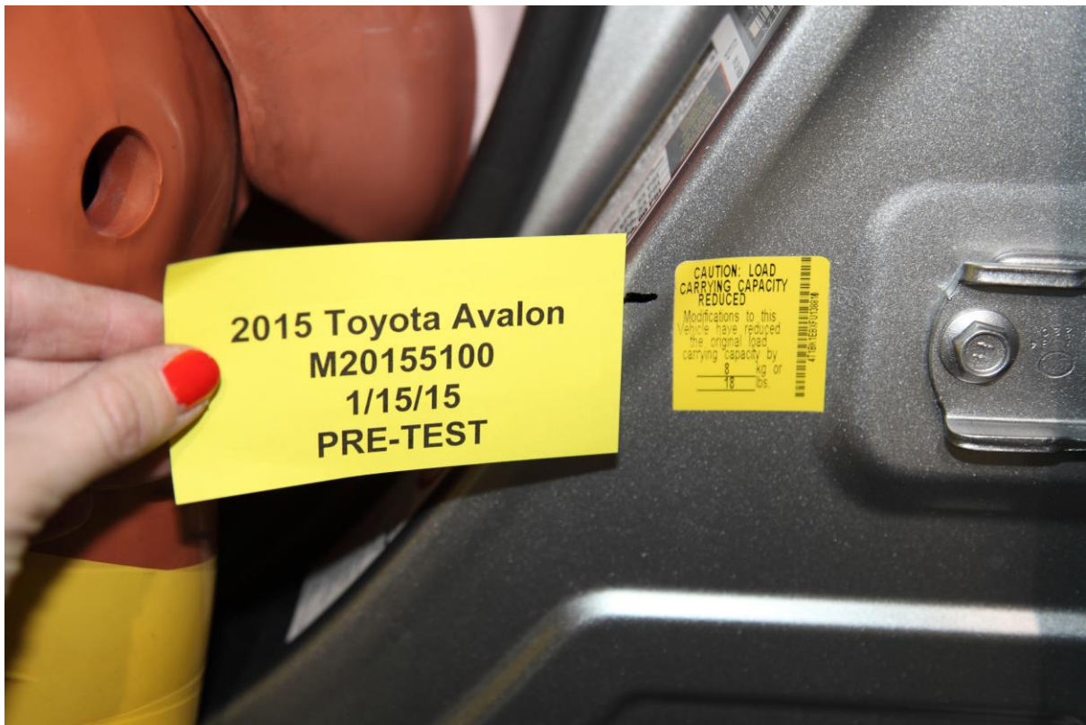
004a Reduced Load Carrying Capacity Label
