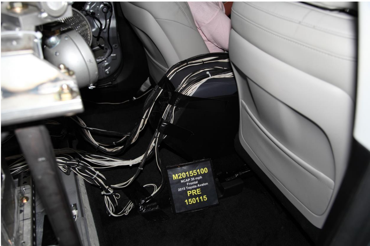
027 Pre-Test Dummy Cable Routing
