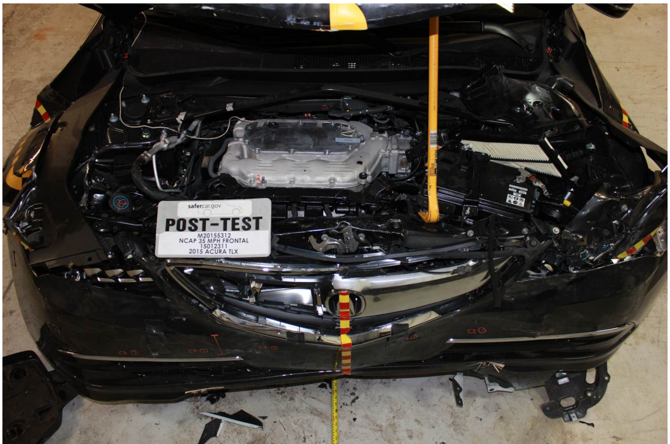
Post-Test Engine Compartment View
