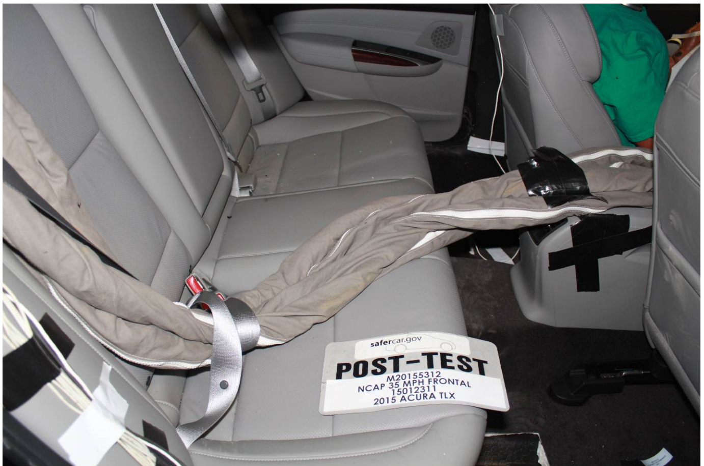
Post-Test Dummy Cable Routing
