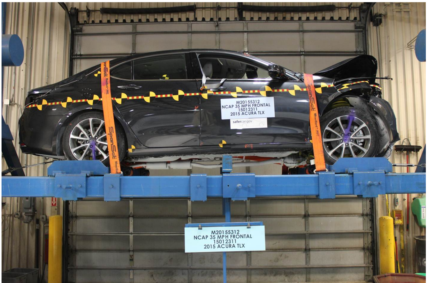
Vehicle at 360 Degrees on Static Rollover Device
