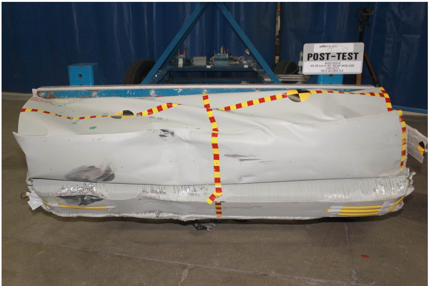
Post-Test Front View of MDB Impactor Face
