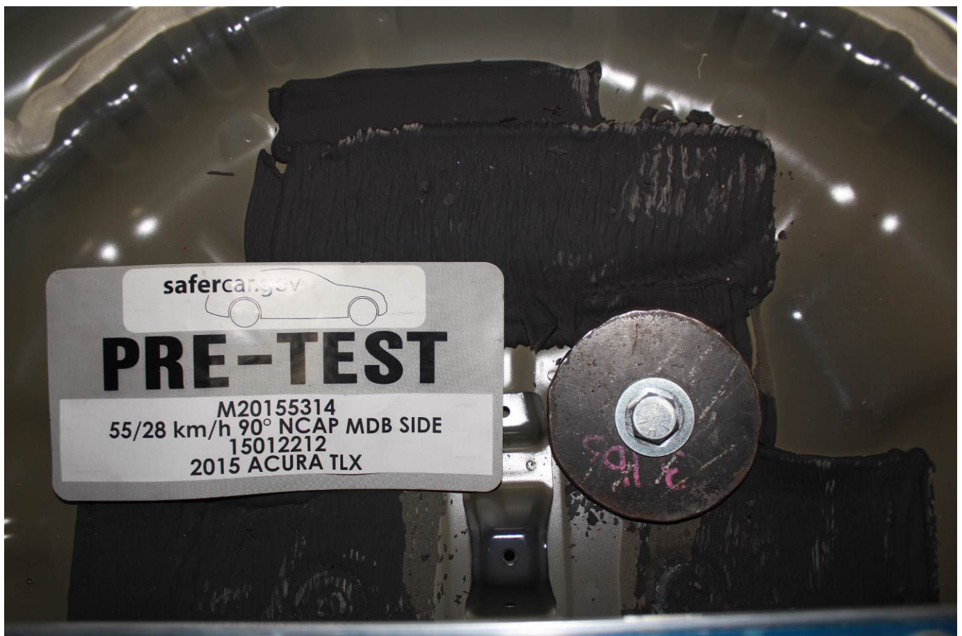
Pre-Test Ballast View
