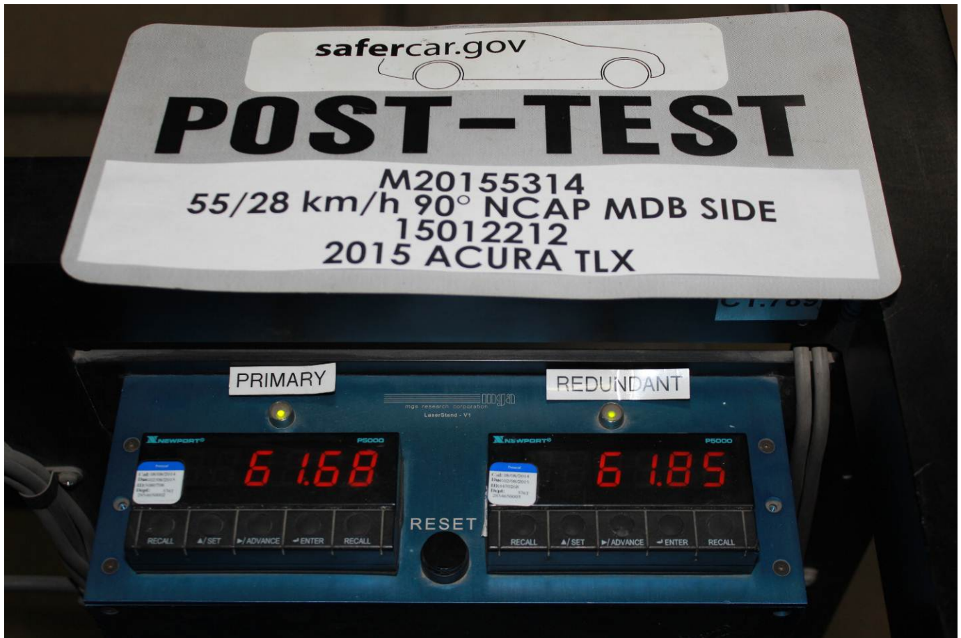
Post-Test Primary and Redundant Speed Trap Read-Out
