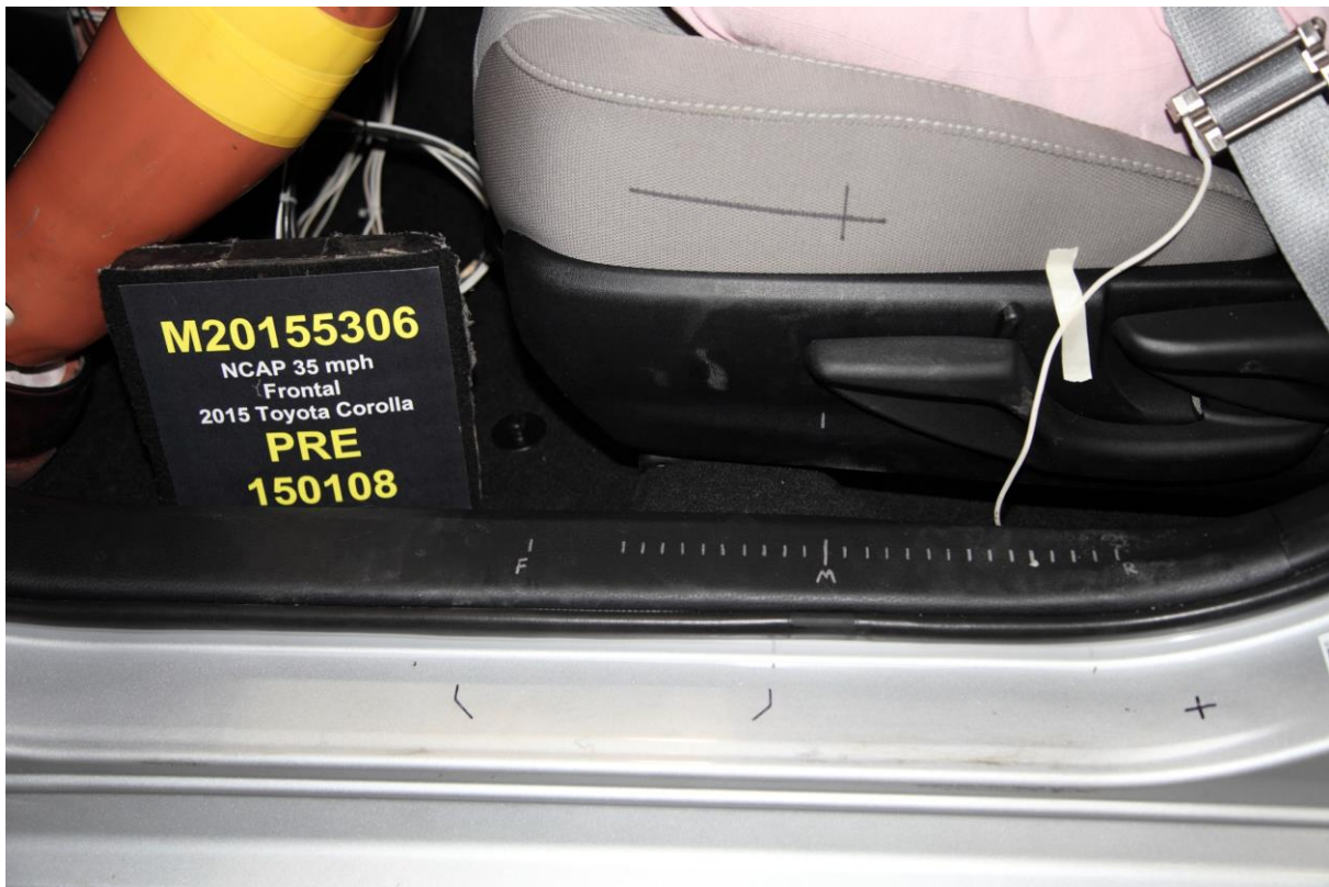
035 Pre-Test Driver's Seat Fore-Aft Markings
